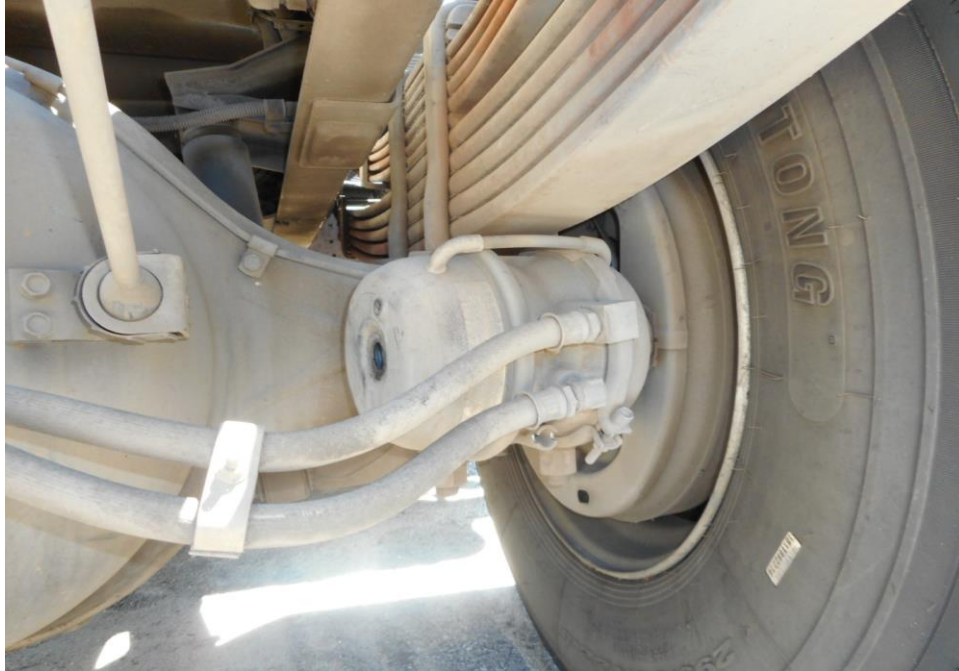
Photo 15 shows the brake pipe (arrowed) at the rear right wheel of the Prime Mover. I did not observe any leakage of brake fluid at the time of my inspection of the Prime Mover. My static tests of the Prime Mover's braking system, along with my visual examination of the various mechanical components in the braking system, had indicated that there was no internal leakage of pressure/vacuum. Hence the braking system of the Prime Mover was likely to be in serviceable condition at the material time of accident.
