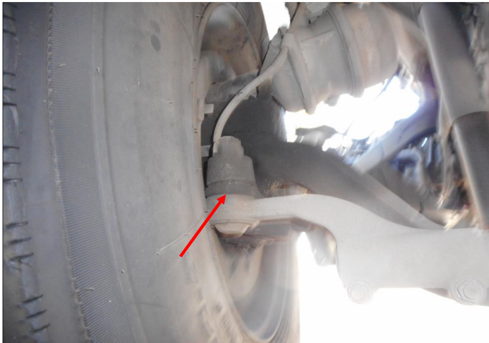
Photo 13 shows the various undercarriage components at the front left wheel of the Prime Mover, in particular the steering tie rod end (arrowed). The various undercarriage components of the Prime Mover were all found to be intact without any visible damage. There was also no sign of fluid stain(s) observed on the various undercarriage components.
