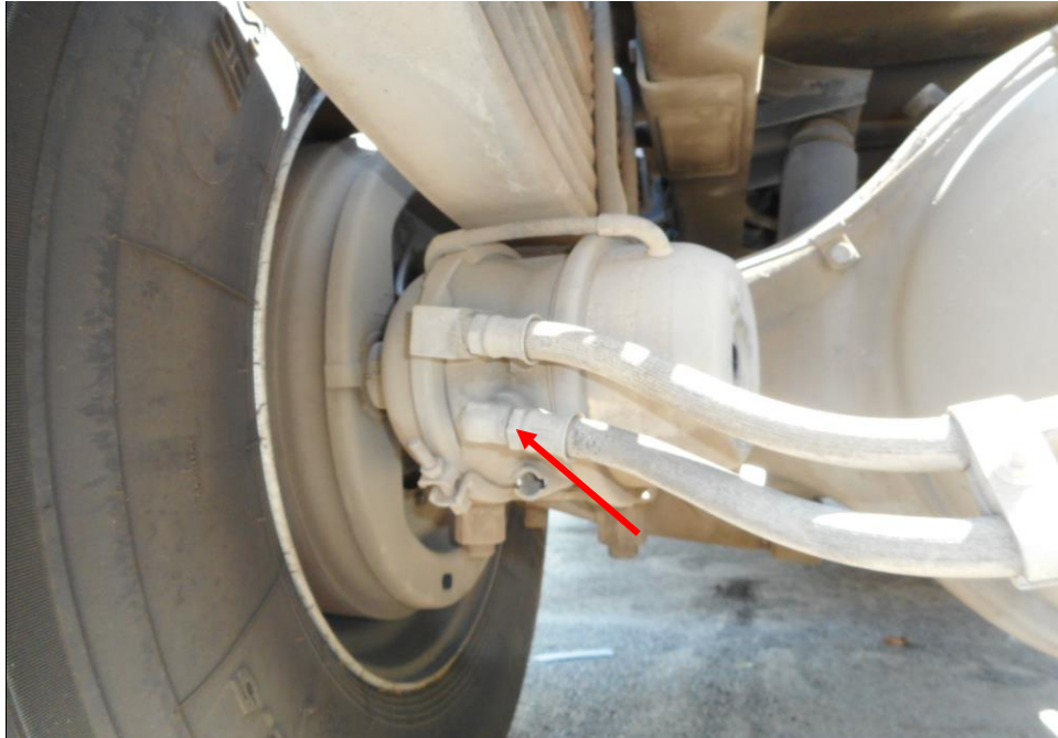
Photo 16 shows the brake pipe (arrowed) at the rear left wheel of the Prime Mover. I did not observe any leakage of brake fluid at the time of my inspection of the Prime Mover. My static tests of the Prime Mover's braking system, along with my visual examination of the various mechanical components in the braking system, had indicated that there was no internal leakage of pressure/vacuum. Hence the braking system of the Prime Mover was likely to be in serviceable condition at the material time of accident.
