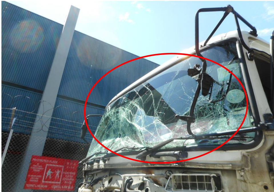
Photo 3 shows the close up view of the Prime Mover front body at the time of my inspection. The Prime Mover was observed to have sustained damage at its front windscreen (circled), as a result of the accident.
