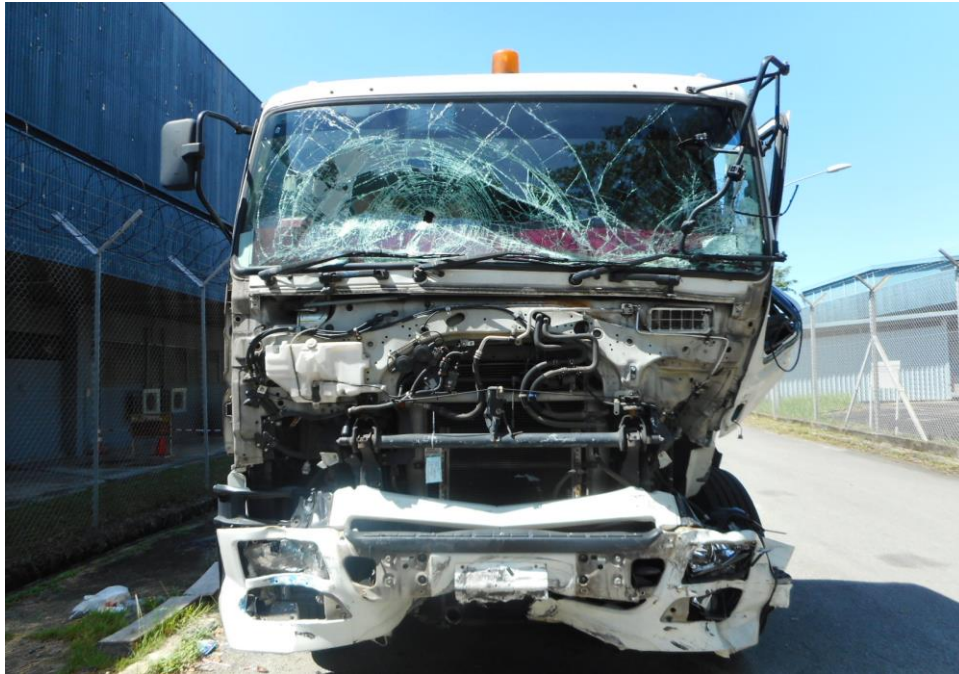
Photo 2 shows a general view of the front body of the Prime Mover at the time of my inspection. The Prime Mover was observed to have sustained damage at its frontal portion. Its front windscreen, front body panel and engine components were amongst the body parts that were damaged as a result of the accident.
