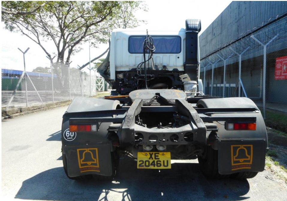
Photo 1 shows a general view of the Prime Mover's rear body at the time of my inspection. There was no damage found to the rear portion of the Prime Mover.
