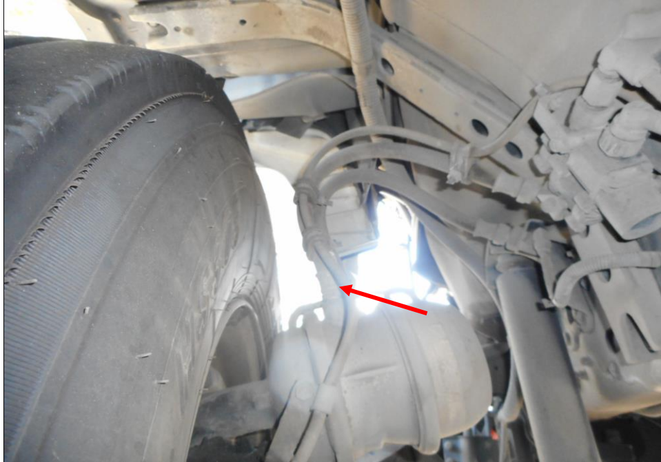
Photo 17 shows the brake pipe (arrowed) at the front left wheel of the Prime Mover. I did not observe any leakage of brake fluid at the time of my inspection of the Prime Mover. My static tests of the Prime Mover's braking system, along with my visual examination of the various mechanical components in the braking system, had indicated that there was no internal leakage of pressure/vacuum. Hence the braking system of the Prime Mover was likely to be in serviceable condition at the material time of accident.
