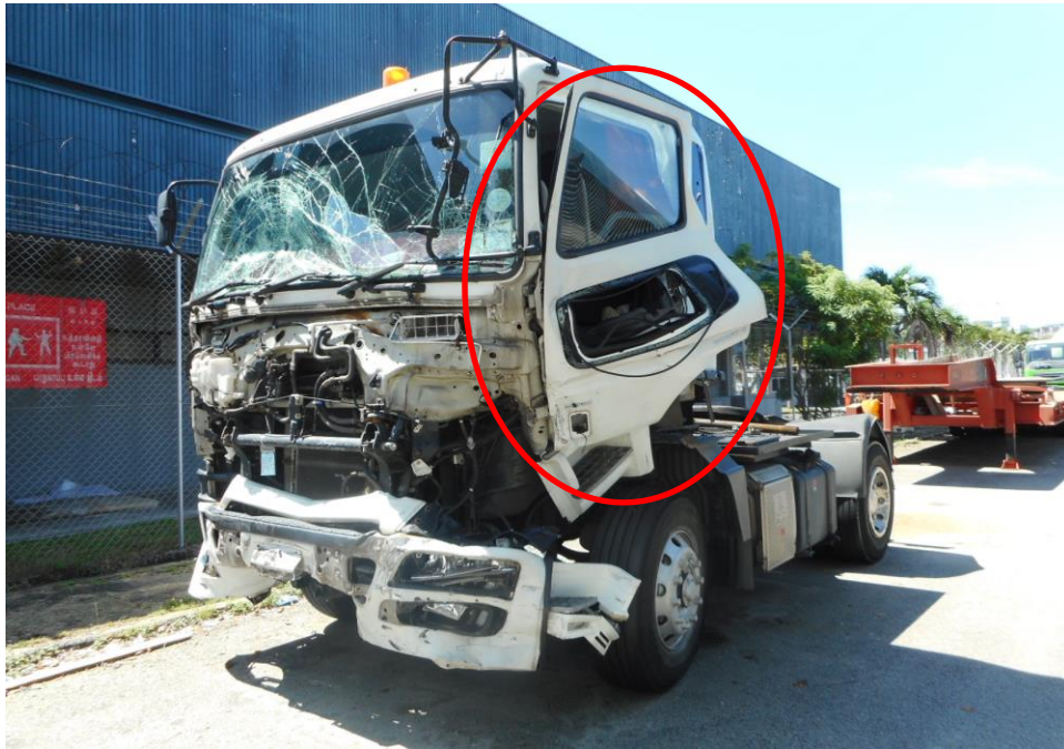
Photo 6 shows a general view of the front right body of the Prime Mover at the time of my inspection, the right door (circled) was observed to have been damaged by the accident.
