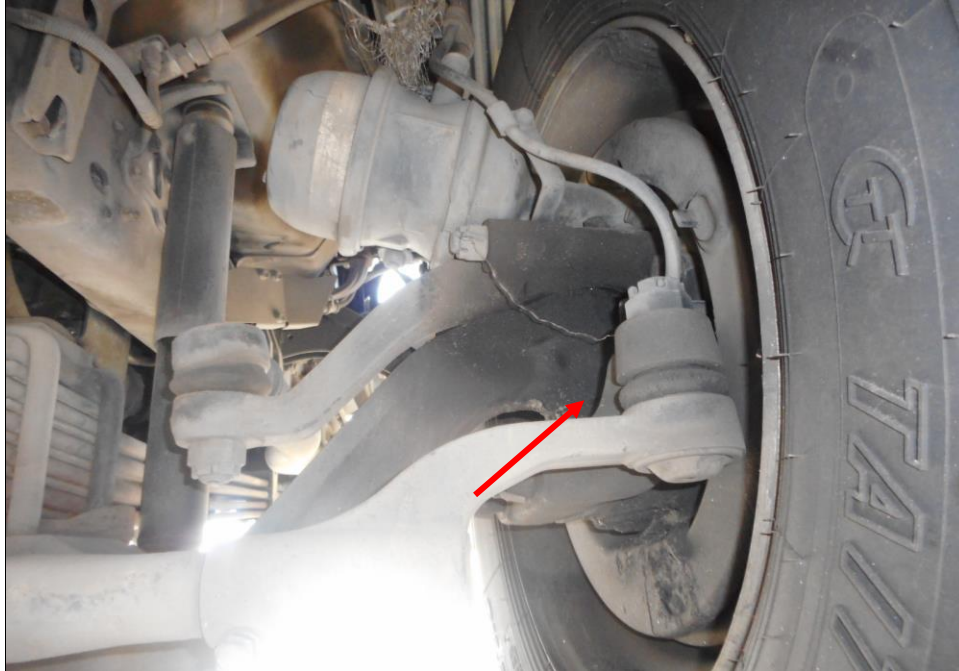
Photo 12 shows the various undercarriage components at the front right wheel of the Prime Mover, in particular the steering tie rod end (arrowed). The various steering components were all found to be intact, suggesting that the steering system of the Prime Mover was likely to be in serviceable condition at the material time of accident. There was also no sign of fluid stain(s) observed on the various undercarriage components.
