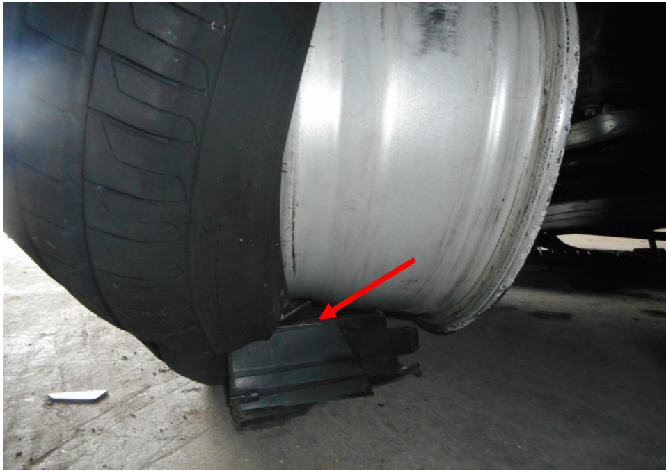
Photo 14 shows the condition of the front left tyre and rim of the Motor Car, which was observed that rim (arrowed) had likely caused cut on the tyre in the midst of the accident due to the impact it sustained from the collision.
