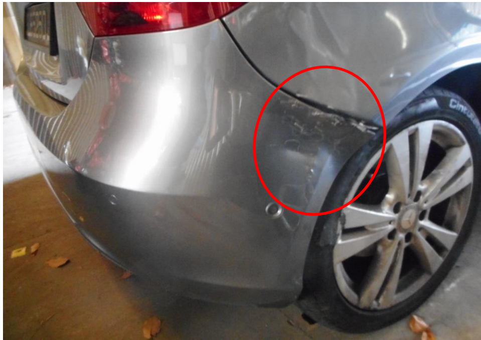
Photo 8 shows the close up view of the Motor Car's rear body at the time of my inspection, its rear bumper (circled) were amongst the body parts that were damaged as a result of the accident.
