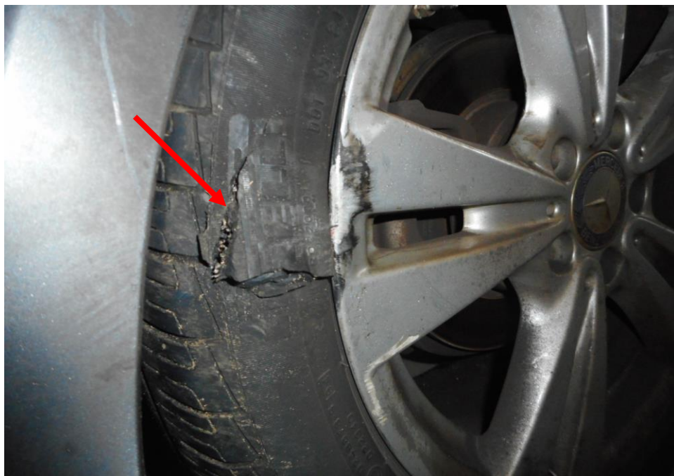
Photo 11 shows the close up condition of the rear right tyre and rim of the Motor Car, which was observed that rim (arrowed) had likely caused cut on the tyre in the midst of the accident due to the impact it sustained from the collision.
