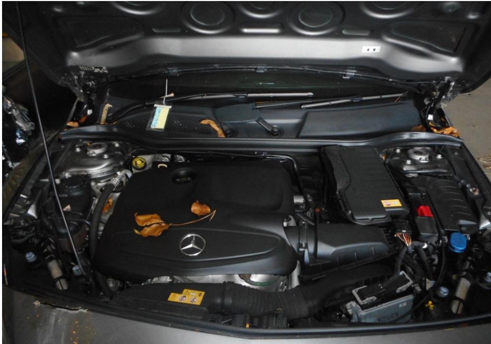
Photo 15 shows a general view of the Motor Car's engine compartment. I had observed the brake fluid and engine coolant were all found to be of sufficient level for operating purposes. Visually, there was also no contamination found to these fluids. However, the engine oil was found to be insufficient due to the damaged to the undercarriage oil sump which had caused the engine oil to flow out as a result of the accident.
