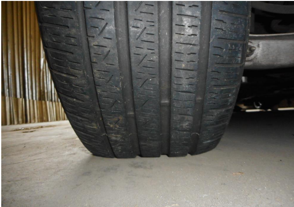
Photo 12 shows the condition of the rear left tyre of the Motor Car, which was observed to be in serviceable condition with remaining tread depth of approximately 4.4mm. There was also no tear, cut or burst mark(s) on the outer and the inner sidewalls as well as across the tread of the Motor Car's rear left tyre.
