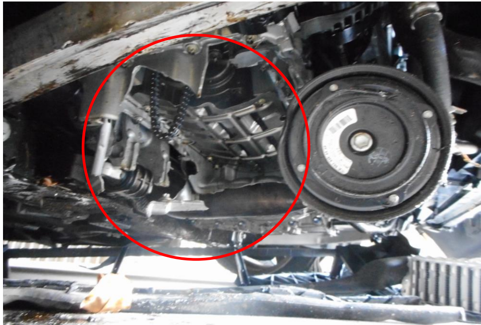
Photo 19 shows the undercarriage of the Motor Car, at the area where the engine housing and transmission housing are located. I did find any sign(s) or indication(s) of fluid leak and/or fluid stain(s) due to the damaged to the undercarriage engine oil sump (circled) on the underside of the Motor Car as a result of the accident.
