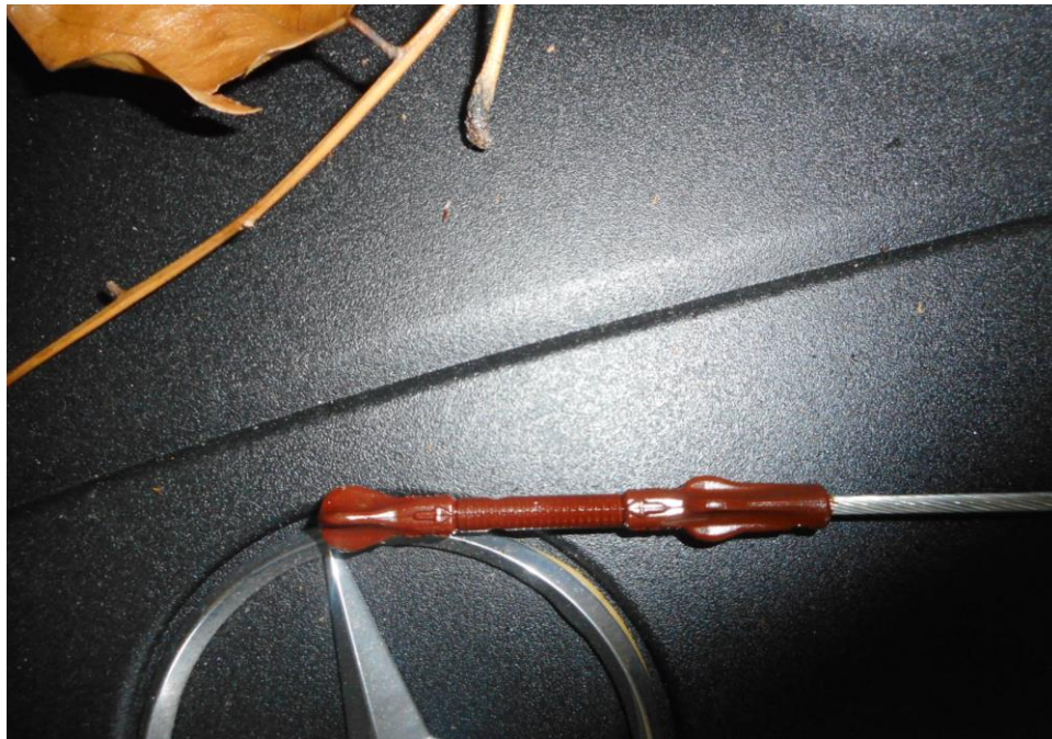
Photo 18 shows the engine oil dip stick of the Motor Car at the time of my inspection. The engine oil was observed to be of insufficient level due to the damaged the undercarriage engine oil sump which caused the coolant to flow out.
