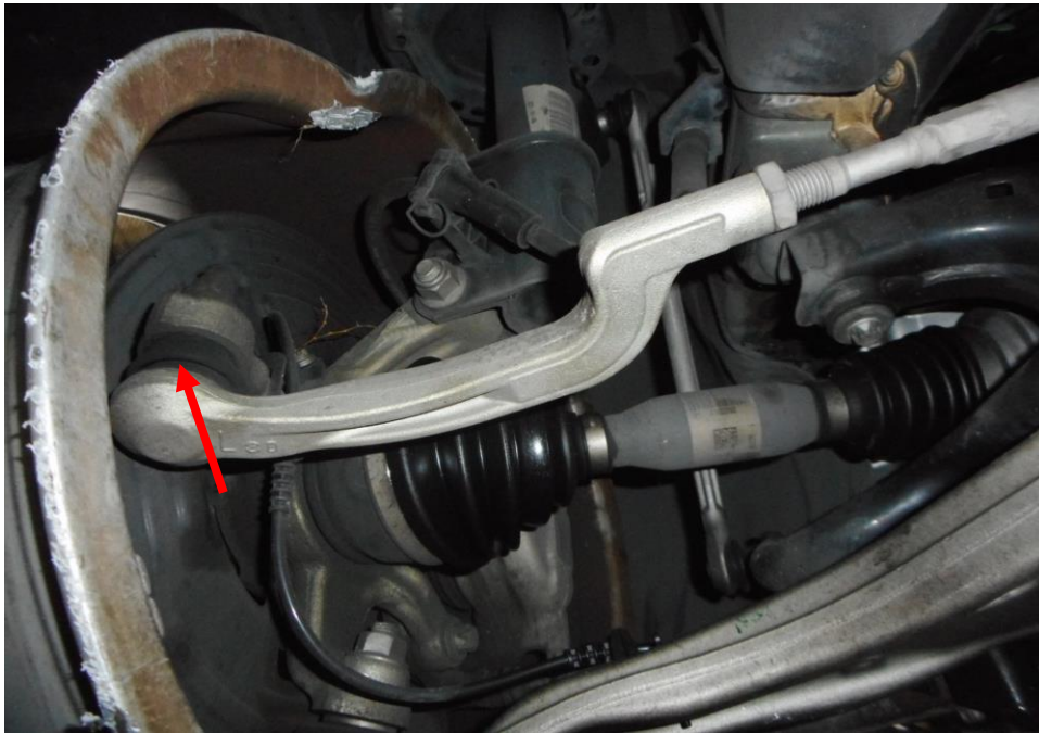
Photo 25 shows the various undercarriage components at the front left wheel of the Motor Car, the steering tie rod (red arrow) the various steering components were all found to be intact, suggesting that the steering system of the Motor Car was likely to be in serviceable condition at the material time of accident. There was also no sign of fluid stain observed on the various undercarriage components at the front left wheel of the Motor Car.
