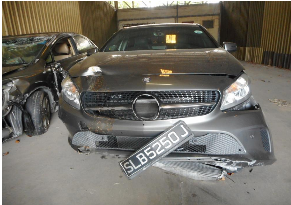
Photo 2 shows a general view of the Motor Car's front body at the time of my inspection. The Motor Car was observed to have sustained damage at its front portion. Its front bonnet, front bumper, front fender and its rear bumper were amongst the body parts that were damaged as a result of the accident.
