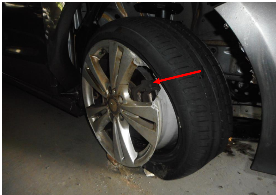
Photo 9 shows the condition of the front right tyre of the Motor Car, which was observed to be in unserviceable condition as it was damaged (arrowed) as a result of the accident with remaining tread depth of approximately 8.1mm.
