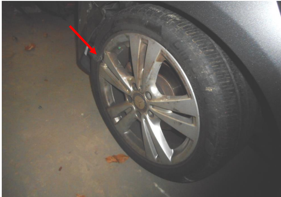
Photo 10 shows the condition of the rear right tyre of the Motor Car, which was observed to be in unserviceable condition as it was damaged (arrowed) as a result of the accident with remaining tread depth of approximately 4.3mm.
