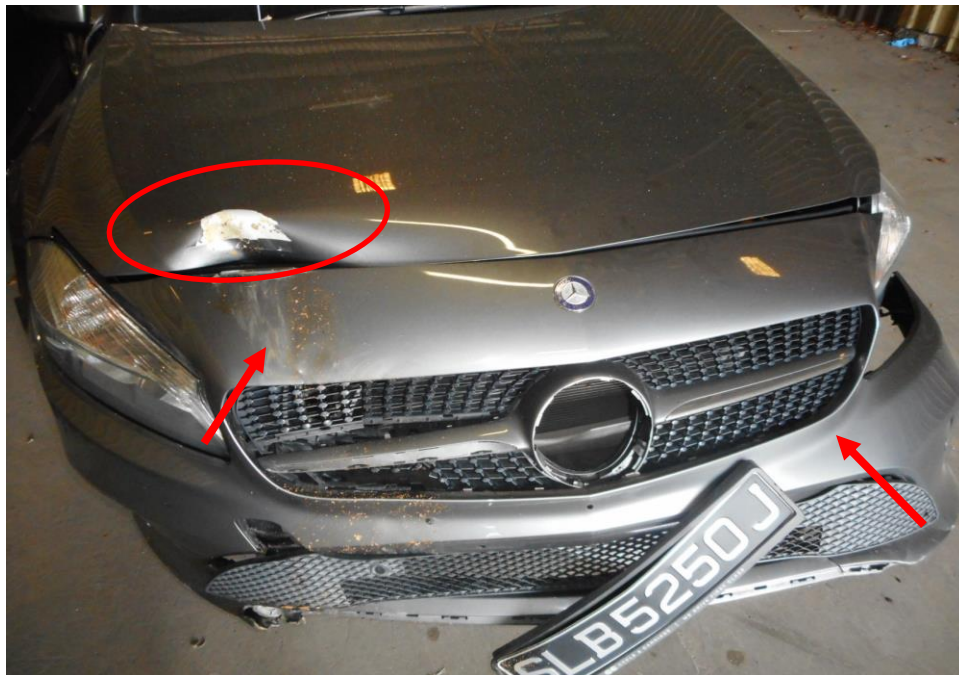
Photo 3 shows a close up view of the Motor Car's front body at the time of my inspection. Its front bonnet (circled), front bumper (arrowed), were amongst the body parts that were damaged as a result of the accident.
