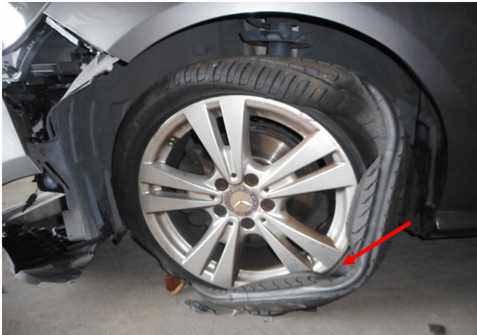
Photo 13 shows the condition of the front left tyre of the Motor Car, which was observed to be in unserviceable condition as it was damaged (arrowed) as a result of the accident with remaining tread depth of approximately 8.2mm.
