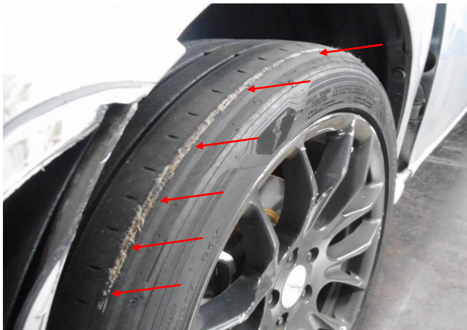
Photo 12 shows the front left tyre of the insured vehicle at the time of my inspection. The rubber compound at the outer side of the tread, around its entire circumference, was observed to be completely worn, exposing the reinforcing belts (arrowed) that are found within the mentioned tyre.
