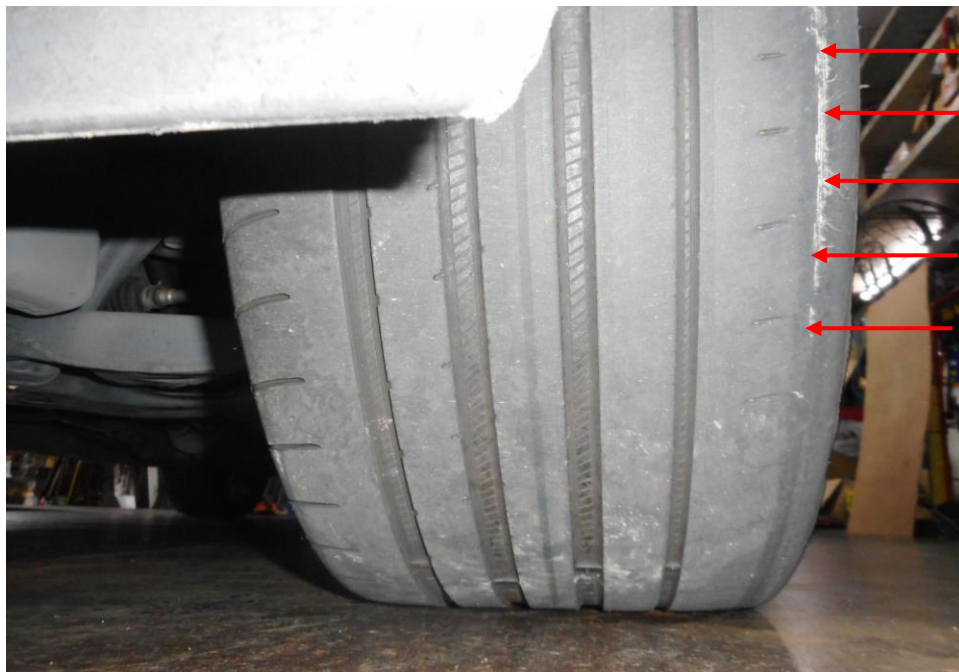
Photo 11 shows the front left tyre of the insured vehicle at the time of my inspection. The rubber compound at the inner side of the tyre, around its entire circumference, was observed to be completely worn, exposing the reinforcing belts (arrowed) that are found within the mentioned tyre.
