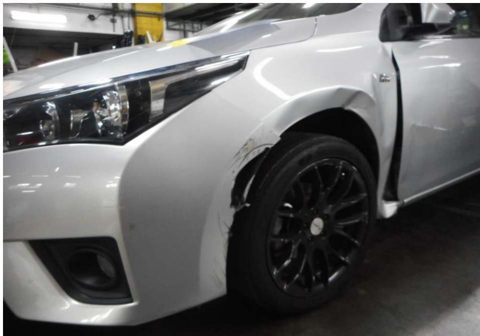
Photo 5 shows the close up view of the left front portion of the insured vehicle at the time of my inspection. Its bumper, body panel, fender and rims was observed to be damaged as a result of the accident.
