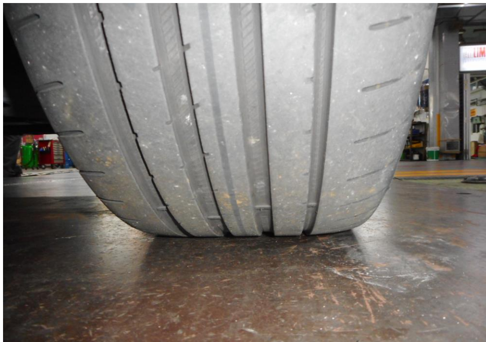
Photo 9 shows the front right tyre of the insured vehicle at the time of my inspection. The front right tyre of the insured vehicle was observed to be in serviceable condition.
