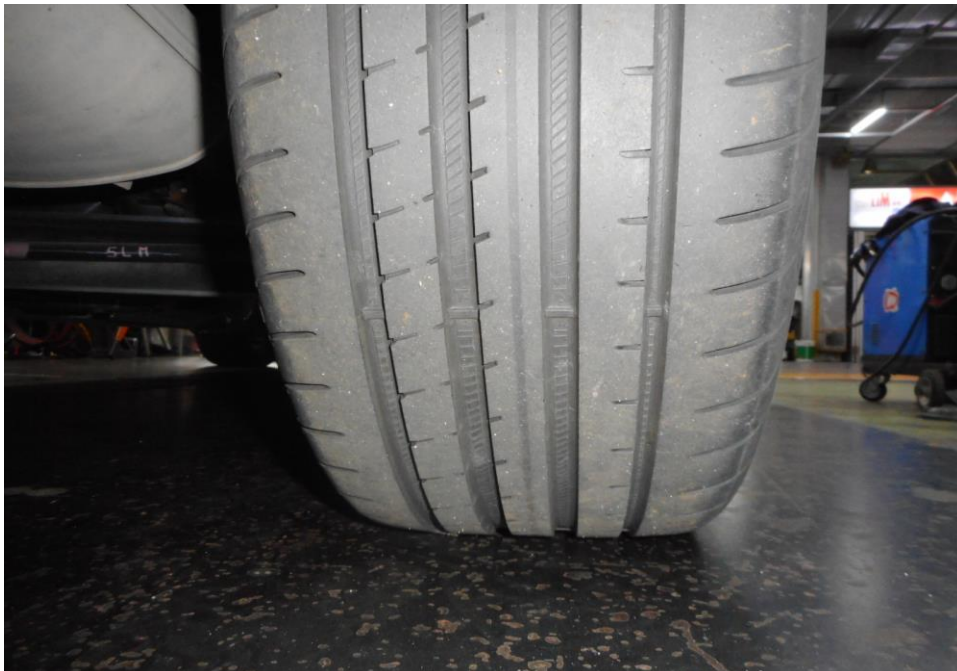
Photo 8 shows the rear right tyre of the insured vehicle at the time of my inspection. The rear right tyre of the insured vehicle was observed to be in serviceable condition.
