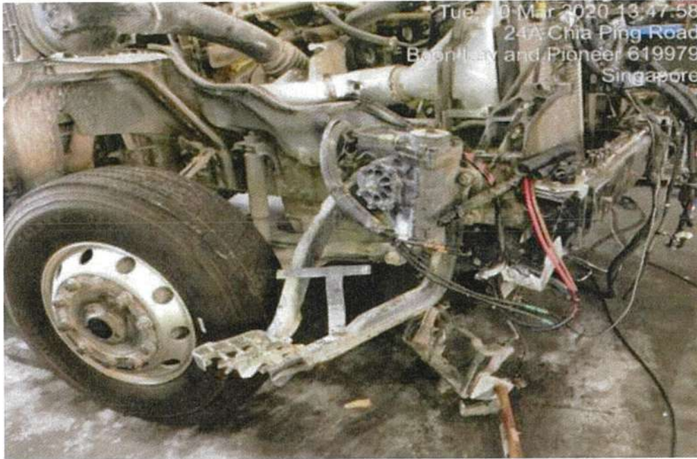
Photo 21 SNAPPED WIRE HARNESS & BENT LOWER STEPS
