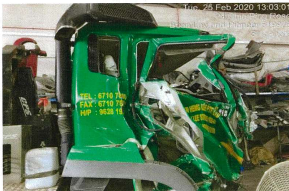
Photo 6 CRUSHED RH SIDE OF CABIN
