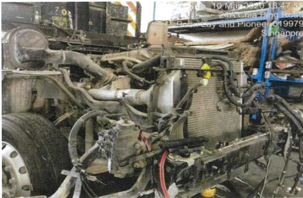
Photo 22 BROKEN AIR FILTER HOUSING
