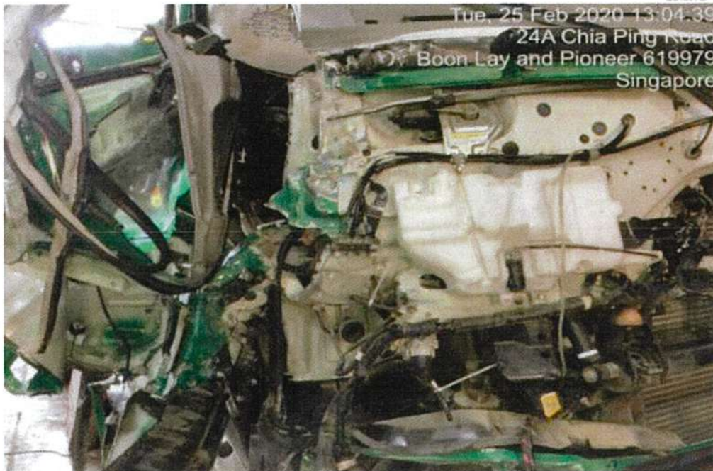
Photo 13 SNAPPED WIPER LINKAGE
