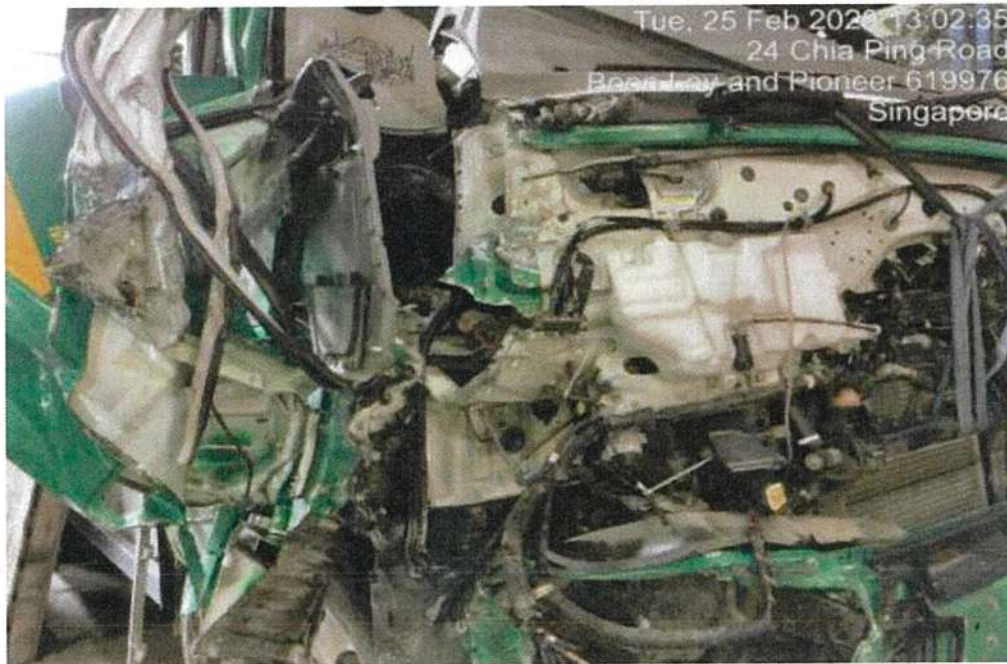
Photo 12 SHEARED FIRE WALL & DEFORMED DASHBOARD
