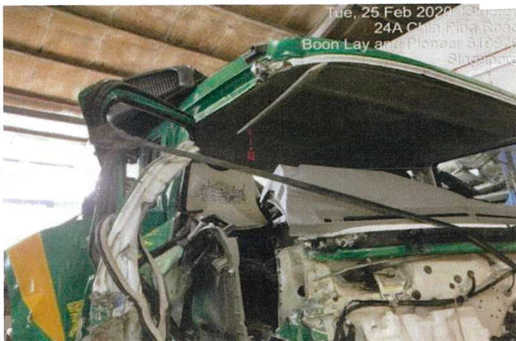
Photo 7 SHEARED RH PILLAR & FIREWALL
