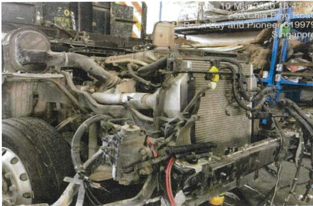
Photo 22 BROKEN AIR FILTER HOUSING
