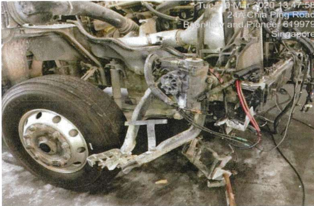
Photo 21 SNAPPED WIRE HARNESS & BENT LOWER STEPS
