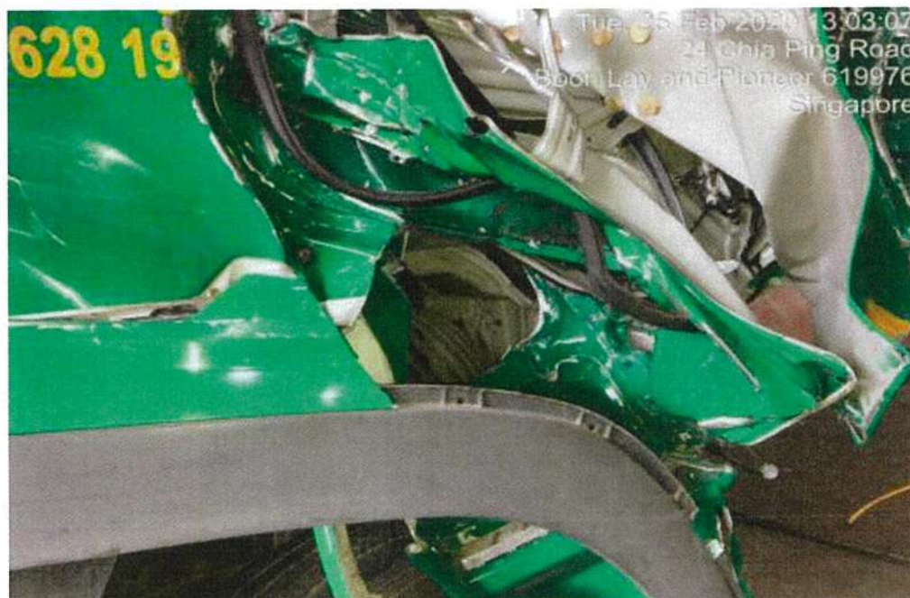
Photo 8 CRUSHED DOOR & DOOR COMPONENTS
