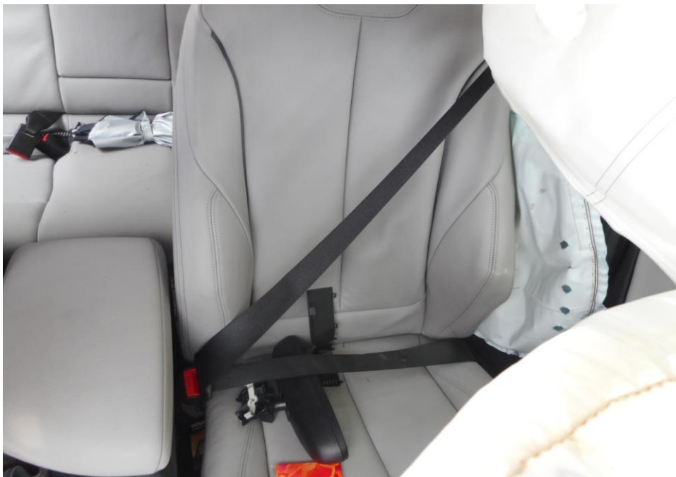
Photo 25 shows that the seat belt on the left seat were able to be fastened securely into the respective pre-tensioners that were fitted at the sides of each seat.
