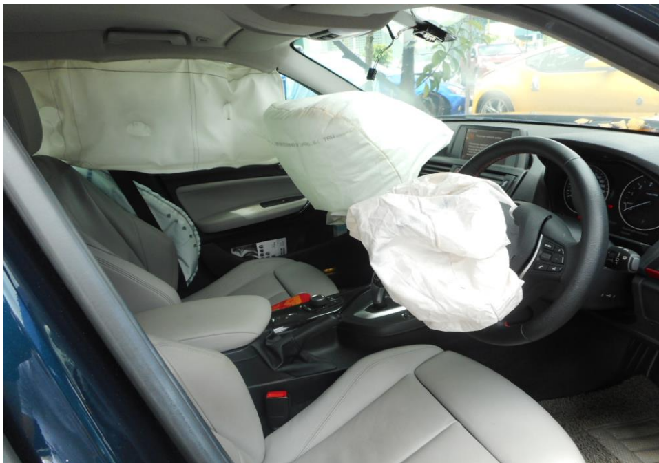
Photo 16 shows the deployment of the Supplemental Restraint System (SRS) airbag in the Motor Car as a result of the accident.
