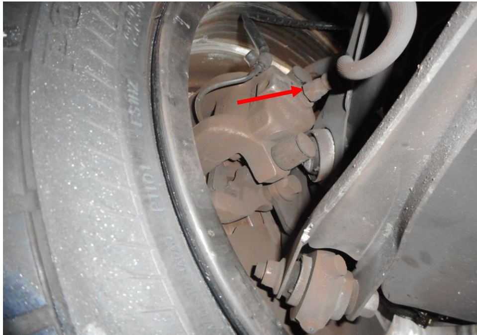
Photo 19 shows the brake hose/pipe (arrowed) at the rear left wheel of the Motor Car. I did not observe any leakage of brake fluid at the time of my inspection of the Motor Car. Static tests of the Motor Car's braking system had indicated that there was no internal leakage of pressure/vacuum. The undercarriage components of the Motor Car were also all found to be intact and without any visible damage.
