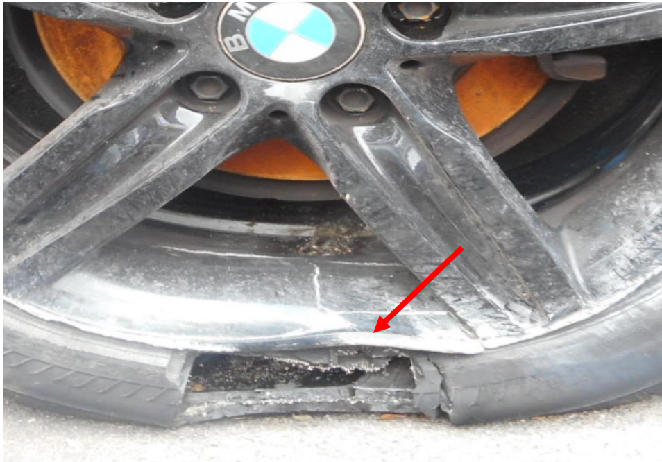
Photo 13 shows the close up condition of the rear right tyre and rim of the Motor Car, which was observed that rim (arrowed) had likely caused cut on the tyre in the midst of the accident due to the impact it sustained from the collision.
