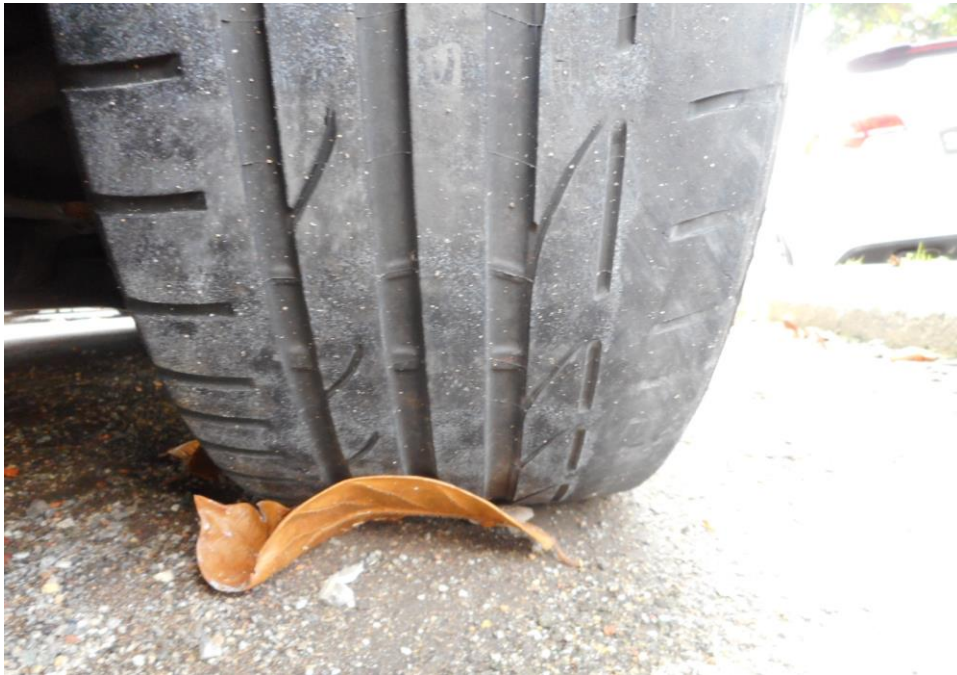
Photo 15 shows the condition of the front left tyre of the Motor Car, which was observed to be in serviceable condition with remaining tread depth of approximately 5.1mm. There was also no tear, cut or burst mark(s) on the outer and the inner sidewalls as well as across the tread of the Motor Car's 2 left tyres.
