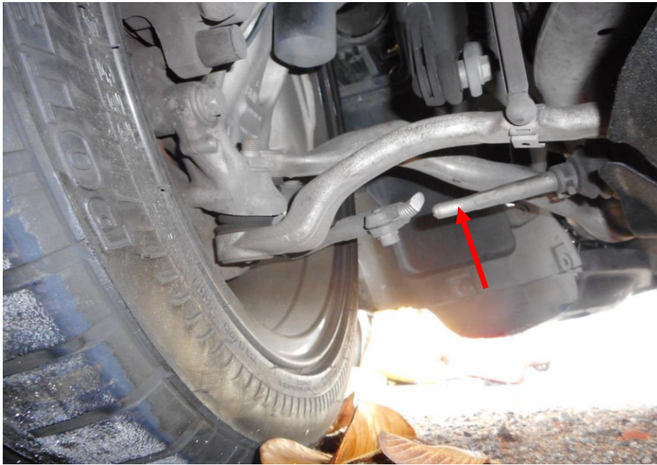
Photo 23 shows the various undercarriage components at the front left wheel of the Motor Car, the steering tie rod (red arrow) was observed to be damaged as a result of the accident.
