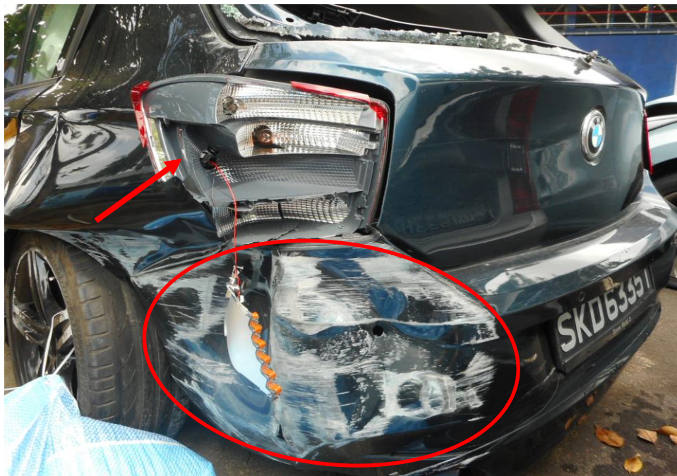
Photo 8 shows the close up view of the Motor Car's rear body at the time of my inspection, its rear left tail lamp (arrowed) and rear bumper (circled) were amongst the body parts that were damaged as a result of the accident.
