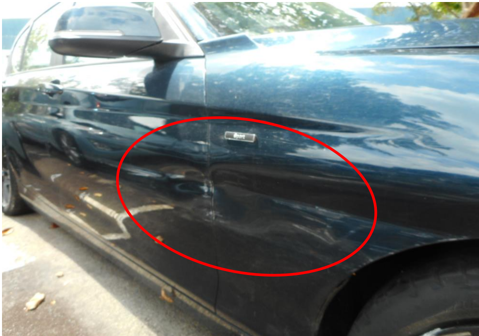
Photo 4 shows the close view of the Motor Car's right body at the time of my inspection. The Motor Car was observed to have sustained damage on its right body panels (circled) were amongst the body parts that were damaged as a result of the accident.
