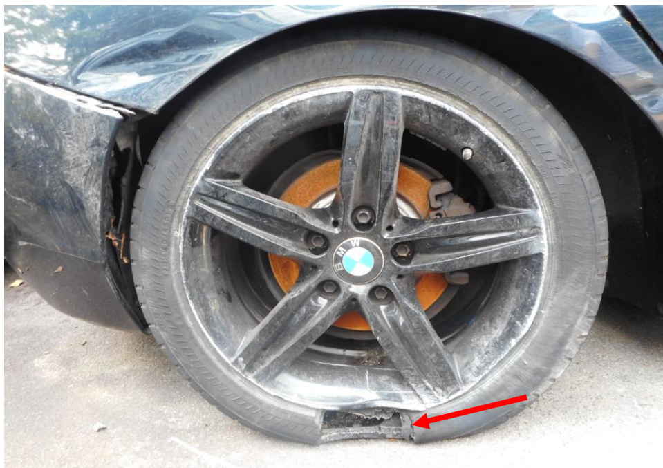
Photo 12 shows the condition of the rear right tyre of the Motor Car, which was observed to be in unserviceable condition as it was damaged (arrowed) as a result of the accident with remaining tread depth of approximately 6mm.
