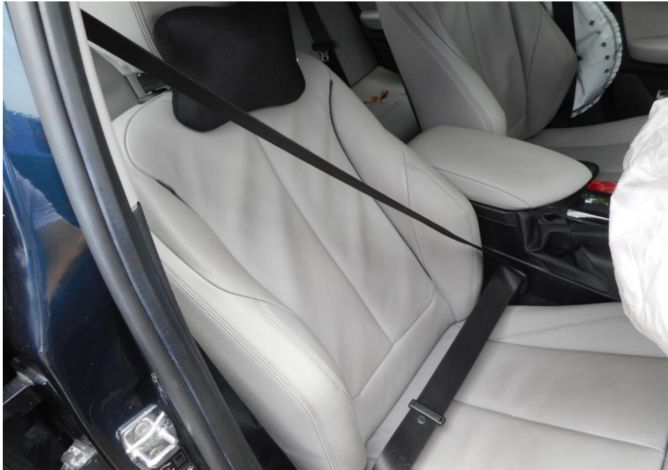
Photo 24 shows that the seat belt on the right seat were able to be fastened securely into the respective pre-tensioners that were fitted at the sides of each seat.
