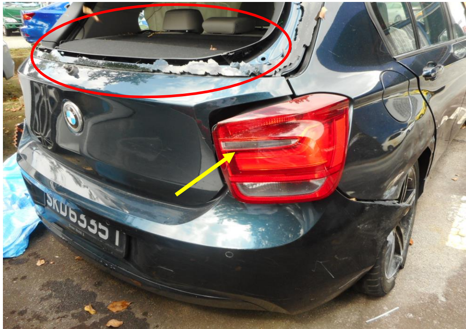
Photo 9 shows the general view of the Motor Car's rear body at the time of my inspection, its rear windscreen (circled) and rear right tail lamp (arrowed) were amongst the body parts that were damaged as a result of the accident.
