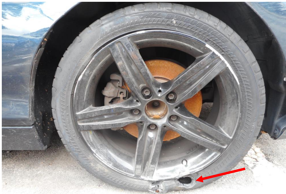
Photo 10 shows the condition of the front right tyre of the Motor Car, which was observed to be in unserviceable condition as it was damaged (arrowed) as a result of the accident with remaining tread depth of approximately 5.2mm.
