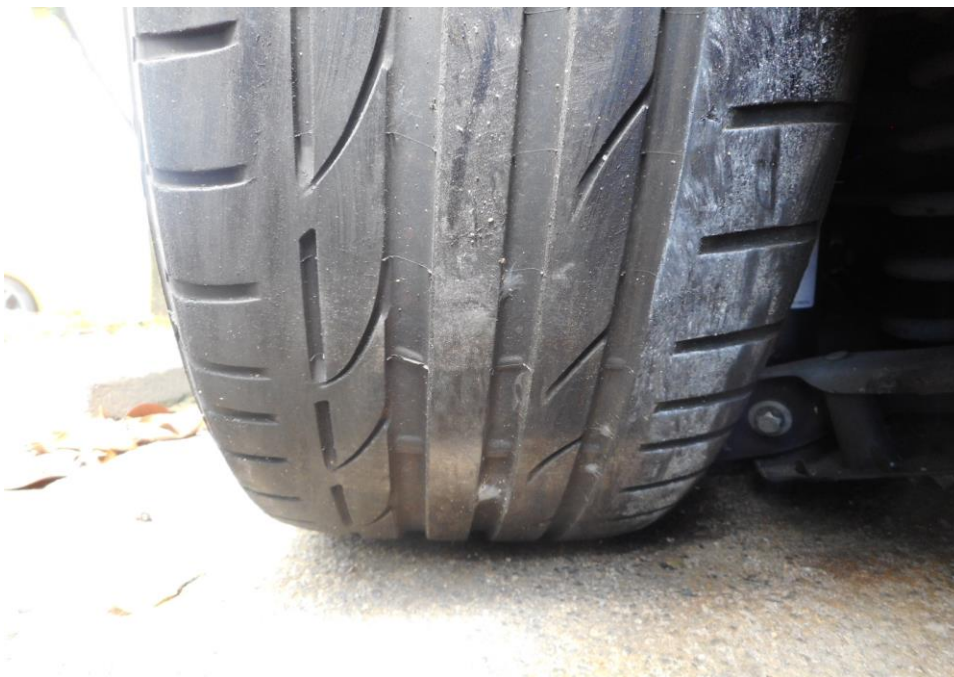
Photo 14 shows the condition of the rear left tyre of the Motor Car, which was observed to be in serviceable condition with remaining tread depth of approximately 4.6mm. There was also no tear, cut or burst mark(s) on the outer and the inner sidewalls as well as across the tread of the Motor Car's 2 left tyres.
