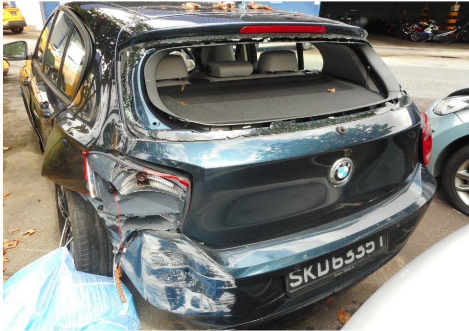
Photo 7 shows the general view of the Motor Car's rear body at the time of my inspection, its rear windscreen, both rear tail lamps and rear bumper were amongst the body parts that were damaged as a result of the accident.
