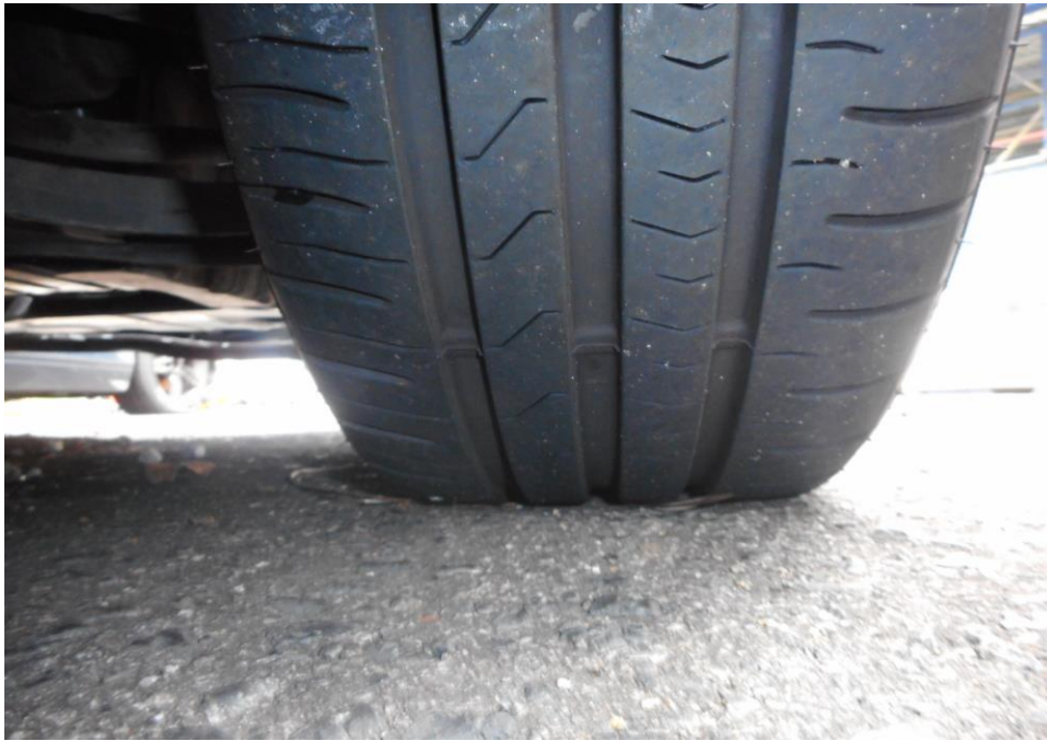
Photo 8 shows the condition of the front right tyre of the Motor Car, which was observed to be in serviceable condition with remaining tread depth of approximately 4.8mm. The tyre was sufficiently inflated for vehicular operation with no tear, cut or burst mark(s) on the outer and the inner sidewalls as well as across the tread. The 4 tyres of the Motor Car were wrapped around standard steel wheel rims without any damage.
