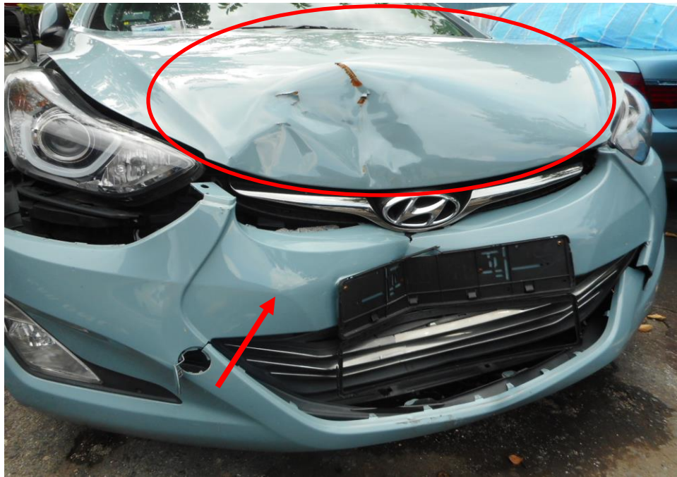
Photo 4 shows the close up view of the Motor Car's front body at the time of my inspection. The Motor Car was observed to have sustained damage at its front portion. Its front bonnet (circled), front bumper (arrowed) were amongst the body parts that were damaged as a result of the accident.
