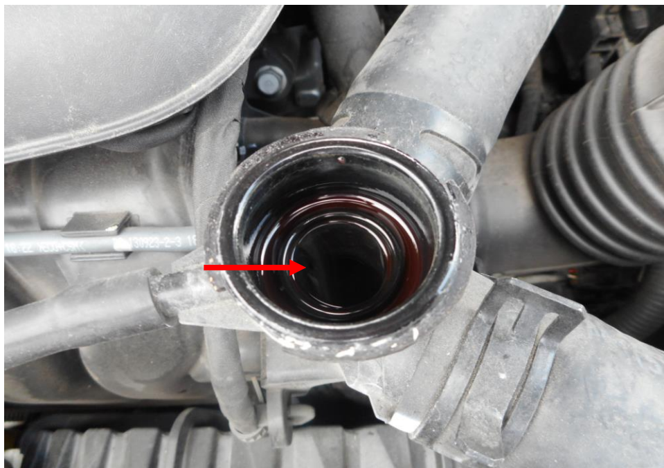
Photo 14 shows checks being carried out to the engine coolant of the Motor Car at the time of my inspection. The engine coolant was observed to be insufficient level (arrowed) due to the damaged the radiator which caused the coolant to flow out.
