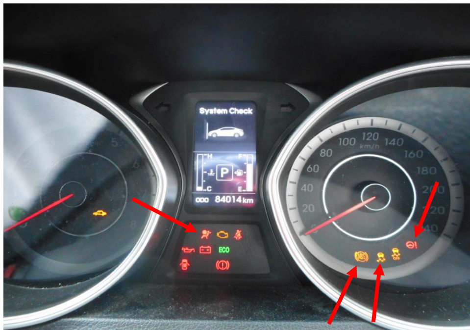
Photo 24 shows the warning light for Anti-Lock Brake System (ABS), Power Steering System (EPS), Traction Control System (TC) and Supplemental Restraint System (SRS) (arrowed) appearing on the instrument panel of the Motor Car during the self-test of its various electronic operating systems when its engine was cranked.
