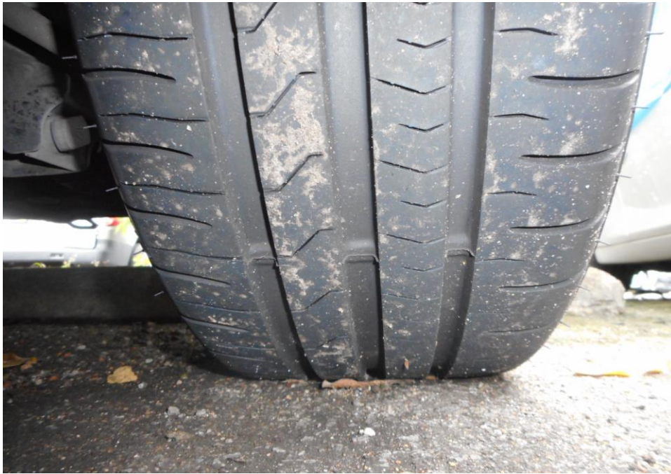
Photo 10 shows the condition of the rear left tyre of the Motor Car, which was observed to be in serviceable condition with remaining tread depth of approximately 6.6mm. The tyre, which was wrapped around steel wheel rim, was also observed to be sufficiently inflated for vehicular operation. The 4 tyres of the Motor Car were wrapped around standard steel wheel rims.
