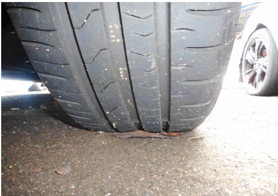
Photo 9 shows the condition of the rear right tyre of the Motor Car, which was observed to be in serviceable condition with remaining tread depth of approximately 6.8mm. The tyre was also observed to be sufficiently inflated for vehicular operation with no tear, cut or burst mark(s).
