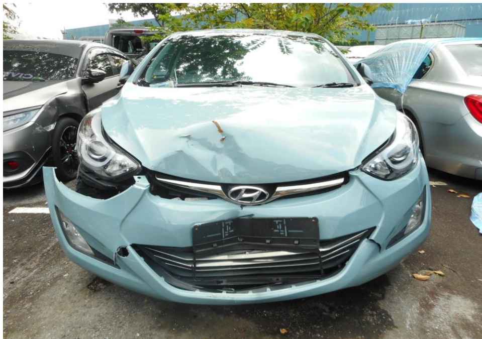
Photo 3 shows a general view of the Motor Car's front body at the time of my inspection. The Motor Car was observed to have sustained damage at its front portion. Its front bonnet, front bumper and its radiator were amongst the body parts that were damaged as a result of the accident.
