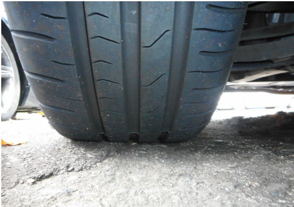
Photo 11 shows the condition of the front left tyre of the Motor Car, which was observed to be in serviceable condition with remaining tread depth of approximately 6.2mm. There was also no tear, cut or burst mark(s) on the outer and the inner sidewalls as well as across the tread of the Motor Car's 4 tyres.
