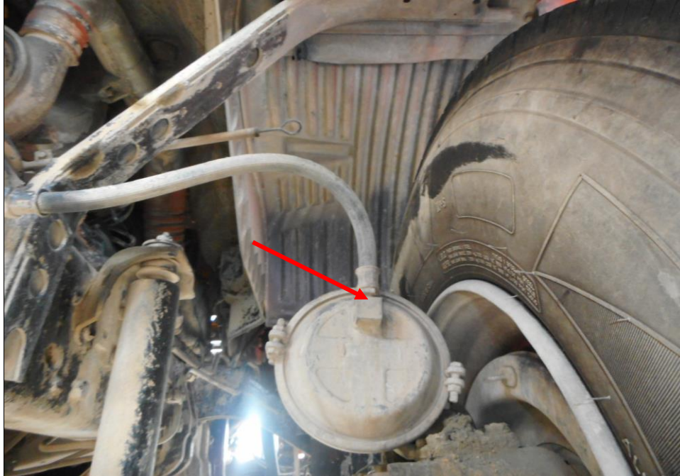
Photo 25 shows the brake pipe (arrowed) at the front right wheel of the Motor Trailer. I did not observe any leakage of brake fluid at the time of my inspection of the Motor Trailer. My static tests of the Motor Trailer's braking system, along with my visual examination of the various mechanical components in the braking system, had indicated that there was no internal leakage of pressure/vacuum. Hence the braking system of the Motor Trailer was likely to be in serviceable condition at the material time of accident.
