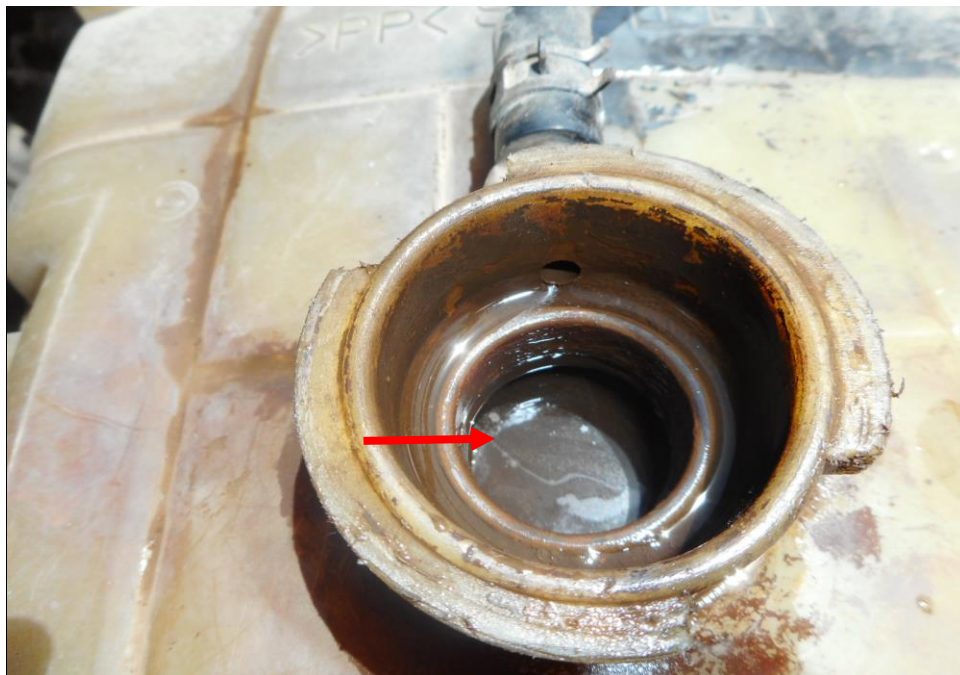
Photo 19 shows the engine coolant reservoir of the Motor Trailer at the time of my inspection. The engine coolant was observed to be of sufficient level (arrowed) and without any visible contamination.
