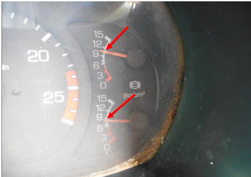
Photo 18 shows the air in the air brake cylinders of the Motor Trailer at the time of my inspection. The air in the cylinder was observed to be of sufficient level & serviceable at the time of the accident.
