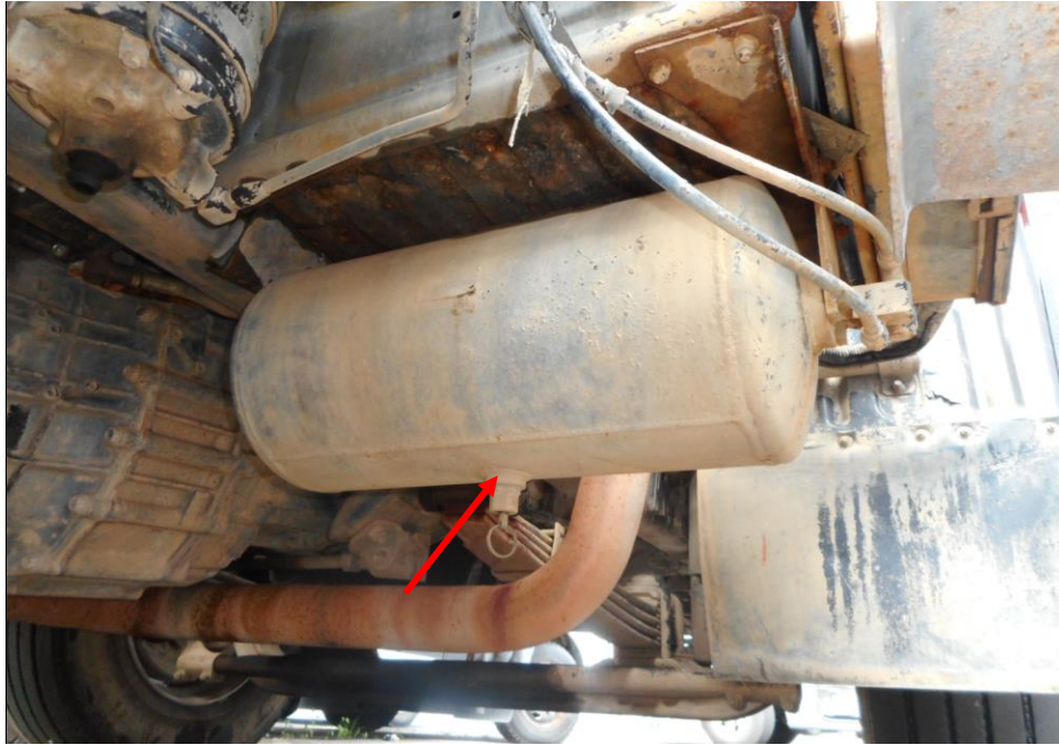
Photo 27 shows the air brake cylinders (arrowed) at the undercarriage of the Motor Trailer. I did not observe any leakage of air brake fluid at the time of my inspection of the Motor Trailer. My static tests of the Motor Trailer's braking system, along with my visual examination of the various mechanical components in the braking system had indicated that there was no internal leakage of pressure/vacuum. Hence the braking system of the Motor Trailer was likely to be in serviceable condition at the material time of accident.
