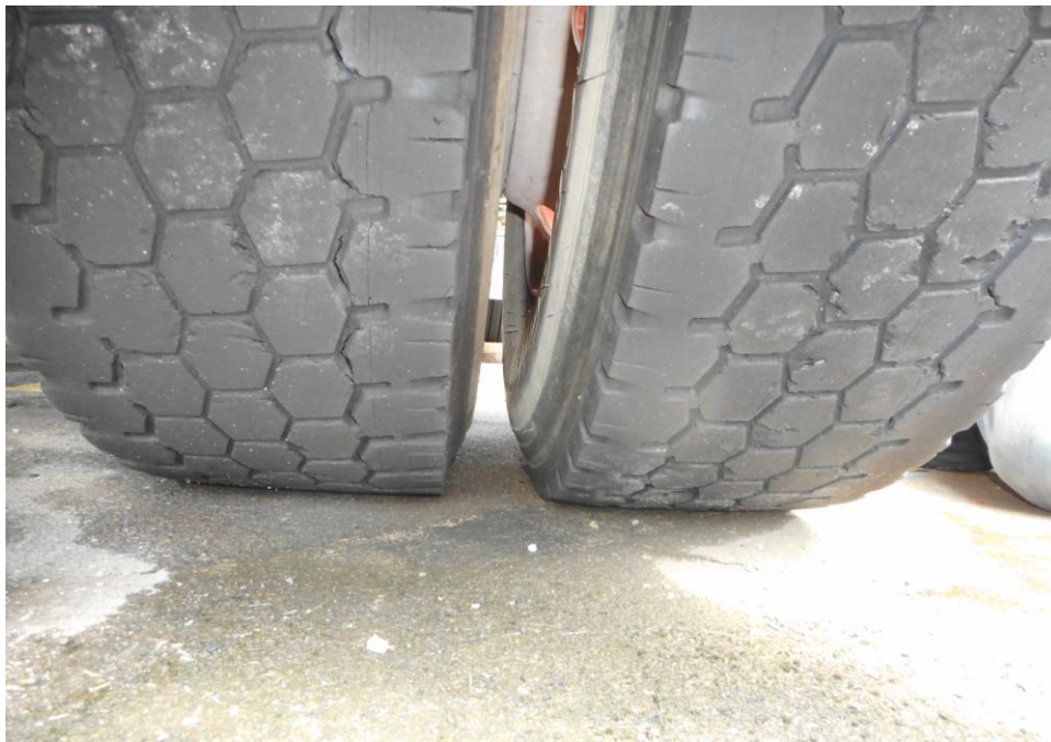
Photo 12 shows the condition of the rear right tyre of the Motor Trailer, which was observed to be in serviceable condition with remaining tread depth of approximately 4.7mm. The tyre, which was wrapped around standard steel wheel rim, was also observed to be sufficiently inflated for vehicular operation.
