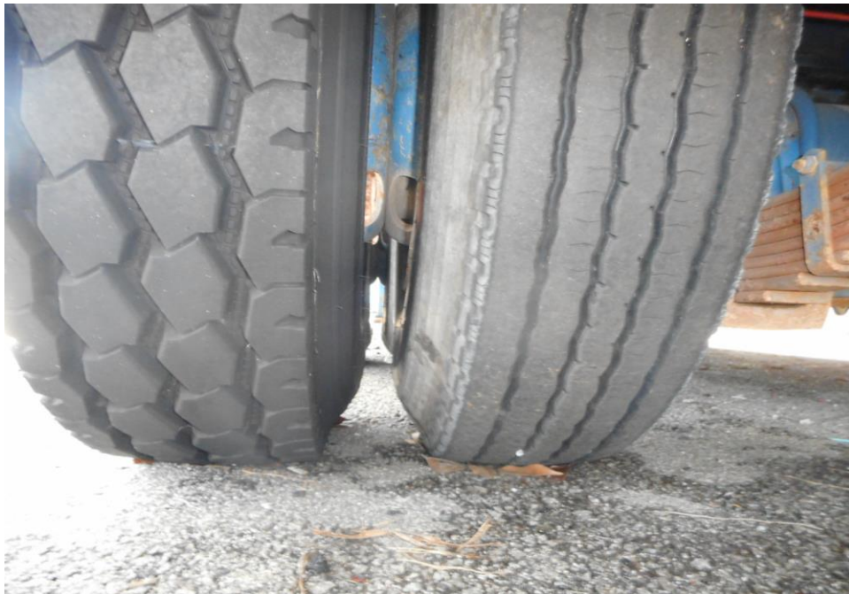
Photo 16 shows the condition of the left tyres of the trailer, which was observed to be in serviceable condition with remaining tread depth of approximately 13.3mm. The tyres, which were wrapped around standard steel wheel rim, were also observed to be sufficiently inflated for vehicular operation. There was also no damage found on all 6 steel wheel rims of the Motor Trailer.
