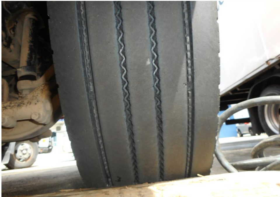
Photo 11 shows the condition of the front right tyre of the Motor Trailer, which was observed to be in serviceable condition with remaining tread depth of approximately 8.5 mm. The tyre, which was wrapped around standard steel wheel rim, was also observed to be sufficiently inflated for vehicular operation. There was no tear, cut or burst mark(s) on the outer and the inner sidewalls as well as across the tread of the 6 tyres that were fitted on the Motor Trailer.
