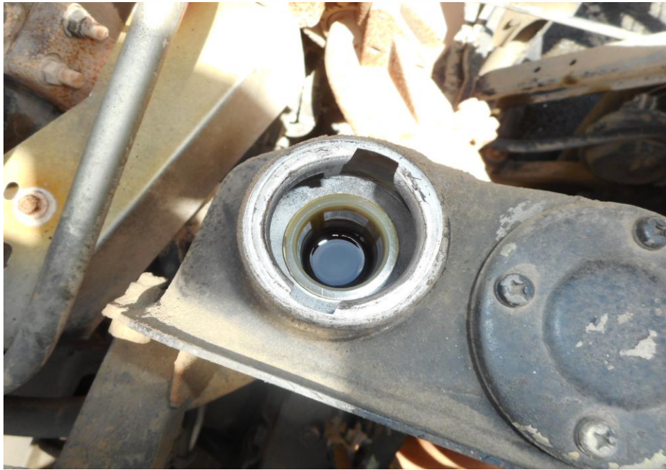
Photo 20 shows the power steering fluid reservoir of the Motor Trailer at the time of my inspection. The power steering fluid was observed to be of sufficient level and without any visible contamination.
