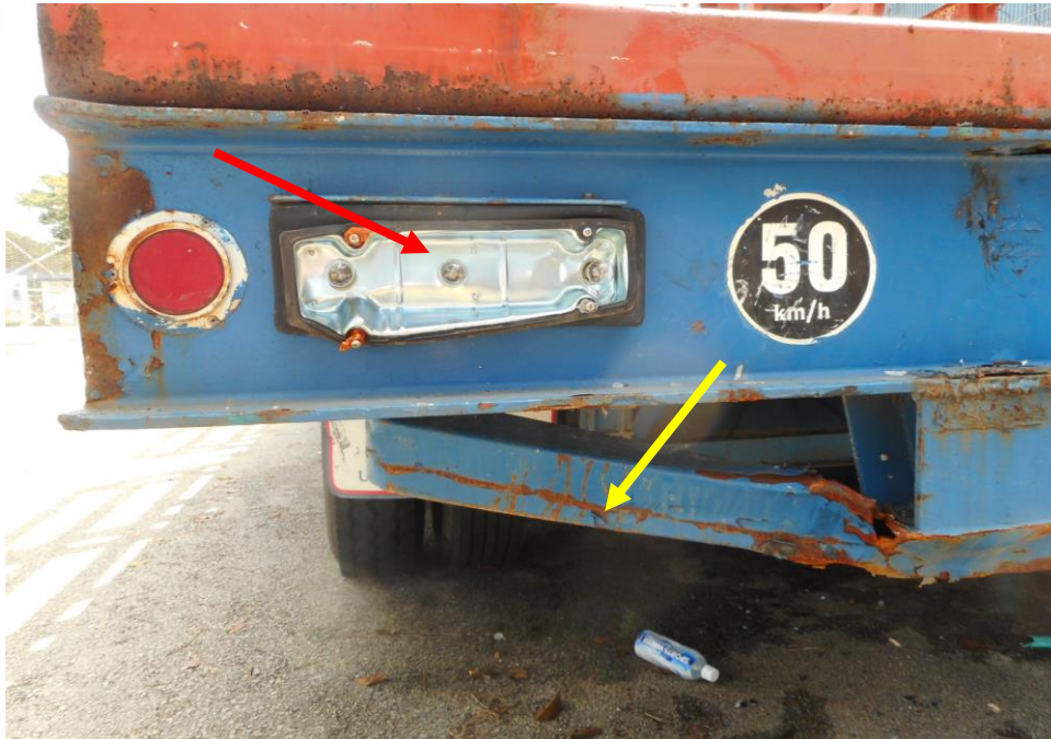
Photo 7 shows a close up view of the front body of the trailer at the time of my inspection. The Motor Trailer was observed to sustained damage at its rear left portion. Its rear left brake lamp (red arrow) & body panel (yellow arrow) was damaged as a result of the accident.
