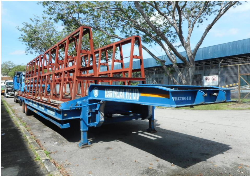
Photo 9 shows a general view of the trailer's right body at the time of my inspection. The Motor Trailer was observed to be intact and unaffected by the accident.
