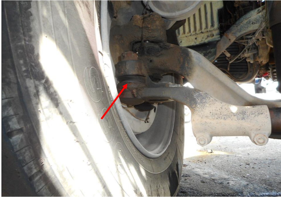
Photo 29 shows the various undercarriage components at the front left wheel of the Motor Trailer, in particular the steering tie rod end (arrowed). The various undercarriage components of the Motor Trailer were all found to be intact without any visible damage. There was also no sign of fluid stain(s) observed on the various undercarriage components.
