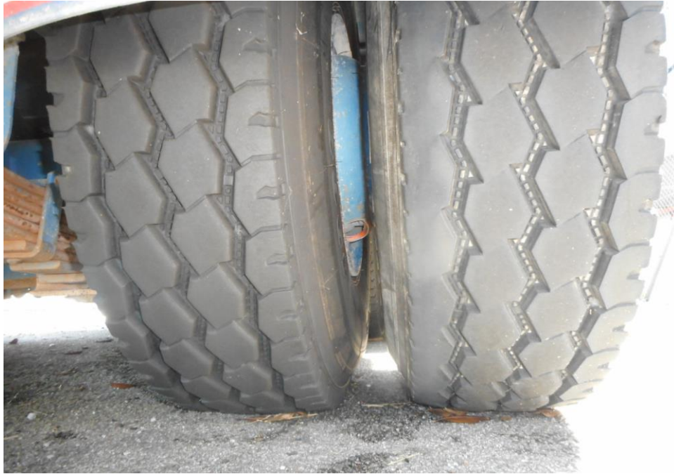
Photo 15 shows the condition of the right tyres of the trailer, which was observed to be in serviceable condition with remaining tread depth of approximately 9.9mm. The tyre, which was wrapped around standard steel wheel rim, was also observed to be sufficiently inflated for vehicular operation.
