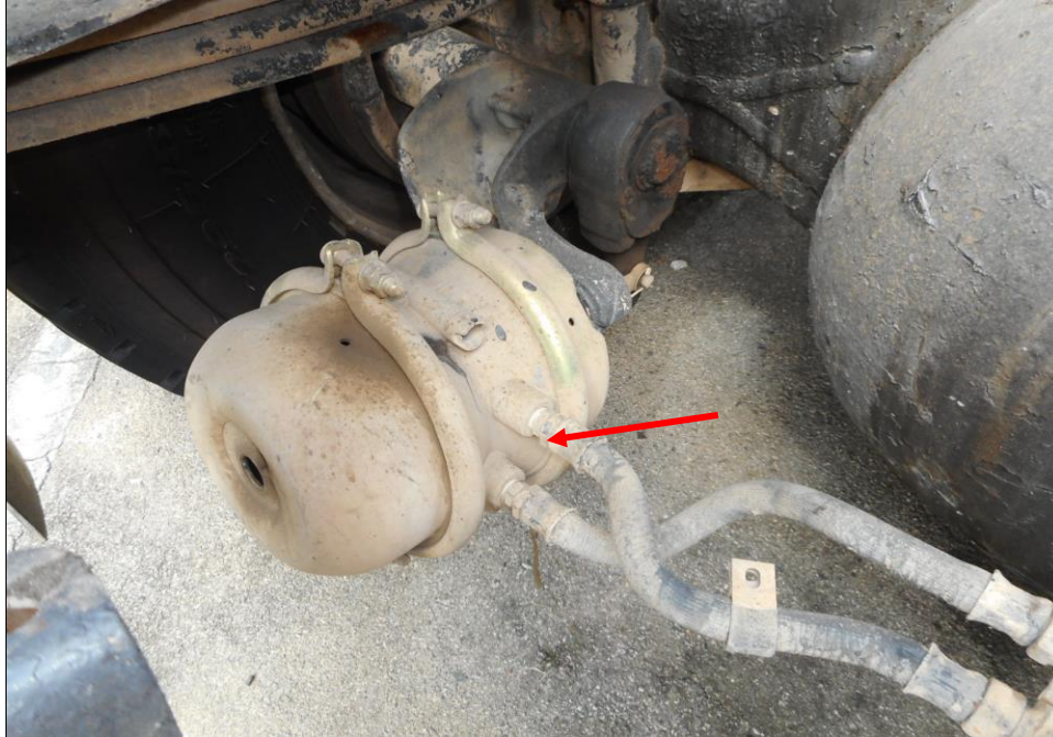
Photo 23 shows the brake pipe (arrowed) at the rear right wheel of the Motor Trailer. I did not observe any leakage of brake fluid at the time of my inspection of the Motor Trailer. My static tests of the Motor Trailer's braking system, along with my visual examination of the various mechanical components in the braking system, had indicated that there was no internal leakage of pressure/vacuum. Hence the braking system of the Motor Trailer was likely to be in serviceable condition at the material time of accident.
