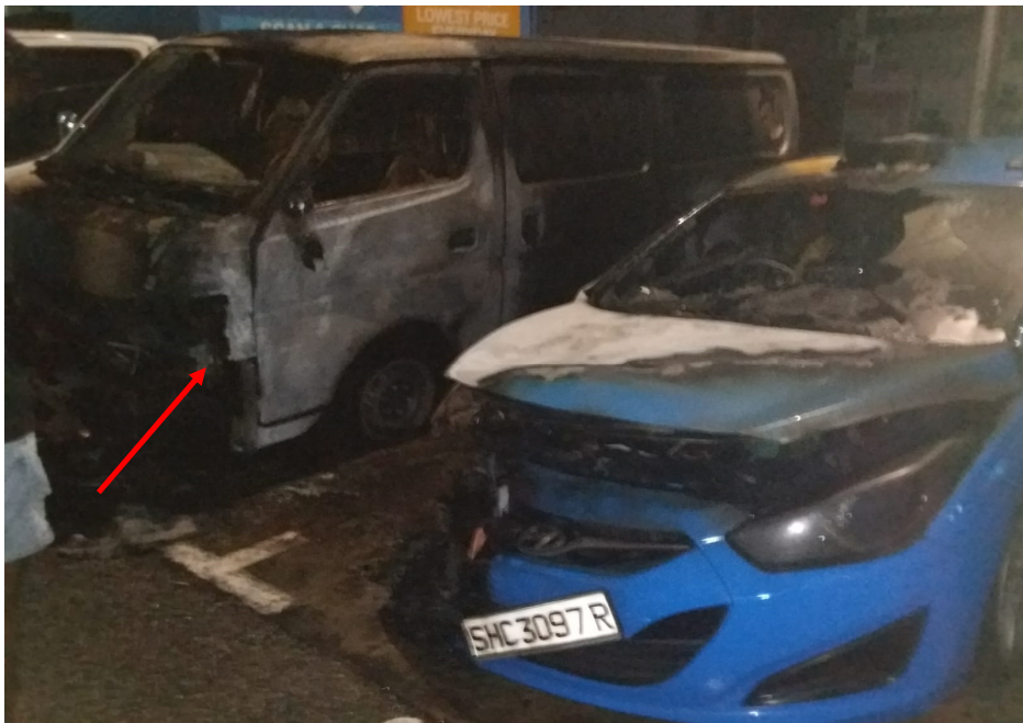
Photo 14 shows Insured Vehicle after the fire was extinguished. A motor van parked on the right side of the Insured Vehicle had sustained damage of heat nature at its left side (arrowed).
