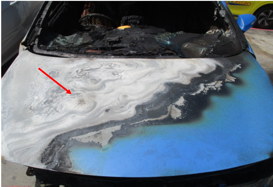
Photo 7 shows the burn pattern and whitish burn marks that were found on the right portion of the front bonnet of the Insured Vehicle (arrowed). Such whitish burn marks are a result of exposure to prolonged heat intensity, which may indicate where the fire had started. Rust would also begin to develop on these areas soon after the fire.
