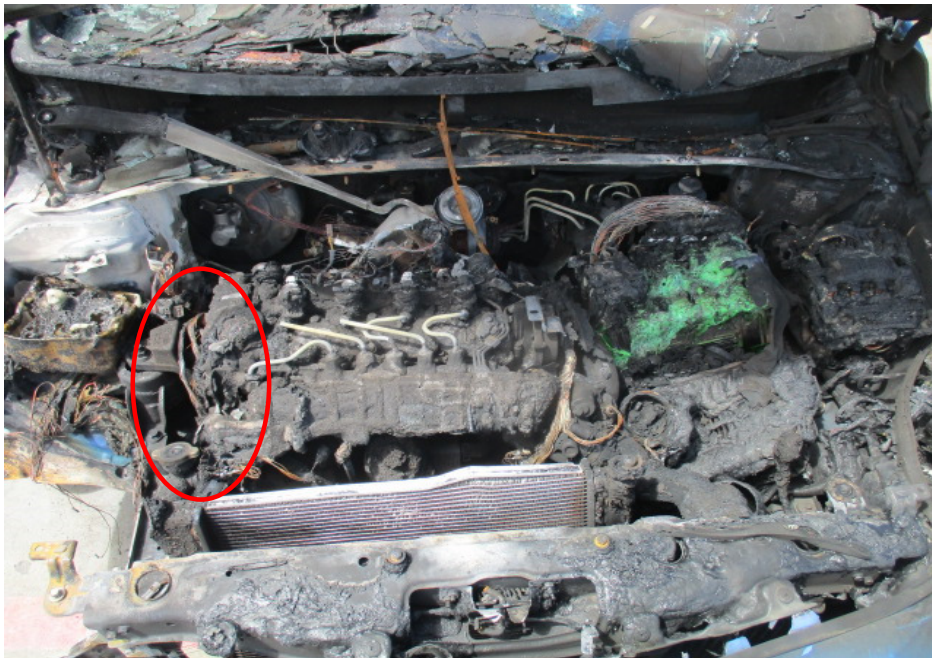
Photo 9 shows the original factory fitted wirings around the right portion of the engine compartment, which is in the immediate vicinity where the fire to the Insured Vehicle had likely started. We had found greenish residue on several burnt stretches of these wirings (circled). The presence of such greenish residue indicates internal heating of copper wires, a sign of an electrical short circuit occurring. The greenish residue is normally left behind from oxidation as a result of chemical reaction involving the copper wires.
