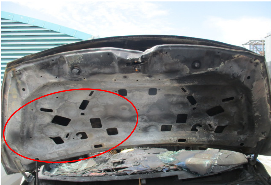
Photo 8 shows the rust that had developed on the underside of the front bonnet, around the right portion (circled). The development of rust is an indication that this area was subjected to prolonged exposure to high heat intensity, which had caused the steel/metal material of the front bonnet to be exposed to natural environmental condition. Hence the fire to the Insured Vehicle can be determined to have originated towards the right portion of the engine compartment.
