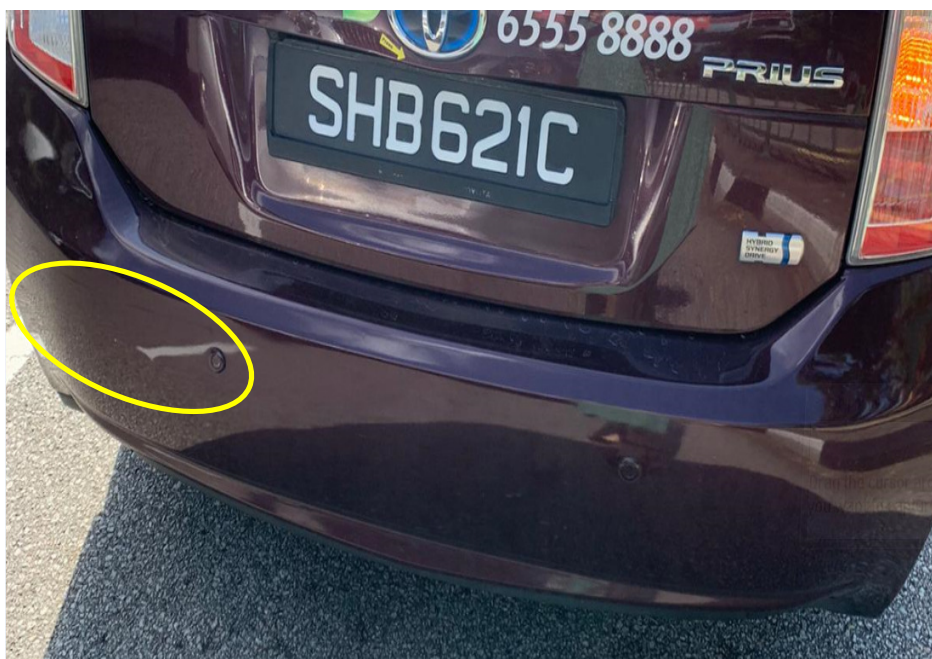
Photo 15 shows a close up view of the rectangular indentation on the left lower portion of the Taxi's rear bumper (circled).
