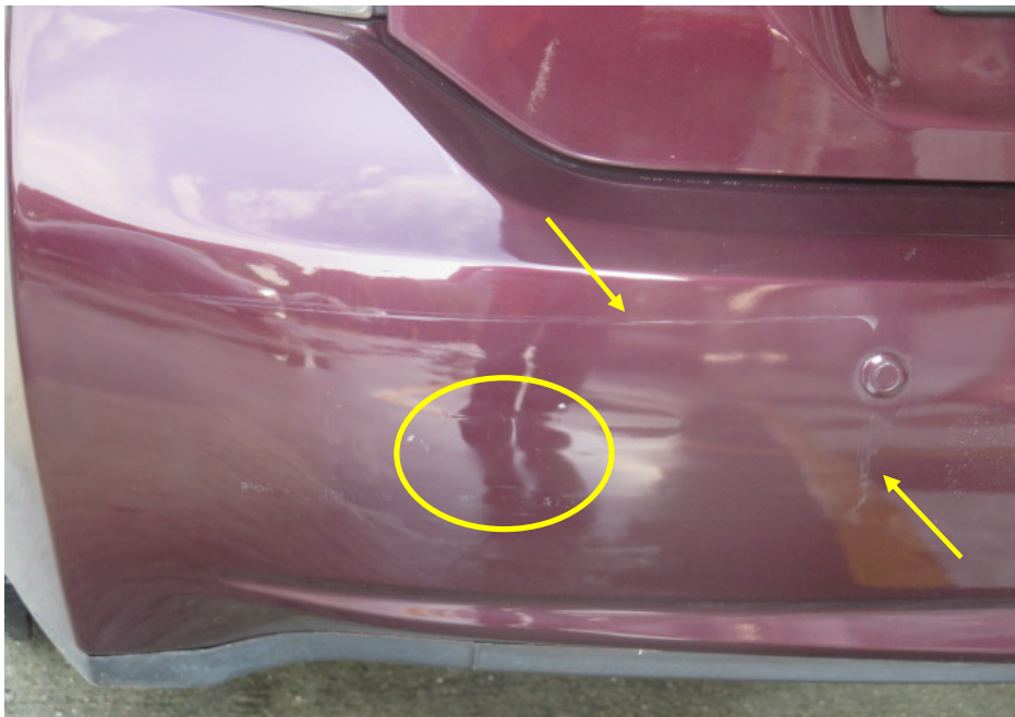
Photo 2 shows a closer view of the left lower portion of the rear bumper of the Taxi. We observed whitish marks (circled) as well as a rectangular indentation (yellow arrows) around the left lower portion of the rear bumper of the Taxi.
