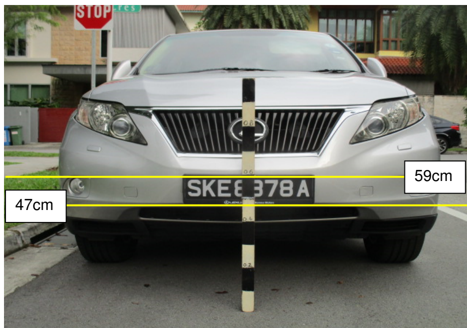
Photo 19 shows the height measurement being conducted on the front portion of the Lexus. The dented front number plate and distorted front number plate frame of the Lexus are within the 47cm to 59cm height range.
