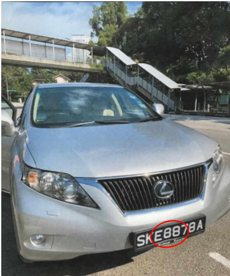
Photo 16 shows the frontal portion of the Lexus post- accident. We observed a dent on the centre portion of the front number plate and distortion of the front number plate frame (circled).
