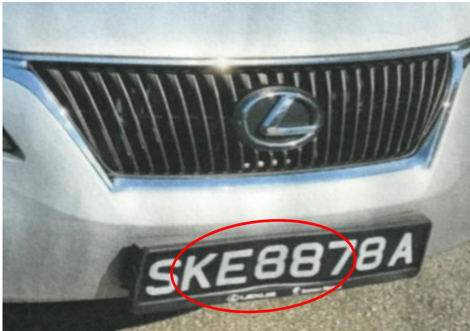
Photo 17 shows a close up view of the dented front number plate and distorted front number plate frame of the Lexus post- accident (circled).
