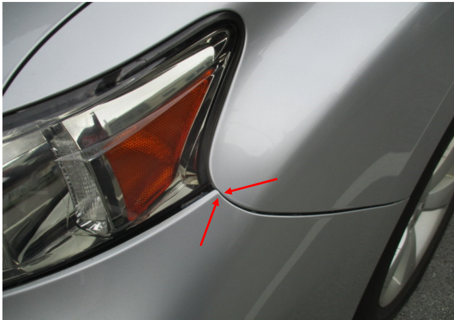
Photo 11 shows a closer view of the left corner edge of the front bumper of the Lexus. We observed that there was a slight misalignment at the corner edges (arrowed).
