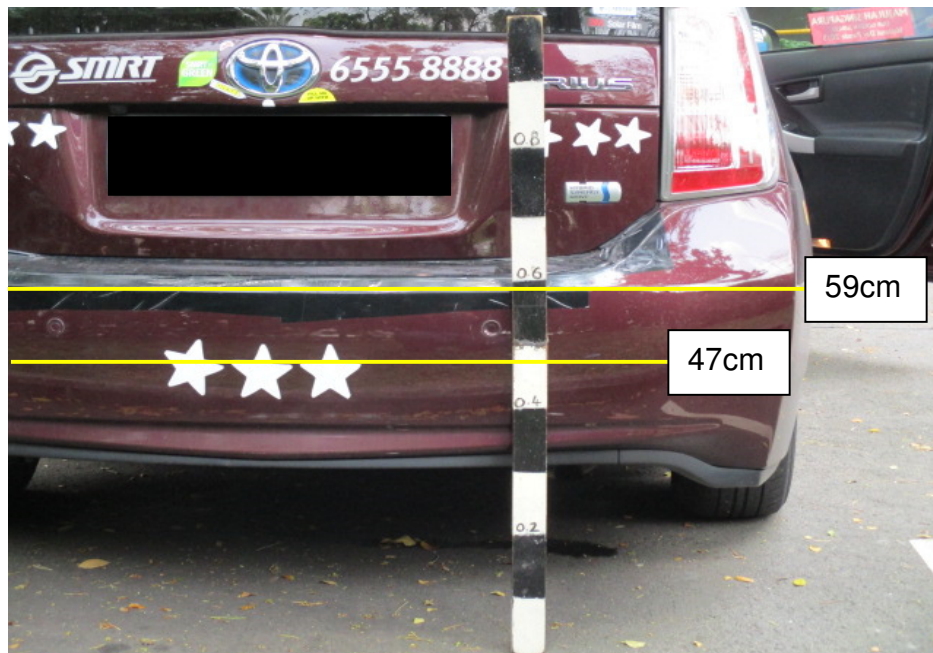
Photo 18 shows the height measurement being conducted on the rear portion of the Taxi (using a similar make and model). The height range of the rectangular indentation and whitish marks found on the lower left portion of the Taxi's rear bumper was between 47cm to 59cm above ground level.
