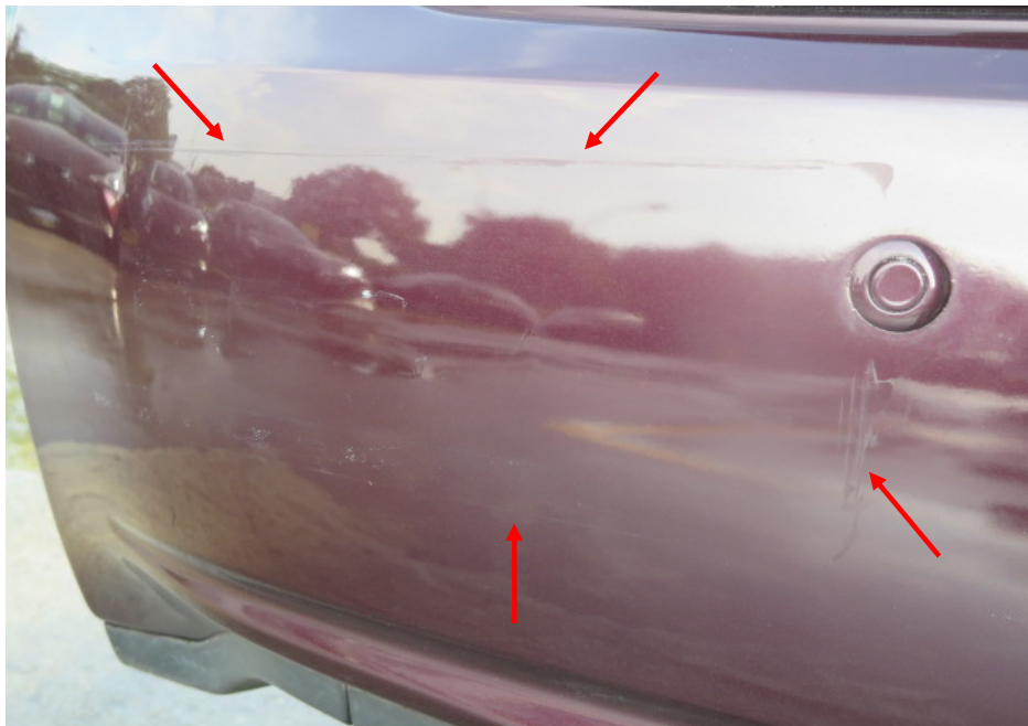
Photo 4 shows a close up view of the rectangular indentation (red arrows) around the left lower portion of the rear bumper of the Taxi.
