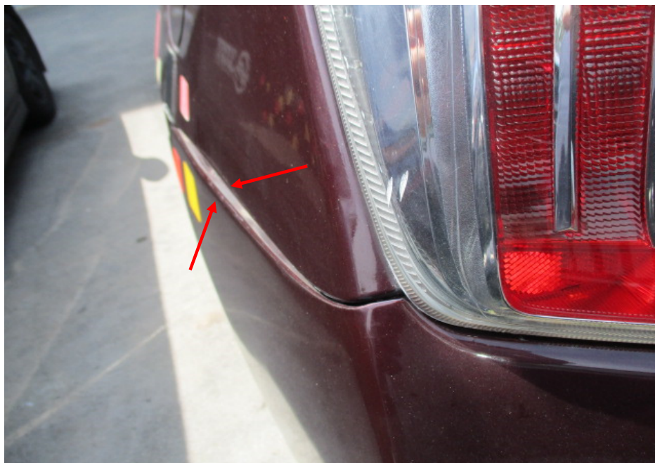
Photo 5 shows a close up view of the left corner edge of the rear bumper of the Taxi. We observed a slight misalignment at the corner edges (red arrows).
