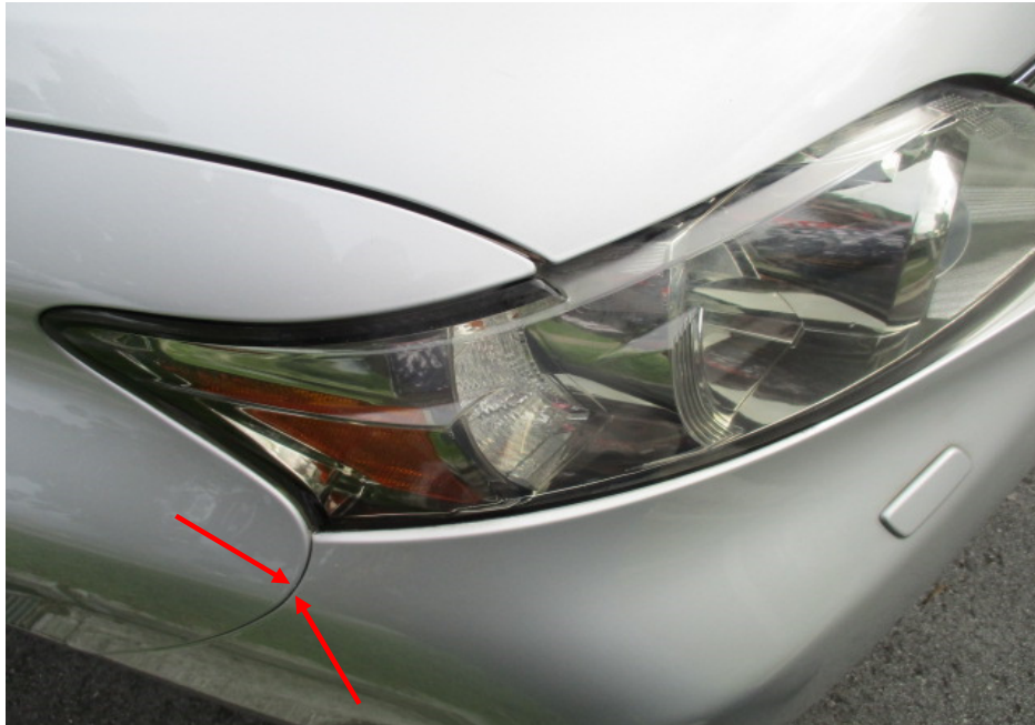
Photo 10 shows a closer view of the right corner edge of the front bumper of the Lexus. We observed that there was no misalignment at the corner edges (arrowed).
