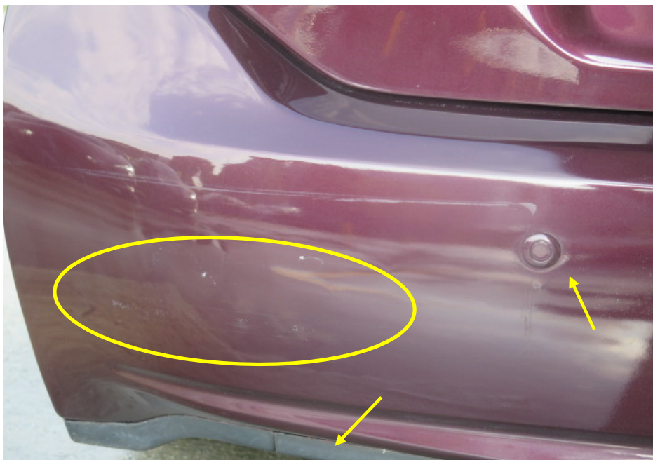
Photo 3 shows a close up view of the whitish marks (circled) at the left lower portion of the rear right bumper of the Taxi.
