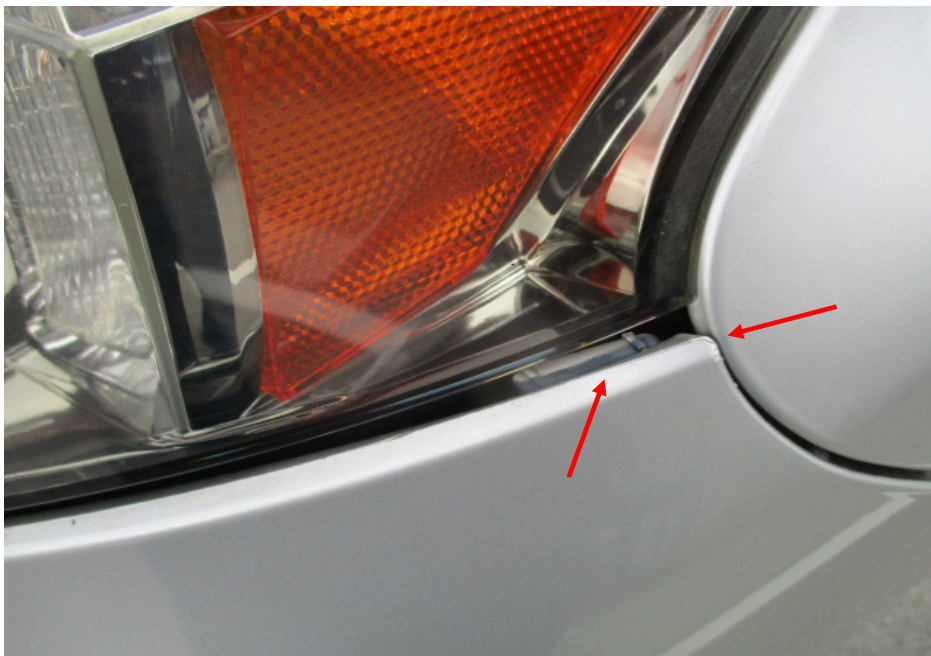
Photo 12 shows a close up view of the misaligned left corner edge of the front bumper of the Lexus (arrowed). Mrs Lim again mentioned that this damage was not related to the accident.
