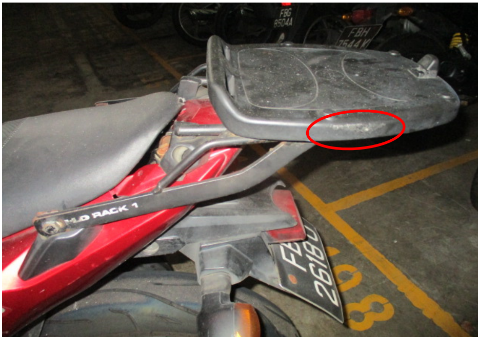
Photo 13 shows the top box rack of the Motorcycle that had sustained damage as a result of the accident (circled).
