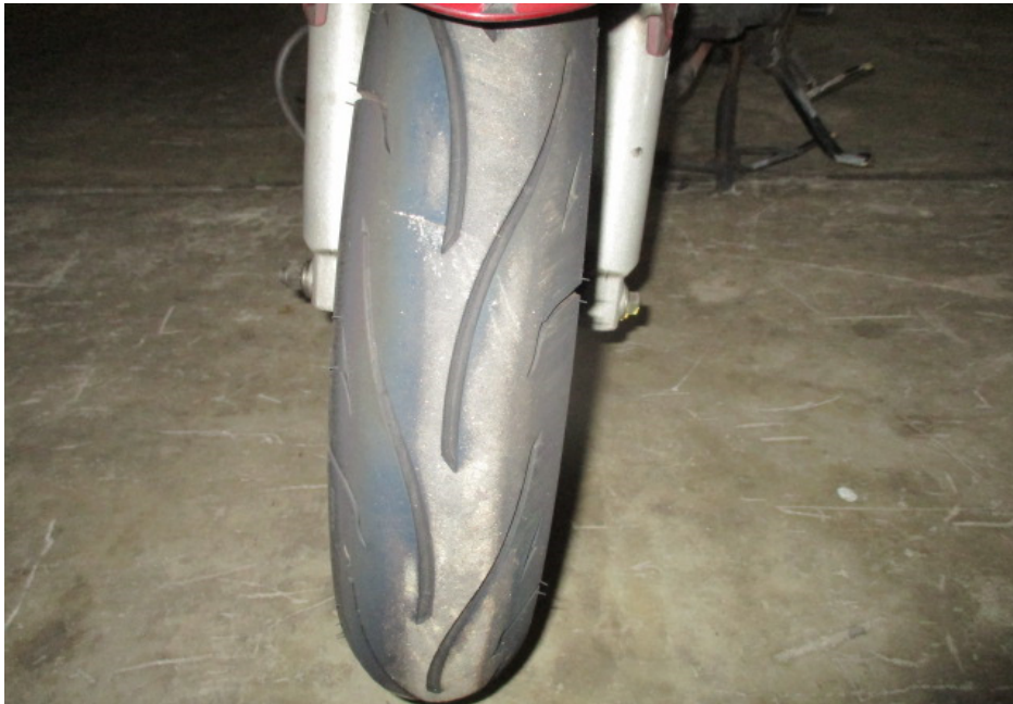
Photo 14 shows the front tyre of the Motorcycle at the time of our inspection. The front tyre was observed to be in serviceable condition with remaining tread depth of approximately 4mm. The pattern of the tread was also clearly visible. There was no tear, burst mark(s) and/or punctured hole(s) on the sidewalls as well as across the tread of the front tyre.
