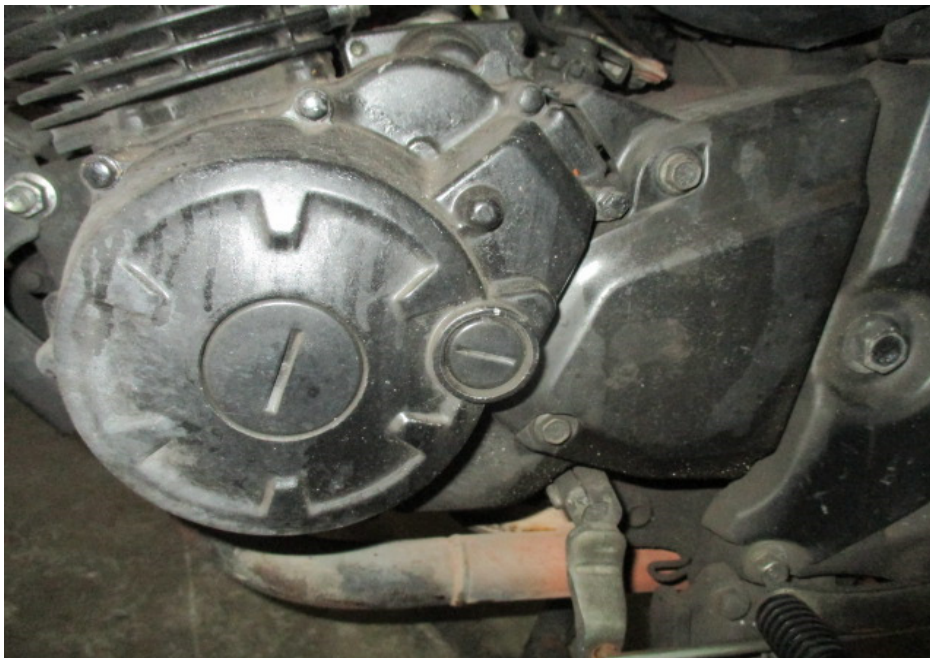
Photo 16 shows the left side of the engine of the Motorcycle at the time of our inspection. The various engine related parts and components were found to be intact with no visible damage. There was also no sign(s) or indication(s) of fluid leak observed around the left engine area of the Motorcycle.
