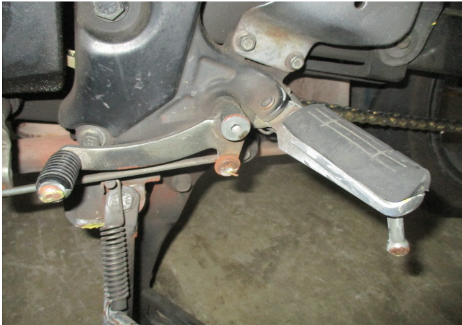
Photo 12 shows the bent gear shift pedal and left front footrest of the Motorcycle as a result of the accident.
