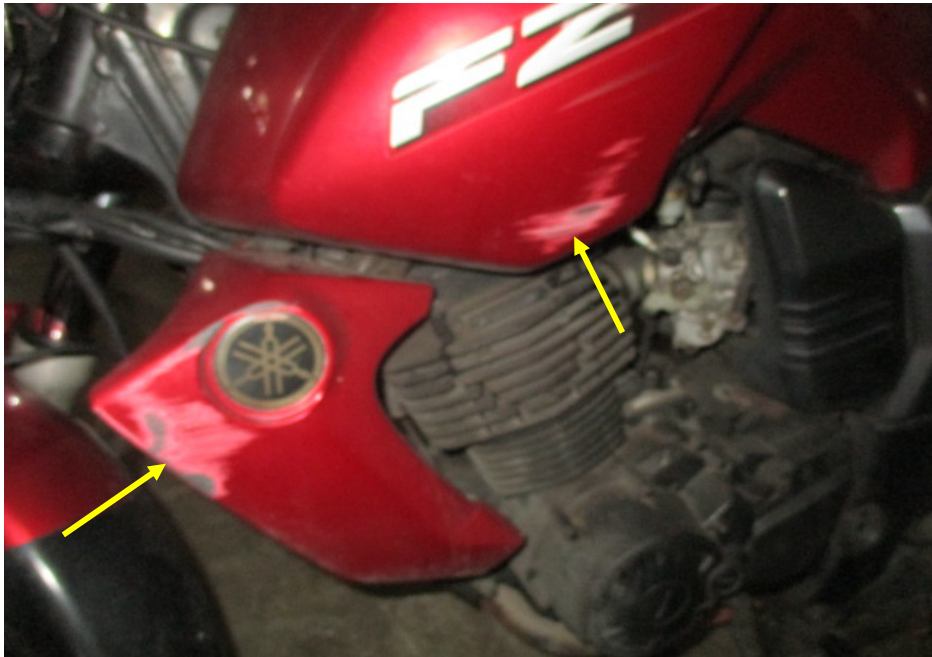
Photo 8 shows the left radiator cover and petrol tank cover (arrowed), which were amongst the body parts of the Motorcycle that had sustained damage as a result of the accident.
