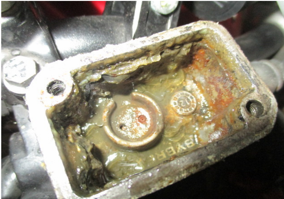
Photo 24 shows the brake fluid reservoir for the front brake of the Motorcycle. The brake fluid reservoir was found to be empty and contaminated.
