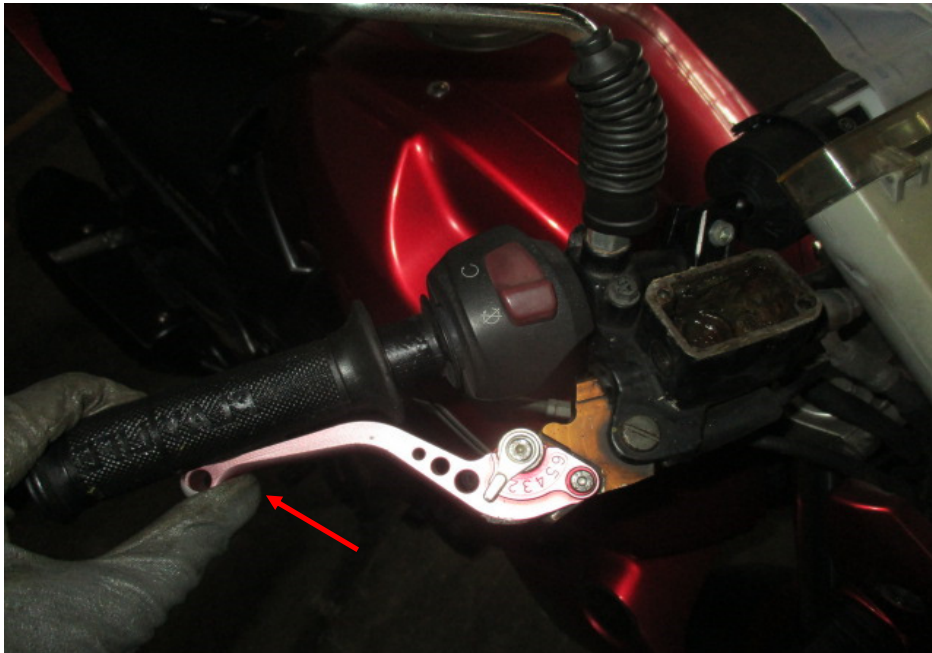
Photo 25 shows the front brake lever being depressed. There was no resistance felt (spongy like feel) upon pressing the front brake lever (arrowed). This would indicate that there may be a leakage of pressure/vacuum in the brake system.
