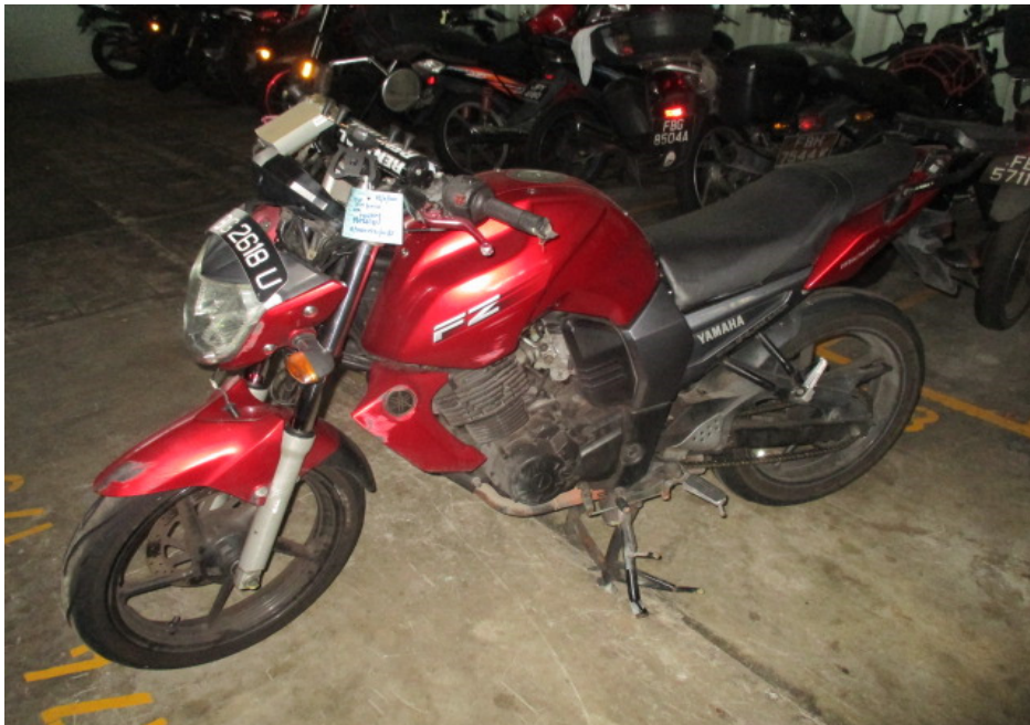
Photo 3 shows a general view of the left body of the Motorcycle at the time of our inspection. The Motorcycle was observed to have sustained damages all around. The body parts that were found to have been damaged include its front cowlings, headlight assembly, front mudguard, left side mirror, handlebar ends, front brake lever, clutch lever, gear shift pedal, left front footrest, left pillion foot peg, left radiator cover, petrol tank cover and top box rack, amongst others.
