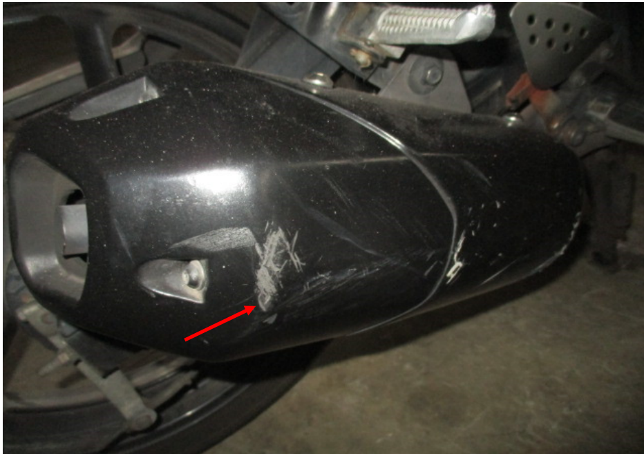
Photo 10 shows a closer view of the exhaust muffler which was amongst the body parts of the Motorcycle that had sustained damages of grazing nature as a result of the accident (arrowed).
