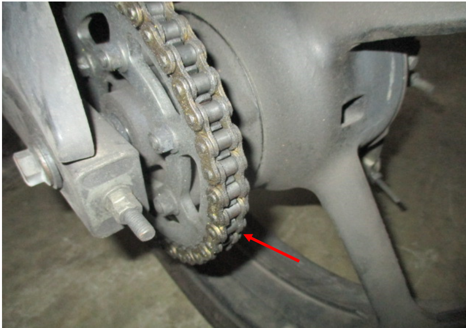
Photo 19 shows a closer view of the gear train (arrowed) of the Motorcycle, which was observed to be intact with no misalignment. It was also adequately lubricated for operating purposes.
