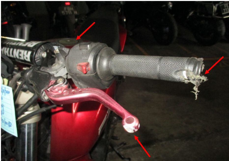
Photo 7 shows the left handlebar end, left side mirror and clutch lever (arrowed), which were amongst the body parts of the Motorcycle that had sustained damage as a result of the accident.
