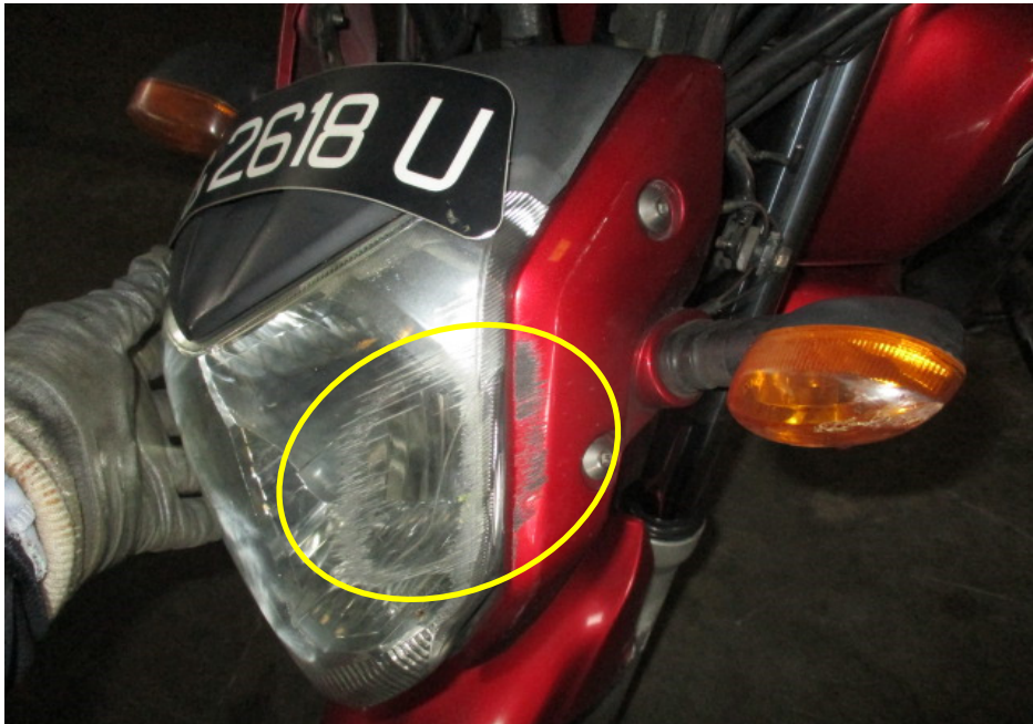
Photo 5 shows a closer view of the headlight and front cowling (circled) which was amongst the body parts of the Motorcycle that had sustained damage as a result of the accident.
