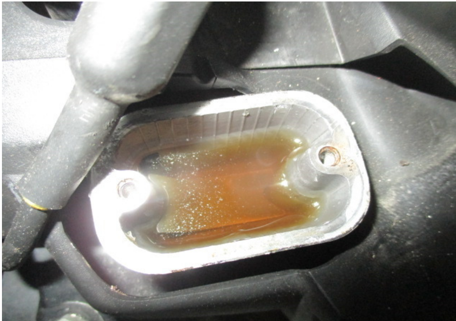
Photo 23 shows the brake fluid reservoir for the front brake of the Motorcycle. The brake fluid was observed to be of sufficient level and without contamination for operational purposes.
