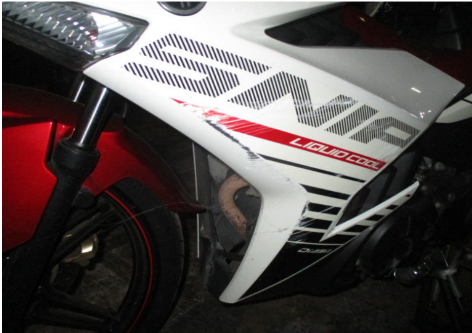
Photo 6 shows a closer view of the left cowling which was amongst the body parts of the Motorcycle that had sustained damage as a result of the accident.
