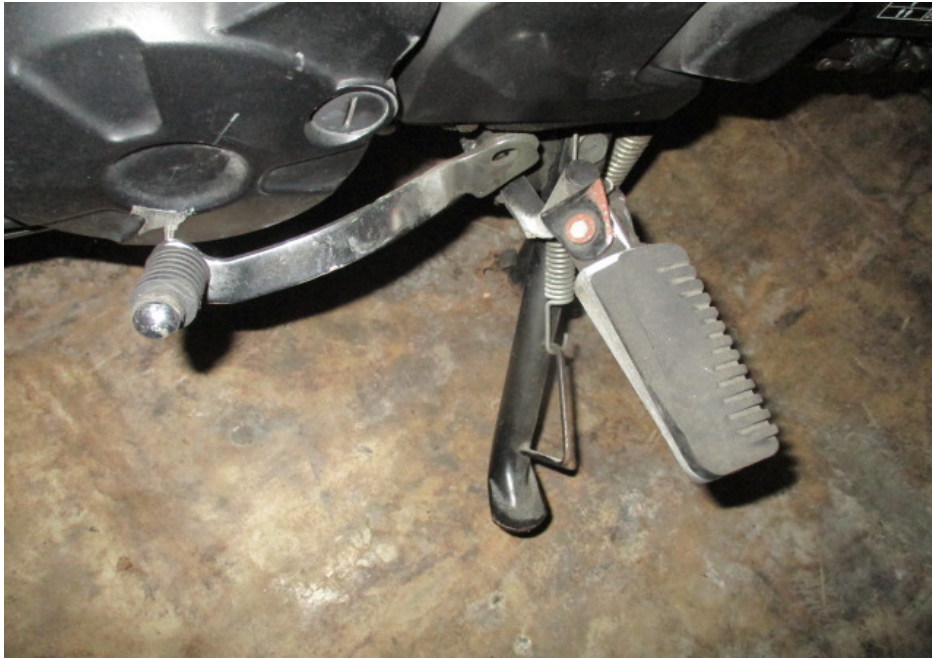
Photo 8 shows a closer view of the bent gear shift pedal and left front footrest which were amongst the body parts of the Motorcycle that had sustained damage as a result of the accident.
