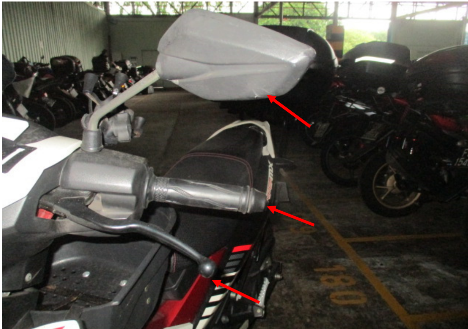
Photo 7 shows the clutch lever, left handlebar end and left side mirror (arrowed), which were amongst the body parts of the Motorcycle that had sustained damage as a result of the accident.
