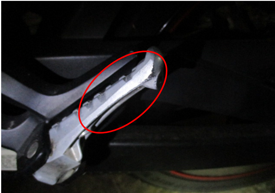
Photo 9 shows a closer view of the left pillion foot peg (circled) which was amongst the body parts of the Motorcycle that had sustained damage as a result of the accident.
