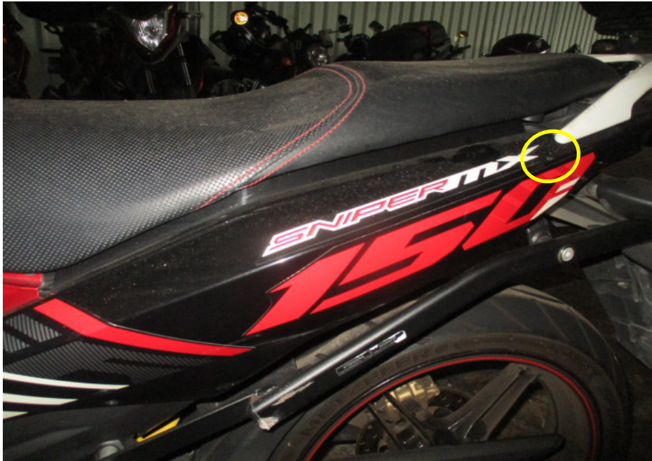
Photo 10 shows a closer view of the left rear side cover (circled) which was amongst the body parts of the Motorcycle that had sustained damage as a result of the accident.
