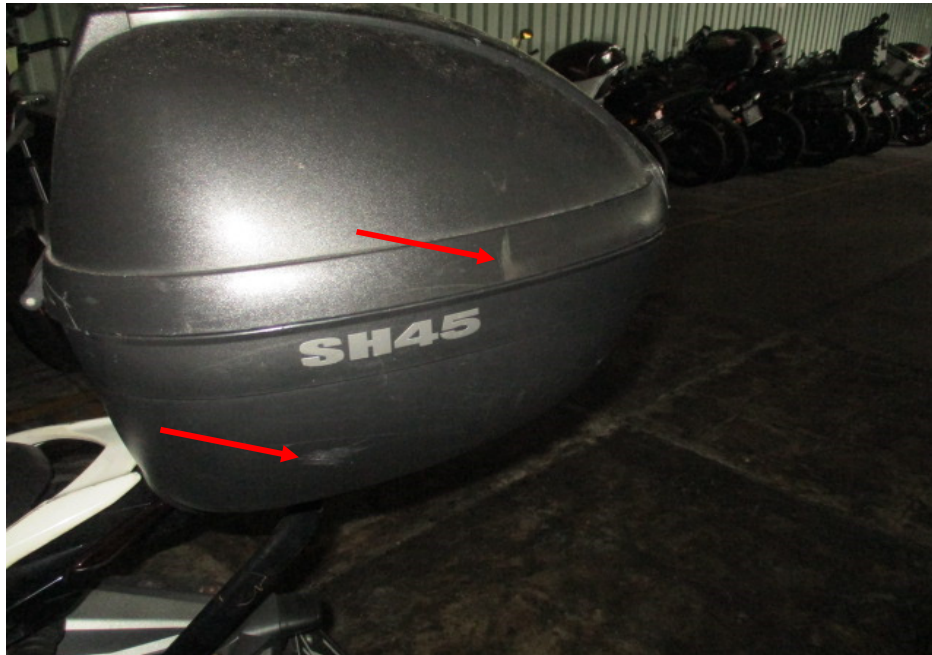
Photo 12 shows the top box of the Motorcycle which sustained damages of grazing nature as a result of the accident (arrowed).
