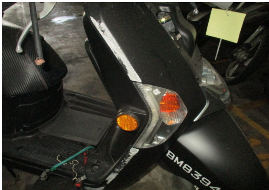
Photo 8 shows the damaged right side cowling of the Motorcycle. The damage sustained was mainly of grazing nature.
