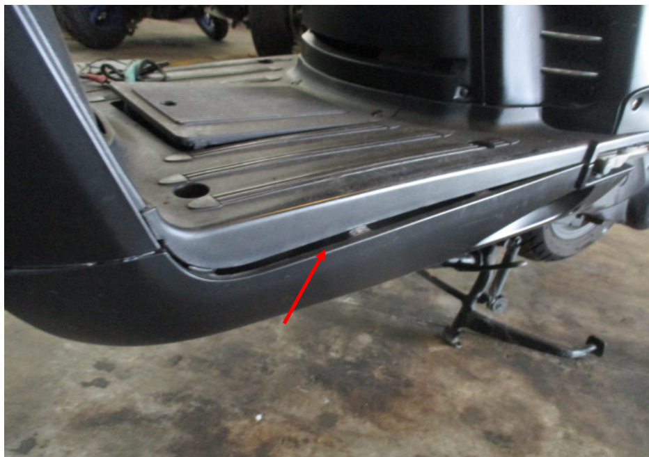
Photo 9 shows a close-up view of the deformed left lower side cowling of the Motorcycle at the time of our inspection (arrowed).
