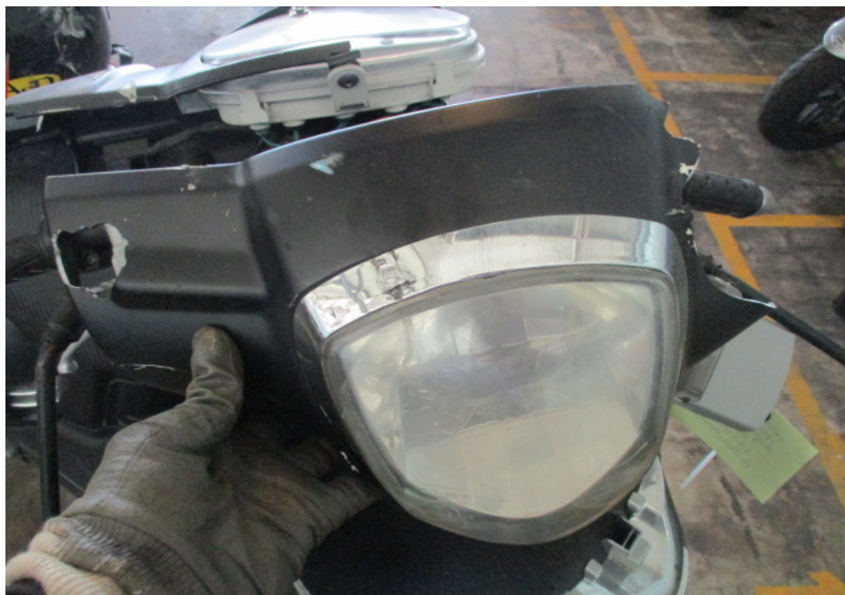
Photo 5 shows a closer view of the broken headlight assembly of the Motorcycle at the time of our inspection.
