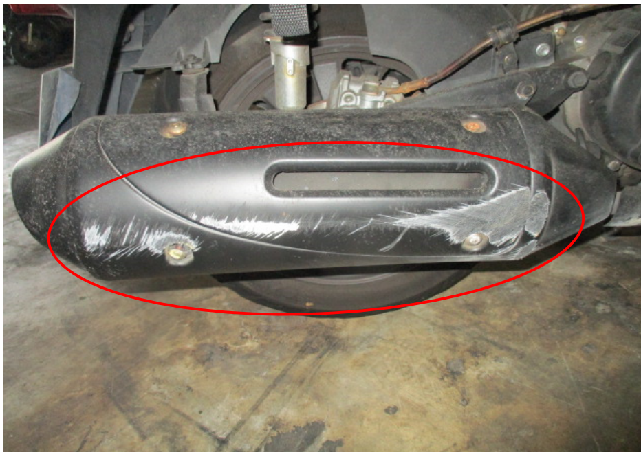
Photo 12 shows a closer view of the damaged exhaust muffler of the Motorcycle at the time of our inspection (circled).
