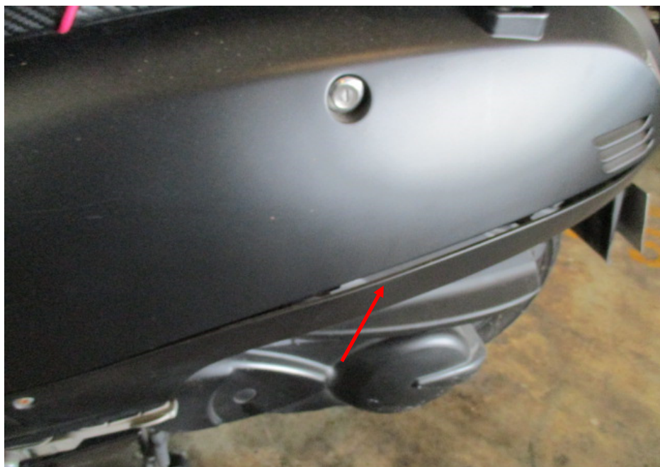
Photo 10 shows a closer view of the deformed left rear side cover of the Motorcycle as a result of the accident (arrowed).
