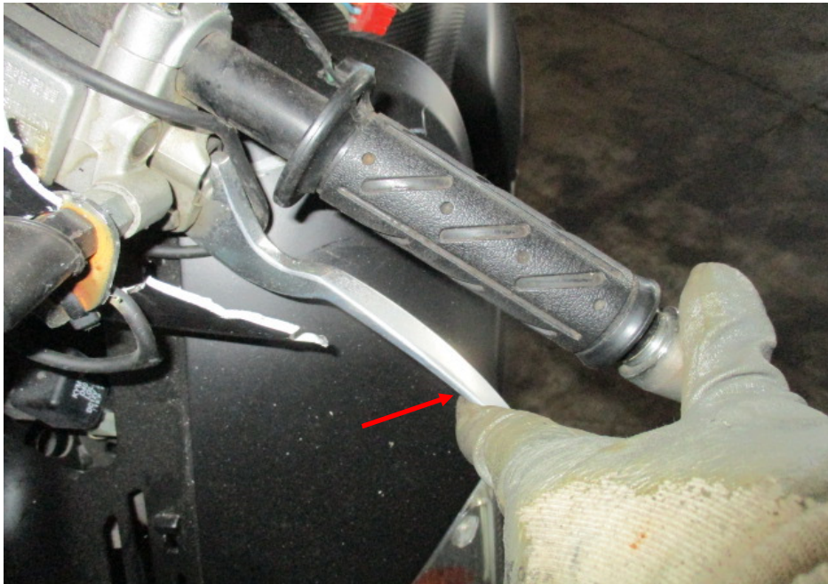
Photo 26 shows the rear brake lever being depressed. There was some resistance felt (spongy like feel) upon pressing the front brake lever (arrowed). This would indicate that there is no leakage of pressure/vacuum in the brake system.
