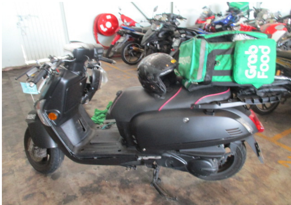
Photo 4 shows a general view of the left body of the Motorcycle at the time of our inspection. The Motorcycle was observed to have sustained damages all around. The body parts that were found to have been damaged include its headlight assembly, front mudguard, front brake lever, right side mirror, right handlebar end, side cowlings, left rear bottom cowlings, rear side covers, top box rack and exhaust muffler, amongst others as a result of the accident.
