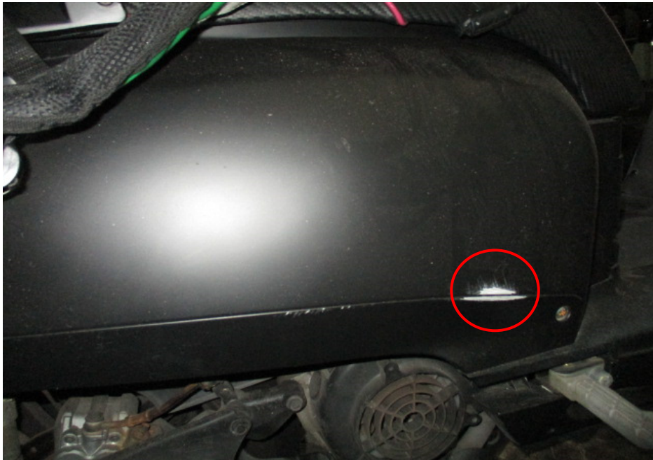
Photo 11 shows a closer view of the right rear side cover of the Motorcycle which sustained damages of grazing nature as a result of the accident (circled).
