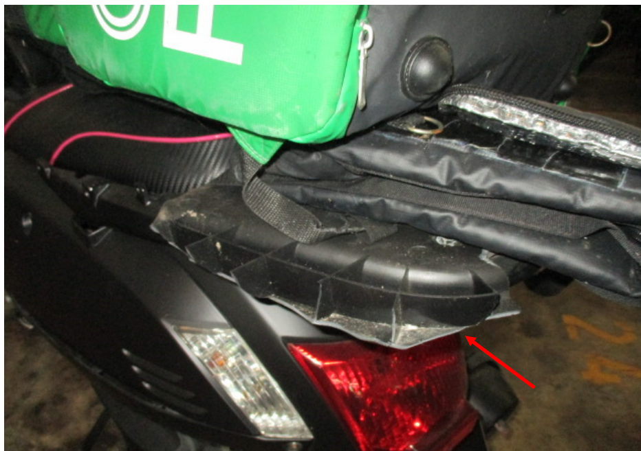
Photo 13 shows a closer view of the cracked top box rack of the Motorcycle as a result of the accident (arrowed).
