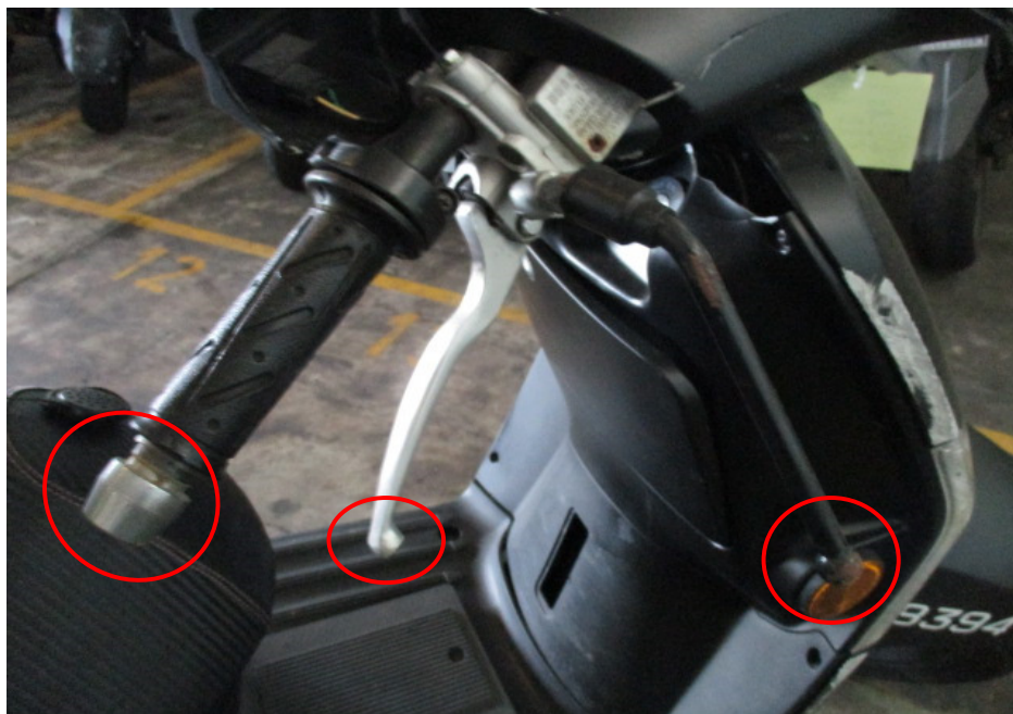
Photo 7 shows a closer view of the right side mirror, right handlebar end and front brake lever of the Motorcycle which were observed to be damaged due to the accident (circled).
