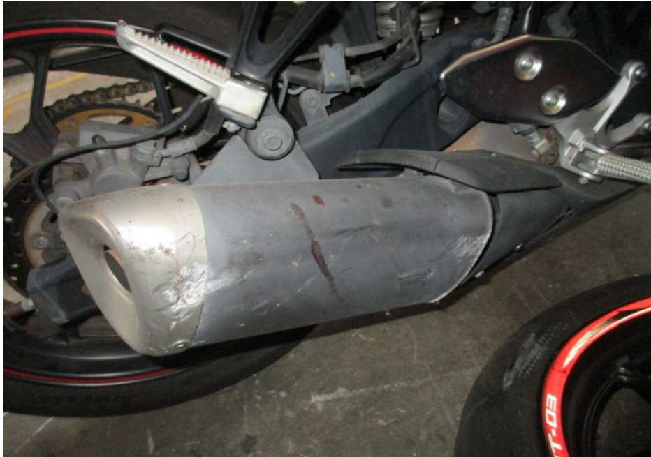
Photo 12 shows a closer view of the exhaust muffler which was amongst the body parts of the Motorcycle that had sustained damages of grazing nature as a result of the accident.
