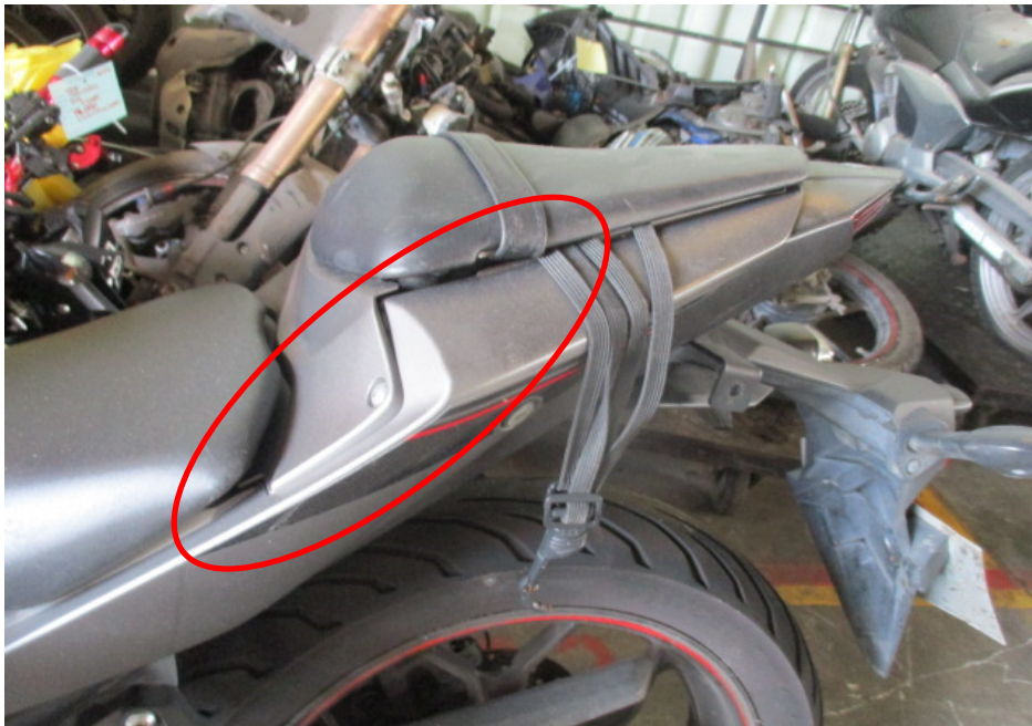
Photo 11 shows the deformed left rear side cover of the Motorcycle as a result of the accident (circled).
