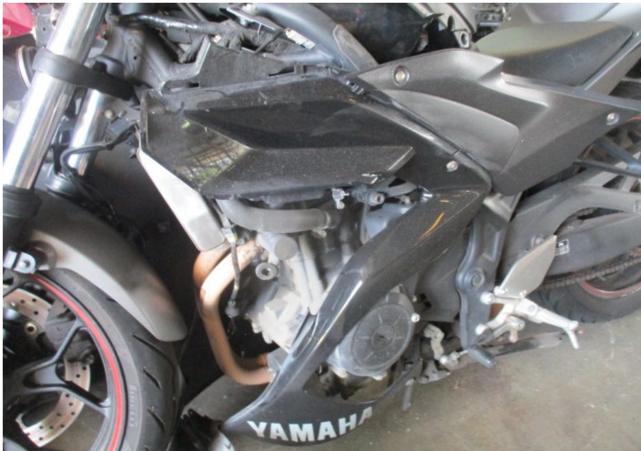
Photo 7 shows a closer view of the cracked left cowling of the Motorcycle as a result of the accident.
