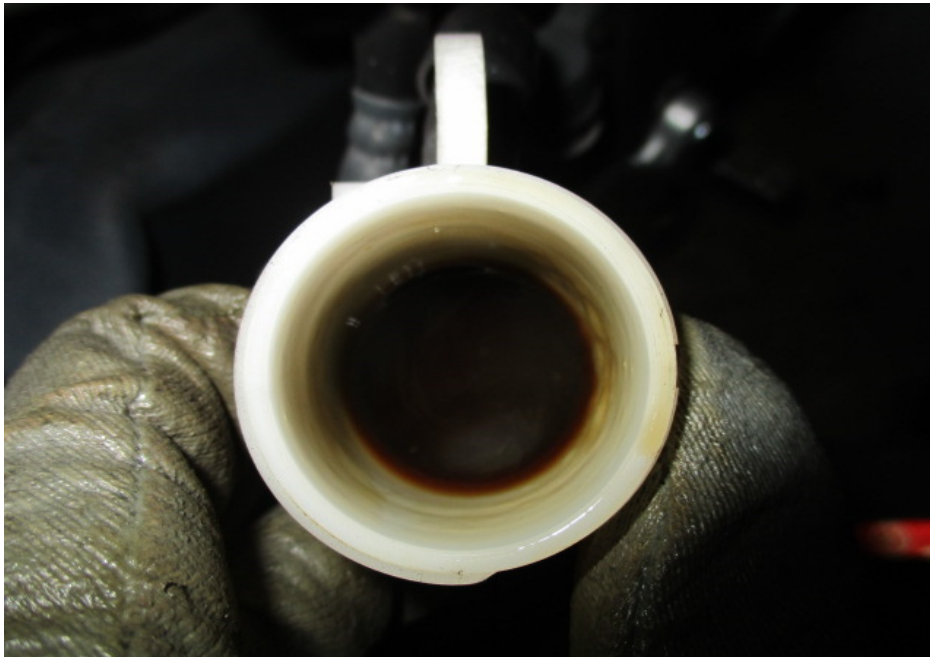
Photo 26 shows the brake fluid reservoir for the rear brake of the Motorcycle. The brake fluid was observed to be of sufficient level and without contamination for operational purposes.
