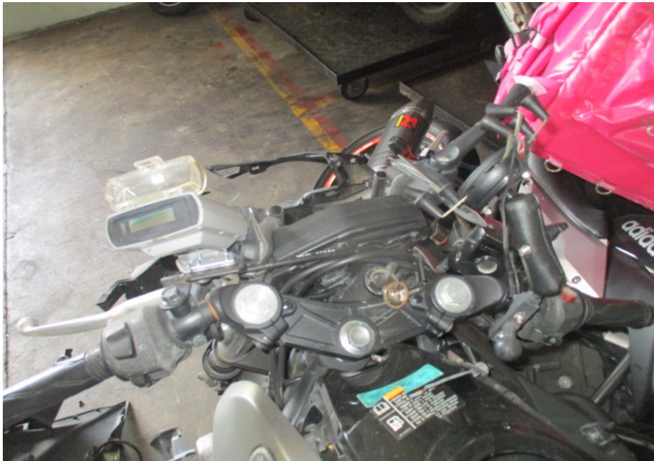
Photo 8 shows a closer view of the handlebar, front brake lever, side mirrors and clutch lever which were amongst the body parts of the Motorcycle that had sustained damage as a result of the accident.
