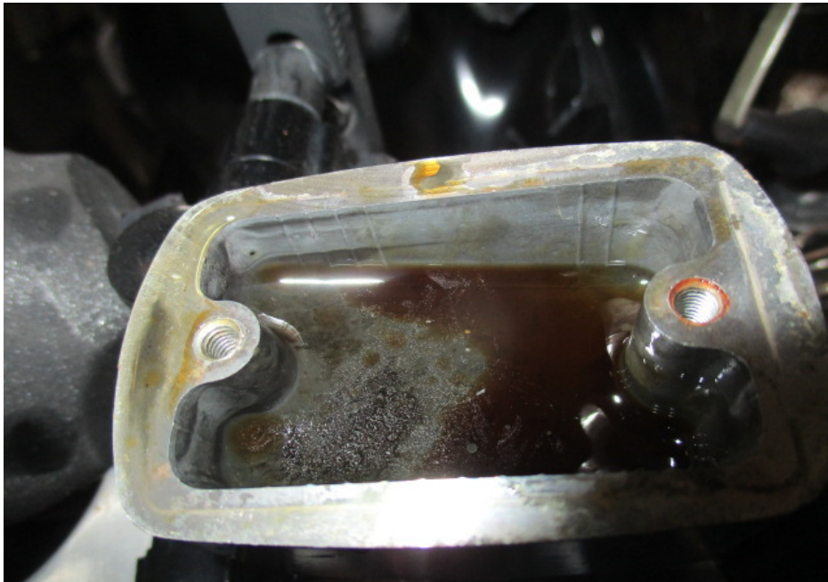
Photo 23 shows the brake fluid reservoir for the front brake of the Motorcycle. The brake fluid was observed to be of sufficient level for operational purposes and without contamination.
