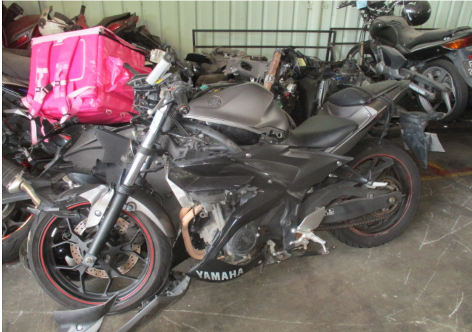
Photo 4 shows a general view of the left body of the Motorcycle at the time of our inspection. The Motorcycle was observed to have sustained damages all around. Amongst the body parts that were found to have been damaged include its head cowl, front mudguard, side cowlings, handlebar, side mirrors, petrol tank, right pillion footrest, left rear side cover and exhaust muffler, amongst others.
