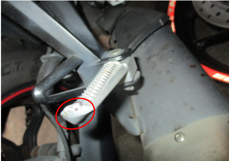
Photo 10 shows a closer view of the right pillion foot peg (circled) which was amongst the body parts of the Motorcycle that had sustained damage as a result of the accident.
