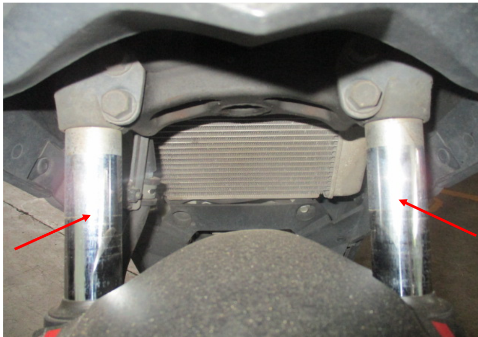
Photo 16 shows the front fork (arrowed) of the Motorcycle. The front fork and fork bracket of the Motorcycle were both found to be intact and undamaged. Turning the Motorcycle's handle bar towards the left and right did not produce any abnormal free play. The steering system of the Motorcycle was in serviceable condition at the time of our inspection.
