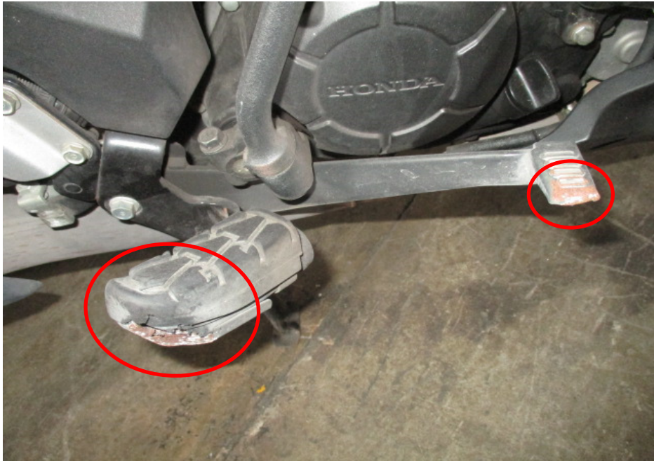
Photo 8 shows a closer view of the rear brake pedal and right front footrest (circled) which were amongst the body parts of the Motorcycle that had sustained damage as a result of the accident.
