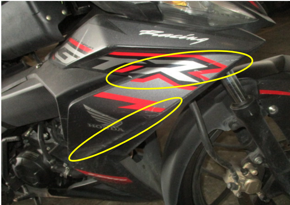
Photo 6 shows a closer view of the right cowling (circled) which was amongst the body parts of the Motorcycle that had sustained damage as a result of the accident.
