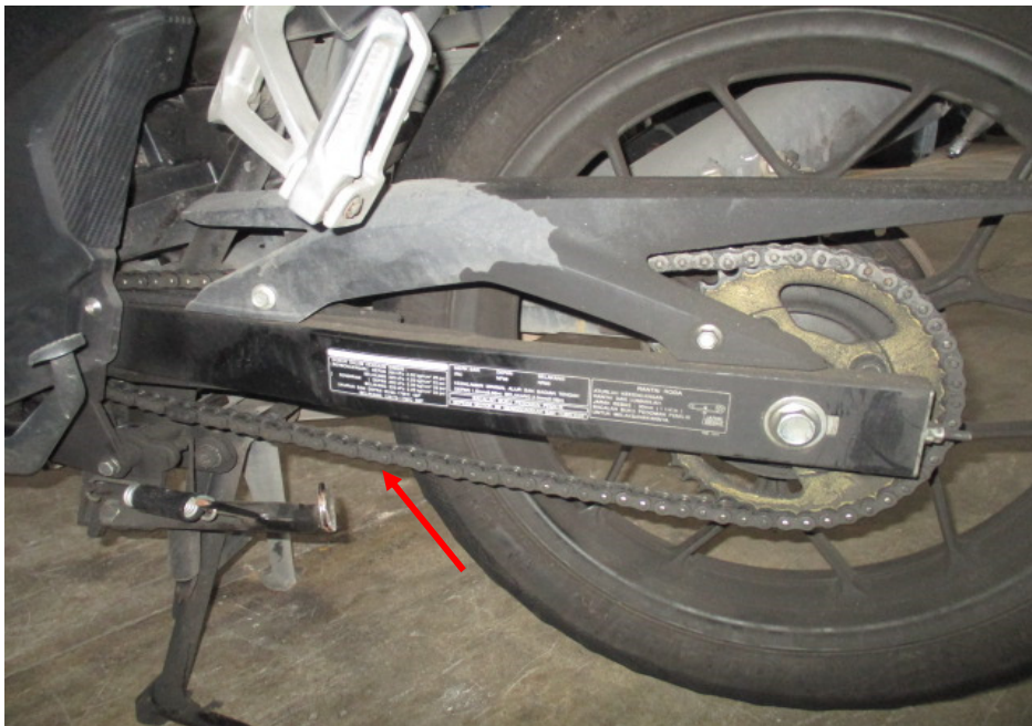
Photo 14 shows the general view of the gear train (arrowed) of the Motorcycle, which was observed to be intact with no misalignment. It was also adequately lubricated for operating purposes.
