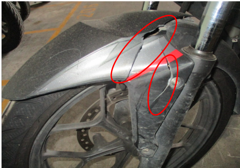
Photo 5 shows a closer view of the cracked front mudguard (circled) of the Motorcycle as a result of the accident.
