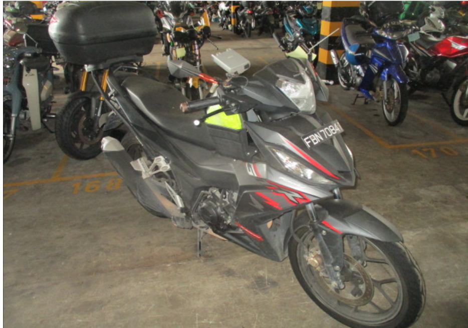
Photo 4 shows a general view of the right body of the Motorcycle at the time of our inspection. The Motorcycle was observed to have sustained damages along its frontal portion and right body. Amongst the right cowling, front mudguard, front brake lever, right side mirror, right handlebar end, rear brake pedal, right front footrest and exhaust muffler, amongst others.
