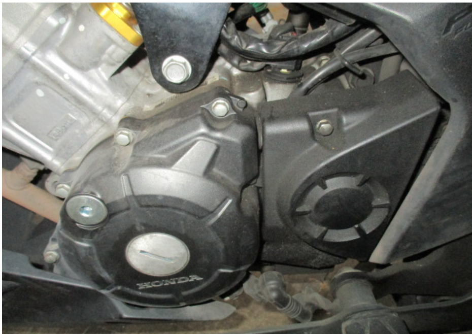
Photo 12 shows the left side of the engine of the Motorcycle at the time of our inspection. The various engine related parts and components were found to be intact with no visible damage. There was also no sign(s) or indication(s) of fluid leak observed around the left engine area of the Motorcycle.
