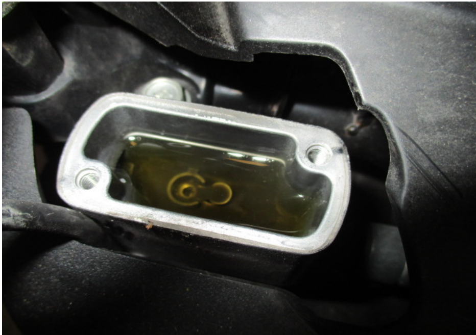
Photo 20 shows the brake fluid reservoir for the front brake of the Motorcycle. The brake fluid was observed to be of sufficient level and without contamination for operational purposes.
