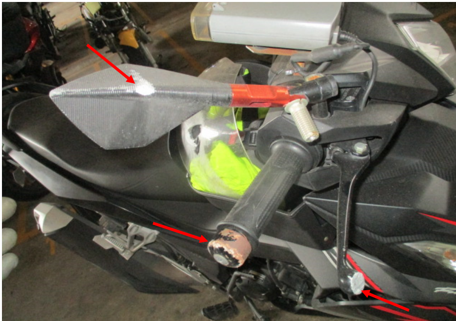
Photo 7 shows the front brake lever, right handlebar end and right side mirror (arrowed), which were amongst the body parts of the Motorcycle that had sustained damage as a result of the accident.
