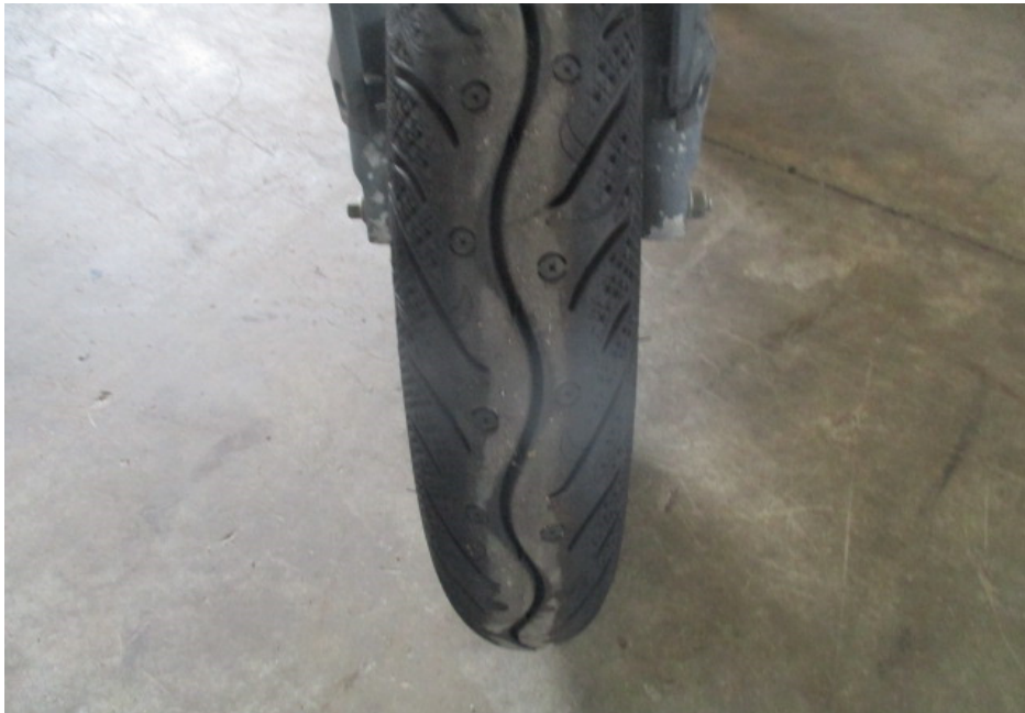
Photo 10 shows the front tyre of the Motorcycle at the time of our inspection. The front tyre was observed to be in serviceable condition with remaining tread depth of approximately 4mm. The pattern of the tread was also clearly visible. There was no tear, burst mark(s) and/or punctured hole(s) on the sidewalls as well as across the tread of the front tyre.
