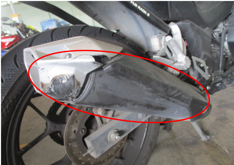
Photo 9 shows the exhaust muffler and exhaust muffler heat shield (circled) of the Motorcycle that had sustained damage as a result of the accident.
