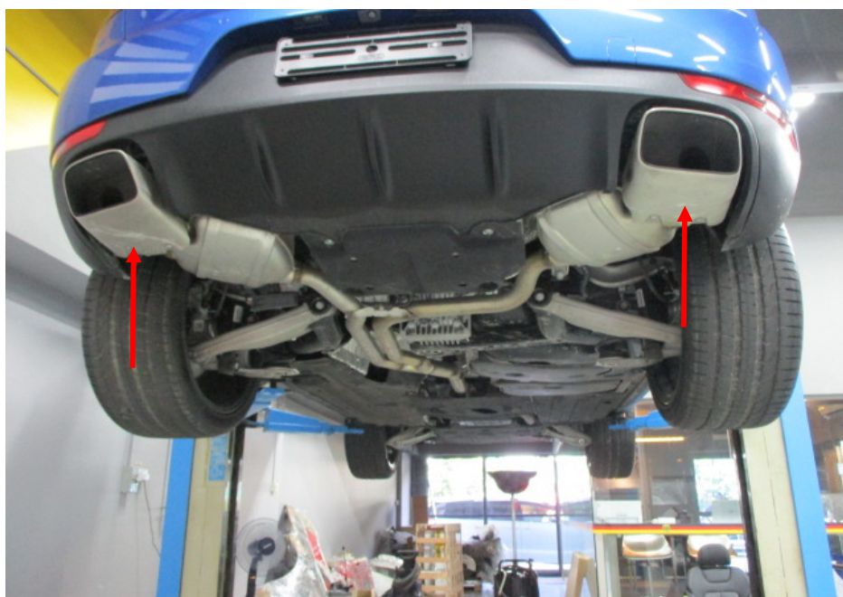
Photo 20 shows the Motor Car's rear mufflers (arrowed). My examination of the Motor Car's exhaust system revealed no sign(s) or indication(s) of any cut or weld marks along its exhaust pipes and on its catalytic converters.
