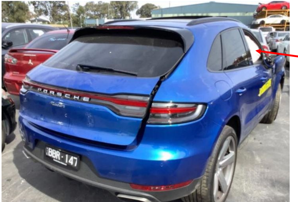
Photo 3 shows the rear right body of the Motor Car prior to any repairs being carried out (photograph provided to me). The right side curtain airbag was observed to be deployed (arrowed).
