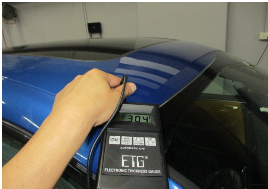
Photo 9 shows measurement being carried out to the thickness of the paint at the right side front of the Motor Car's roof panel. This area of the roof panel was observed to be damaged (refer to photograph 1 above). The reading of the paint thickness was recorded at 304micron. The readings obtained at the left and right front of the Motor Car's roof panel were relatively close, which indicates that the roof panel was replaced.
