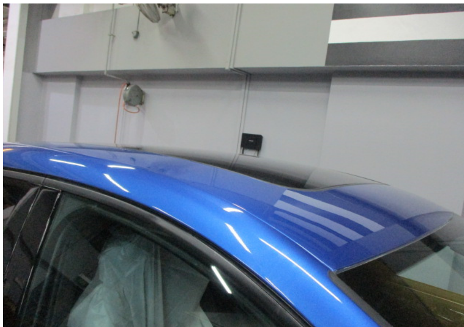
Photo 7 shows the roof panel of the Motor Car at the time of my inspection. The roof panel of the Motor Car were visually examined, and it was observed that the repair/restoration works carried out to the damaged area of the Motor Car were reasonably adequate and in order
