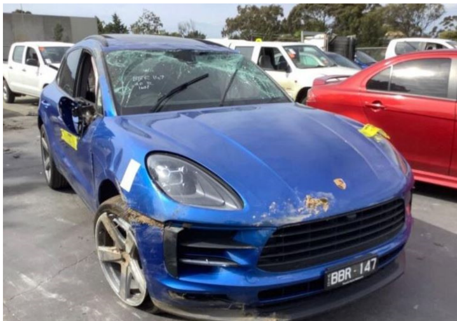
Photo 1 shows the front right body of the Motor Car prior to any repairs being carried out (photograph provided to me). The Motor Car was observed to have sustained damages at its front right body. The body parts observed to be damaged include its front bumper, front right fender, front right door, right side wing mirror, right side "A" pillar and roof panel amongst others. The front right wheel rim was also observed to be broken.
