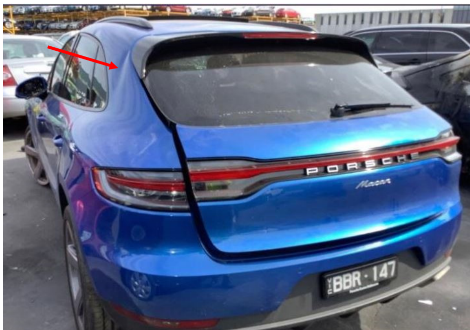
Photo 2 shows the rear left body of the Motor Car prior to any repairs being carried out (photograph provided to me). The rear left fender was observed to be dented (arrowed).
