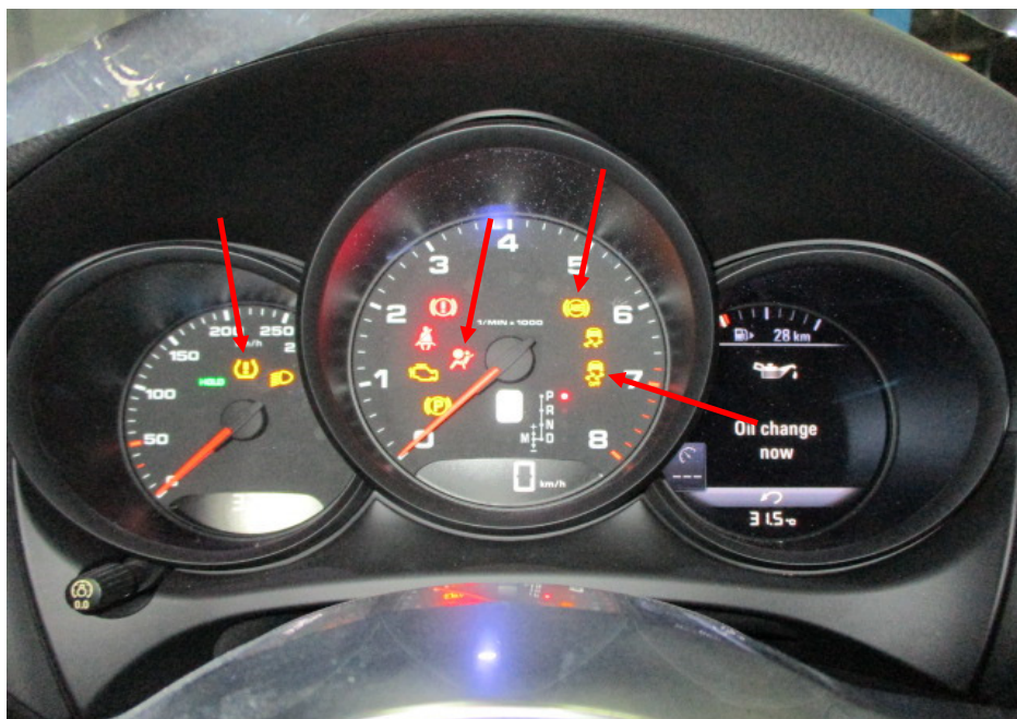
Photo 14 shows the warning lights for the various electronic safety features appearing on the instrument panel of the Motor Car during its self-test when the engine is cranked, in particular the ABS, SRS, TPM and TCS lights (arrowed).
