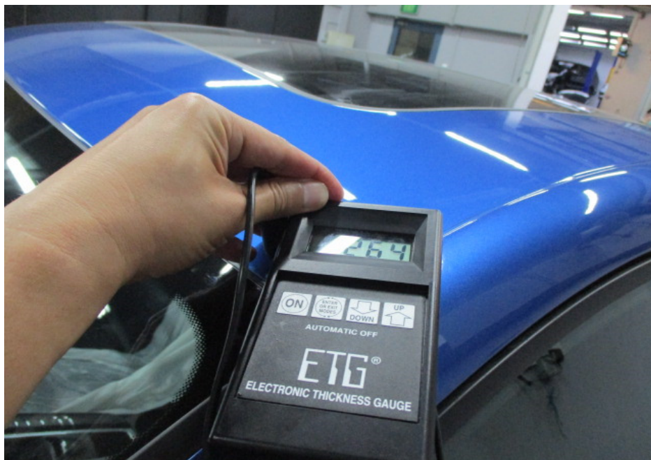
Photo 8 shows measurement being carried out to the thickness of the paint at the left side front of the Motor Car's roof panel. This area of the roof panel was observed to be damaged (refer to photograph 1 above). The reading of the paint thickness was recorded at 264micron.
