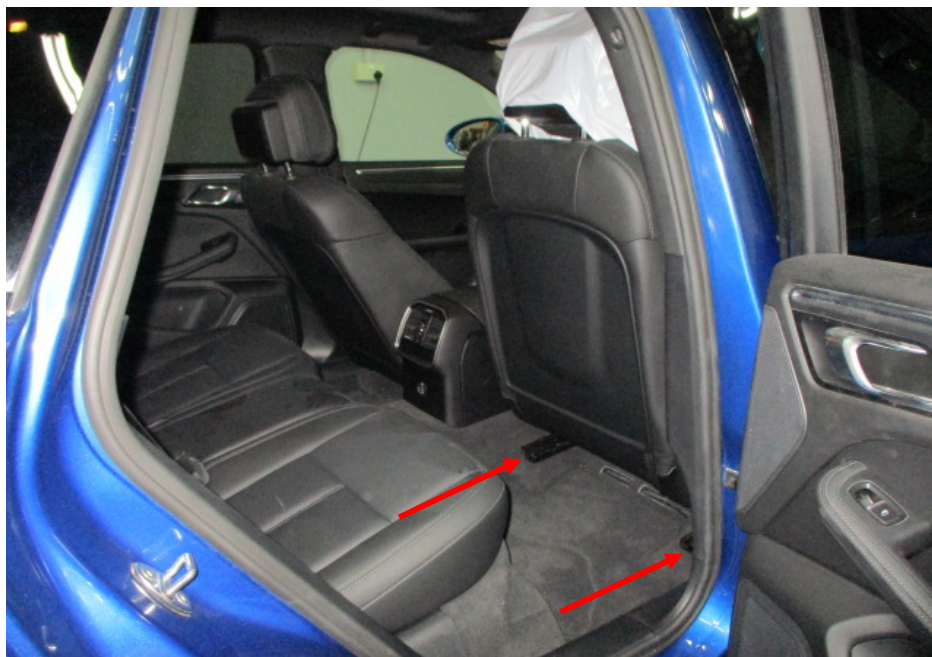
Photo 13 shows the seats of the Motor Car, which were secured via seat rails (arrowed) to the floor board. All the seats of the Motor Car were fitted with a retractable seat belt reel and pre-tensioner. The seat belts were tested and able to be fastened into the respective pre-tensions that were fitted on the side of each individual seat.
