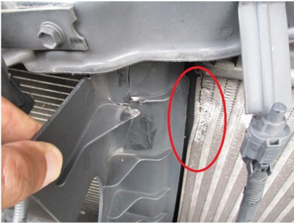
Photo shows the intercooler's side edge bent/dented with fresh damage to the fins after the taxi's front bumper was dismantled in surveyor's presence.
