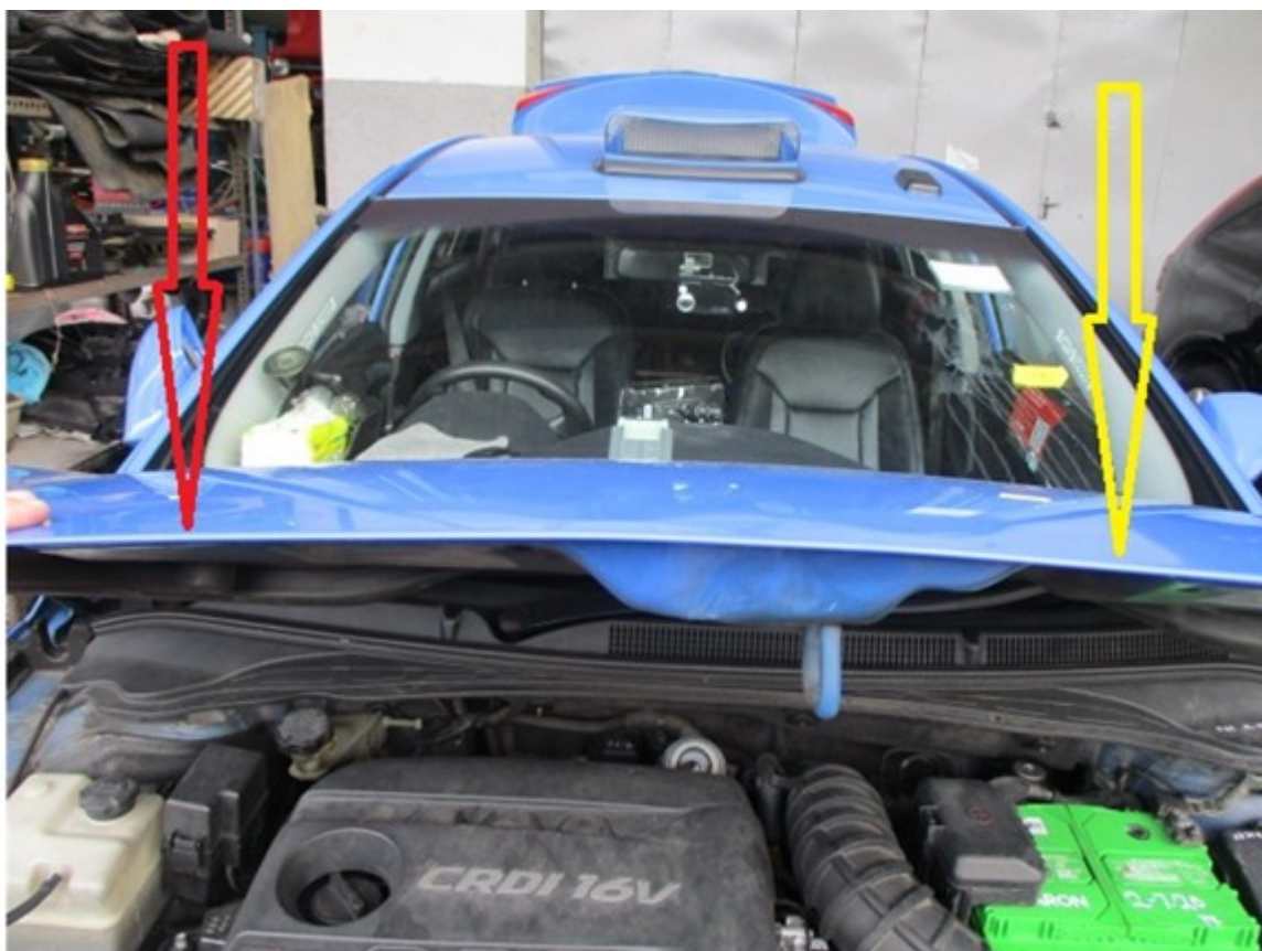
Photo show the right side of the front bonnet (red arrow) higher than the left side (yellow arrow) at the leading edge of the front bonnet. Panel beating at the edge may distort the original shape of the front bonnet and result in uneven alignment when re-fit.
