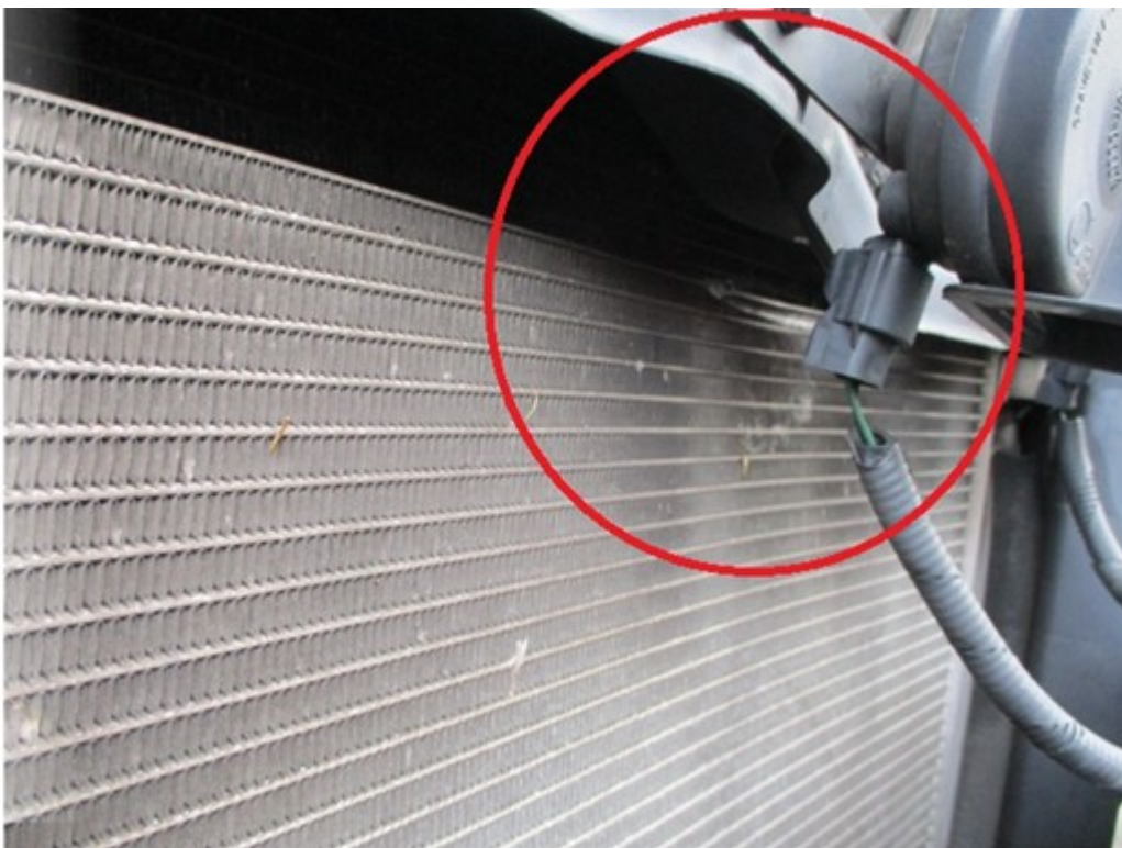
Photo shows the aircon condenser bent at the top centre area after the taxi's front bumper was dismantled in surveyor's presence.
