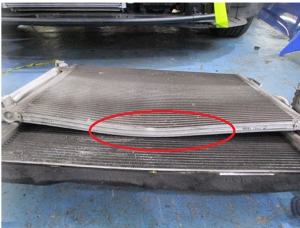
Photo show the aircon condenser bent at the top centre area. The bent aircon condenser had contacted onto the radiator leading to the damage of the radiator fins.
