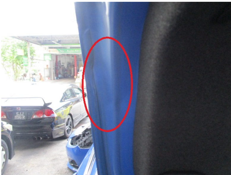
Photo show inner left side of rear bootlid dented. The dented area was at the contour of the rear bootlid, which made panel beating difficult.
