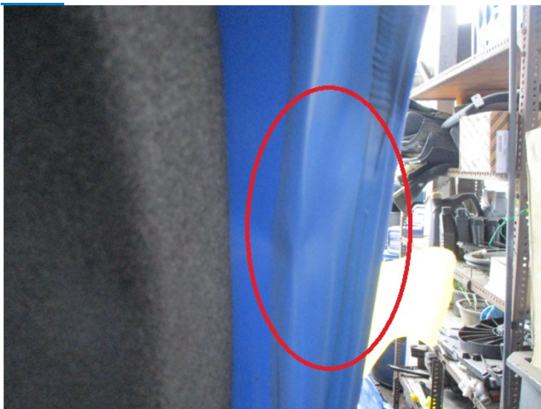
Photo show inner right side of rear bootlid dented. The dented area was at the contour of the rear bootlid, which made panel beating difficult.
