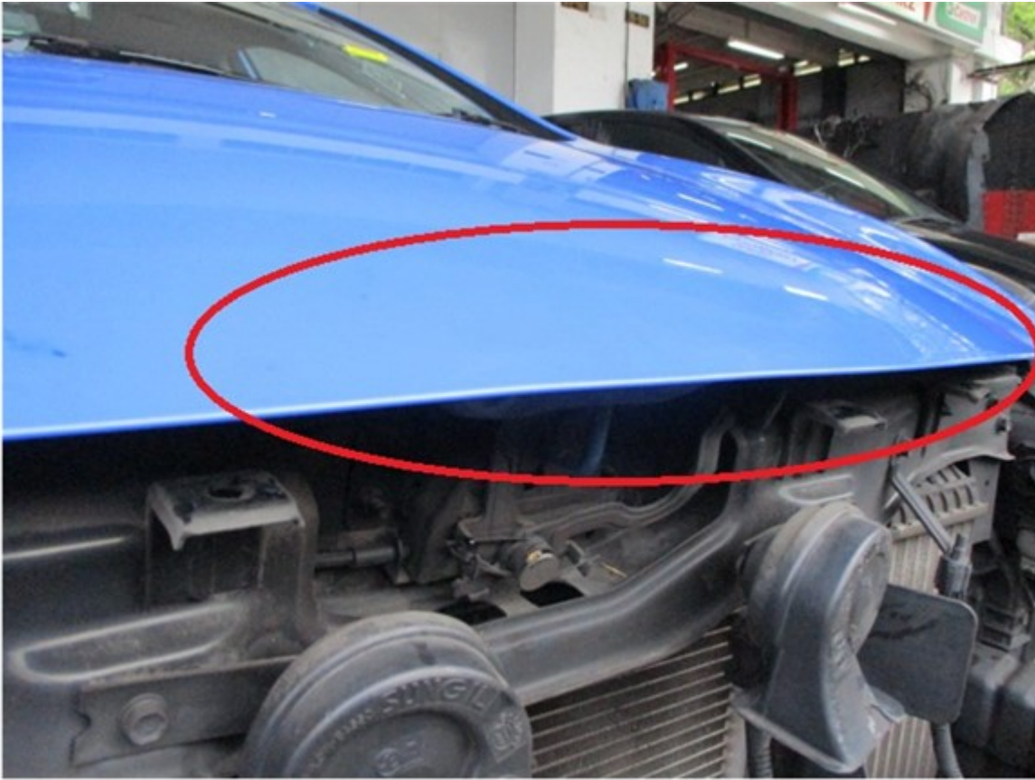
Photo show another view of the front bonnet bent.
