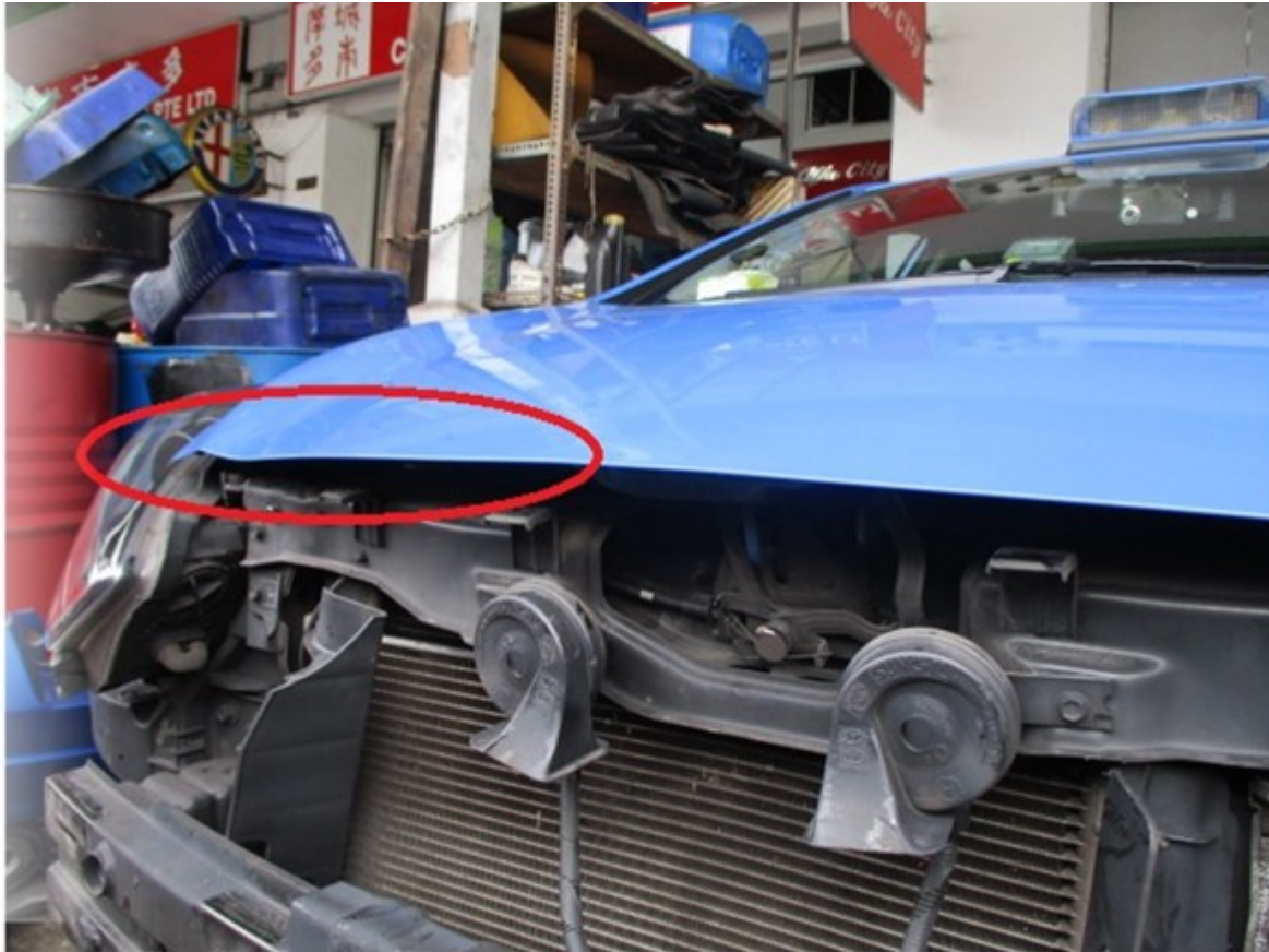
Photo show the front bonnet bent at the leading edge. Panel beating at the edge may distort the original shape of the front bonnet and result in uneven alignment when re-fit.
