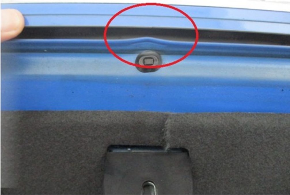
Photo show rear bootlid bent due to the rear end panel pushed inwards.
