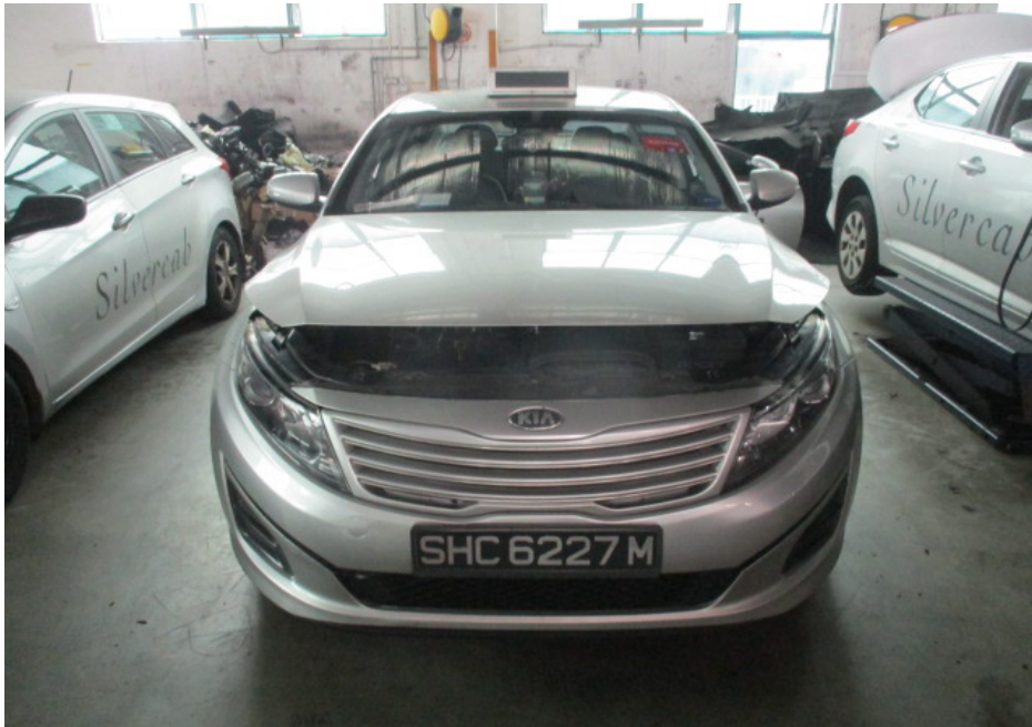
Photo 1 shows the general view of the front portion of the Insured Vehicle at the time of our inspection. The fire damage to the Insured Vehicle was confined to its front portion. Its front bonnet, front windscreen and side panels were amongst the body parts that were found to have been affected as a result of the fire.
