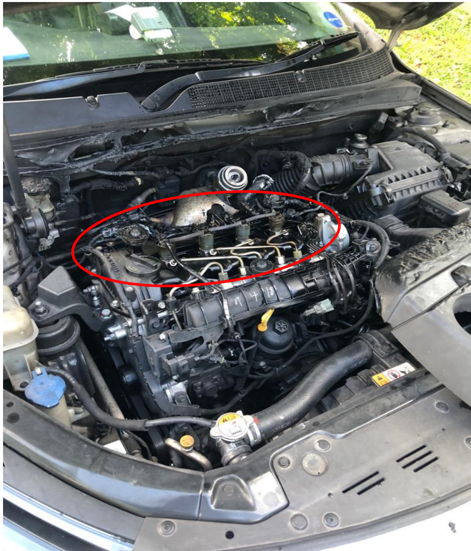
Photo 16 shows the Insured Vehicle at the incident scene after the fire was extinguished. In general, the information that could be gathered from this photograph had corresponded to the events that were related to us by Mr Teng, which is the fire had started in the rear centre portion of the engine compartment (circled).
