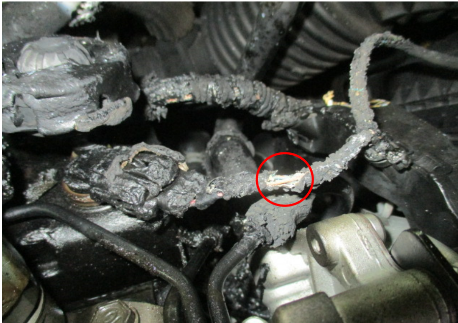
Photo 11 shows a closer view of the greenish residue found on some of the burnt stretches of original factory fitted wirings (circled). The presence of such greenish residue suggests occurrence of an electrical short circuit.
