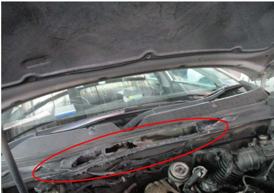
Photo 9 shows a close up view of the melted wiper panel found upon our inspection of the Insured Vehicle (circled).
