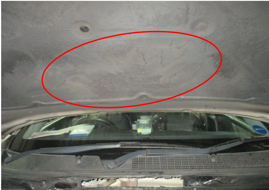
Photo 8 shows a close up view of the cracks in the insulating material on the underside of the front bonnet of the Insured Vehicle (circled).
