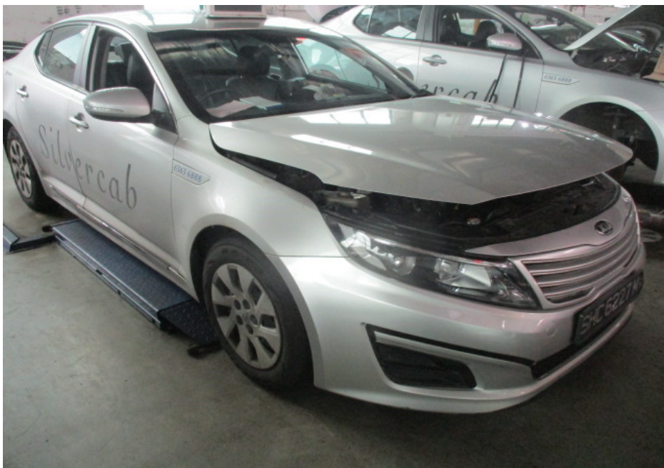
Photo 2 shows the general view of the right body of the Insured Vehicle at the time of our inspection. The exterior body of the Insured Vehicle had sustained visible fire damage. This included its front windscreen, front bonnet and right front panel.
