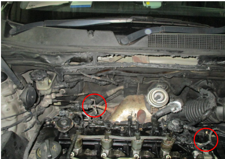
Photo 10 shows the original factory fitted wirings around the rear centre portion of the engine compartment, which is in the immediate vicinity where the fire to the Insured Vehicle had likely started. We had found greenish residue on several burnt stretches of these wirings (circled). The presence of such greenish residue indicates internal heating of copper wires, a sign of an electrical short circuit occurring. The greenish residue is normally left behind from oxidation as a result of chemical reaction involving the copper wires.
