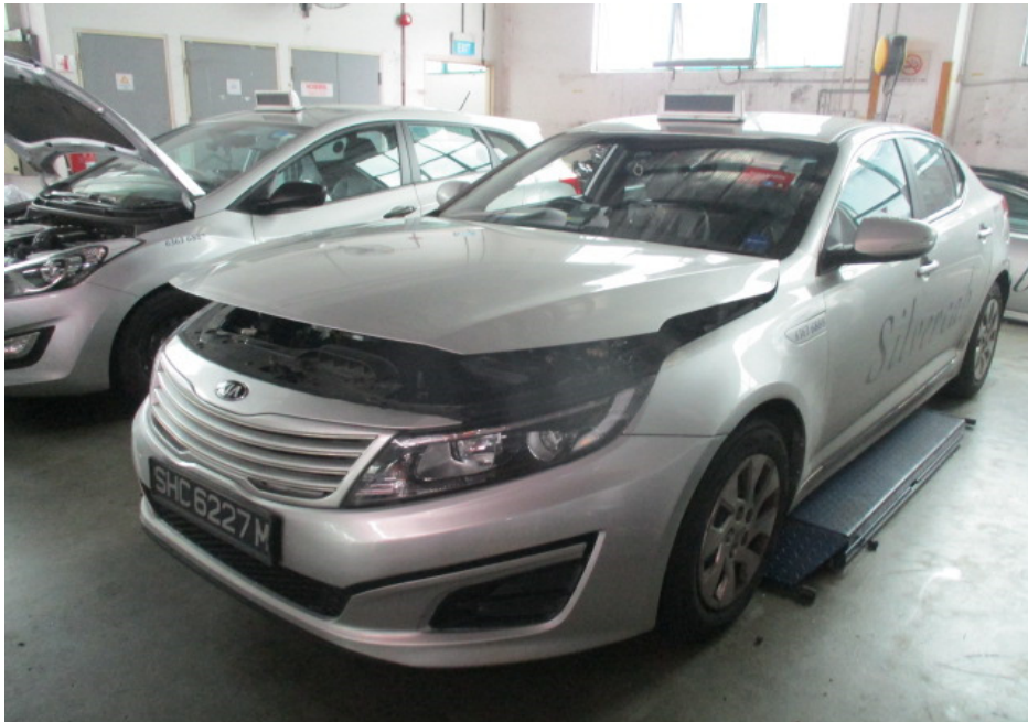
Photo 3 shows the general view of the left body of the Insured Vehicle at the time of our inspection. The exterior body of the Insured Vehicle had sustained visible fire damage. This included its front windscreen, front bonnet and left front panel.
