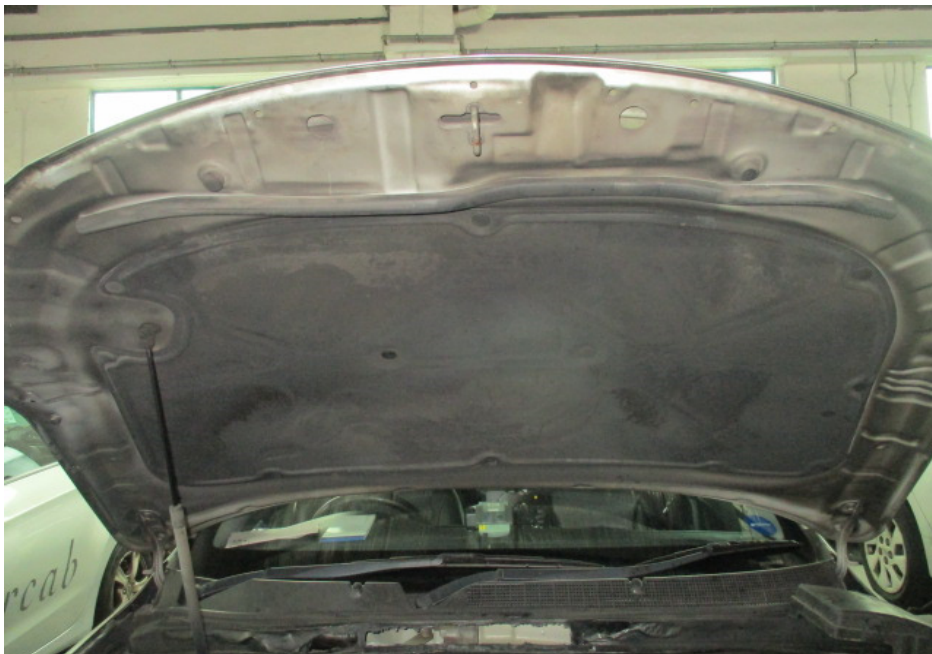
Photo 4 shows a closer view of the underside of the front bonnet of the Insured Vehicle at the time of our inspection. The fire damage to the Insured Vehicle was confined to its front portion. Its insulating material on the underside of the front bonnet was amongst the body parts that were found to have been affected by the fire.
