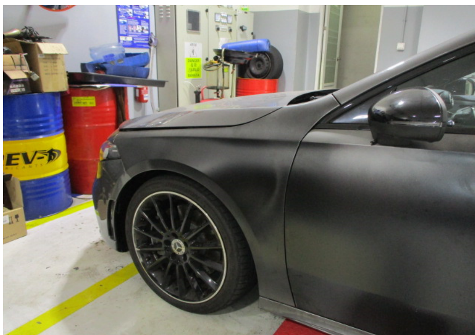
Photo 6 shows a newly replaced left front fender and left front door of the Motor Car. The body parts along the left side front of the Motor Car were visually examined and it was observed that the repair/restoration works carried out to the damaged area of the Motor Car (refer photograph 1 above) were reasonably adequate and in order.
