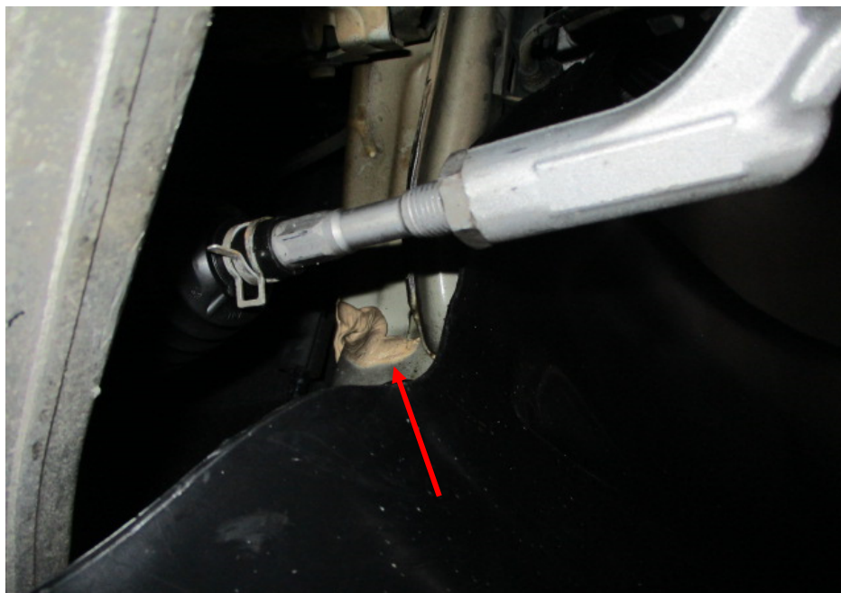
Photo 19 shows the chassis/structural body at the underside front left of the Motor Car. Visually, I did not find any weld marks other than original spot weld marks on the chassis/structural body of the Motor Car. The original factory sealant (arrowed) at the joints along the chassis/structural body was also untouched, indicating no work was done on the chassis/structural body of the Motor Car and that the chassis/structural body was originally fitted.
