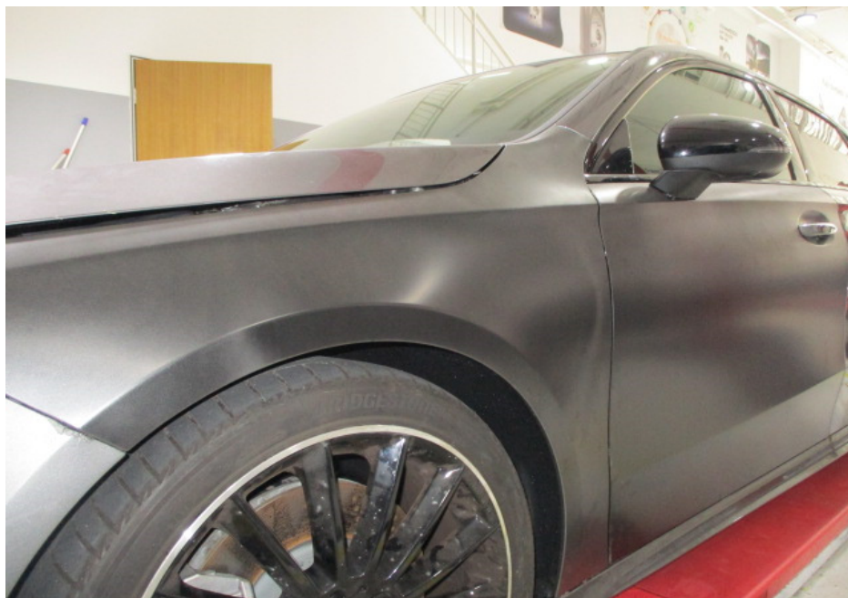
Photo 5 shows a newly replaced left front fender and left front door of the Motor Car. The body parts along the left side front of the Motor Car were visually examined and it was observed that the repair/restoration works carried out to the damaged area of the Motor Car (refer photograph 1 above) were reasonably adequate and in order.
