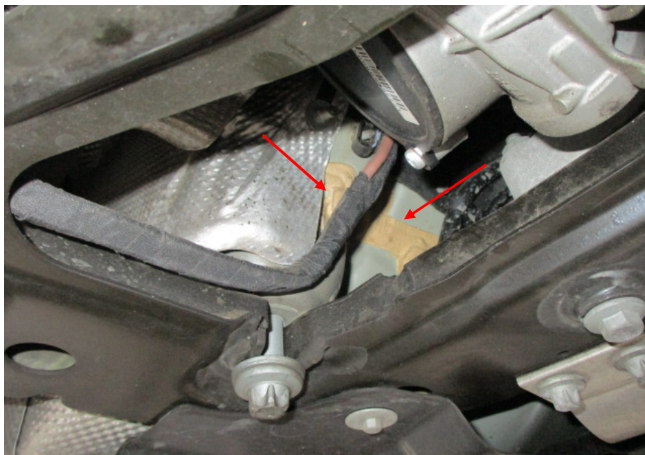
Photo 21 shows the floor board at the underside left front of the Motor Car. The original factory sealant (arrowed) at the joints along the non-detachable body panels were untouched, indicating no work was done on the non-detachable body panels of the Motor Car; and that these body panels were originally fitted.
