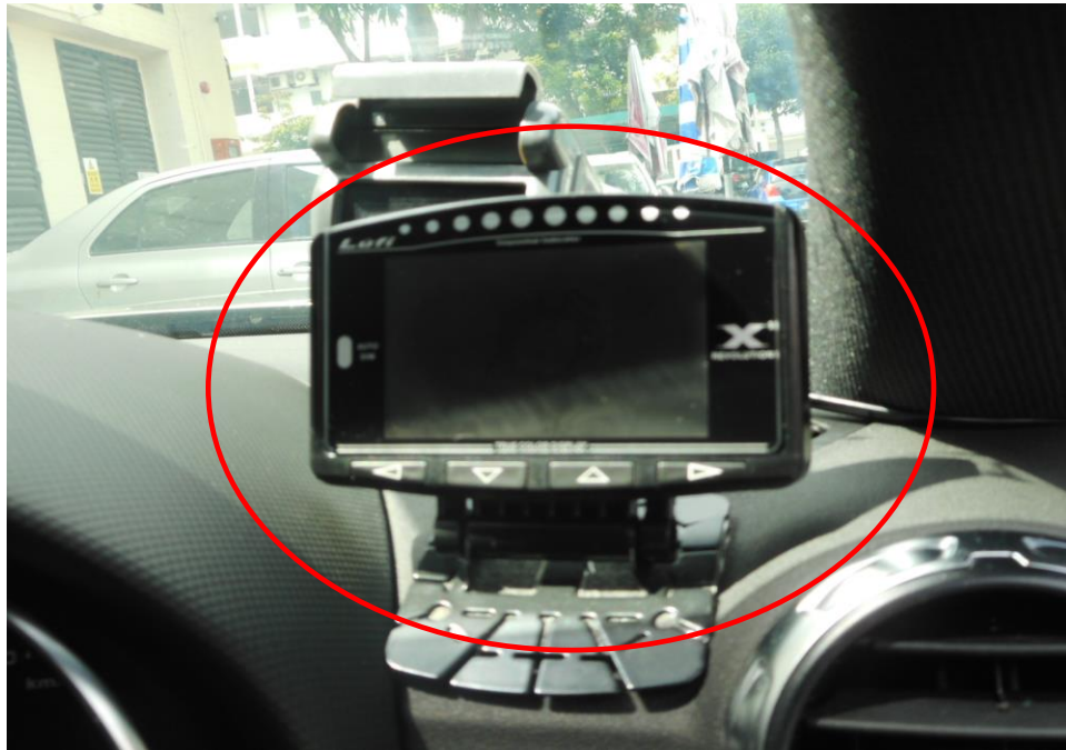
Photo 9 shows an aftermarket monitoring gauge (circled) on the Insured Vehicle, which was observed to be unaffected by the fire.
