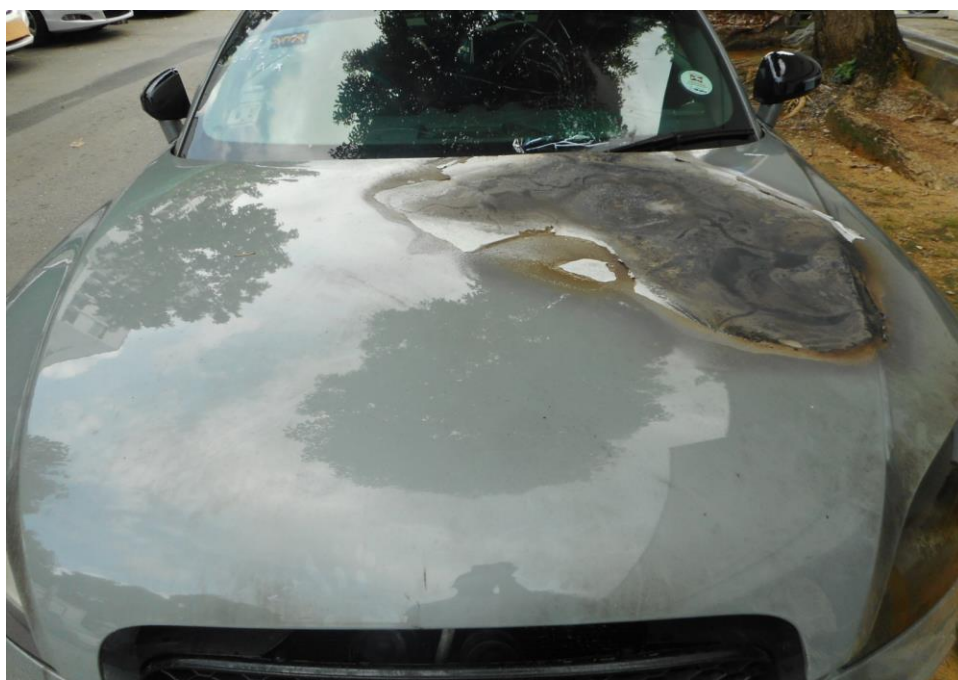
Photo 13 shows the top of the front bonnet cover of the Insured Vehicle at the time of our inspection. The high heat intensity burn marks (whitish burn marks) and rust that had development on the left exterior surface of the bonnet indicates that the fire had originated from the left engine compartment portion of the Insured Vehicle.
