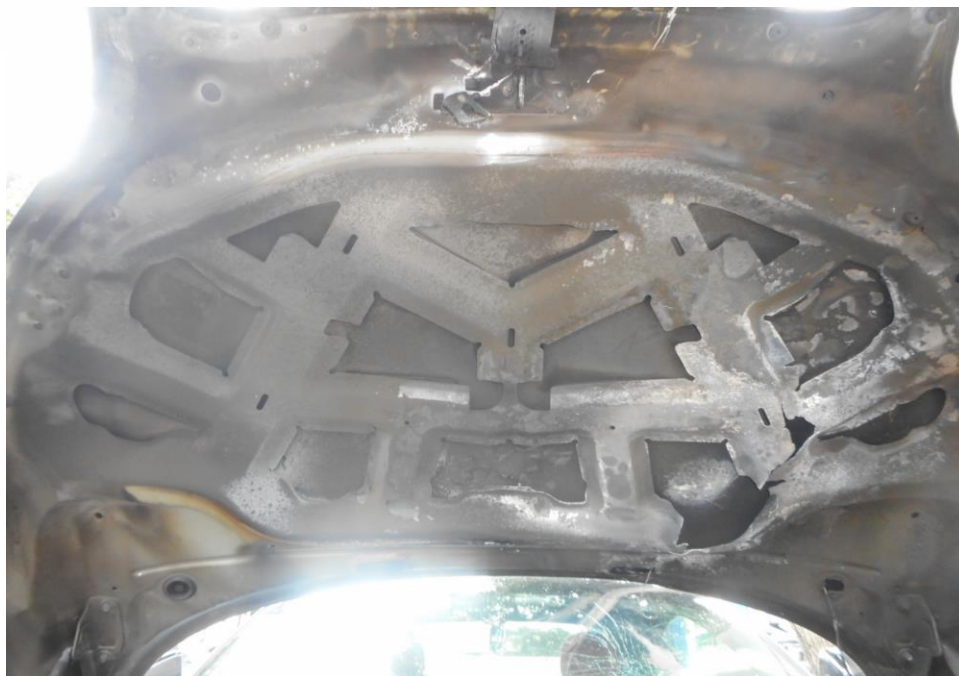
Photo 14 shows the underside of the front bonnet cover of the Insured Vehicle at the time of our inspection. The High heat intensity burn marks (whitish burn marks) and rust that had development found on the exterior surface of the bonnet indicates that the fire had originated from the left engine compartment portion of the Insured Vehicle.
