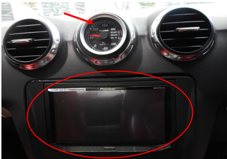
Photo 8 shows an aftermarket audio head unit (arrowed) and monitoring gauge (circled) on the Insured Vehicle, which was observed to be unaffected by the fire.
