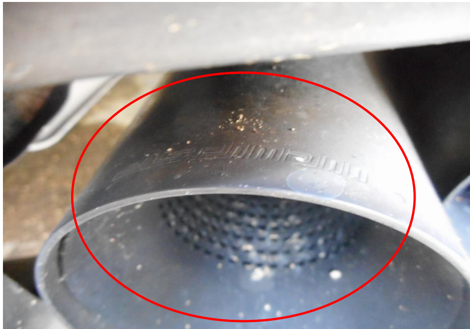
Photo 12 shows a set of aftermarket exhaust system (circled) on the Insured Vehicle, which was observed to be unaffected by the fire.
