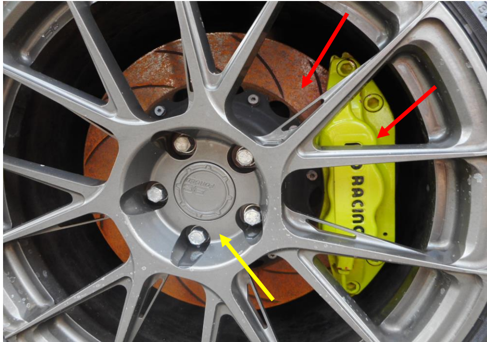
Photo 11 shows an aftermarket rim (yellow arrow) and upgraded brake caliper and disc brake (red arrow) on the Insured Vehicle, which was observed to be unaffected by the fire.
