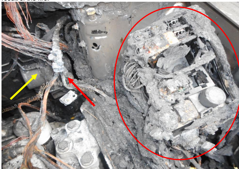
Photo 16 shows the close up view of the front right engine compartment portion of the Insured Vehicle at the time of our inspection. The fire damage to the Insured Vehicle was confined to its engine compartment portion and. Its fuse box (circled), original wiring harnesses (red arrow) and abs pump (yellow arrow) and was amongst the parts in the compartment that were found to have been affected as a result of the fire.
