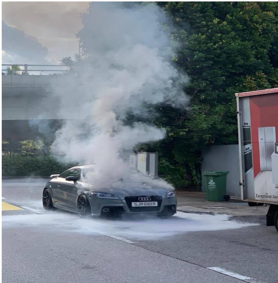
Photo 19 shows the smoke emitting from the front and undercarriage of the Insured Vehicle before the arrival of the SCDF. In general, the information that could be gathered from this photograph had corresponded to the events that were related to us by Mr Lim, location when the fire broke out.
