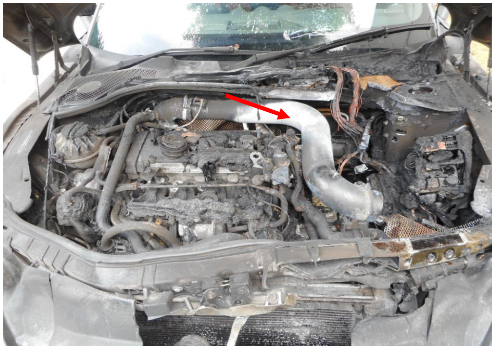
Photo 7 shows an aftermarket air filter pipe (arrowed) on the Insured Vehicle, which was observed to be affected by the fire.
