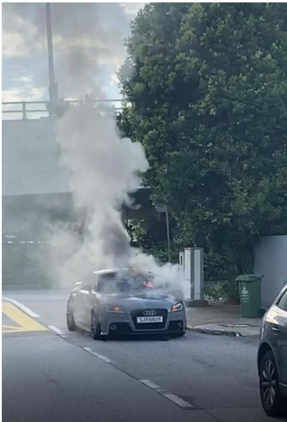
Photo 20 shows the start of the fire at the front left engine compartment of the Insured Vehicle before the arrival of the SCDF. In general, the information that could be gathered from this photograph had corresponded to the events that were related to us by Mr Lim, location when the fire broke out.
