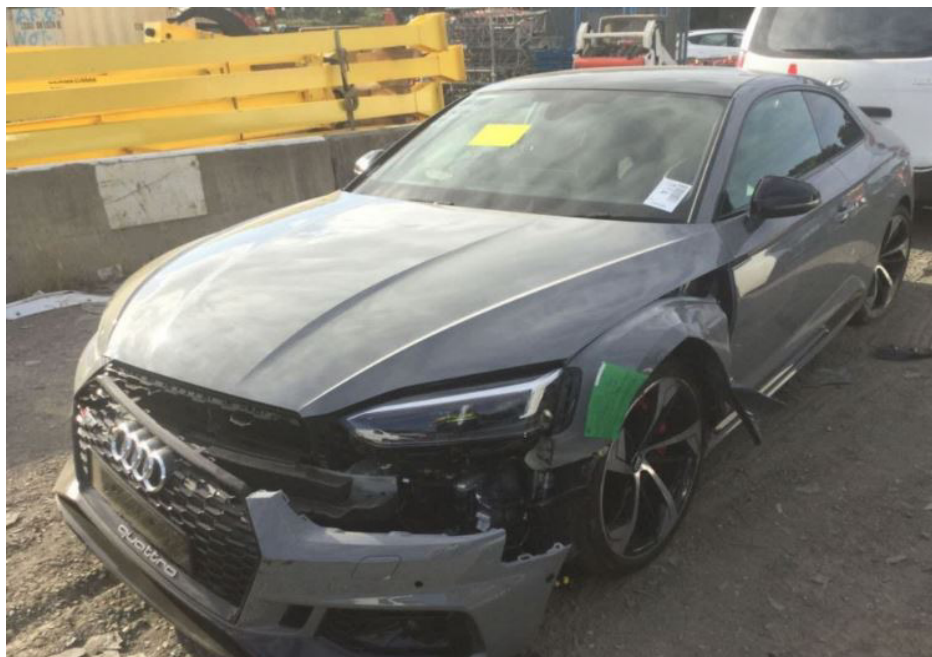
Photo 1 shows the front left body of the Motor Car prior to any repairs being carried out (photograph provided to me). The Motor Car was observed to have sustained damages at its front left body. The body parts observed to be damaged and/or dislodged had included its front bumper, front grille, front left fender and front left wheel rim amongst others.
