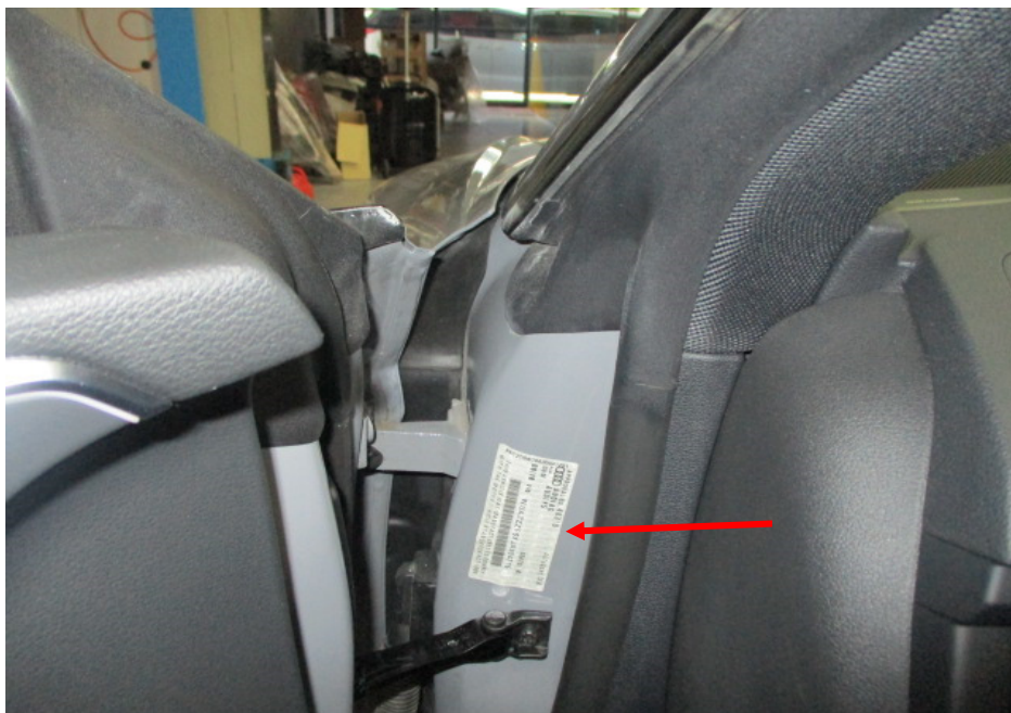
Photo 21 shows the left side "A" pillar of the Motor Car. The original factory label (arrowed) was seen at the left side "A" pillar indicating that the left side "A" pillar was originally fitted.
