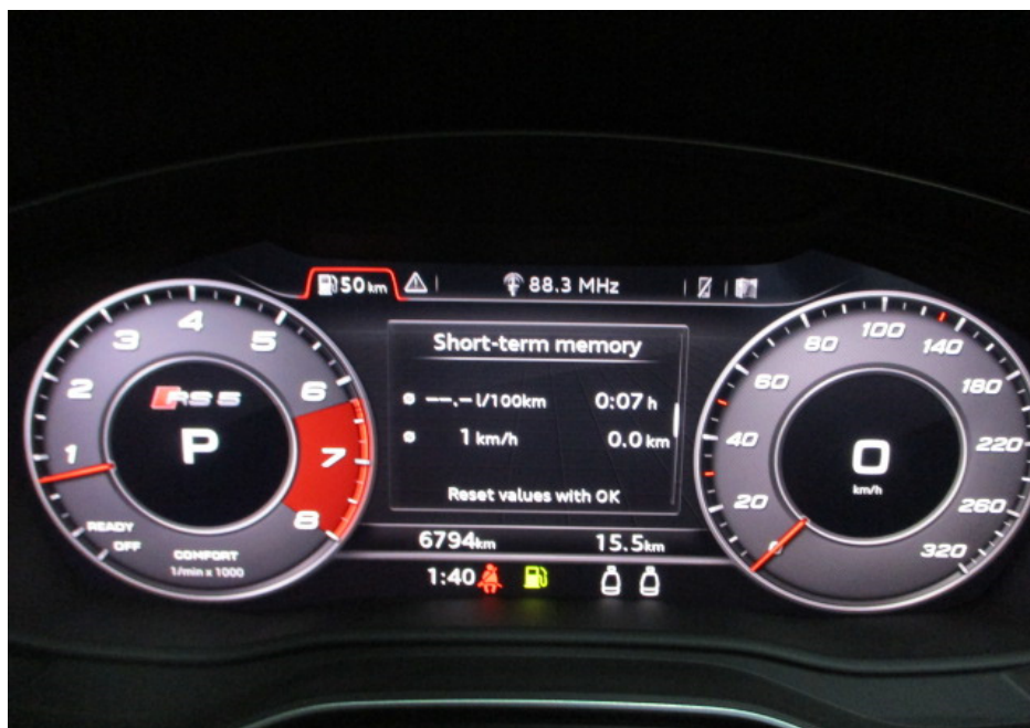
Photo 12 shows the respective warning lights no longer illuminated, indicating that there is no fault detected to the ABS, SRS, EPS, ESC and TPM systems of the Motor Car during the self-test. These electronic systems were hence in working condition at the time of my inspection.
