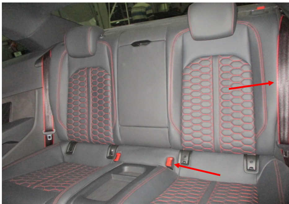
Photo 10 shows the rear seats of the Motor Car. All the seats of the Motor Car were fitted with a retractable seat belt reel and pre-tensioner (arrowed). The seat belts were tested and able to be fastened into the respective pre-tensions that were fitted on the side of each individual seat.
