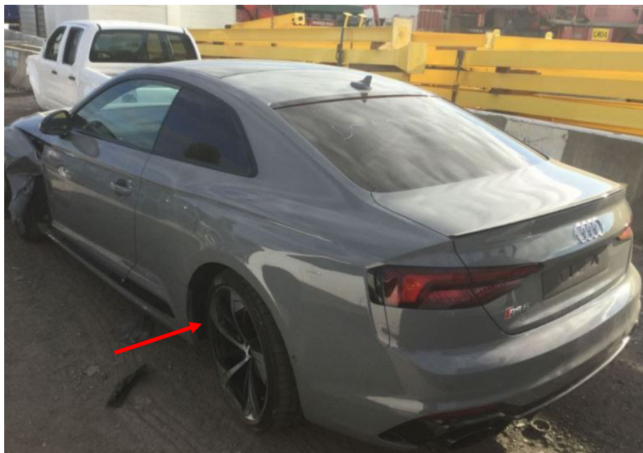
Photo 2 shows the rear left body of the Motor Car prior to any repairs being carried out (photograph provided to me). The rear left wheel rim was observed to be oriented towards the right (arrowed), which would indicate that the rear left undercarriage parts of the Motor Car were affected.
