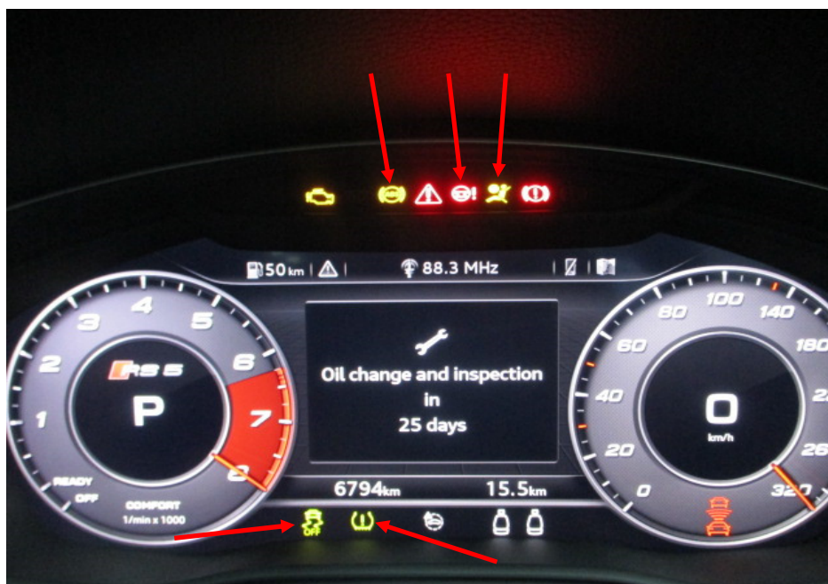
Photo 11 shows the warning lights for the various electronic safety features appearing on the instrument panel of the Motor Car during its self-test when the engine is cranked, in particular the ABS, SRS, EPS, ESC and TPM lights (arrowed).
