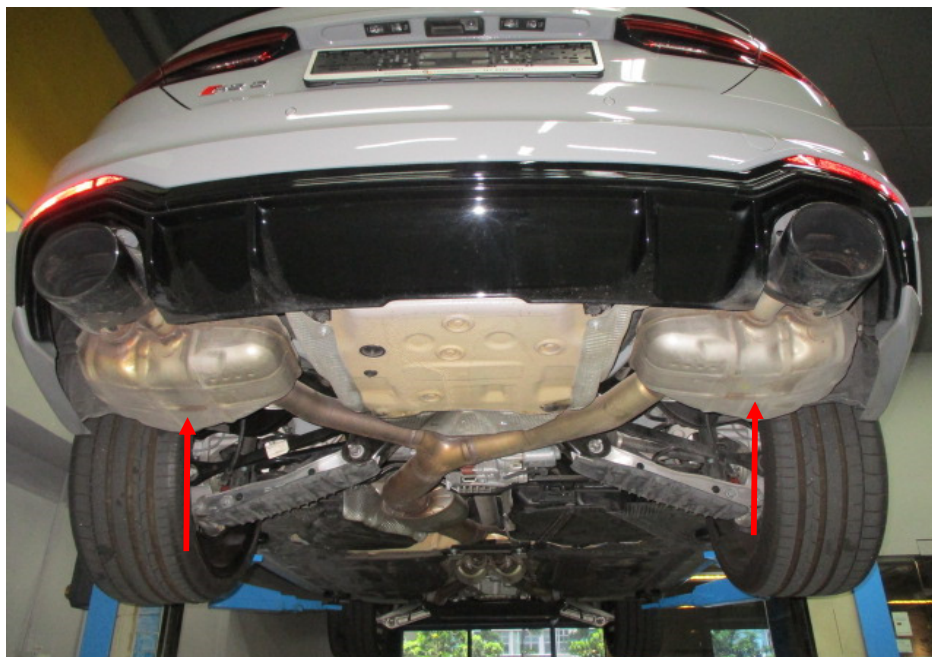
Photo 17 shows the Motor Car's rear mufflers (arrowed). My examination of the Motor Car's exhaust system revealed no sign(s) or indication(s) of any cut or weld marks along its exhaust pipes and on its catalytic converters.
