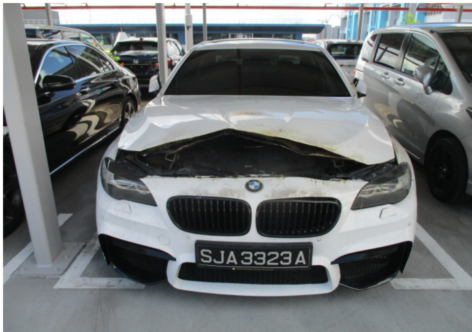
Photo 2 shows the general view of the front portion of the Insured Vehicle at the time of our inspection. The exterior body of the Insured Vehicle had sustained visible fire damage. This included its front windscreen, front bonnet, headlights, front bumper and side panels.
