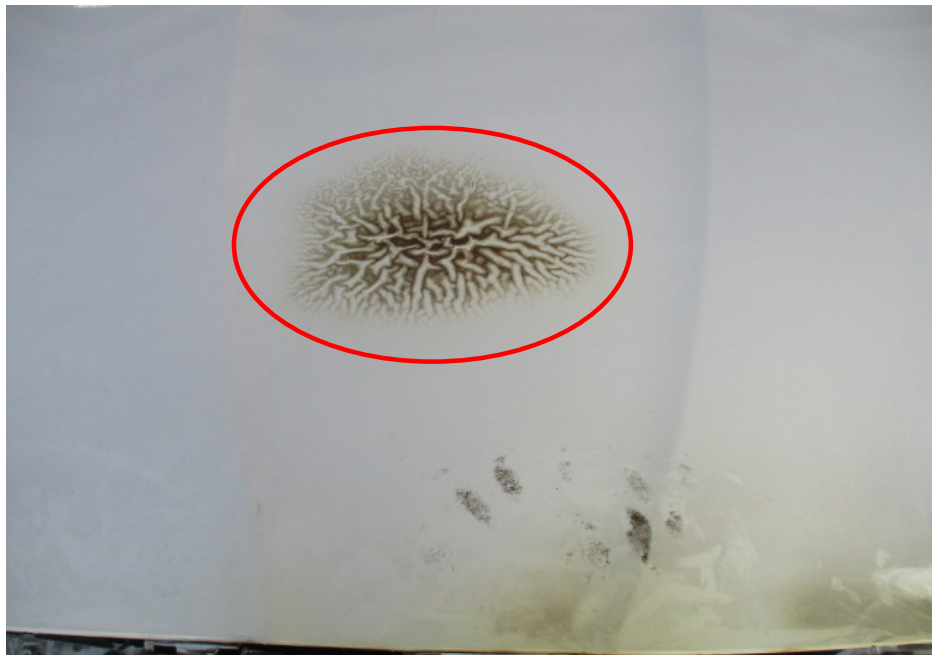
Photo 11 shows the burn marks and paint bubbles on the front centre portion of the front bonnet of the Insured Vehicle (circled).
