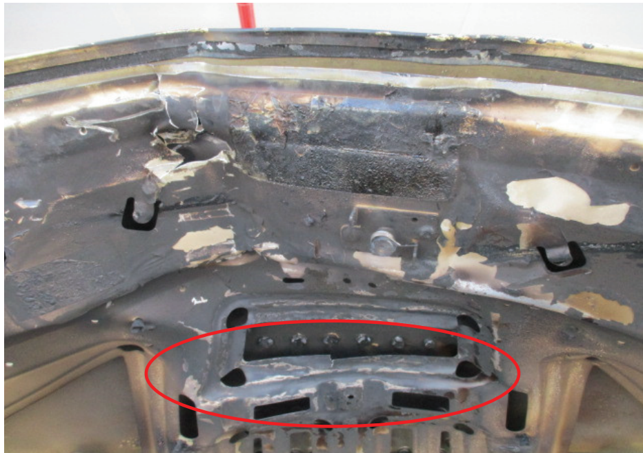
Photo 10 shows upon closer examination, we noticed whitish burn marks on the top centre portion on the underside of the bonnet of the Insured Vehicle due to prolonged exposure to high heat intensity caused by the fire (circled).
