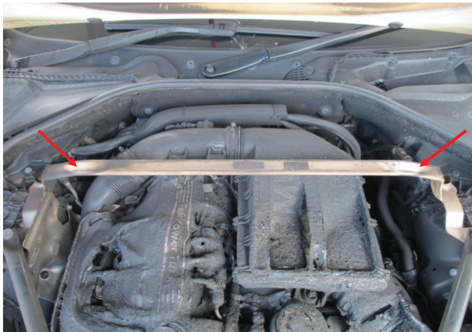
Photo 7 shows the engine strut bar (arrowed) fitted on the Insured Vehicle. However it had sustained minor fire damage.
