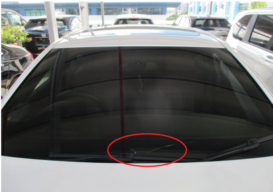
Photo 4 shows a closer view of the front windscreen of the Insured Vehicle at the time of our inspection. The front windscreen had sustained minimal fire damage (circled).
