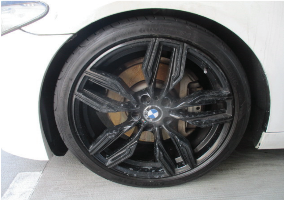
Photo 8 shows the non-standard rim found to be fitted on the Insured Vehicle at the time of our inspection. The 20- inch alloy rims fitted on the Insured Vehicle were not the standard type for the Insured Vehicle.
