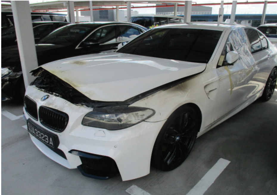
Photo 3 shows the general view of the left frontal portion of the Insured Vehicle at the time of our inspection. The exterior body of the Insured Vehicle had sustained visible fire damage. This included its front windscreen, front bonnet, left headlight, front bumper and left side panel.
