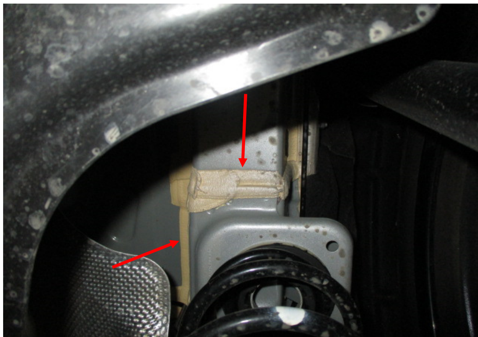
Photo 20 shows the chassis/structural body at the underside rear right of the Motor Car. Visually, The original factory sealant (arrowed) at the joints along the chassis/structural body was untouched, indicating no work was done on the chassis/structural body of the Motor Car and that the chassis/structural body was originally fitted.
