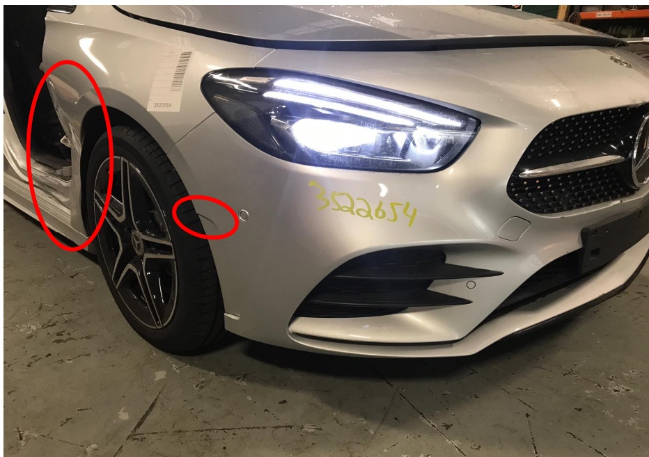
Photo 3 shows the front right body of the Motor Car prior to any repairs being carried out (photograph provided to me). The front bumper and front right fender (circled) were amongst the body parts that were observed to be damaged.
