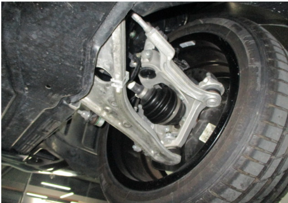
Photo 16 shows the various undercarriage components at the front right wheel of the Motor Car. The mechanical components, control arms and linkages were all found to be intact and secured in an appropriate manner.
