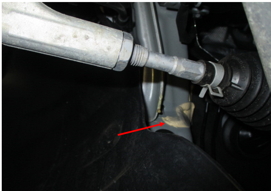
Photo 19 shows the chassis/structural body at the underside front right of the Motor Car. Visually, I did not find any weld marks other than original spot weld marks on the chassis/structural body of the Motor Car. The original factory sealant (arrowed) at the joints along the chassis/structural body was also untouched, indicating no work was done on the chassis/structural body of the Motor Car and that the chassis/structural body was originally fitted.
