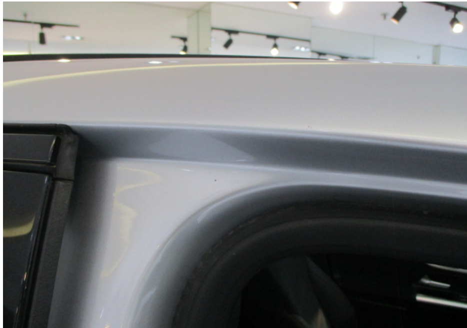
Photo 7 shows the right side "B" pillar of the Motor Car. The body parts along the right side of the Motor Car were visually examined and it was observed that the repair/restoration works carried out to the damaged area of the Motor Car (refer photograph 1 to 3 above) were reasonably adequate and in order.
