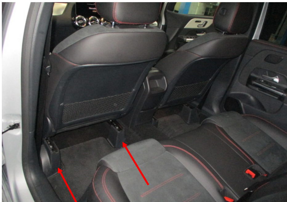
Photo 11 shows the seats of the Motor Car, which were secured via seat rails (arrowed) to the floor board. All the seats of the Motor Car were fitted with a retractable seat belt reel and pre-tensioner. The seat belts were tested and able to be fastened into the respective pre-tensions that were fitted on the side of each individual seat.
