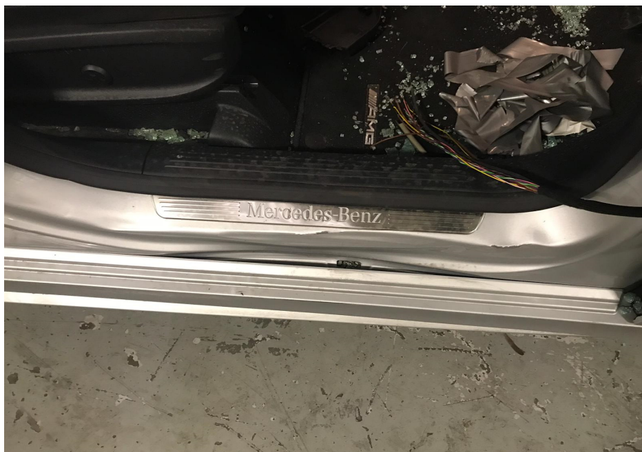
Photo 2 shows the right side rocker panel of the Motor Car prior to any repairs being carried out (photograph provided to me). The Motor Car was observed to have sustained damages along its right side. Amongst the body parts damaged was the right side rocker panel.
