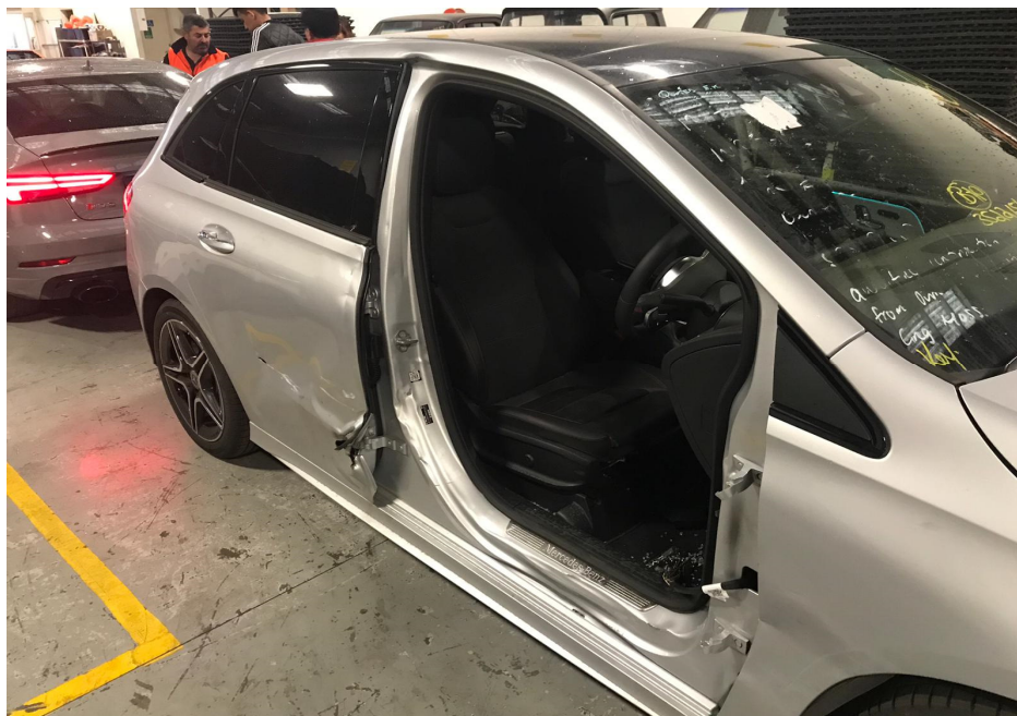
Photo 1 shows the right side of the Motor Car prior to any repairs being carried out (photograph provided to me). The Motor Car was observed to have sustained damages along its right side. The body parts observed to be damaged and/or dislodged had included its front right fender, front right door, rear right door, right side "B" pillar, right side rocker panel and front right door hinges amongst others.
