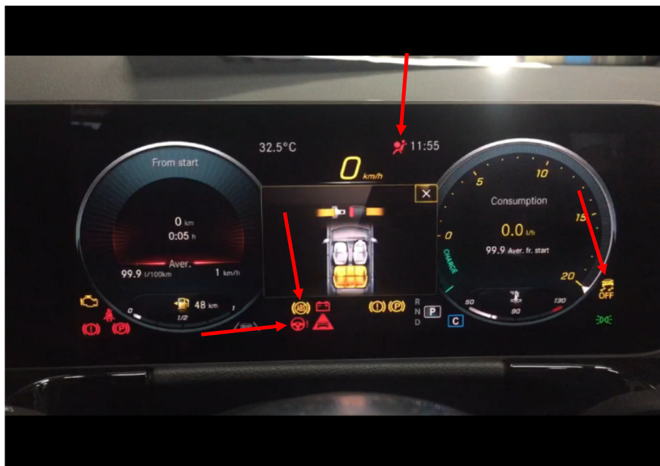
Photo 12 shows the warning lights for the various electronic safety features appearing on the instrument panel of the Motor Car during its self-test when the engine is cranked, in particular the ABS, SRS, EPS and ESP lights (arrowed).
