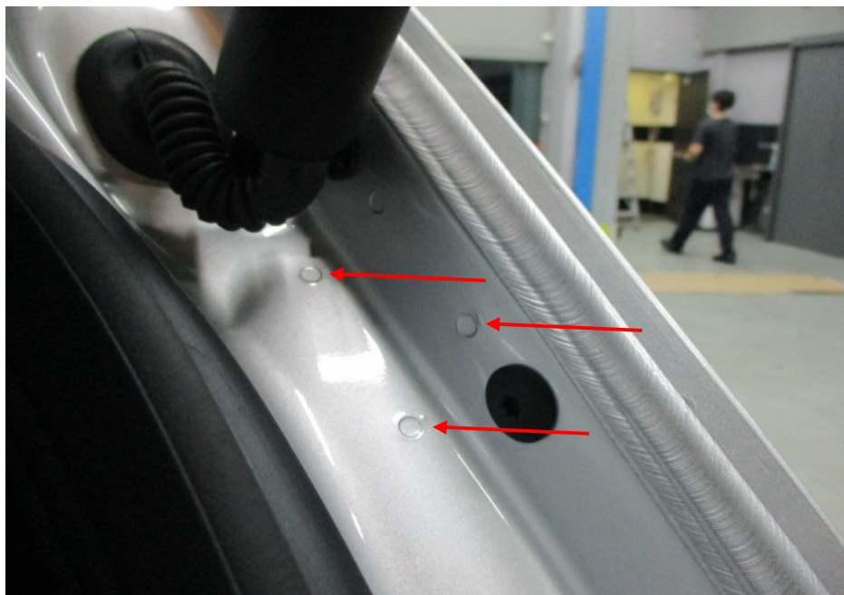
Photo 21 shows the right rear body panel of the Motor Car. I did not find any weld marks other than original spot weld marks (arrowed) on the non-detachable body panels of the Motor Car, indicating that there was no re-welding works carried out; and that the non-detachable body panels of the Motor Car were originally fitted.
