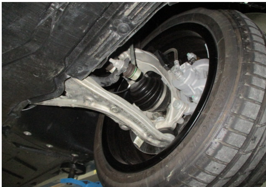
Photo 17 shows the various undercarriage components at the front left wheel of the Motor Car. The mechanical components, control arms and linkages were all found to be intact and secured in an appropriate manner. I also did not observe any fluid leak and/or fluid stain on the underside of the Motor Car.
