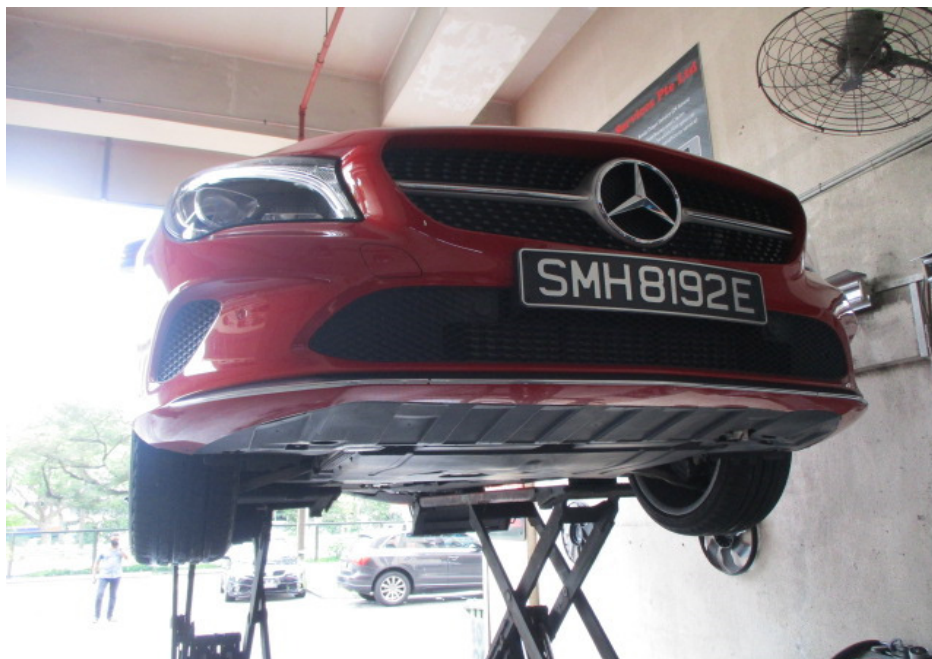
Photo 7 shows the Motor Car hoisted up for checks on its undercarriage. There was no sign(s) or indication(s) of fluid leakage and/or fluid stain(s) on the underside of the Motor Car. The undercarriage components of the Motor Car were also all observed to be intact and secured in an appropriate manner.
