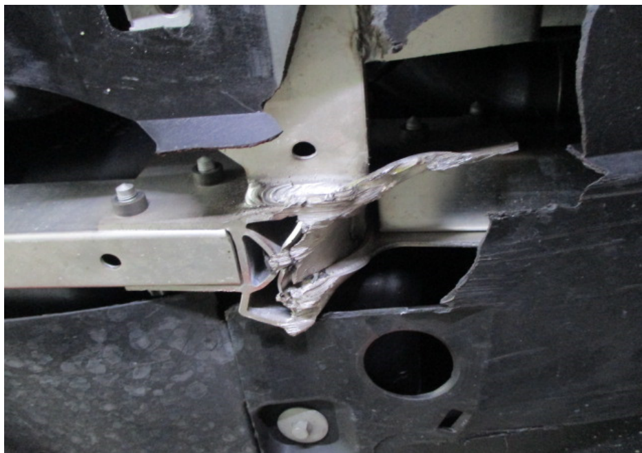
Photo 14 shows another view of the aluminium crossmember that was found to be dented/damaged.
