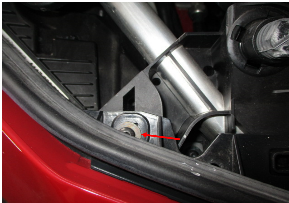
Photo 18 shows one of the Motor Car's front bumper attaching screws. Upon my close examination, this attaching screw at the right side of the front bumper appears to have been removed and re-fitted as the positioning of the washer (arrowed) was not align to its original position as seen from the circular imprint mark that was formed when the washer was at its original position.
