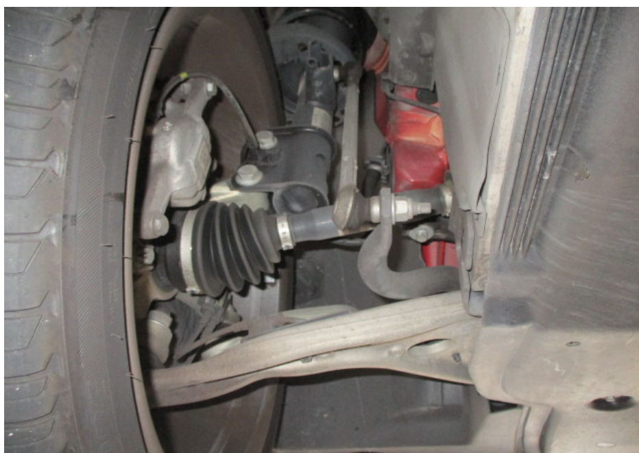
Photo 9 shows the various undercarriage components at the front right wheel of the Motor Car. The mechanical components, control arms and linkages were all found to be intact and secured in an appropriate manner.
