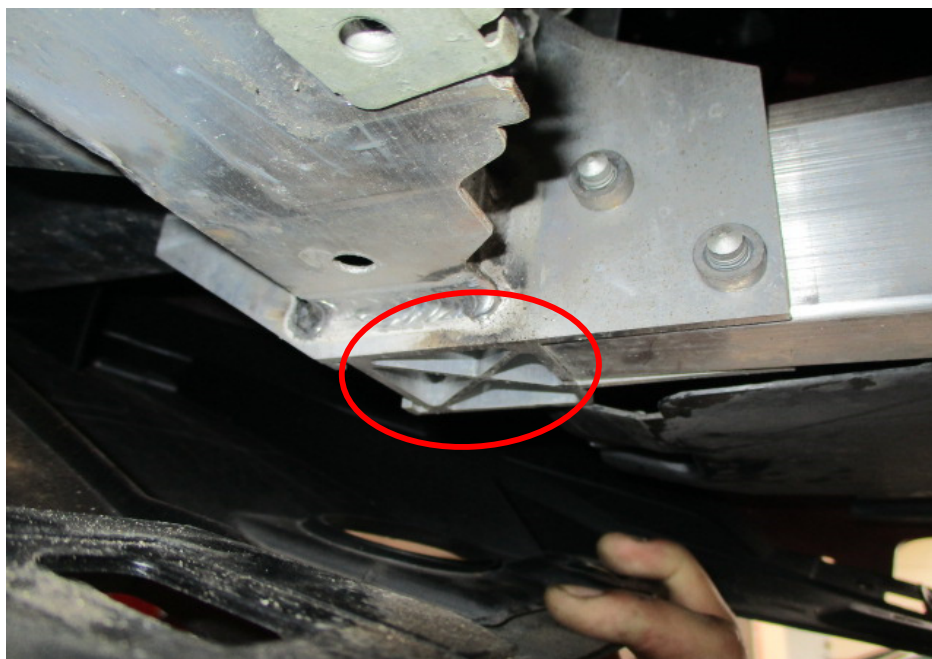
Photo 15 shows the same area (circled) at the right side of the aluminium crossmember, which was undamaged, for comparison with the dented/damaged area at the left side (refer to photograph 14 above).
