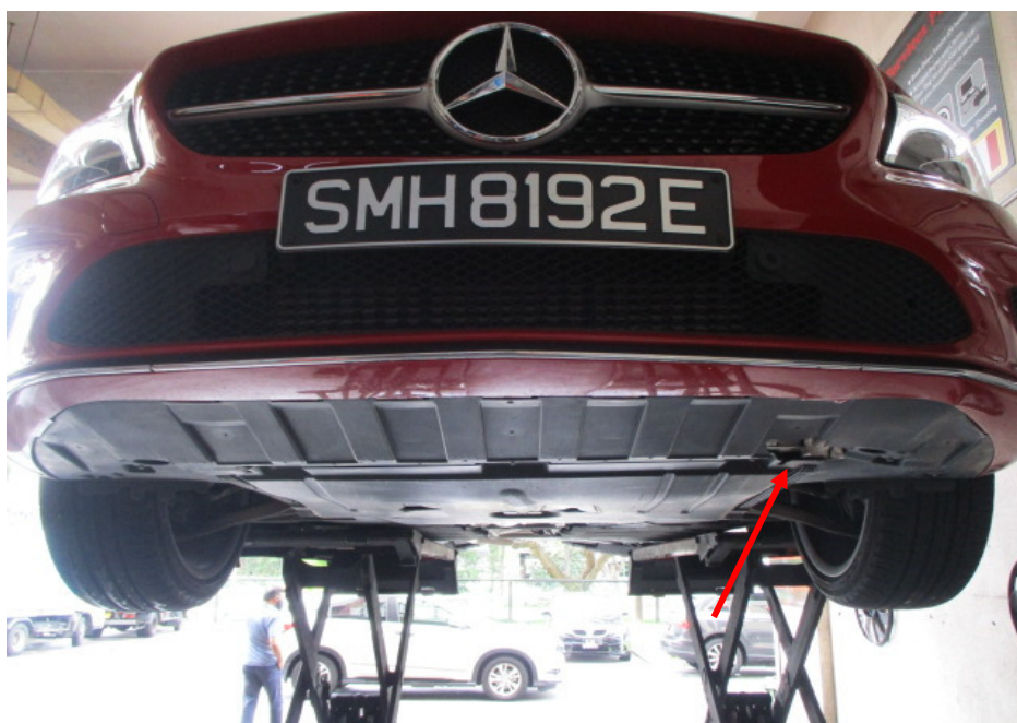
Photo 11 shows the front underside of the Motor Car. During my examination of the Motor Car's underside, I had observed that the engine undercover was broken at the left side (arrowed).
