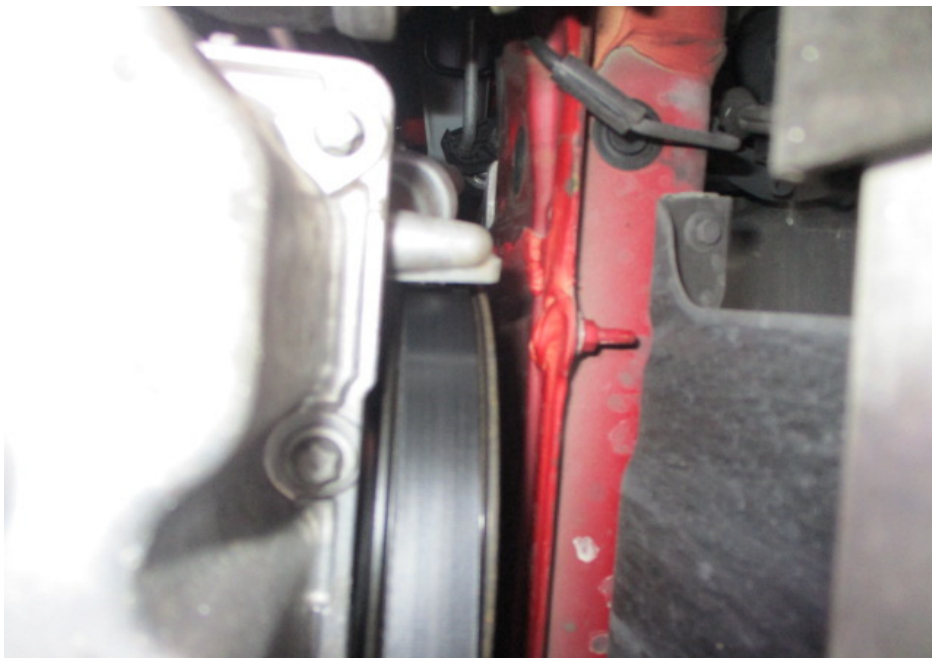
Photo 17 shows the front section of the front right chassis member of the Motor Car. The paint of the front section does not appear to be as bright when compared to the same area of the front left chassis member (refer to photograph 16 above). This would suggest that the front section of the front left chassis member of the Motor Car was recently repainted.
