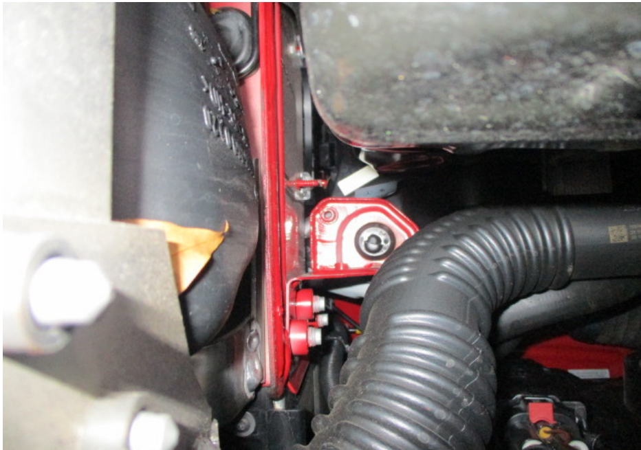
Photo 16 shows the front section of the front left chassis member of the Motor Car. The paint of the front section appears to be fresh as compared to the same area of the front right chassis member (refer to photograph 17 below).
