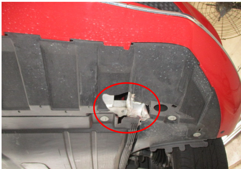
Photo 12 shows a closer view of the broken (circled) engine undercover. Upon closer examination, the Motor Car's aluminium crossmember was found to be dented/damaged at the area where the engine undercover was torn.
