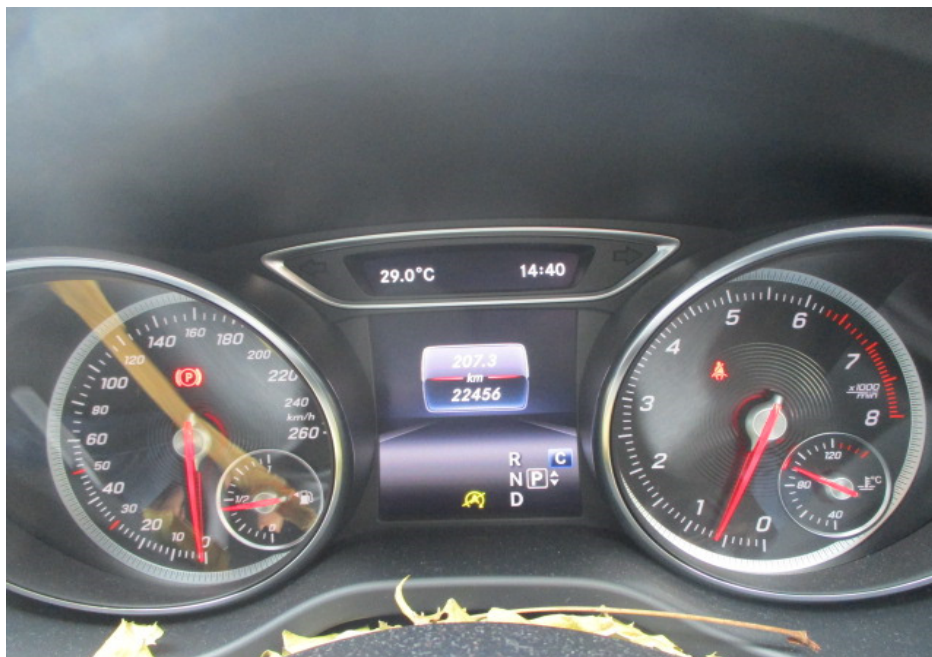
Photo 6 shows the respective warning lights no longer illuminated, indicating that there is no fault detected to the ABS, SRS, TPM and TCS systems of the Motor Car during the self-test. These electronic systems were hence in working condition at the time of my inspection.
