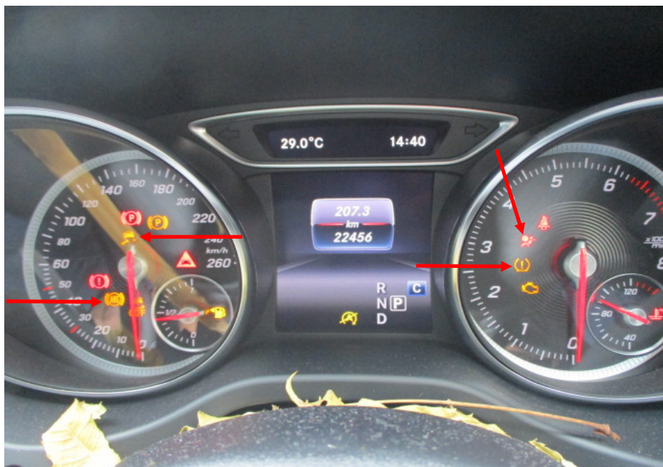
Photo 5 shows the warning lights for the various electronic safety features appearing on the instrument panel of the Motor Car during its self-test when the engine is cranked, in particular the ABS, SRS, TPM and TCS lights (arrowed).
