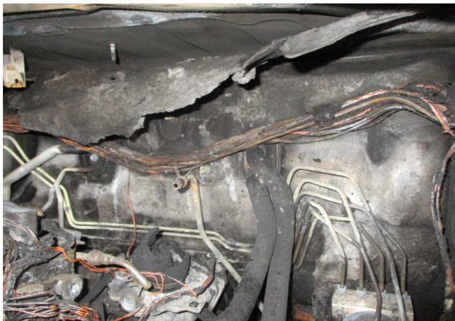
Photo 13 shows other stretches of original wire harnesses, around the rear left area of the Insured Vehicle's engine compartment, that were found burnt to its bare copper state. Such condition normally indicates internal heating of copper wires, which is a sign of an electrical short circuit. The condition of the wirings seen at the area where the fire had originated supports the cause of fire to the Insured Vehicle being due to electrical in nature.
