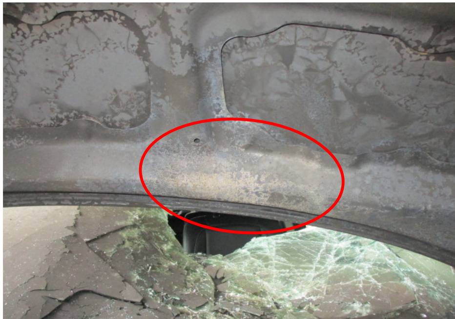
Photo 9 shows the underside of the Insured Vehicle's front bonnet. Similar high heat intensity burn marks (circled) were found on the underside rear left area of the Insured Vehicle's front bonnet. This was directly below the area where similar nature of high heat intensity burn marks were formed on the top side of the Insured Vehicle's front bonnet.
