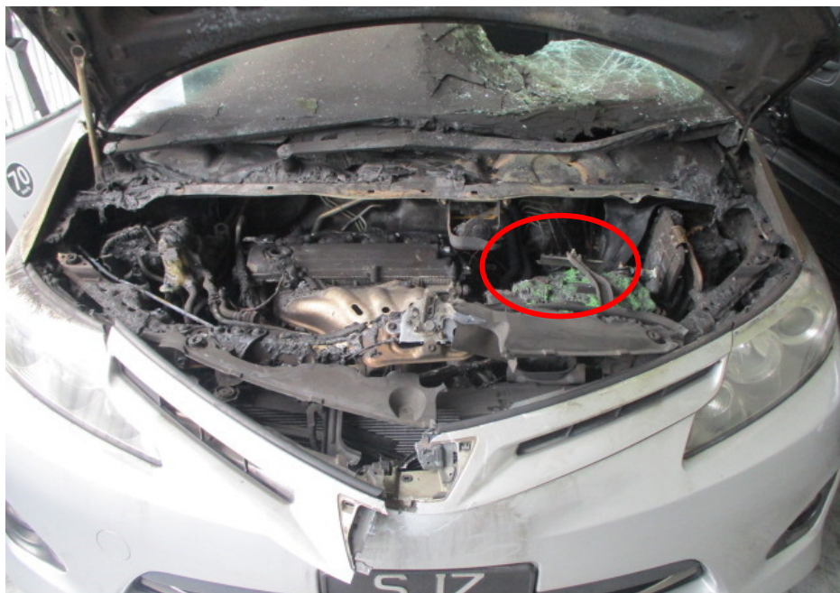
Photo 10 shows the engine compartment of the Insured Vehicle. Following the burn pattern, in particular the location where the high heat intensity burn marks were found on the front bonnet, and the characteristic of heat rising upwards, the fire to the Insured Vehicle can be determined to have originated around the rear left side (circled) of the engine compartment.
