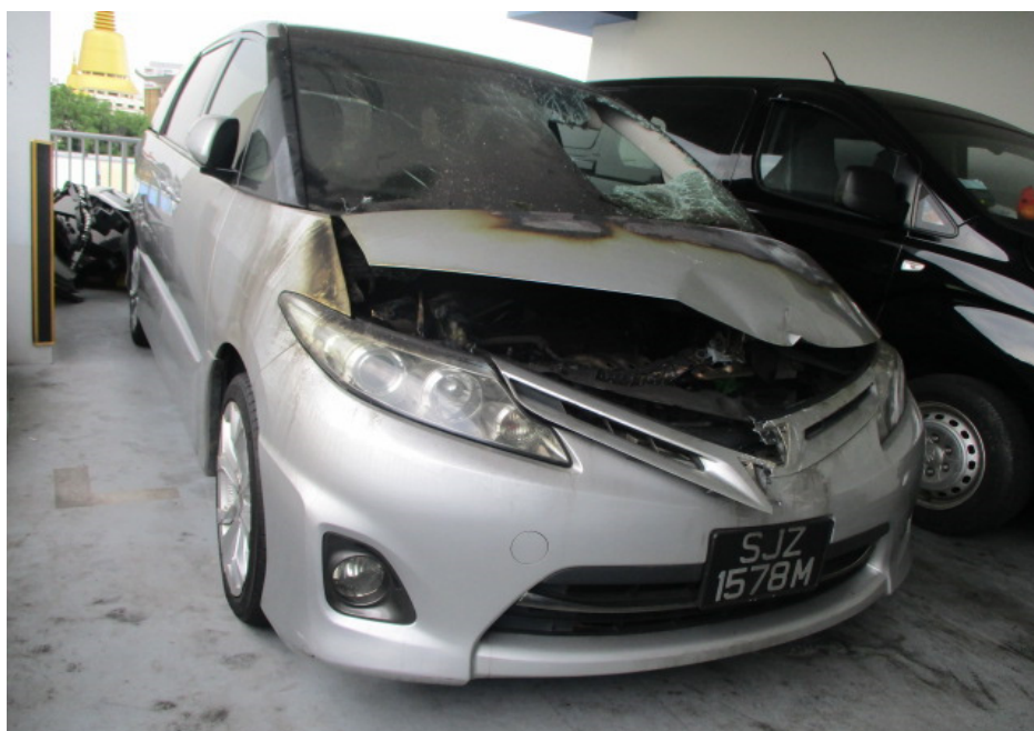
Photo 1 shows a general view of the front right body of the Insured Vehicle at the time of my inspection. The fire damage to the Insured Vehicle was confined to its frontal portion. Its front bumper, front bonnet, front right headlamp and front right fender were amongst the exterior body parts that were found to have been affected as a result of the fire.
