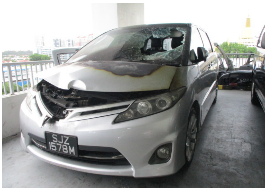
Photo 2 shows a general view of the front left body of the Insured Vehicle at the time of my inspection. The front left fender, front bonnet, front grille, front left headlamp and front windscreen were amongst the exterior body parts that were found to have been affected as a result of the fire.
