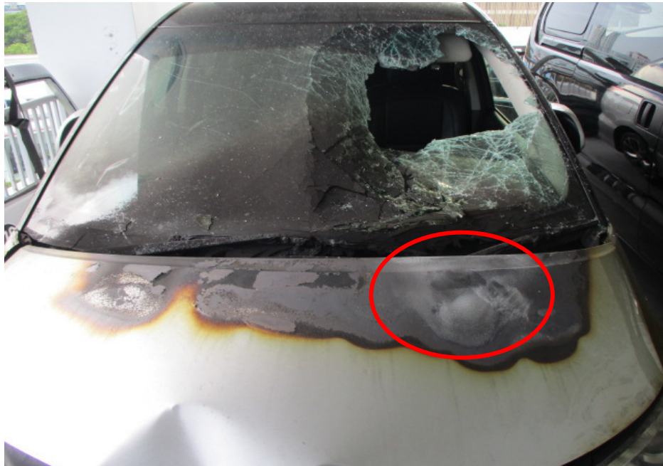
Photo 8 shows the high heat intensity burn marks (circled) that were found on the rear left area of the Insured Vehicle's front bonnet, within an area of the front bonnet that was found with paint blackened. Such whitish burn marks are a result of exposure to prolong heat intensity. Following the characteristic of heat rising upwards, the fire to the Insured Vehicle can then be determined to have originated around the rear left area of the engine compartment.
