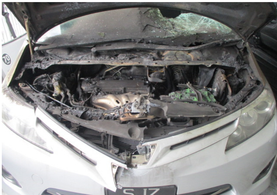
Photo 3 shows the engine compartment of the Insured Vehicle at the time of my inspection. Almost all the parts inside the engine compartment were observed to have been burnt and/or melted. The parts include the air intake manifold, engine top cover, battery, fuse box, various hoses and pipes amongst others.
