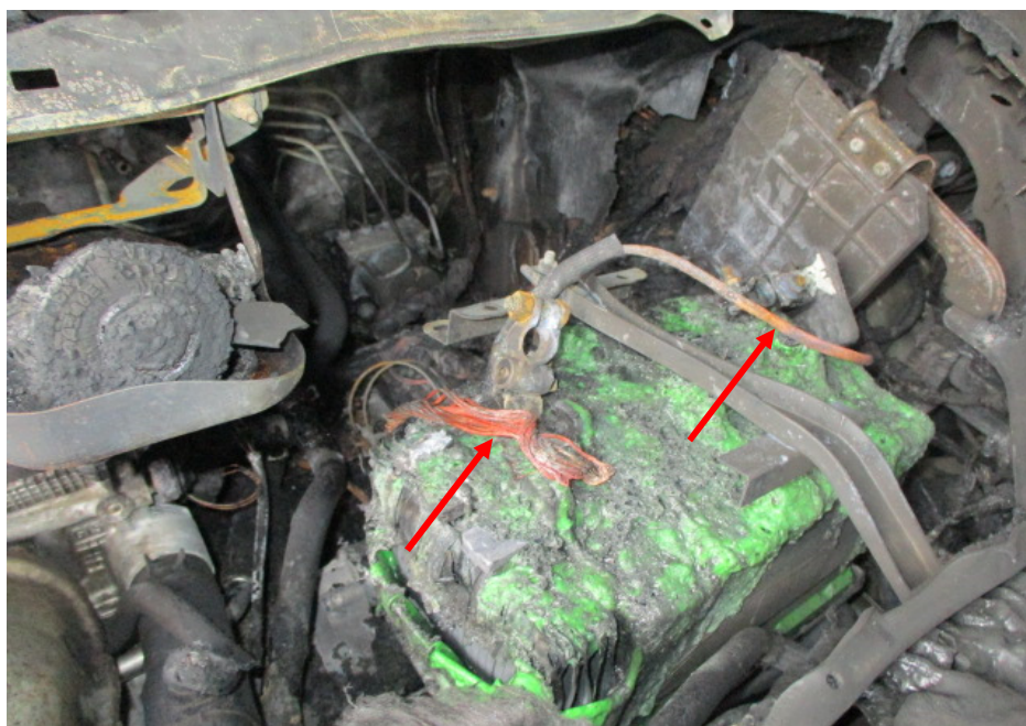
Photo 11 shows the wirings around the area where the fire to the Insured Vehicle had originated. Several stretches of original wire harnesses around this area were found to be burnt to its bare copper state. The battery wire cable (arrowed) for the positive terminal was observed to be in bright reddish colour, indicating internal heating of copper wires, which is a sign of an electrical short circuit.
