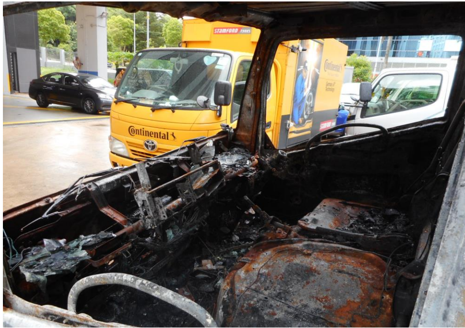
Photo 3 shows the general view of the interior compartment of the Insured Vehicle. The entire windscreen and the interior compartment have been badly burnt by the fire.
