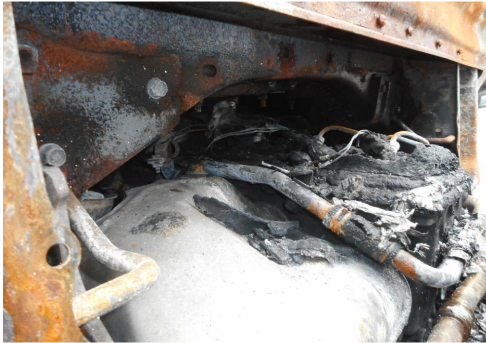
Photo 9 shows the engine compartment of the Insured Vehicle at the time of our inspection. The front cabin of the Insured Vehicle was not able to be lifted due to the damage it sustained from the fire, the engine unit was observed to be damaged by the fire.
