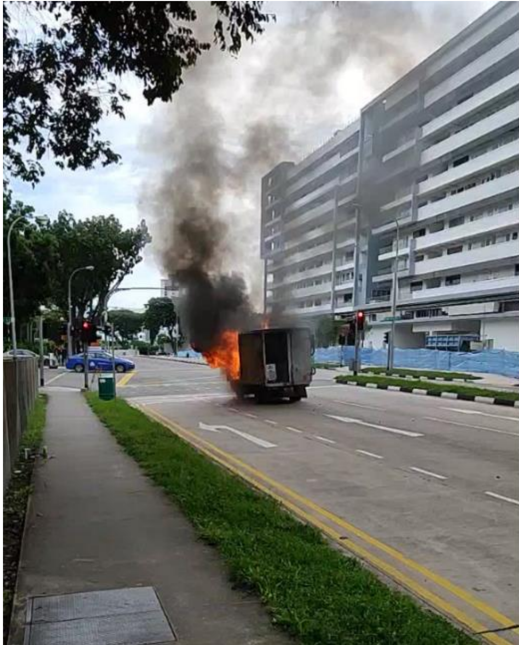
Photo 17 shows rear view of the Insured Vehicle on fire, as the fire has started from the front cabin and spread towards the rear cabin. In general, the information that could be gathered from this photograph had corresponded to the events that were related to us by Mr Amli, where the fire had started on the Insured Vehicle.
