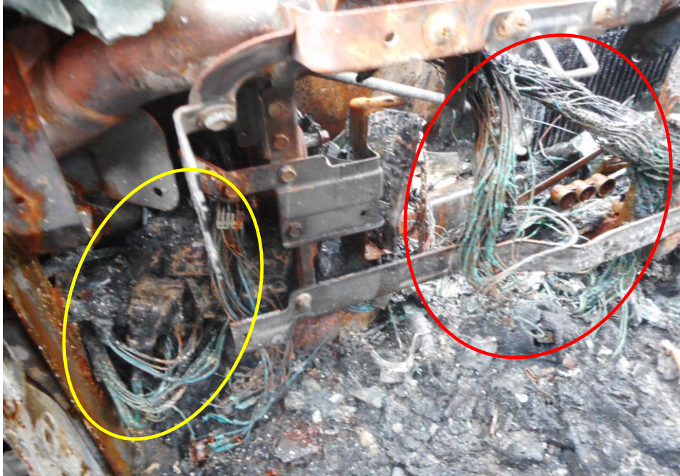
Photo 13 shows a close up view of the original wiring harness leading to the fuse box in the front cabin compartment. The original wiring harness (red circle) and fuse box wirings (yellow circle) was observed with greenish residue on the surface. The presence of greenish residue indicates internal heating of copper wires, a sign of an electrical short circuit occurring. The greenish residue is normally left behind from oxidation as a result of chemical reaction involving the copper wires.
