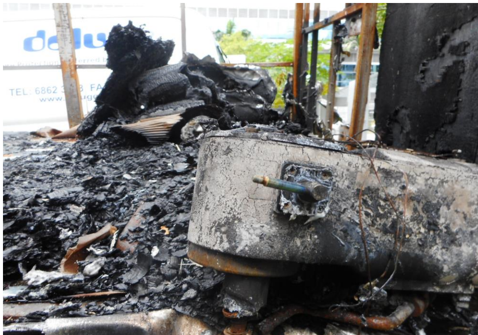
Photo 10 shows a closer view of the rear portion of the Insured Vehicle at the time of our inspection. The entire rear cabin compartment and the goods inside had sustained severe visible fire damage.
