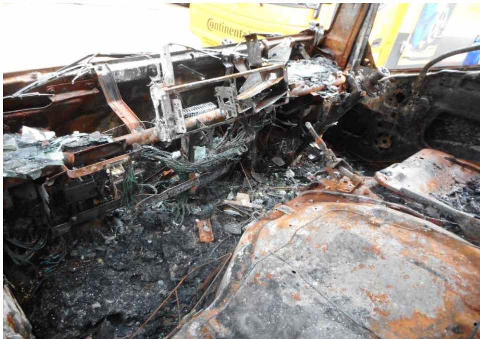
Photo 4 shows the close up view of the interior compartment of the Insured Vehicle. The interior compartment have been badly burnt by the fire.
