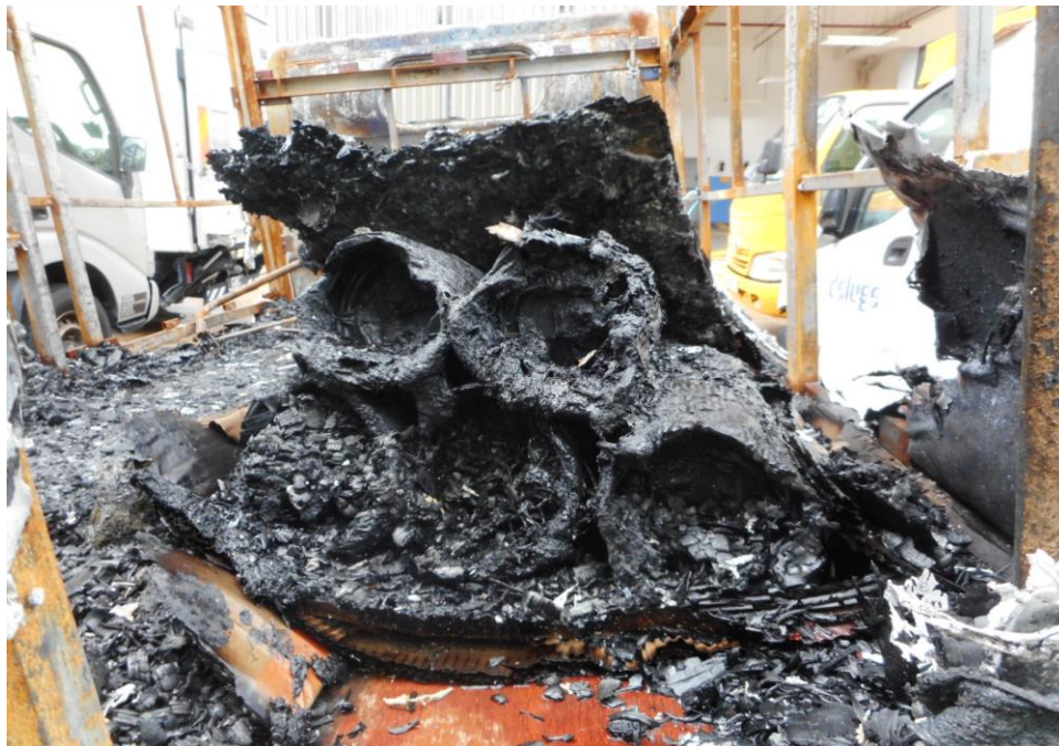
Photo 11 shows a closer view of the rear cabin compartment of the Insured Vehicle at the time of our inspection. The rear cabin was significantly burnt and/or melted as a result of the fire. We also found remnants of cardboard and various other items in the rear cabin compartment.
