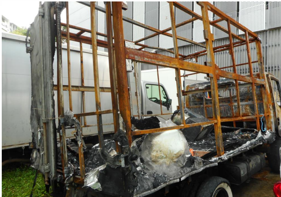
Photo 5 shows the rear cabin of the Insured Vehicle from the right side at the time of our inspection. The fire damage to the Insured Vehicle had burnt down the entire rear portion compartment. The whole rear cabin panel were amongst the parts that were observed to have been affected by the fire.
