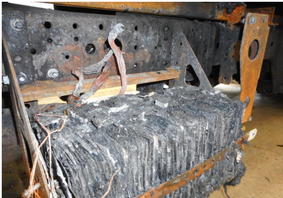
Photo 8 shows the battery unit of the Insured Vehicle at the time of our inspection. The battery unit and the battery terminal was damaged by the fire of the Insured Vehicle.
