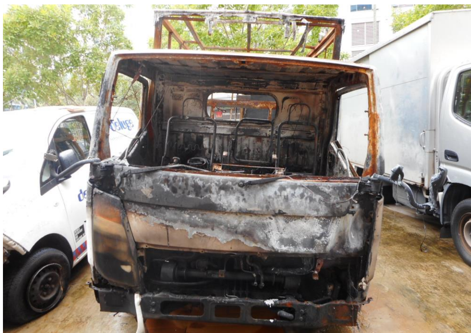
Photo 2 shows the front view of the Insured Vehicle at the time of our inspection. The fire damage to the Insured Vehicle had affected the whole Insured Vehicle.
