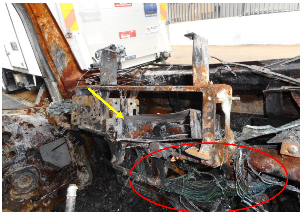
Photo 12 shows the general view of the interior compartment of the Insured Vehicle at the time of our inspection. The fire damage to the Insured Vehicle has affected its engine and interior compartment. Its interior dashboard (circled), radio head unit (yellow arrow), various original wiring harnesses was amongst the parts in the compartment that were found to have been affected as a result of the fire.
