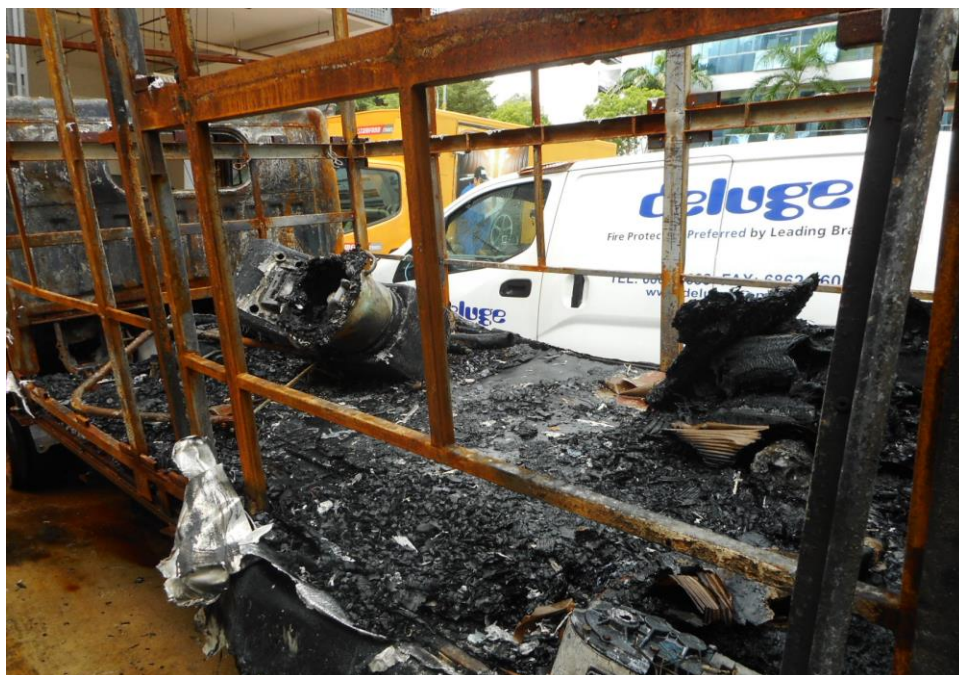
Photo 6 shows the rear cabin of the Insured Vehicle from the left side at the time of our inspection. The fire damage to the Insured Vehicle had burnt down the entire rear portion compartment. The goods in the rear cabin that the Insured Vehicle was carrying were amongst the parts that were observed to have been burnt by the fire.
