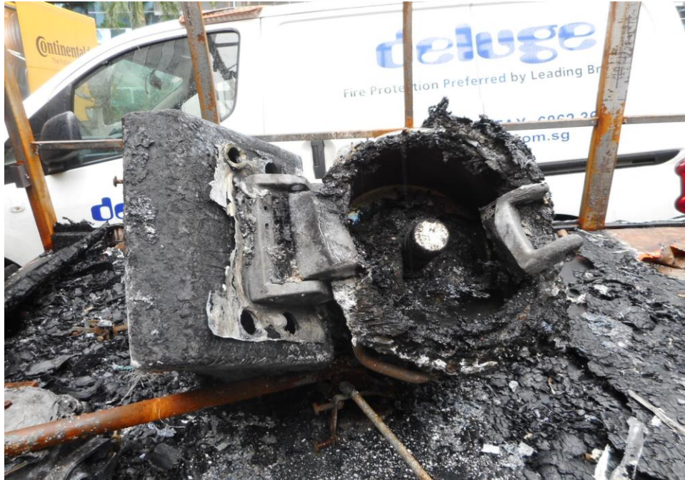
Photo 7 shows the close up view of the goods in the rear cabin of the Insured Vehicle at the time of our inspection. The fire damage to the Insured Vehicle had burnt down the entire rear portion compartment. The goods in the rear cabin that the Insured Vehicle was carrying were amongst the parts that were observed to have been burnt by the fire.
