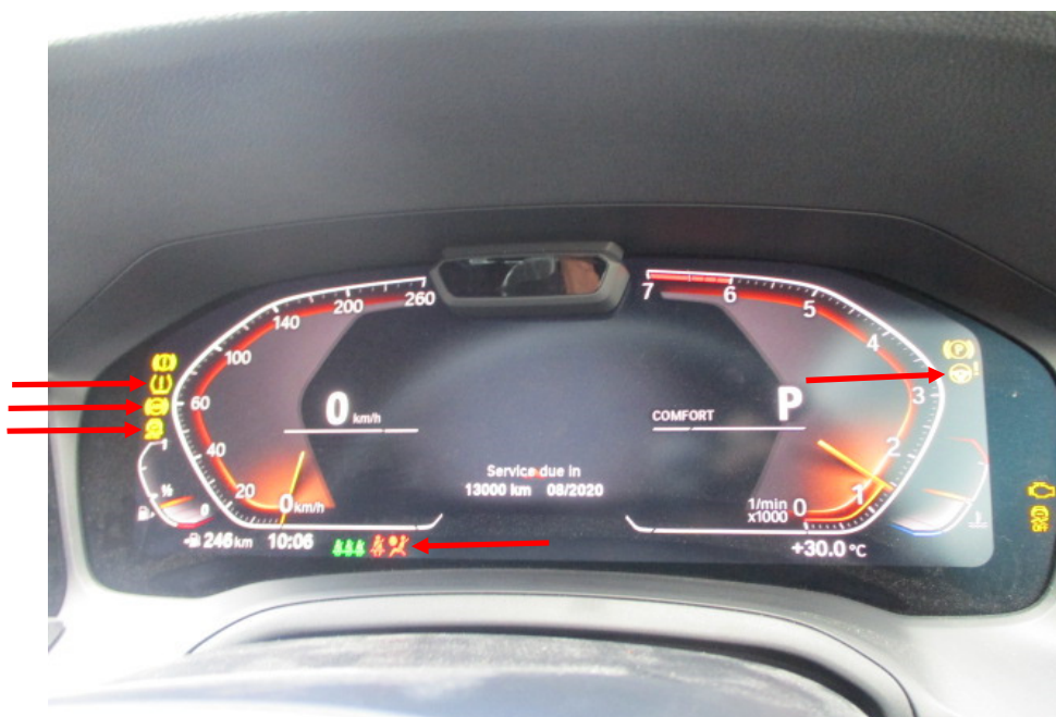
Photo 10 shows the warning lights for the various electronic safety features appearing on the instrument panel of the Motor Car during its self-test when the engine is cranked, in particular the ABS, SRS, IAS, TPM and DSC lights (arrowed).
