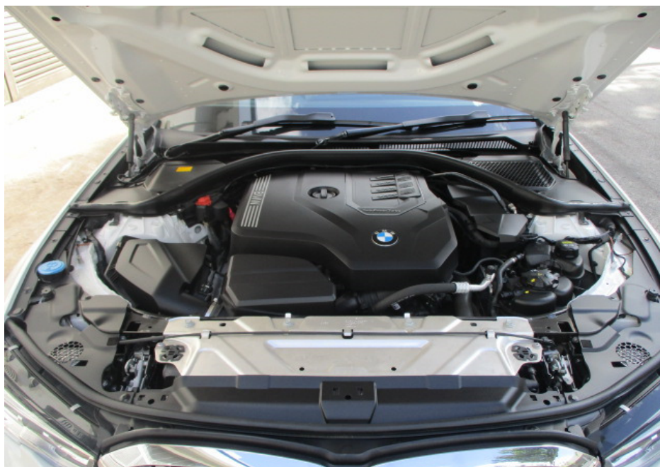
Photo 8 shows a general view of the engine compartment of the Motor Car at the time of my inspection. The various parts and components inside the engine compartment were all observed to be intact and properly fitted. There was also no sign(s) or indication(s) of fluid leak and/or fluid stain found inside the engine compartment.
