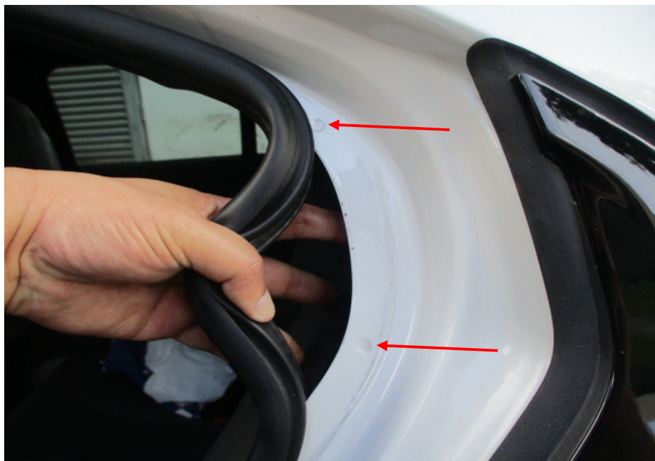
Photo 21 shows the left "C" pillar of the Motor Car. I did not find any weld marks other than original spot weld marks (arrowed) on the non-detachable body panels of the Motor Car, indicating that there was no re-welding works carried out; and that the non-detachable body panels of the Motor Car were originally fitted.
