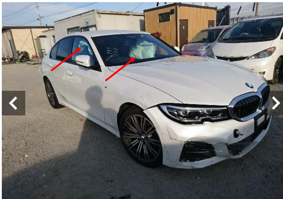
Photo 1 shows the front right body of the Motor Car prior to any repairs being carried out (photograph provided to me). The Motor Car was observed to have sustained damages at its front portion. The body parts observed to be damaged had include its front bumper, front right headlamp and front right fender amongst others. The right side and left side curtain airbags (arrowed) were also observed to have been deployed.
