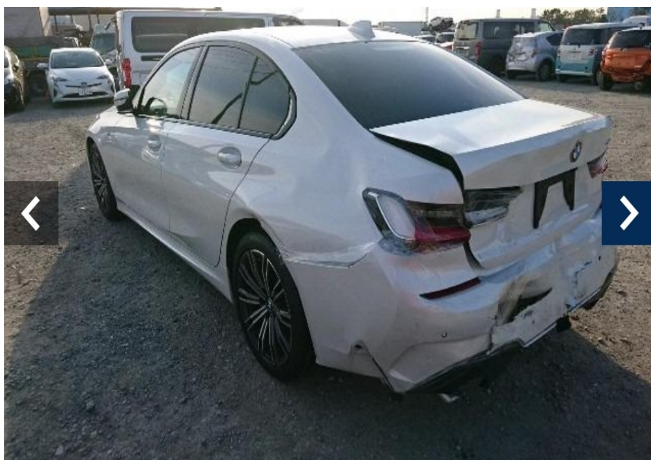
Photo 2 shows the rear left body of the Motor Car prior to any repairs being carried out (photograph provided to me). Apart for the front portion, the Motor Car had also sustained damages at its rear portion. Body parts damaged had include its rear bumper, rear left taillamp, rear left fender and rear bootlid amongst others.
