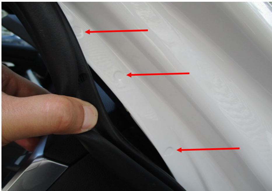
Photo 20 shows the right "A" pillar of the Motor Car. I did not find any weld marks other than original spot weld marks (arrowed) on the non-detachable body panels of the Motor Car, indicating that there was no re-welding works carried out; and that the non-detachable body panels of the Motor Car were originally fitted.
