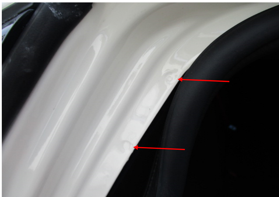
Photo 20 shows the right "C" pillar of the Motor Car. I did not find any weld marks other than original spot weld marks (arrowed) on the non-detachable body panels of the Motor Car, indicating that there was no re-welding works carried out; and that the non-detachable body panels of the Motor Car were originally fitted.
