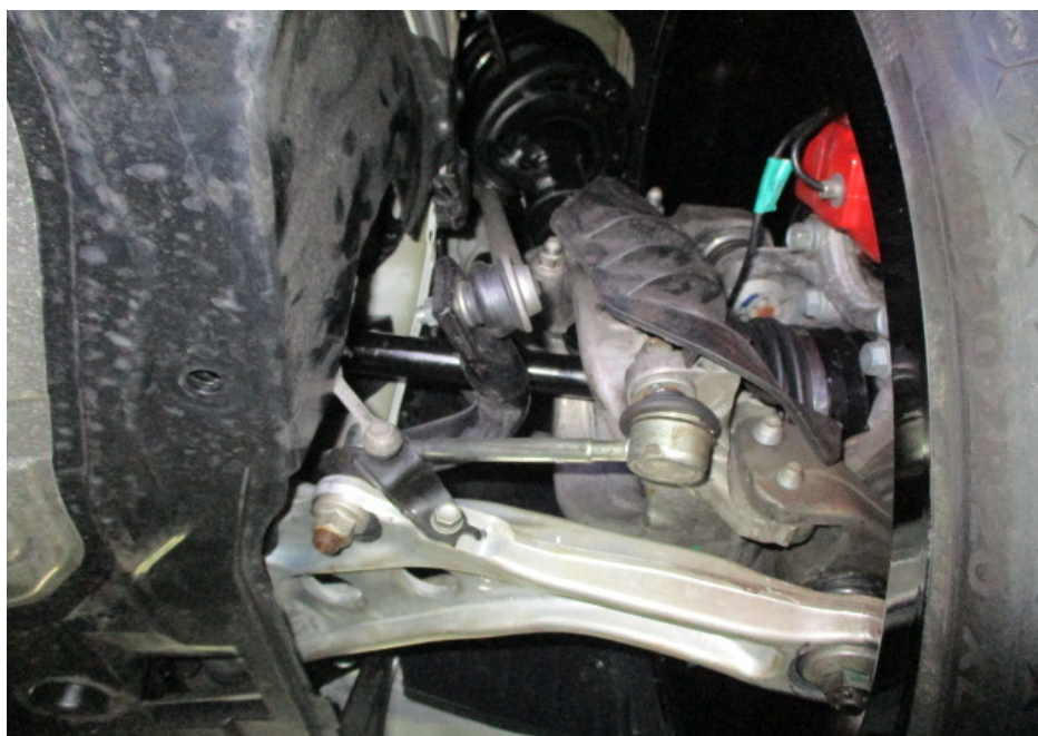
Photo 16 shows the various undercarriage components at the front left wheel of the Motor Car. The mechanical components, control arms and linkages were all found to be intact and secured in an appropriate manner. I also did not observe any fluid leak and/or fluid stain on the underside of the Motor Car.
