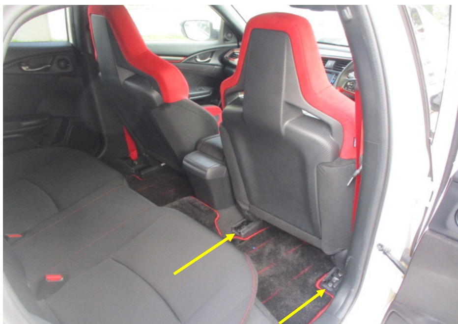
Photo 10 shows the seats of the Motor Car, which were secured via seat rails (arrowed) to the floor board. All the seats of the Motor Car were fitted with a retractable seat belt reel and pre-tensioner. The seat belts were tested and able to be fastened into the respective pre-tensions that were fitted on the side of each individual seat.
