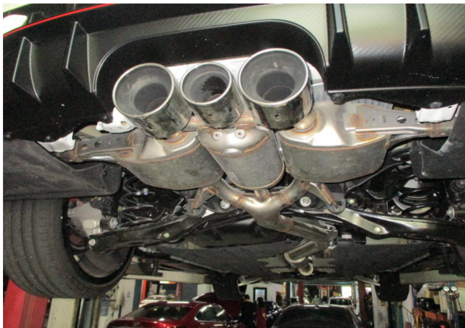
Photo 17 shows the Motor Car's rear exhaust mufflers. My examination of the Motor Car's exhaust system revealed no sign(s) or indication(s) of any cut or weld marks along its exhaust pipes and on its catalytic converter.
