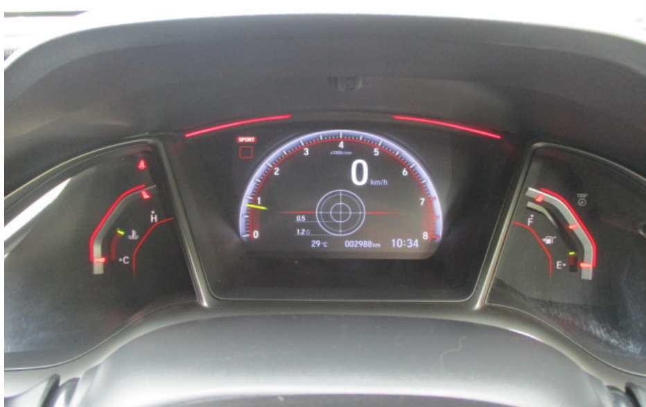
Photo 12 shows the respective warning lights no longer illuminated after the engine was started, indicating that there was no fault detected to the ABS, SRS, VSA and EPS systems of the Motor Car during the self-test. These electronic systems were hence in working condition at the time of my inspection.
