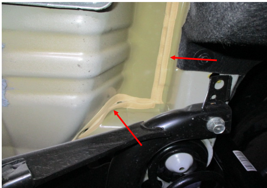
Photo 19 shows the chassis/structural body at the underside rear right of the Motor Car. The original factory sealant (arrowed) at the joints along the chassis/structural body was untouched, indicating no work was done on the chassis/structural body of the Motor Car and that the chassis/structural body was originally fitted.
