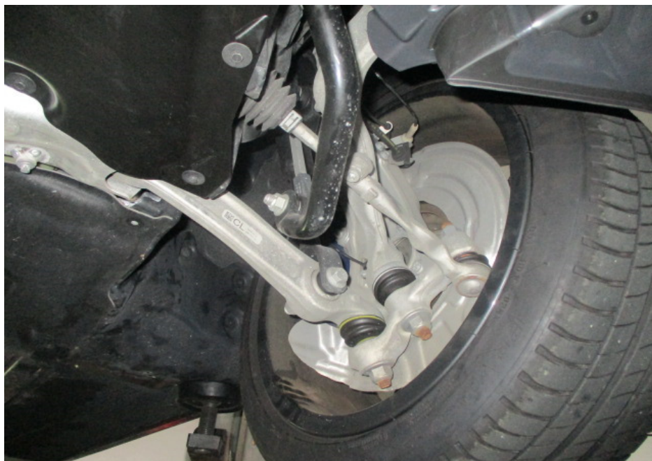
Photo 14 shows the various undercarriage components at the front left wheel of the Motor Car. The mechanical components, control arms and linkages were all found to be intact and secured in an appropriate manner.
