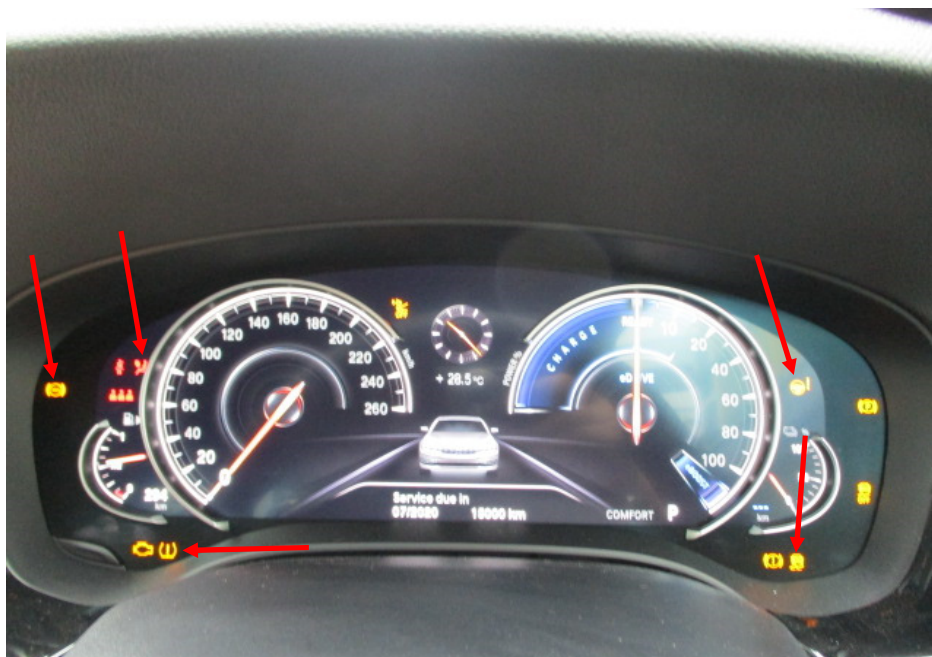
Photo 10 shows the warning lights for the various electronic safety features appearing on the instrument panel of the Motor Car during its self-test when the engine is cranked, in particular the ABS, SRS, IAS, TPM and DSC lights (arrowed).
