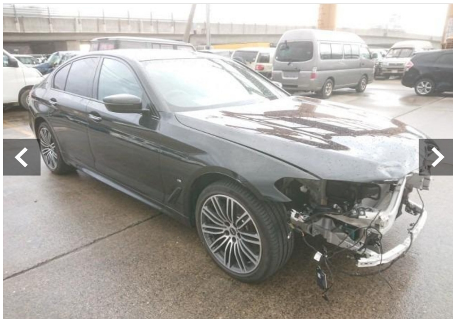
Photo 2 shows the front right body of the Motor Car prior to any repairs being carried out (photograph provided to me). The Motor Car was observed to have sustained damages at its frontal portion. The body parts observed to be damaged and/or dislodged had included its front bumper, front right headlamp and front bonnet amongst others.
