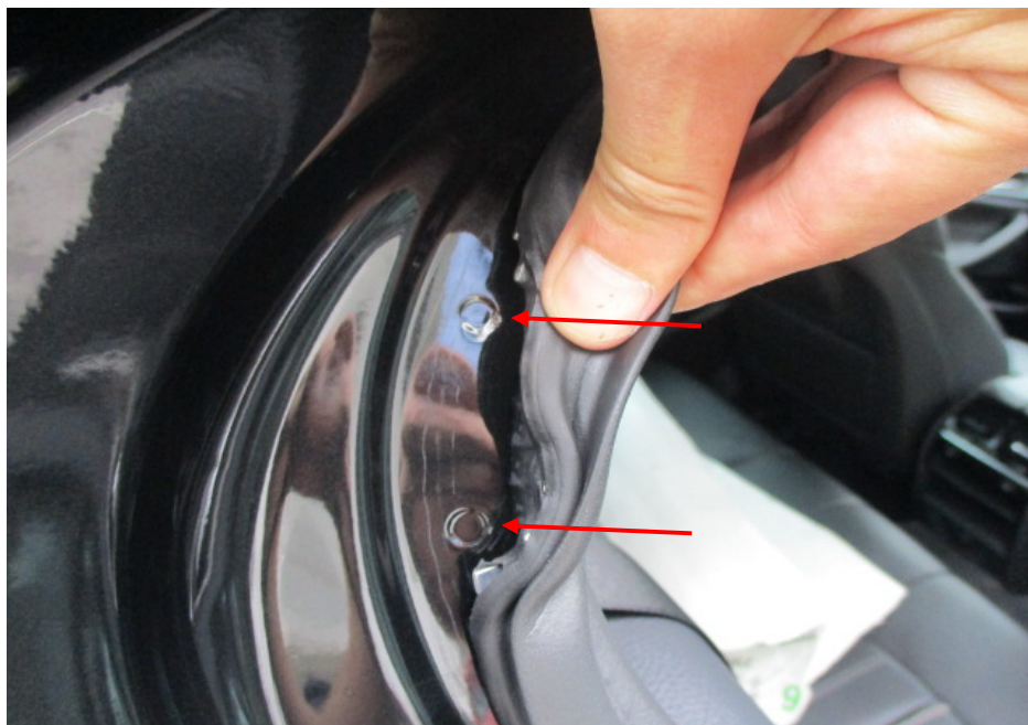
Photo 21 shows the right "C" pillar of the Motor Car. I did not find any weld marks other than original spot weld marks (arrowed) on the non-detachable body panels of the Motor Car, indicating that there was no re-welding works carried out; and that the non-detachable body panels of the Motor Car were originally fitted.
