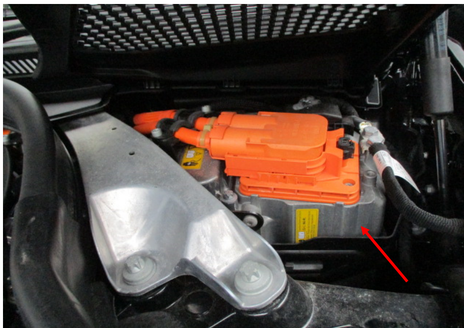
Photo 18 shows the Motor Car's electric motor that was fitted within the engine compartment, at the rear left side (arrowed). The cable connections were checked and found to be securely fitted into the respective connectors.
