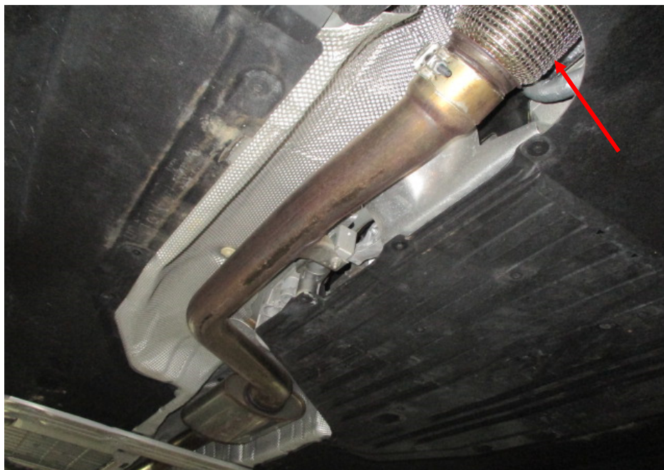
Photo 16 shows the Motor Car's catalytic convertor (arrowed). My examination of the Motor Car's exhaust system revealed no sign(s) or indication(s) of any cut or weld marks along its exhaust pipes and on its rear muffler.
