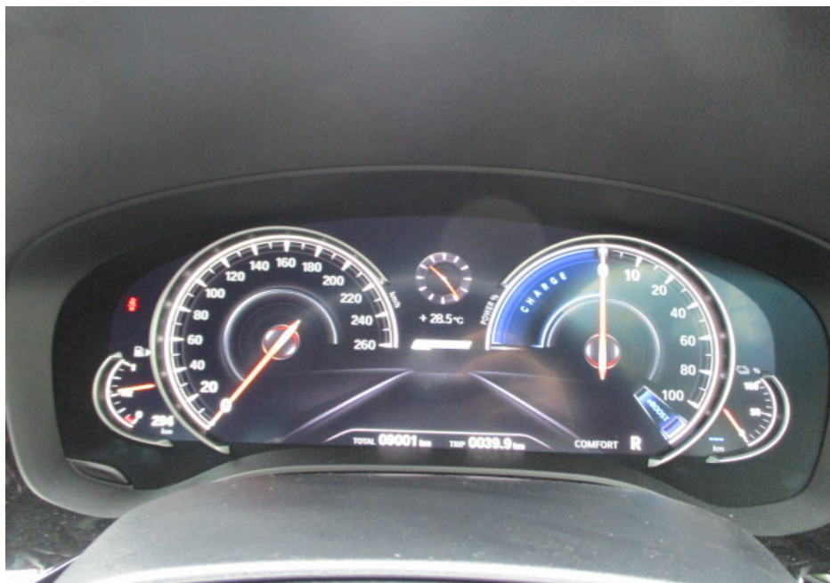
Photo 11 shows the respective warning lights no longer illuminated, indicating that there is no fault detected to the ABS, SRS, IAS, TPM and DSC systems of the Motor Car during the self-test. These electronic systems were hence in working condition at the time of my inspection.
