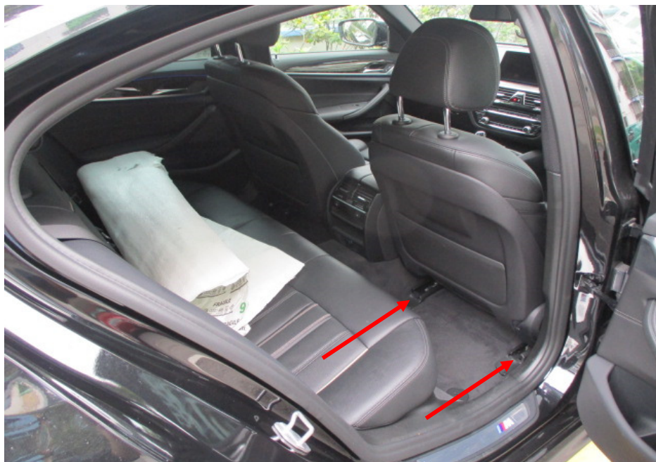
Photo 9 shows the seats of the Motor Car, which were secured via seat rails (arrowed) to the floor board. All the seats of the Motor Car were fitted with a retractable seat belt reel and pre-tensioner. The seat belts were tested and able to be fastened into the respective pre-tensions that were fitted on the side of each individual seat.
