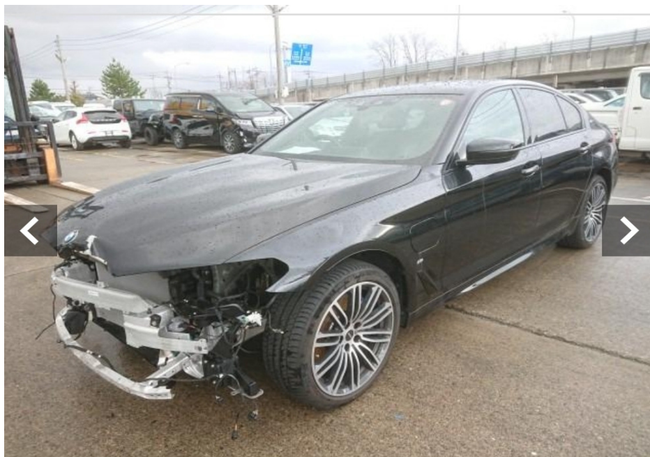
Photo 1 shows the front left body of the Motor Car prior to any repairs being carried out (photograph provided to me). The Motor Car was observed to have sustained damages at its frontal portion. The body parts observed to be damaged and/or dislodged had included its front bumper, front left headlamp, front bonnet, front bumper reinforcement and front radiator grilles amongst others. Basing on the photographs provided to me, the airbags of the Motor Car were not deployed.
