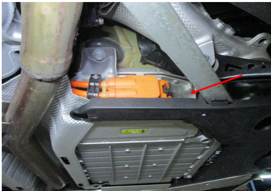
Photo 17 shows the Motor Car's electric battery that was fitted on the underside rear floor board (arrowed). The cable connections were checked and found to be securely fitted into the respective connectors. The electric battery was also observed to be fitted securely and not mounted onto any part of the Motor Car's chassis/structural body.
