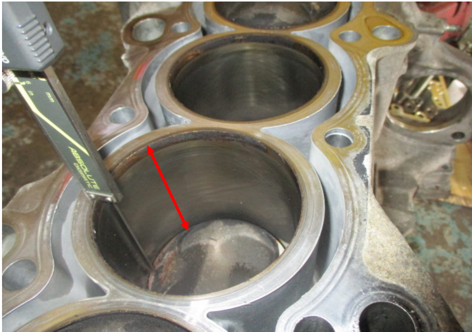
Photo 13 shows measurement of the stroke (arrowed) for cylinder 2 of the Honda engine that I had inspected.
