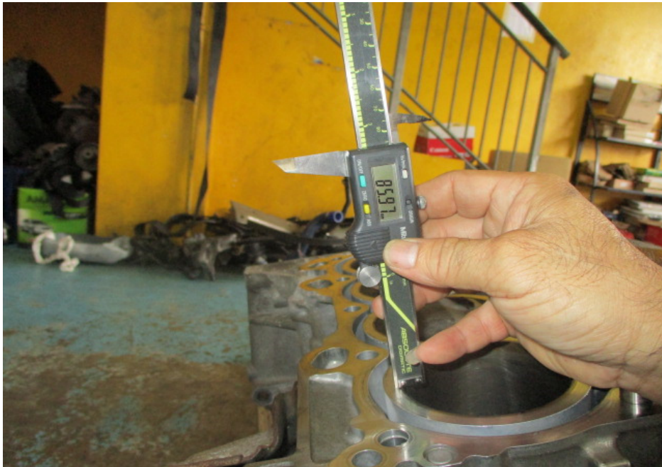
Photo 11 shows the stroke measurement of cylinder 1, which was recorded to be 85.97mm.
