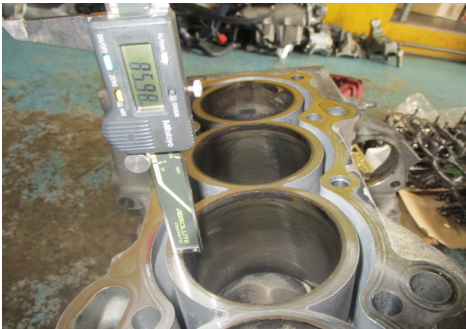
Photo 14 shows the stroke measurement of cylinder 2, which was recorded to be 85.98mm.
