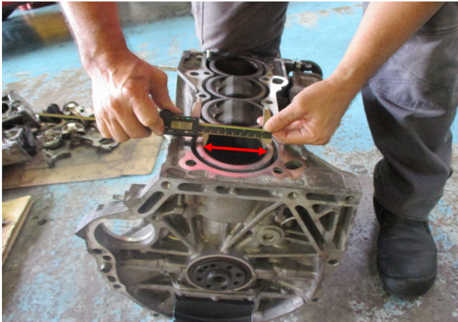
Photo 19 shows measurement being carried out to the bore (arrowed) of cylinder 4 of the Honda engine. The bore and stroke measurements of the Honda engine were carried out using a digital Vernier Caliper.
