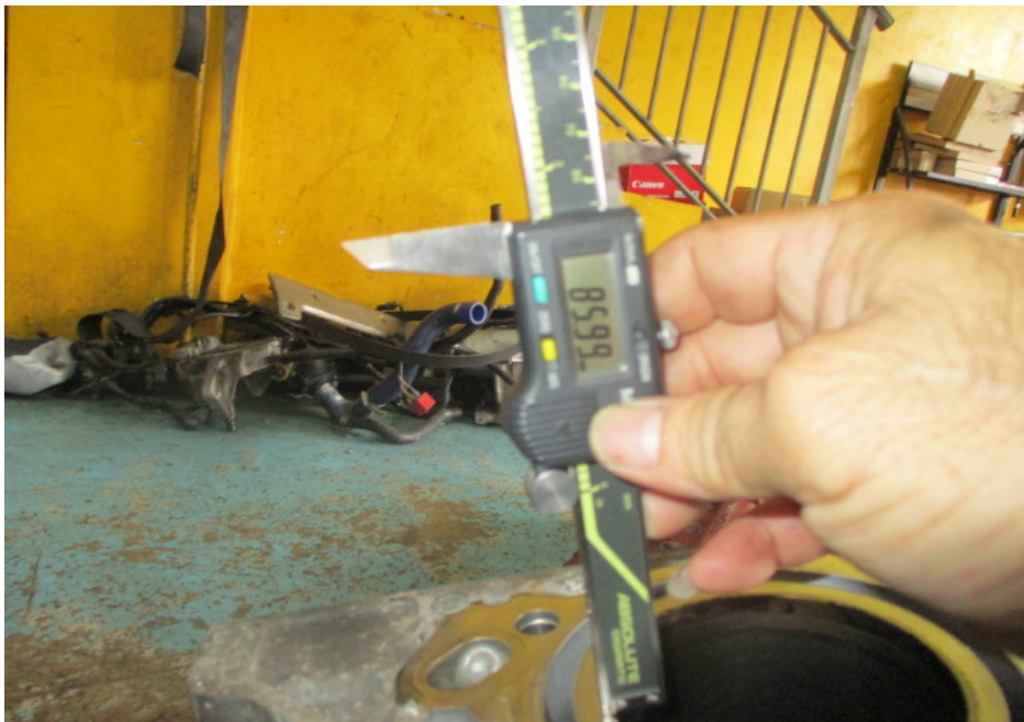
Photo 22 shows the stroke measurement of cylinder 4, which was recorded to be 85.99mm.
