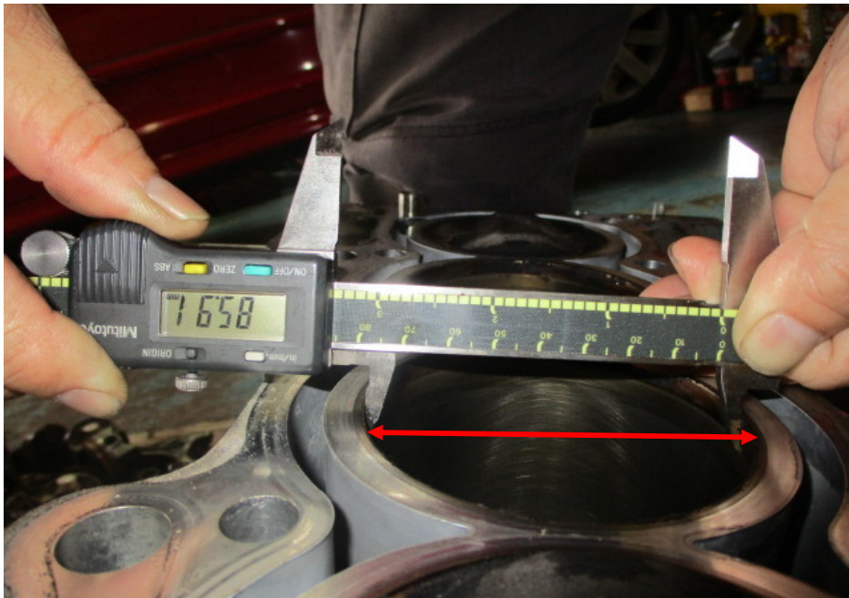
Photo 16 shows measurement being carried out to the bore (arrowed) of cylinder 3 of the Honda engine. The bore measurement of cylinder 3 was recorded to be 85.91mm.
