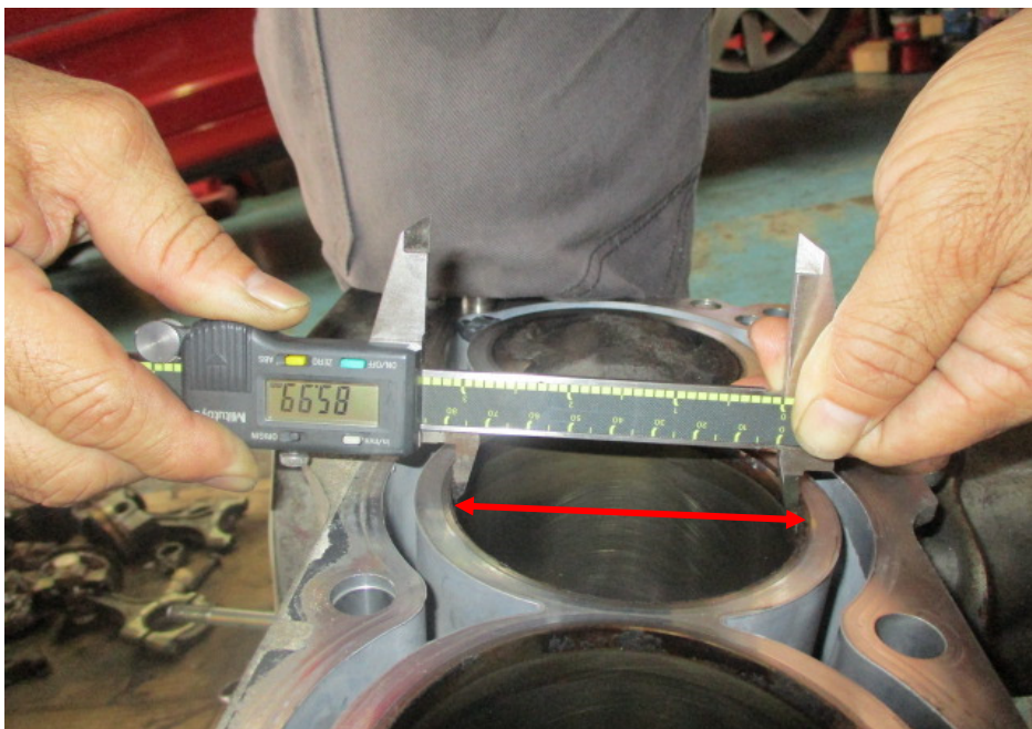
Photo 12 shows measurement being carried out to the bore (arrowed) of cylinder 2 of the Honda engine. The bore measurement of cylinder 2 was recorded to be 85.99mm.
