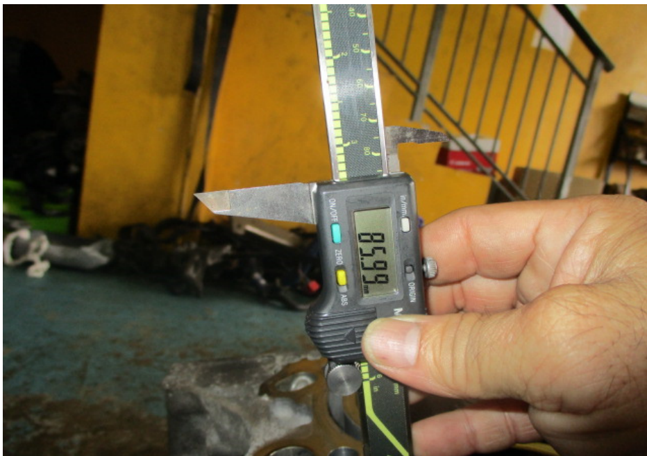
Photo 18 shows the stroke measurement of cylinder 3, which was recorded to be 85.99mm.
