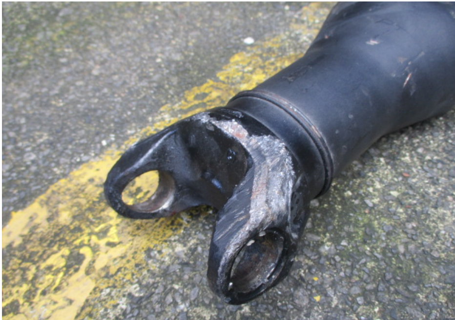
Photo 5 shows a close up view of the grazed/cut marks at one end of the PH's propeller shaft rear section.
