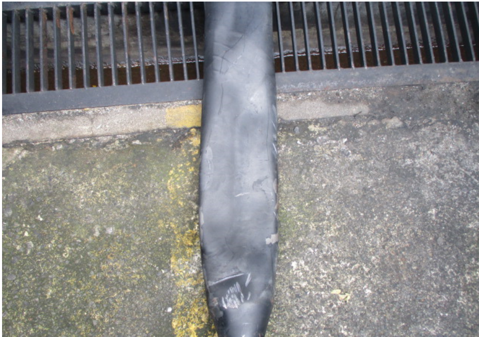
Photo 6 shows the propeller shaft rear section dented to a flatten shape from an original cylindrical shape.
