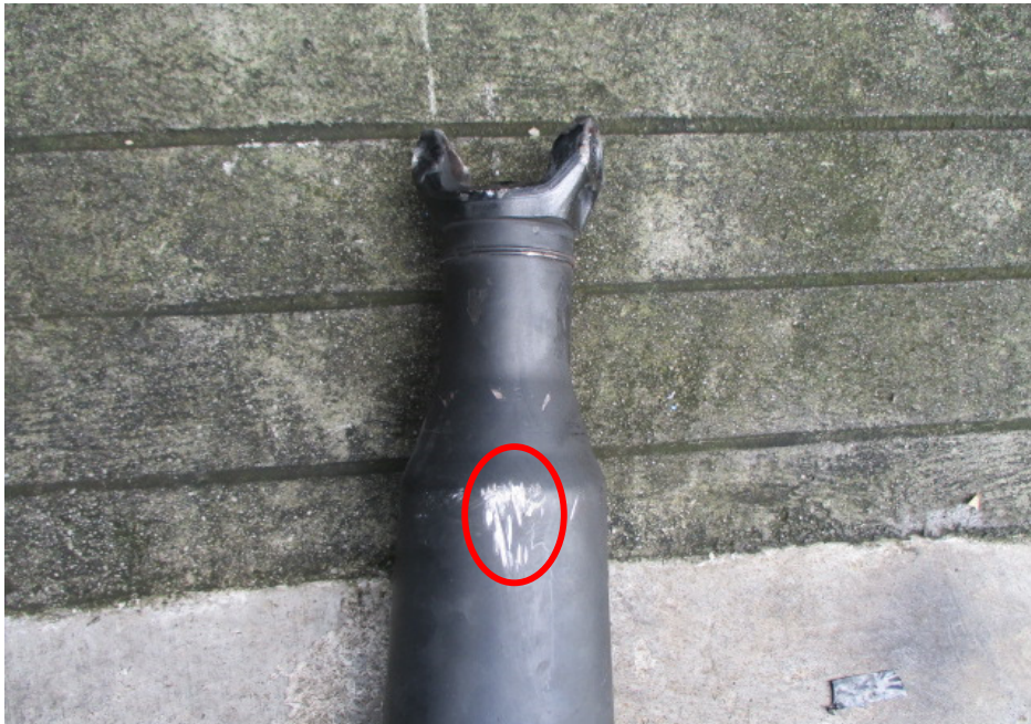
Photo 7 shows the grazed/cut marks (circled) at another area of the PH's propeller shaft rear section. Grazed/cut marks were found on multiple areas on the top and bottom sides of the rear section.
