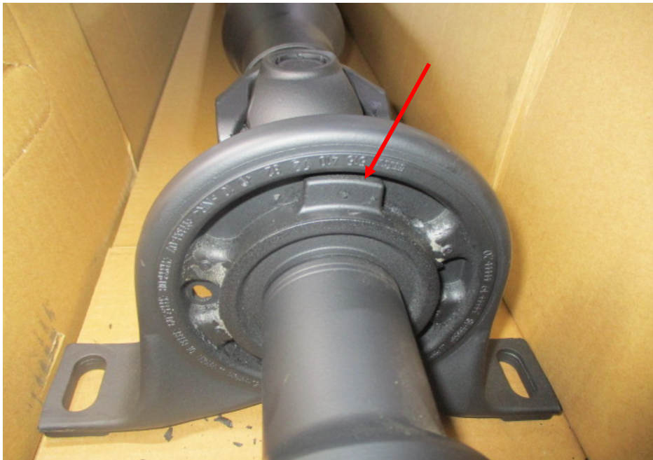
Photo 19 shows the same rubber bushing (arrowed) of a new propeller shaft front section for comparison purposes with the rubber bushing as seen in photograph 17 & 18 above.
