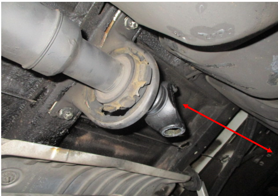
Photo 17 shows the propeller shaft front section of the PH. One end of the propeller shaft rear section is secured/attached to this front section via a "U" joint while the other end of the propeller shaft rear section is secured/attached to the differential gearbox as shown in photograph 16 above. The location where the propeller shaft rear section was supposed to be fitted is indicated by the red arrow. As seen from the photograph, the "U" joint was missing.
