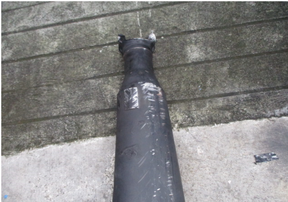
Photo 8 shows the grazed/cut marks at another area on the bottom side of the propeller shaft rear section.
