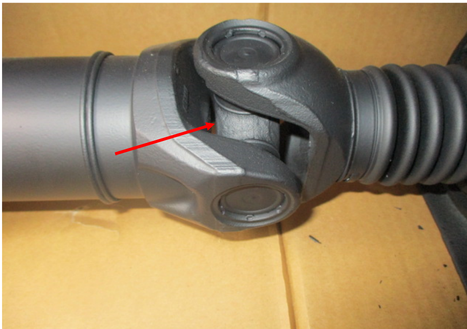
Photo 15 shows a closer view of the “U” joint (arrowed) of a new propeller shaft rear section. The “U” joint shown is for the end where the propeller shaft rear section is secured/attached to the propeller shaft front section. The purpose of the “U” joint is to secure/attach one end of the propeller shaft rear section to the propeller shaft front section and the other end to the input shaft of the differential gearbox. The “U” joint at the end of both sides of the PH’s damaged propeller shaft rear section was missing. Refer to photograph 5, 7 & 9 above.
