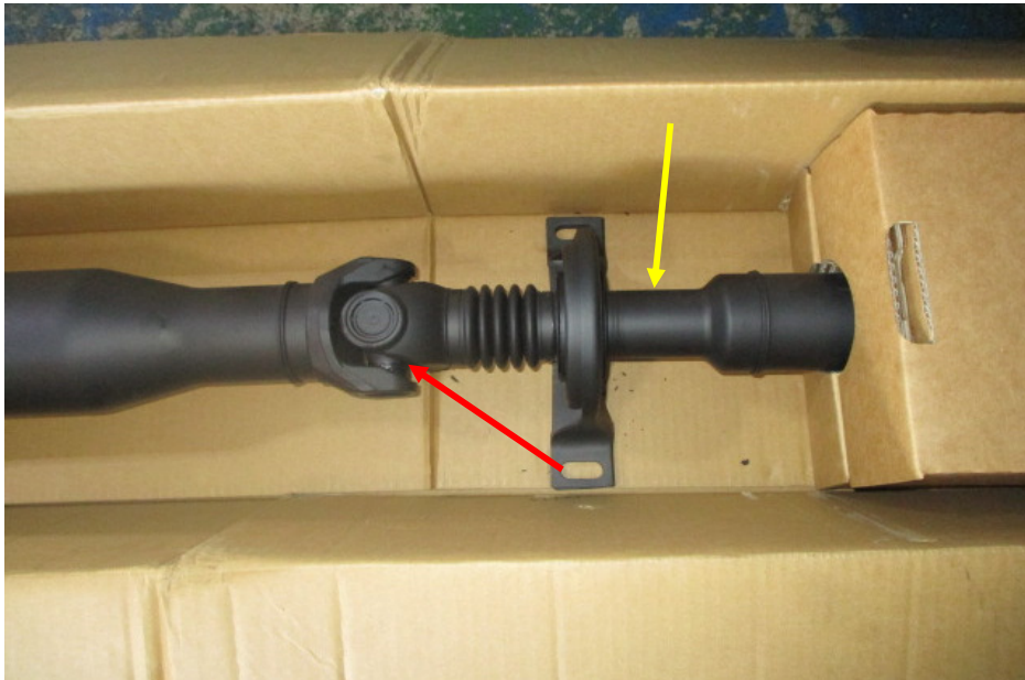
Photo 14 shows the “U” joint (red arrow) of a new propeller shaft rear section. The “U” joint, shown in the photograph above, is for the end that secures/attach the propeller shaft rear section to the propeller shaft front section (yellow arrow). The “U” joint at the end of both sides of the PH’s damaged propeller shaft rear section was missing. Refer to photograph 5, 7 & 9 above.
