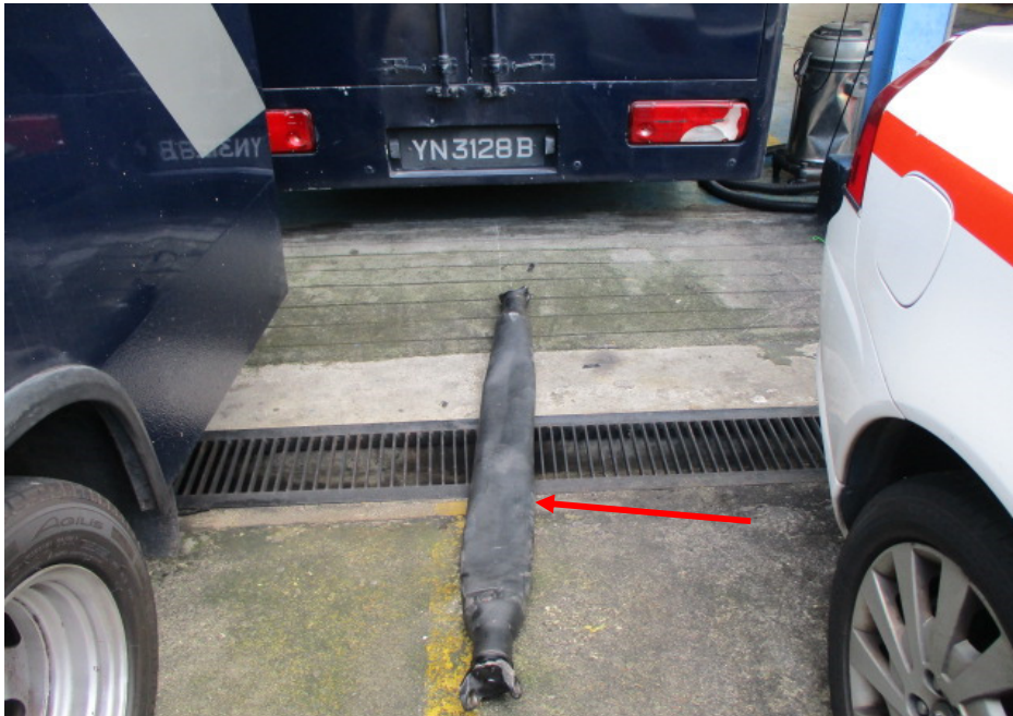
Photo 4 shows the dislodged rear section of the PH's propeller shaft (arrowed). From an original cylindrical shape, the rear section was observed to be dented to a flattened shape with grazed/cut marks at multiple areas on the top and bottom sides.
