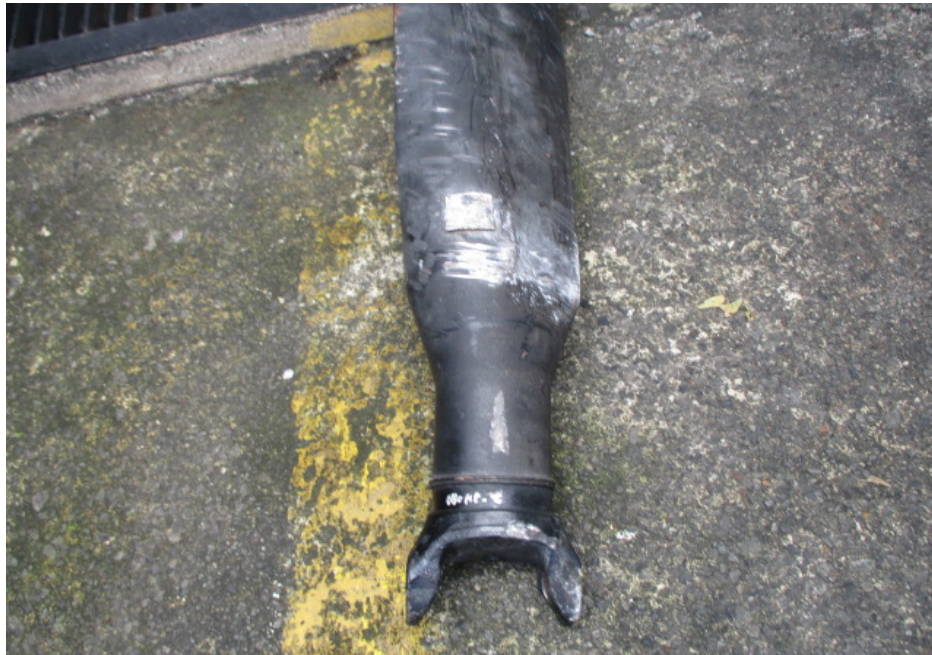
Photo 9 shows the grazed/cut marks at another area on the bottom side of the propeller shaft rear section. Generally, the dislodged rear section of the PH's propeller shaft, was observed to be dented. From an original cylindrical shape, it was dented to a flatten shape with grazed/cut marks at multiple areas on the top and bottom sides.
