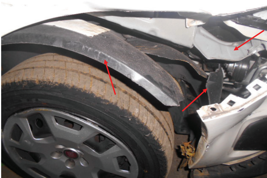
Photo 11 shows upon closer inspection, the Insured Vehicle also sustained damages to the front bumper retainer, right front fender liner and right front fender top garnish (arrowed).
