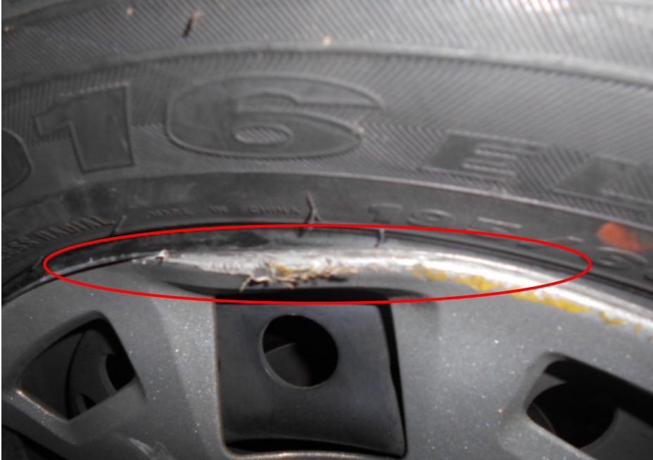
Photo 14 shows a close up view of the relatively minor marks of grazing nature observed around the edges of the front right wheel rim (circled) as a result of Mr Siva grazing the base of the railings.
