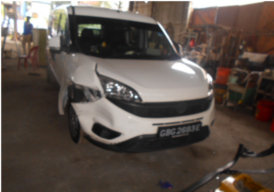
Photo 9 shows the general front view of the Insured Vehicle during the physical inspection at YK. The Insured Vehicle had sustained significant damages to its right portion, particularly to its front bonnet, front bumper, right front fender, right headlamp, and rear bumper.
