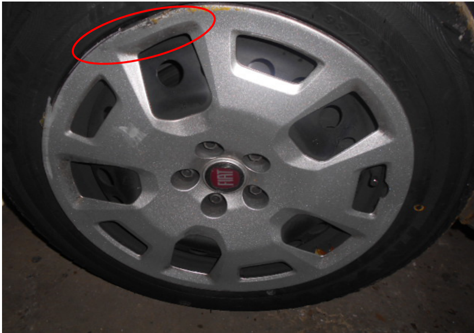
Photo 13 shows some relatively minor marks of grazing nature observed around the edges of the front right wheel rim (circled) as a result of Mr Siva grazing the base of the railings.
