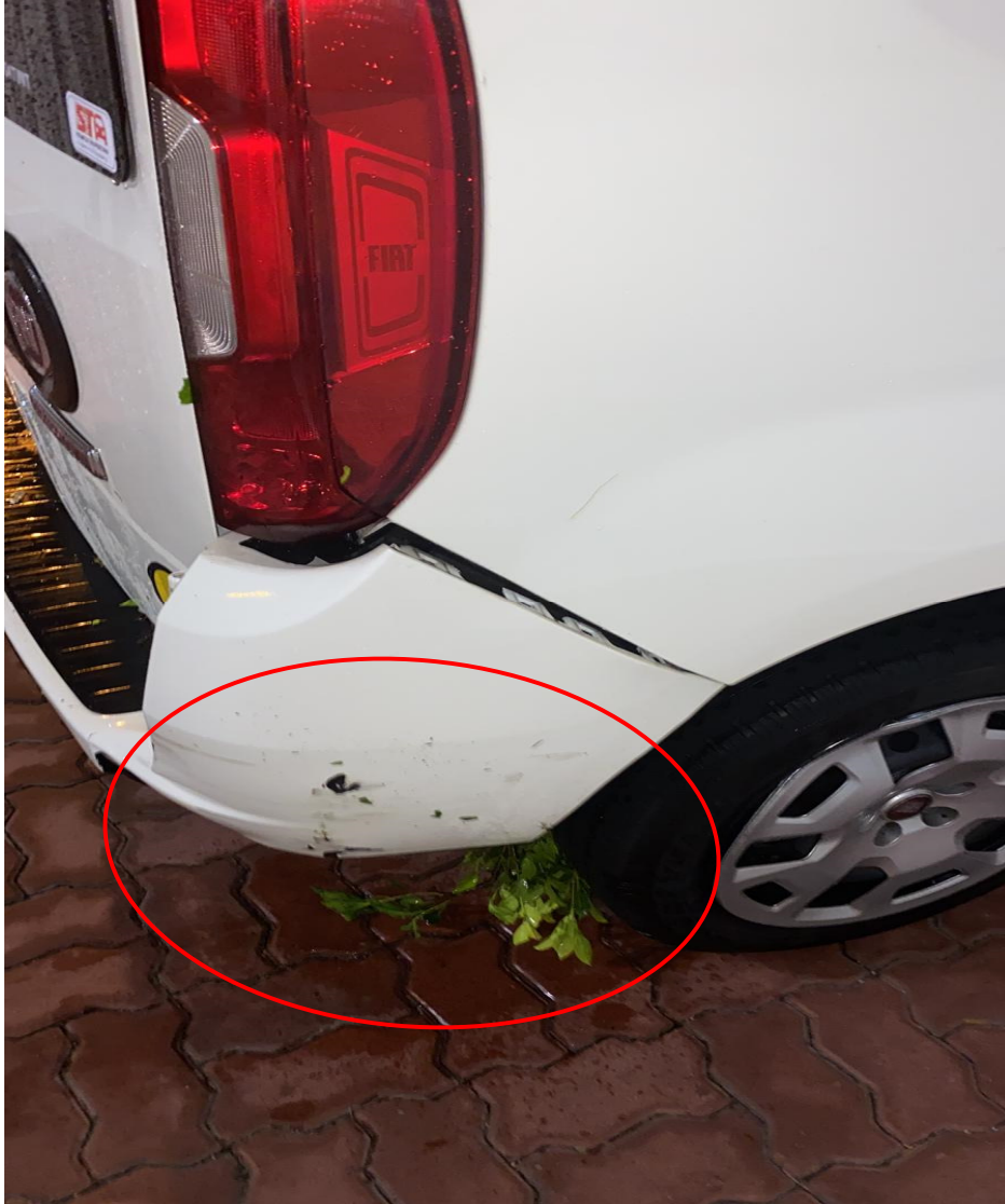
Photo 8 shows the right rear portion of the Insured Vehicle at the office premises post- incident. The Insured Vehicle had sustained damages at its right portion. The grass that was found stuck to the right rear portion of the Insured Vehicle (circled) correlates with Mr Siva's statement that the Insured Vehicle spun out of control into a grass patch along the road shoulder after he drove through a puddle of water.
