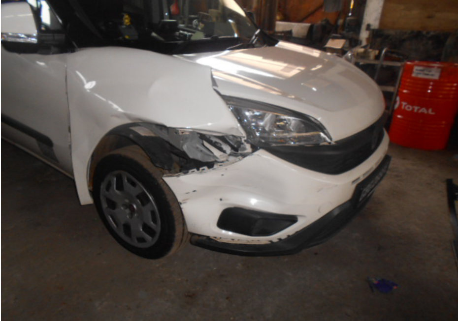
Photo 10 shows a closer view of the damaged front bonnet, front bumper, right front fender and right headlamp of the Insured Vehicle as a result of the incident.
