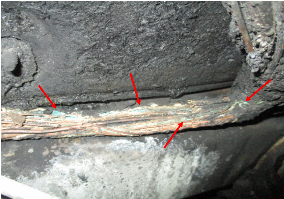
Photo 11 shows a close up view of the greenish residue found on some of the burnt stretches of original factory fitted wirings (arrowed). The presence of such greenish residue suggests occurrence of an electrical short circuit.
