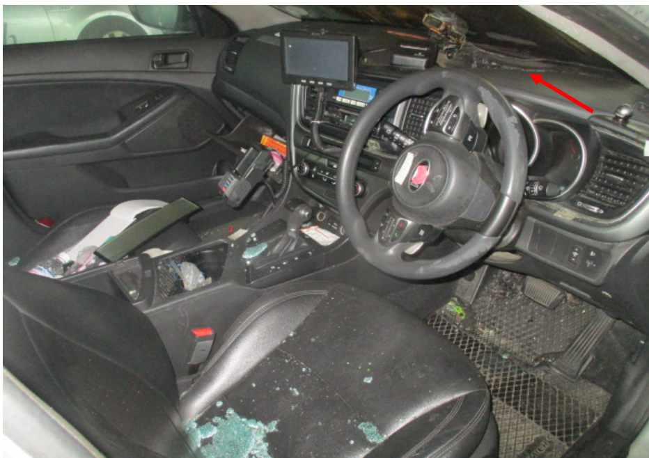
Photo 6 shows the interior compartment of the Insured Vehicle, which was slightly affected by the fire, particularly the dashboard (arrowed).
