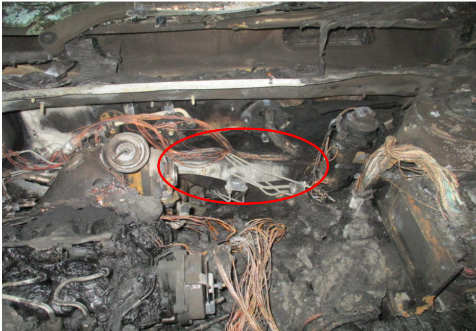
Photo 9 shows the original factory fitted wirings around the rear centre portion of the engine compartment, which is in the immediate vicinity where the fire to the Insured Vehicle had likely started. We had found greenish residue on several burnt stretches of these wirings (circled). The presence of such greenish residue indicates internal heating of copper wires, a sign of an electrical short circuit occurring. The greenish residue is normally left behind from oxidation as a result of chemical reaction involving the copper wires.
