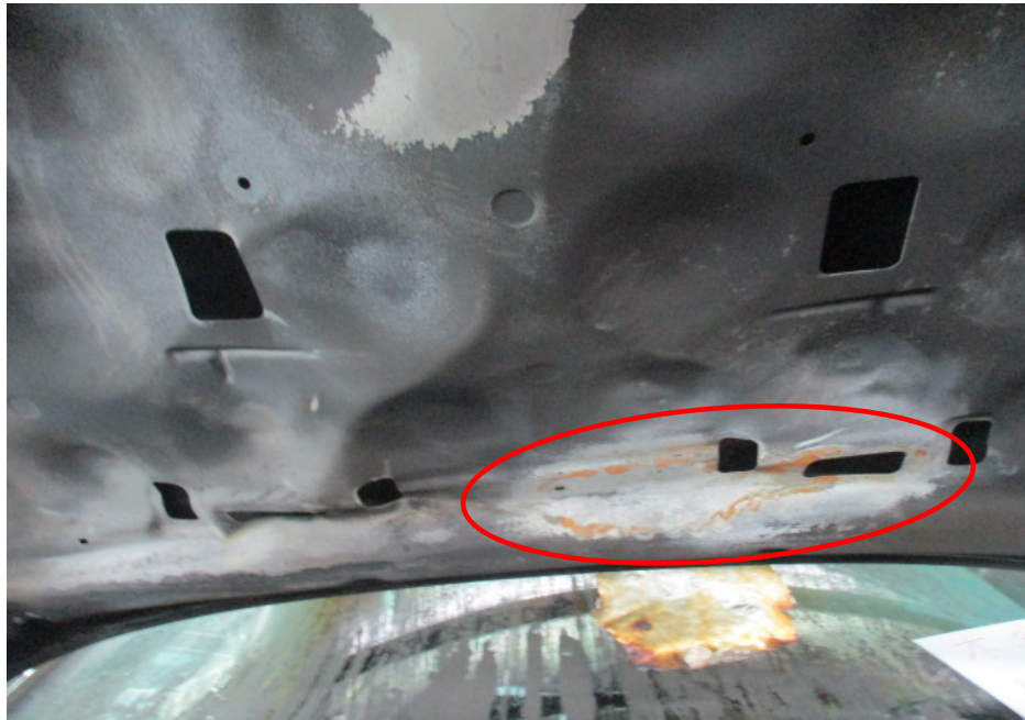
Photo 8 shows the rust that had developed on the underside of the front bonnet, around the bottom centre portion (circled). The development of rust is an indication that this area was subjected to prolonged exposure to high heat intensity, which had caused the steel/metal material of the front bonnet to be exposed to natural environmental condition. Hence the fire to the Insured Vehicle can be determined to have originated towards the rear centre portion of the engine compartment.
