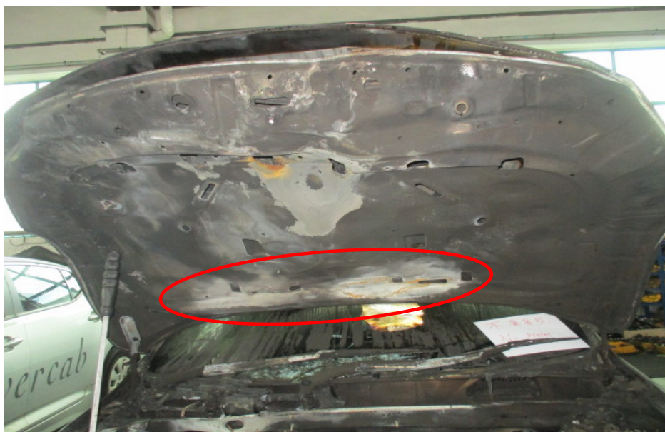
Photo 7 shows the burn pattern and whitish burn marks and also the rust that had developed on the underside of the front bonnet, at the bottom centre portion of the Insured Vehicle (circled). Such whitish burn marks are a result of exposure to prolonged heat intensity, which may indicate where the fire had started. Rust would also begin to develop on these areas soon after the fire.
