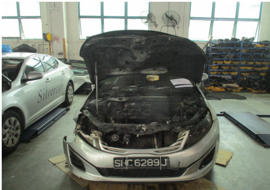
Photo 2 shows the general view of the front portion of the Insured Vehicle at the time of our inspection. The fire damage to the Insured Vehicle was confined to its front portion. Its front bumper, front bonnet, front grille, front headlamps, front windscreen, front rims and front tyres were amongst the body parts that were found to have been affected as a result of the fire.
