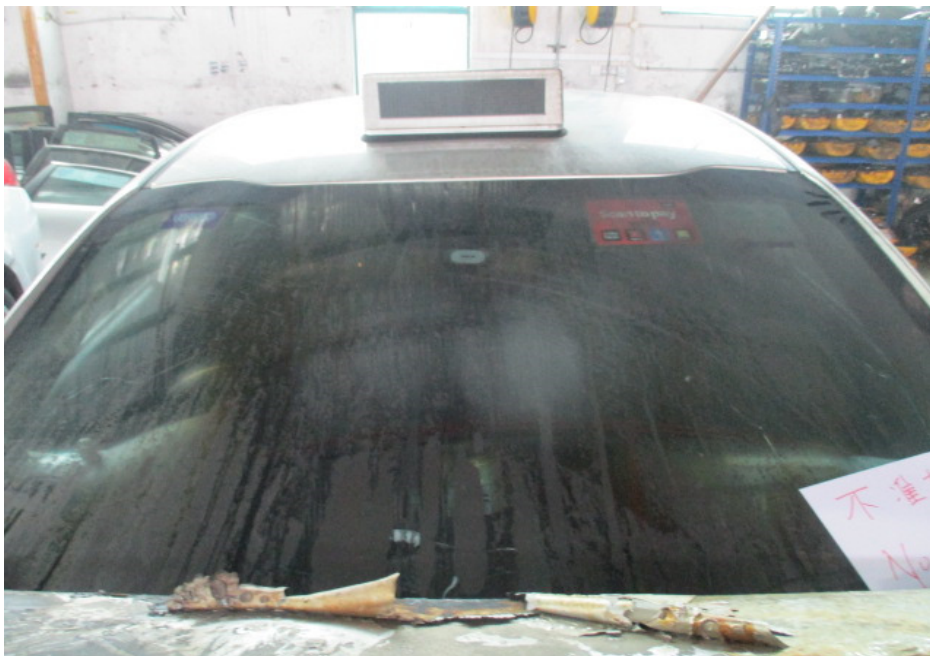
Photo 4 shows the general view of the front windscreen of the Insured Vehicle at the time of our inspection. The front windscreen was seriously affected by the fire.
