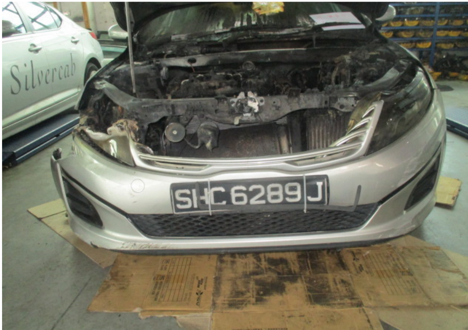
Photo 3 shows a closer view of the front portion of the Insured Vehicle at the time of our inspection. The fire damage to the Insured Vehicle was confined to its front portion. Its front bumper, front bonnet, front tyres and front headlamps were amongst the body parts that were found to have been affected by the fire.
