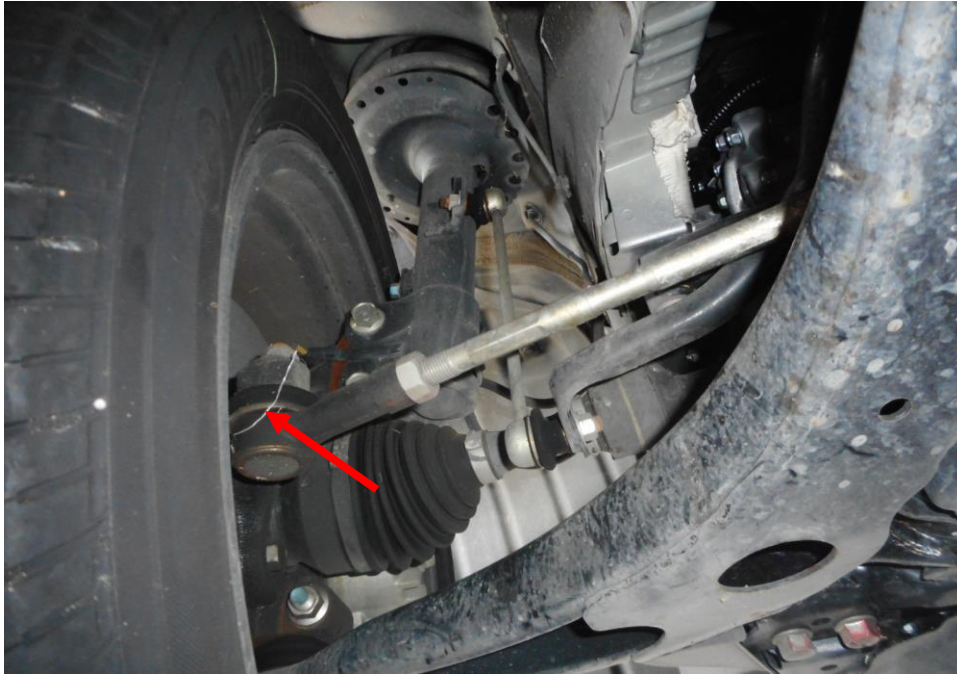
Photo 22 shows the various undercarriage components at the front left wheel of the Motor Car, which had included the steering tie rod (arrowed). The various undercarriage components of the Motor Car were all found to be intact without any visible damage.
