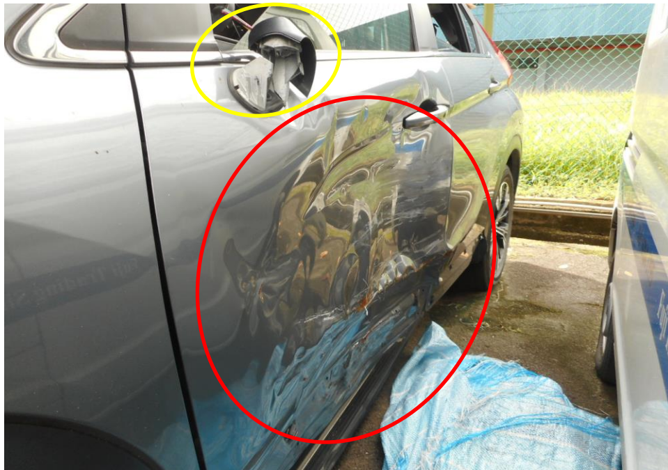
Photo 3 shows the close up view of the Motor Car's left body at the time of my inspection. The Motor Car was observed to have sustained damage at its front left door panel (red circle) and its rear view mirror (yellow circle), as a result of the accident.
