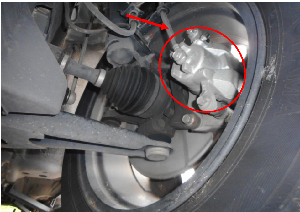
Photo 19 shows the brake hose/pipe (arrowed) at the front left wheel of the Motor Car. No leakage of brake fluid was observed. Visual examination of the various components of the braking system like the brake caliper (circled), brake booster, brake pedal etc had revealed all to be intact and without visible damage.
