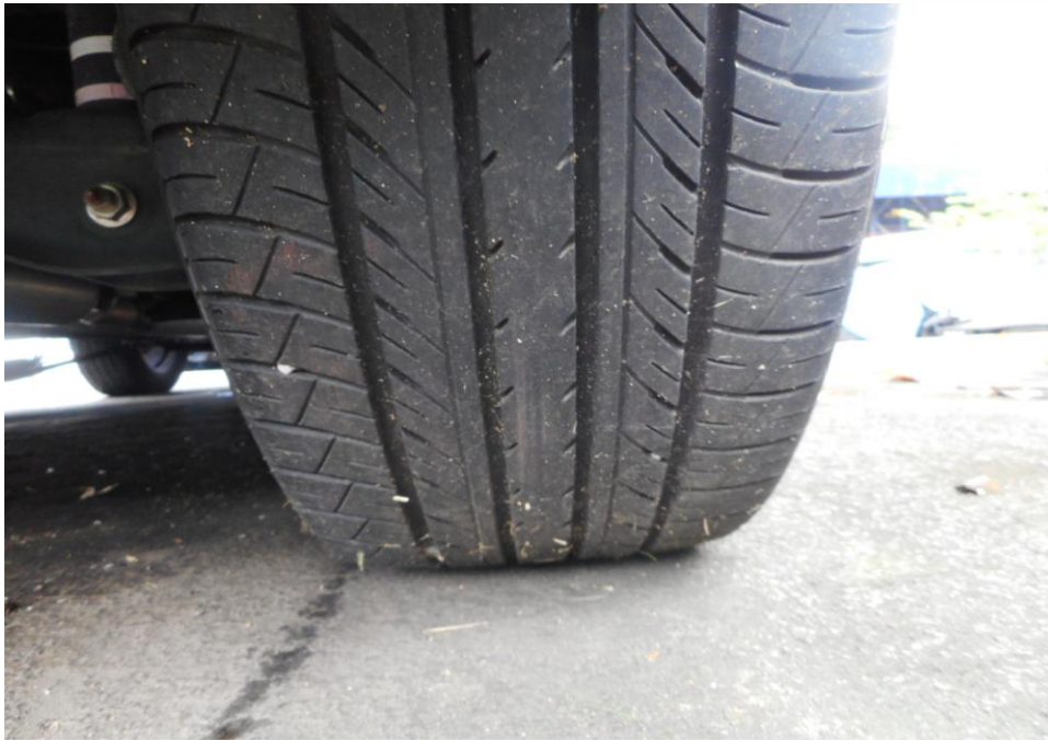
Photo 8 shows the condition of the rear right tyre of the Motor Car, which was observed to be in serviceable condition with remaining tread depth of approximately 5.2mm. The tyre was also observed to be sufficiently inflated for vehicular operation with no tear, cut or burst mark(s).
