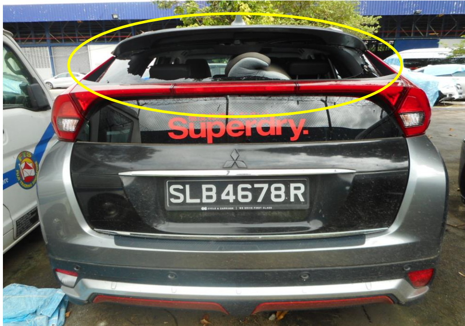
Photo 6 shows the general view of the Motor Car's rear body at the time of my inspection. The Motor Car rear windscreen (circled) was observed to be damaged as a result of the accident.
