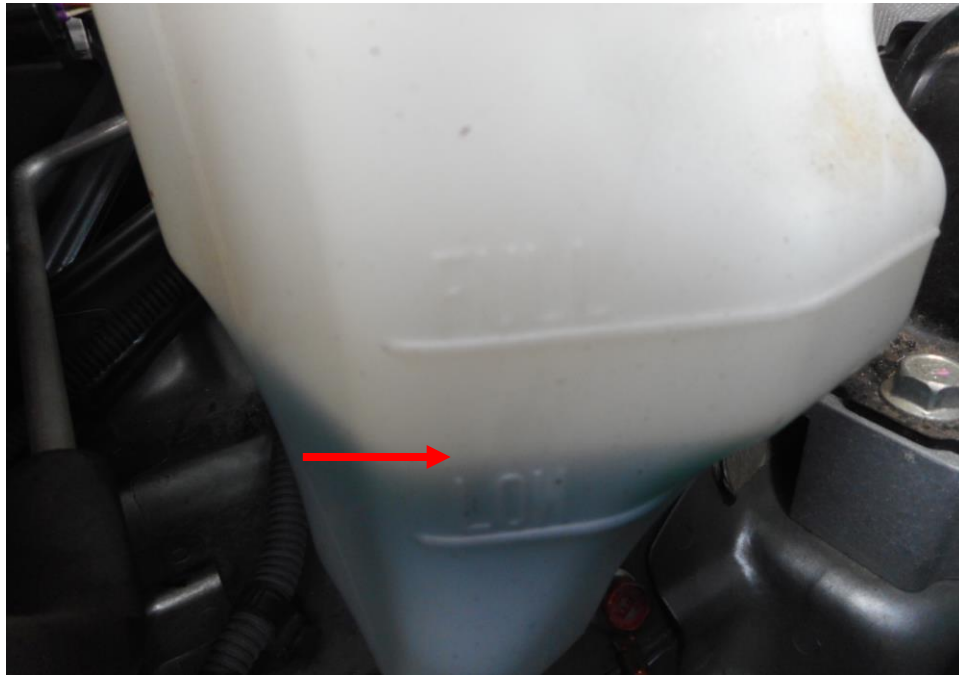
Photo 13 shows checks being carried out to the engine coolant of the Motor Car at the time of my inspection. The engine coolant was observed to be of sufficient level (arrowed) and without any visible contamination.
