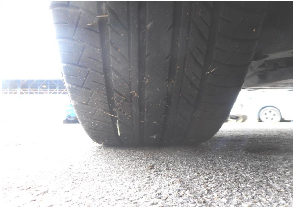
Photo 10 shows the condition of the front left tyre of the Motor Car, which was observed to be in serviceable condition with remaining tread depth of approximately 4.9mm. There was also no tear, cut or burst mark(s) on the outer and the inner sidewalls as well as across the tread of the Motor Car's 4 tyres.
