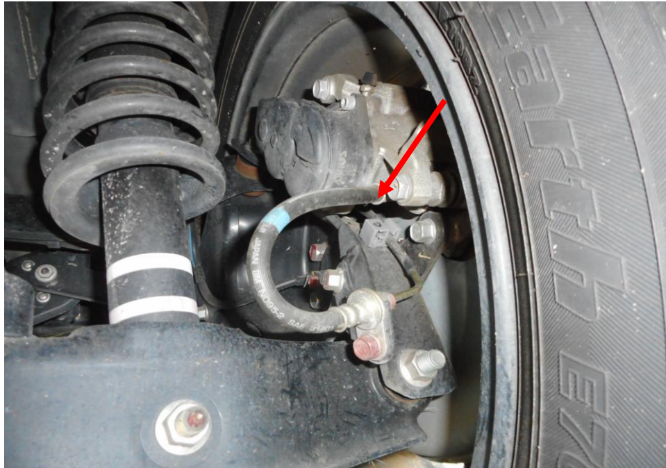
Photo 16 shows the brake hose/pipe (arrowed) at the rear right wheel of the Motor Car. No leakage of brake fluid was observed. Visual examination of the various components of the braking system like the drum brake, brake booster, brake pedal etc. had revealed all to be intact and without visible damage.
