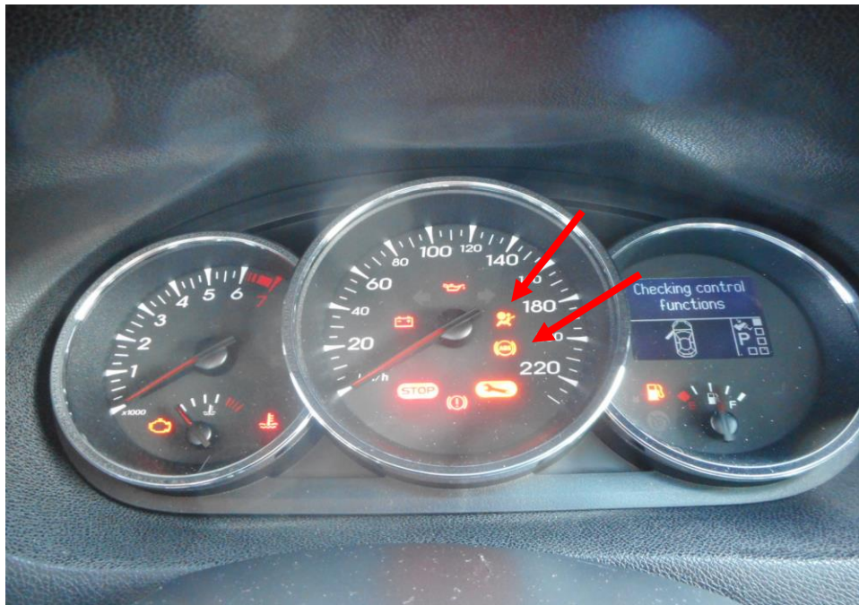
Photo 22 shows the warning light for Anti-Lock Brake System (ABS) and Supplemental Restraint System (SRS) (arrowed) appearing on the instrument panel of the Motor Car during the self-test of its various electronic operating systems when its engine was cranked.
