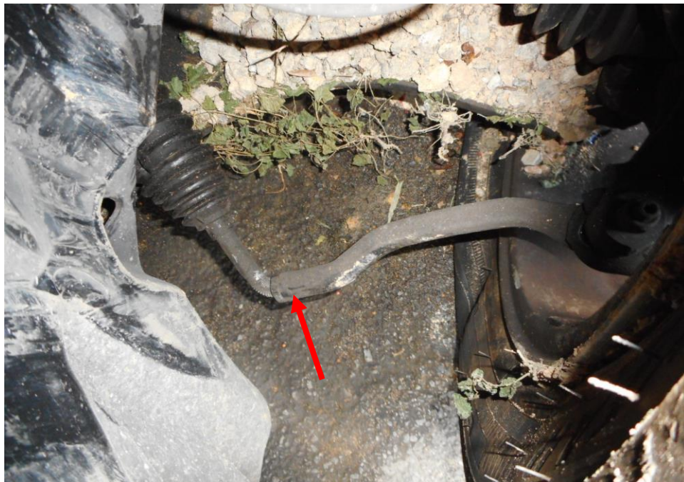
Photo 21 shows the various undercarriage components at the front right wheel of the Motor Car, the steering tie rod (red arrow) was observed to be damaged as a result of the accident.
