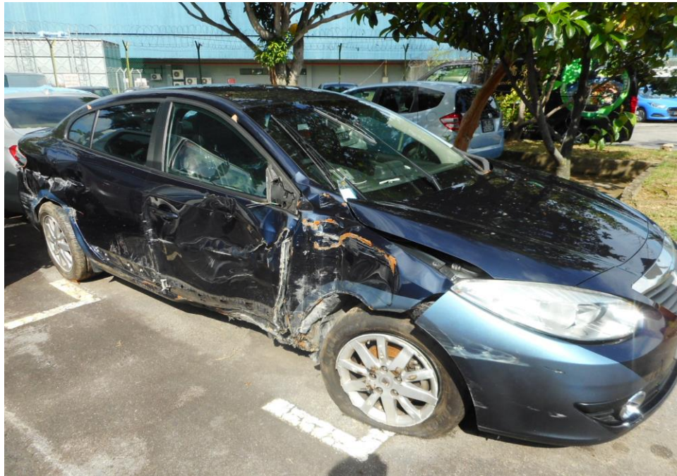
Photo 2 shows a general view of the Motor Car's right body at the time of my inspection. The Motor Car was observed to have sustained damage at its right portion. Its front bumper, front right fender and right body panels were amongst the body parts that were damaged as a result of the accident.
