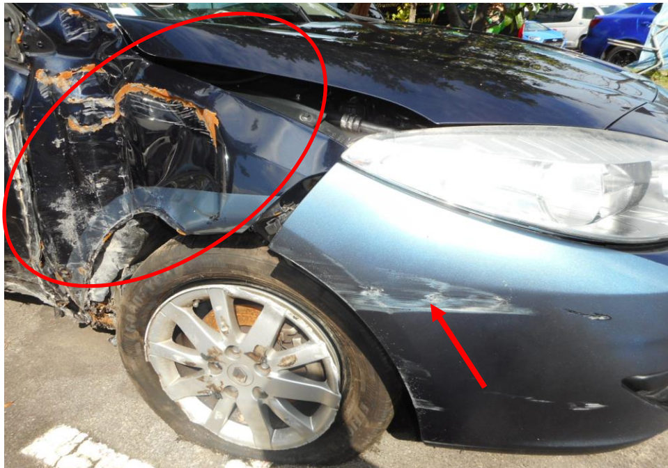
Photo 3 shows the close up view of the Motor Car's right portion at the time of my inspection. The Motor Car was observed to have sustained damage at its front bumper (arrowed) and front right fender (circled) as a result of the accident.
