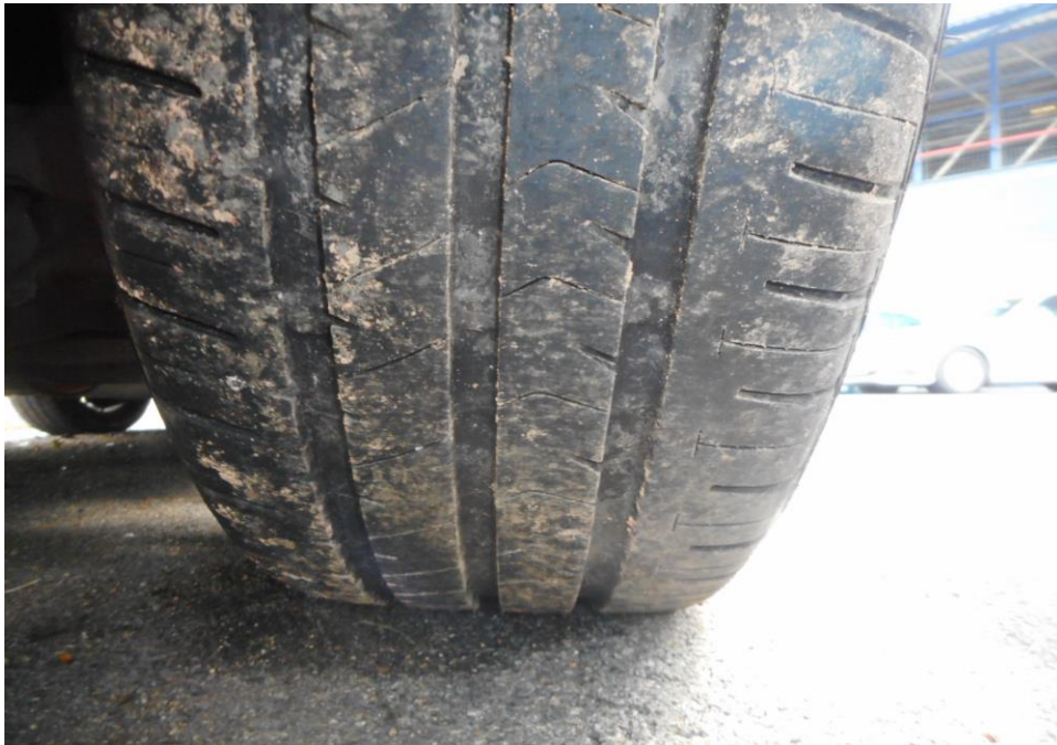
Photo 8 shows the condition of the rear right tyre of the Motor Car, which was observed to be in serviceable condition with remaining tread depth of approximately 6.1mm. The tyre was also observed to be sufficiently inflated for vehicular operation with no tear, cut or burst mark(s).
