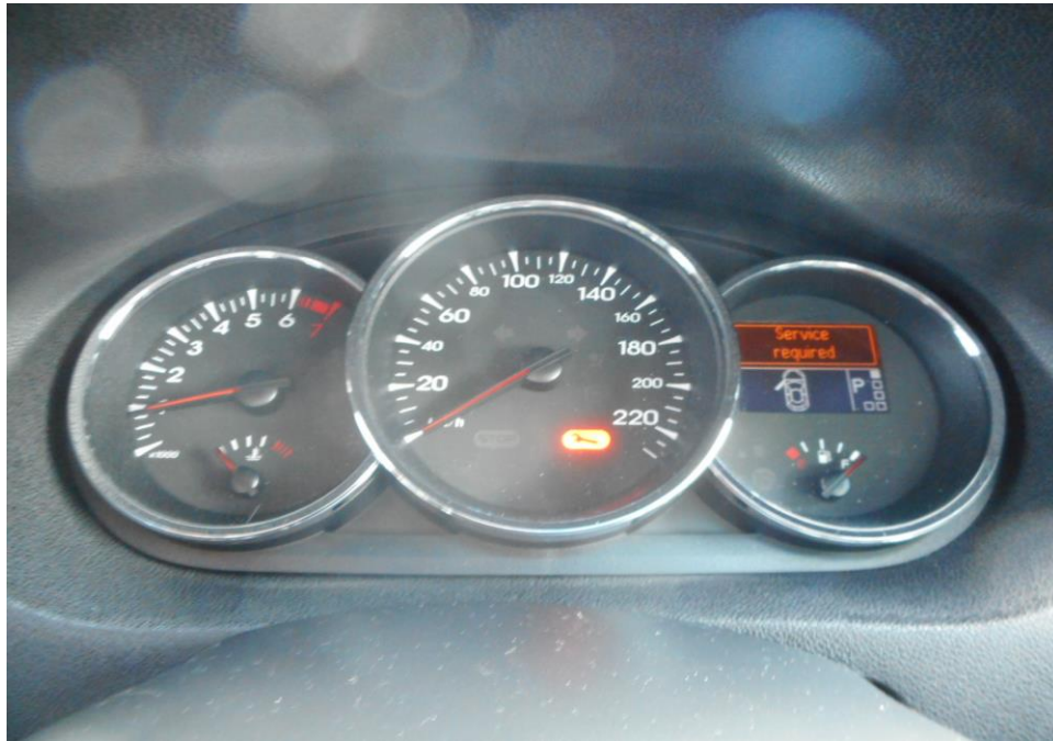
Photo 23 shows no warning lights illuminated on the instrument panel of the Motor Car after the engine was cranked. This would suggest that there was no abnormality to the electronic operating system of the Motor Car, like the ABS and SRS etc.
