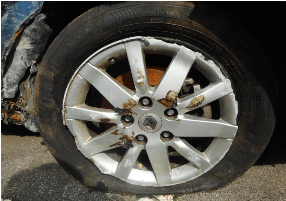
Photo 7 shows the condition of the front right tyre of the Motor Car, which was observed to be in unserviceable condition as it was damaged as a result of the accident with remaining tread depth of approximately 5.7mm.
