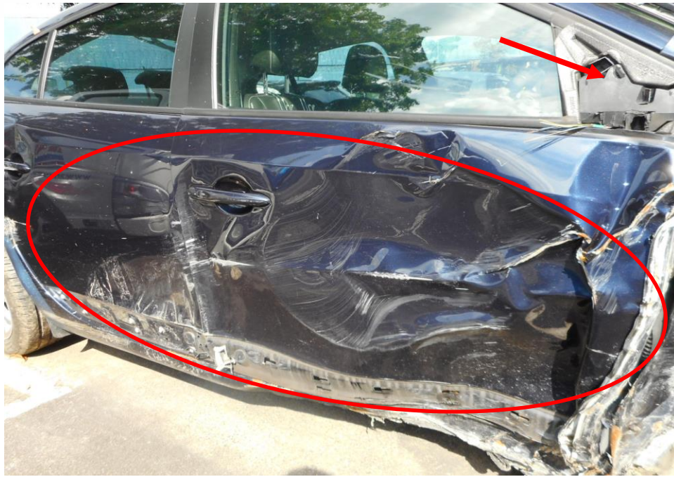
Photo 4 shows the close up view of the Motor Car's front right body at the time of my inspection. The Motor Car was observed to have sustained damage at its right rear view mirror (arrowed) right body panel (circled) as a result of the accident.
