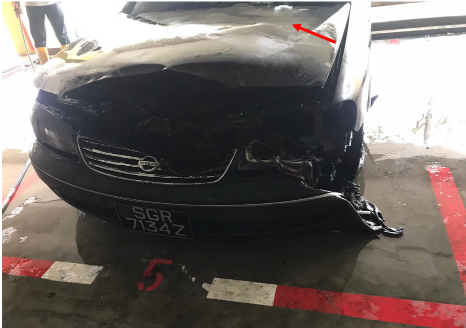
Photo 13 shows the Insured Vehicle at the incident scene after the fire was extinguished. Whitish burn marks (arrowed) were observed on the rear left portion of the front bonnet, which indicates that the fire had started in the engine compartment.
