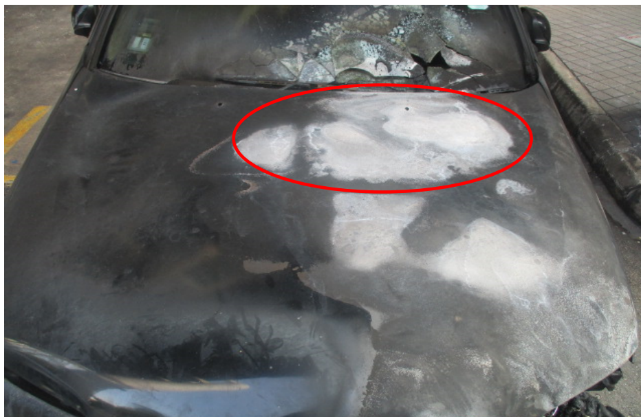
Photo 7 shows the burn pattern and whitish burn marks (circled) that were found on the rear left side of the front bonnet of the Insured Vehicle. Such whitish burn marks are a result of exposure to prolonged heat intensity, which may indicate where the fire had started. Rust would also begin to develop on these areas soon after the fire.
