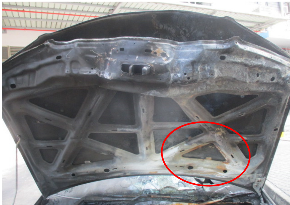
Photo 8 shows the rust (circled) that had developed on the underside of the front bonnet, around the bottom left area. The development of rust is an indication that this area was exposed to prolonged exposure to high heat intensity, which had caused the steel/metal material of the front bonnet to be exposed to natural environmental condition. Hence the fire to the Insured Vehicle can be determined to have originated towards the rear left portion of the engine compartment.
