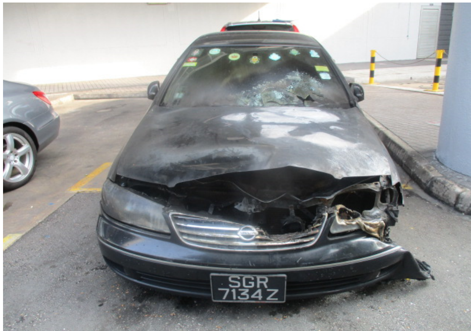
Photo 1 shows the general view of the front portion of the Insured Vehicle at the time of our inspection. The fire damage to the Insured Vehicle was confined to its front portion. Its front bonnet, front grille, front windscreen and front headlamps were amongst the body parts that were found to have been affected as a result of the fire.
