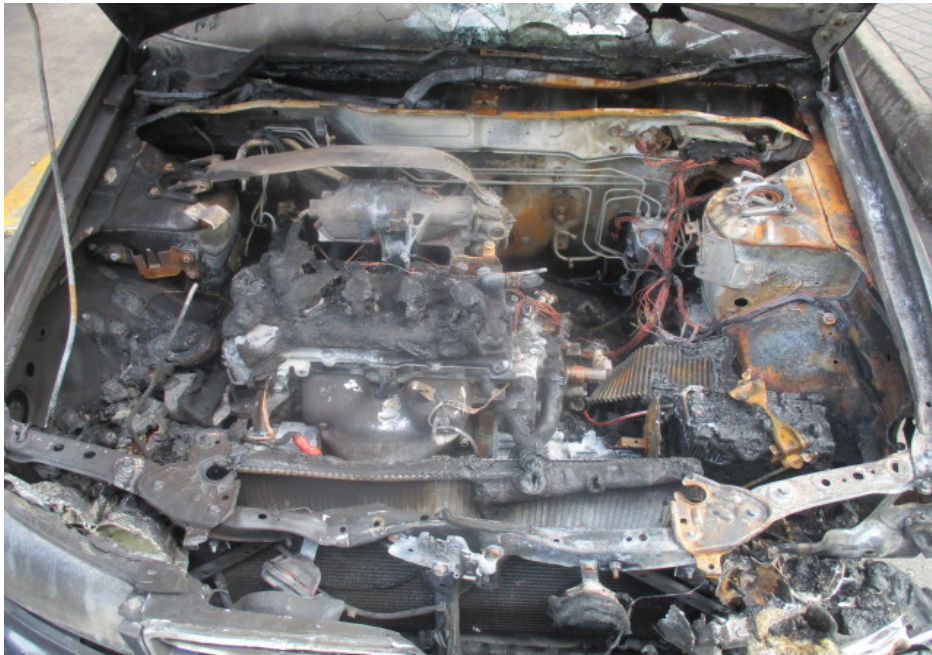
Photo 5 shows the engine compartment of the Insured Vehicle at the time of our inspection. The nature of fire damage to the engine compartment of the Insured Vehicle was observed to be extensive. Most of the parts inside the engine compartment were found to be severely burnt and/or melted as a result of the fire.
