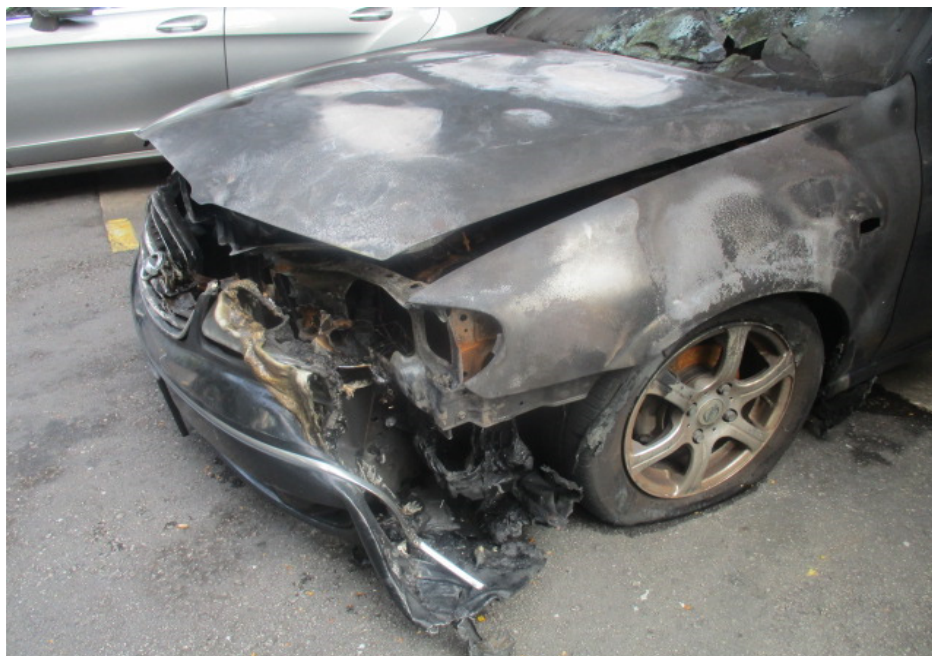
Photo 2 shows the general view of the front left portion of the Insured Vehicle at the time of our inspection. The fire damage to the Insured Vehicle was confined to its front portion. Its front bonnet, left front panel and front left headlamp were amongst the body parts that were found to have been affected as a result of the fire.
