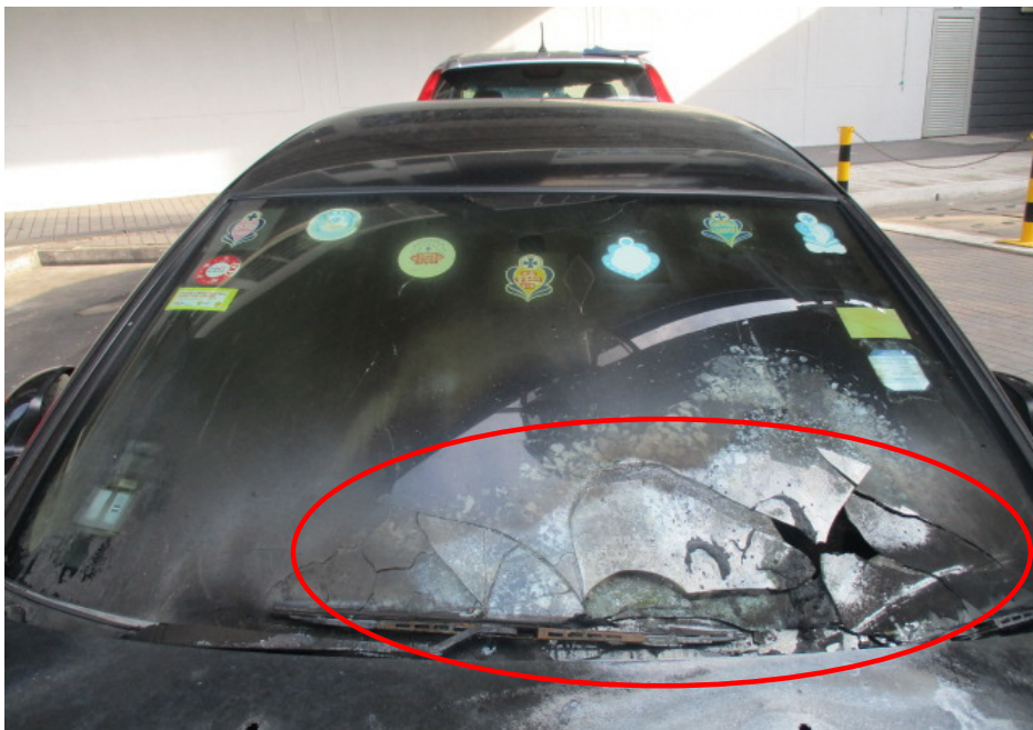
Photo 4 shows the general view of the front windscreen of the Insured Vehicle at the time of our inspection. The fire damage to the Insured Vehicle was confined to its left portion (circled).
