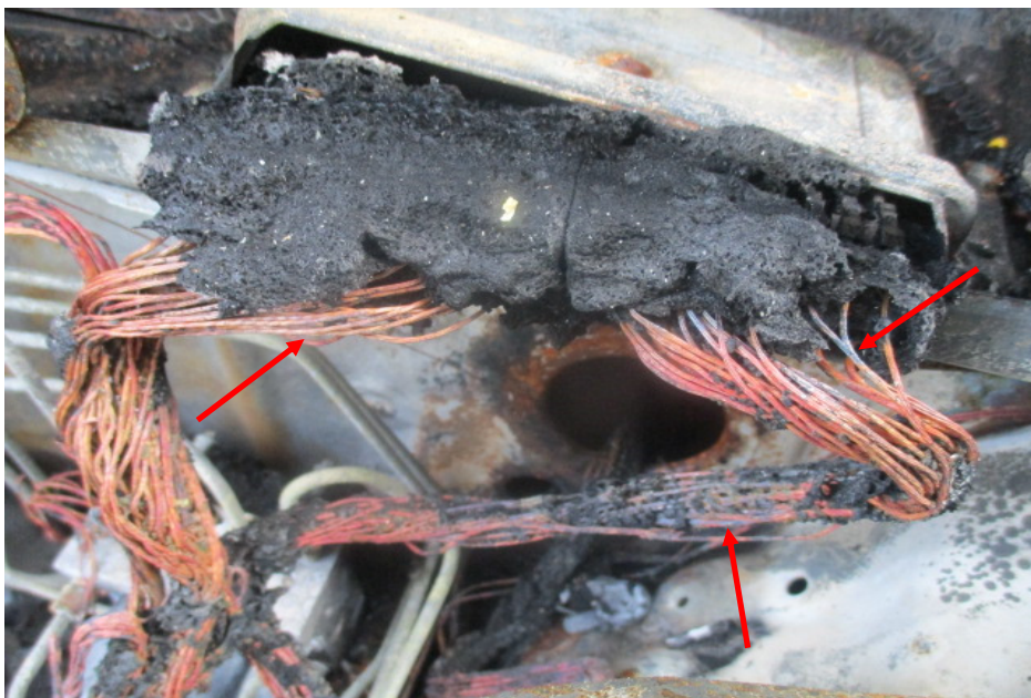
Photo 10 shows a closer view of some of the wirings with greenish residue (red arrows). The presence of such greenish residue suggest occurrence of an electrical short circuit.
