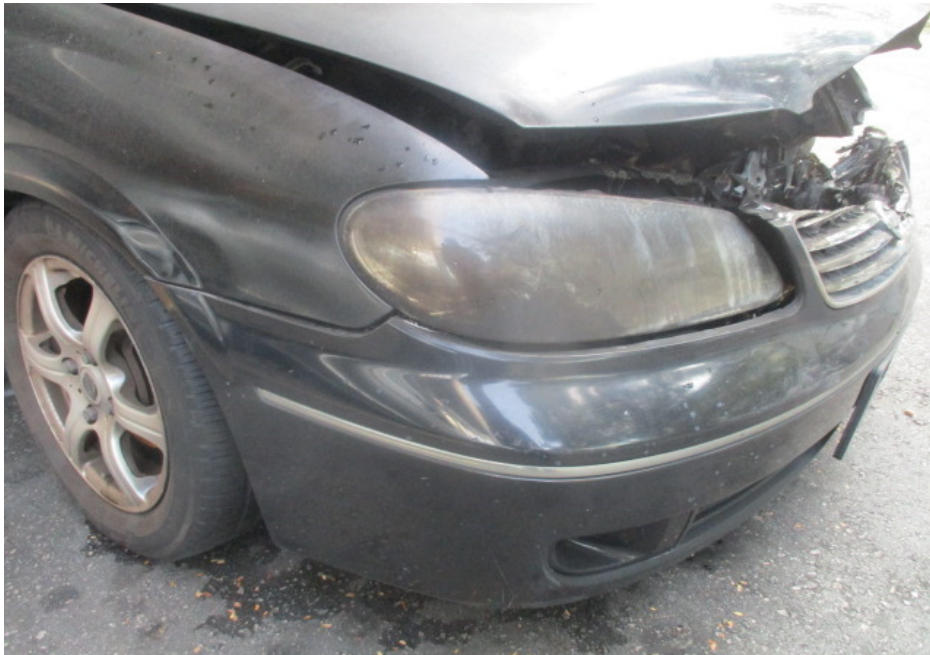
Photo 3 shows the general view of the front right portion of the Insured Vehicle at the time of our inspection. The fire damage to the Insured Vehicle was confined to its front portion. Its front bonnet, right front panel and front right headlamp were amongst the body parts that were found to have been affected as a result of the fire.
