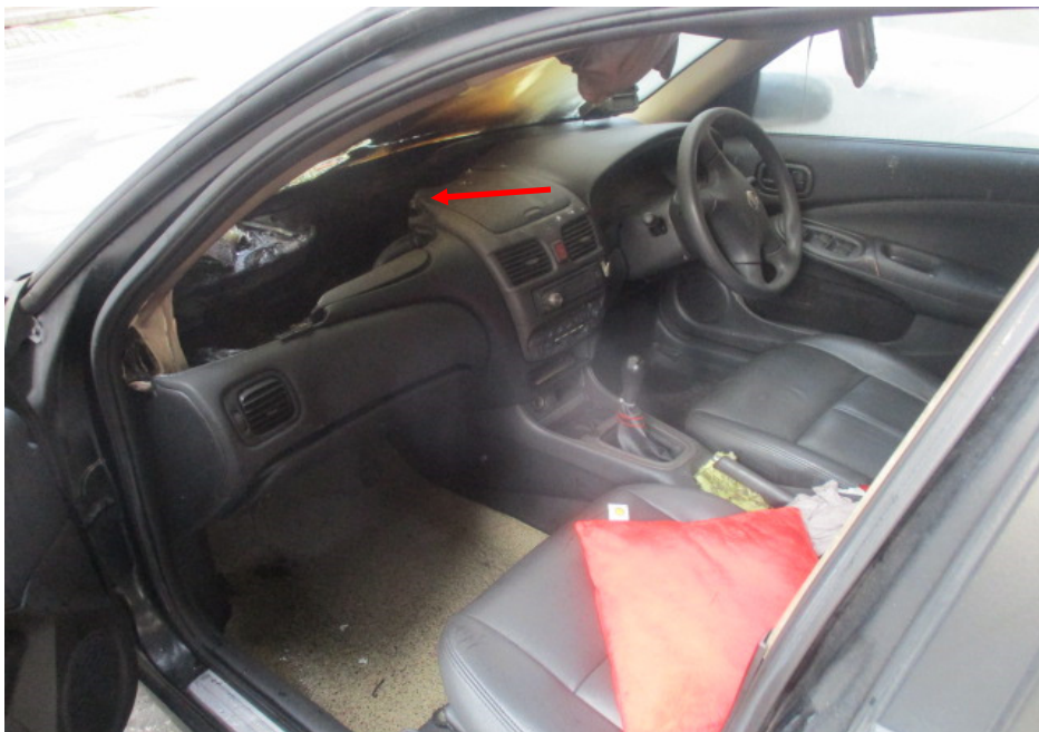
Photo 6 shows the interior compartment of the Insured Vehicle which was observed to be slightly affected by the fire, particularly the left portion of the dashboard (arrowed).
