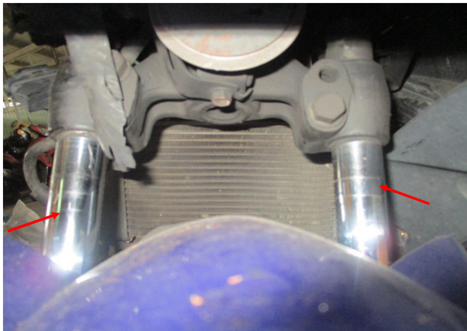
Photo 18 shows the front fork (arrowed) of the Motorcycle. The front fork and fork bracket of the Motorcycle were both found to be intact and undamaged. Turning the Motorcycle's handle bar towards the left and right did not produce any abnormal free play. The steering system of the Motorcycle was in serviceable condition at the time of our inspection.
