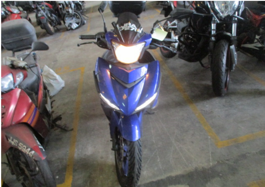
Photo 2 shows a general view of the front body of the Motorcycle at the time of our inspection. The Motorcycle was observed to have sustained damages frontal portion and right body.
