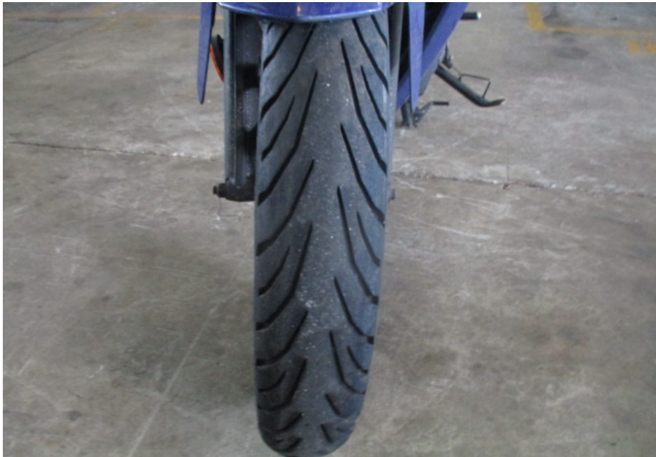
Photo 12 shows the front tyre of the Motorcycle at the time of our inspection. The front tyre was observed to be in serviceable condition with remaining tread depth of approximately 4mm. The pattern of the tread was also clearly visible. There was no tear, burst mark(s) and/or punctured hole(s) on the sidewalls as well as across the tread of the front tyre.
