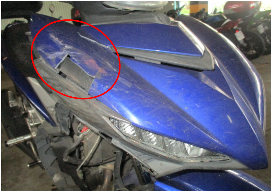
Photo 4 shows a close up view of the cracked front cowling (circled) which was amongst the body parts of the Motorcycle that had sustained damage as a result of the accident.
