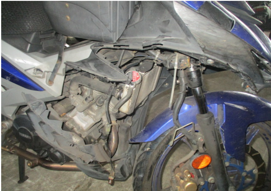
Photo 6 shows a closer view of the cracked right cowling which was amongst the body parts of the Motorcycle that had sustained damage as a result of the accident.
