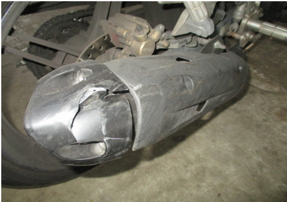
Photo 10 shows the exhaust muffler and exhaust muffler heat shield of the Motorcycle that had sustained damage as a result of the accident.
