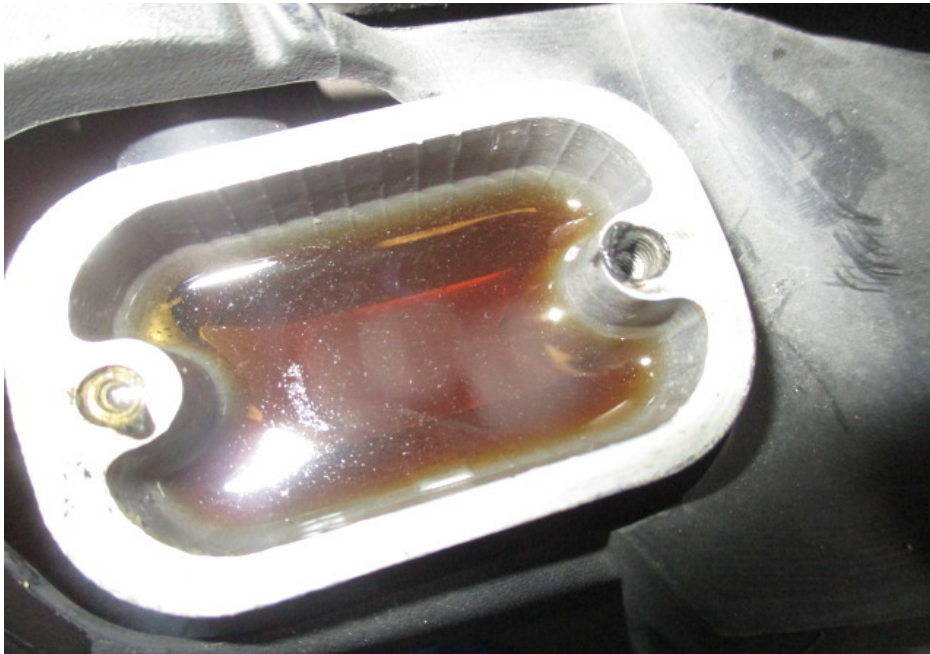
Photo 22 shows the brake fluid reservoir for the front brake of the Motorcycle. The brake fluid was observed to be of sufficient level and without contamination for operational purposes.
