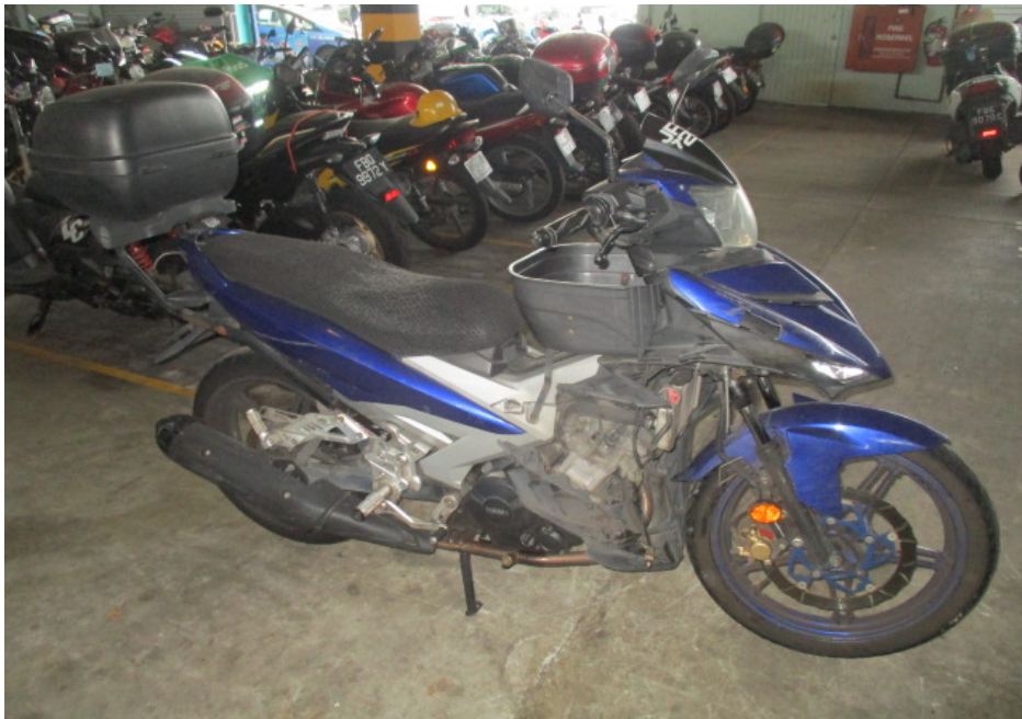
Photo 3 shows a general view of the right body of the Motorcycle at the time of our inspection. The Motorcycle was observed to have sustained damages along its frontal portion and right body. The body parts that were found to have been damaged include its front cowling, right cowling, front mudguard, right handlebar end, front brake lever, right side mirror, right front footrest, right rear side cover, exhaust muffler and top, amongst others.
