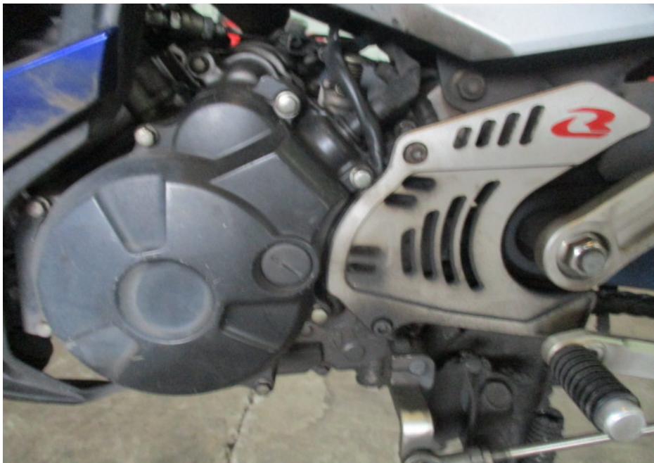
Photo 14 shows the left side of the engine of the Motorcycle at the time of our inspection. The various engine related parts and components were found to be intact with no visible damage. There was also no sign(s) or indication(s) of fluid leak observed around the left engine area of the Motorcycle.
