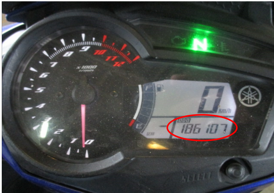
Photo 1 shows the speedometer gauge of the Motorcycle. The mileage of the Motorcycle at the time of our inspection was 186, 107km (circled).
