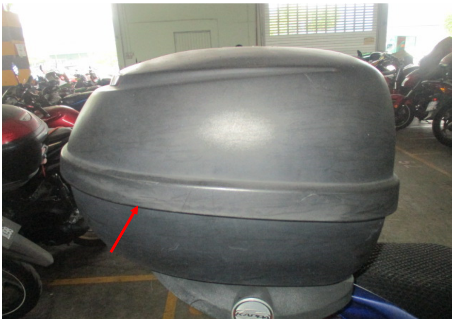
Photo 11 shows a closer view of the top box which was amongst the body parts of the Motorcycle that had sustained damages of grazing nature as a result of the accident (arrowed).
