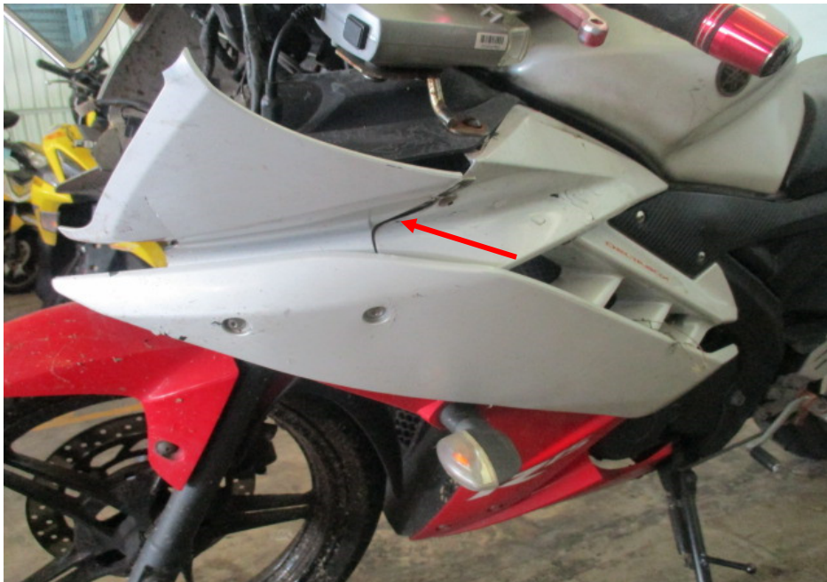
Photo 8 shows a closer view of the cracked left cowling of the Motorcycle as a result of the accident (arrowed).
