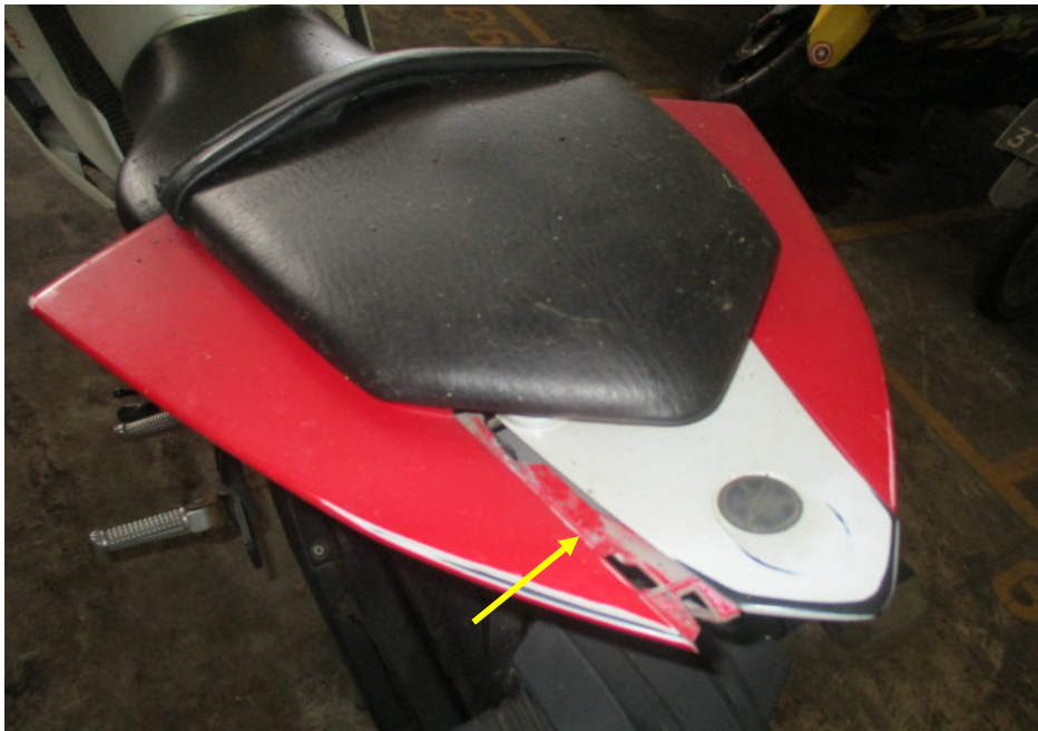
Photo 12 shows a closer view of the deformed left rear side cover which was amongst the body parts of the Motorcycle that had sustained damage as a result of the accident (arrowed).
