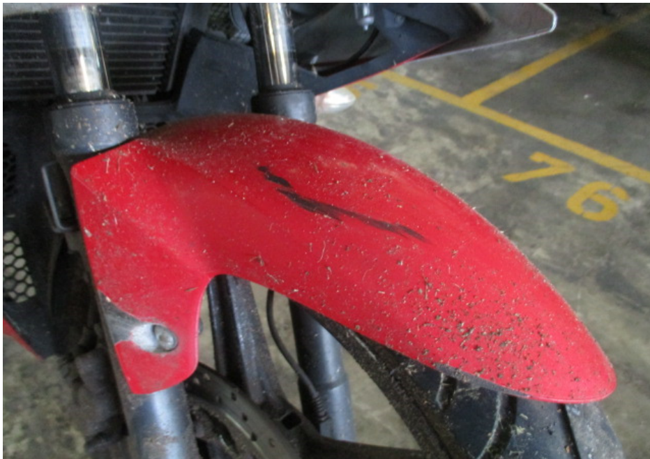
Photo 6 shows a close up view of the front mudguard cowling which was amongst the body parts of the Motorcycle that had sustained damage as a result of the accident.
