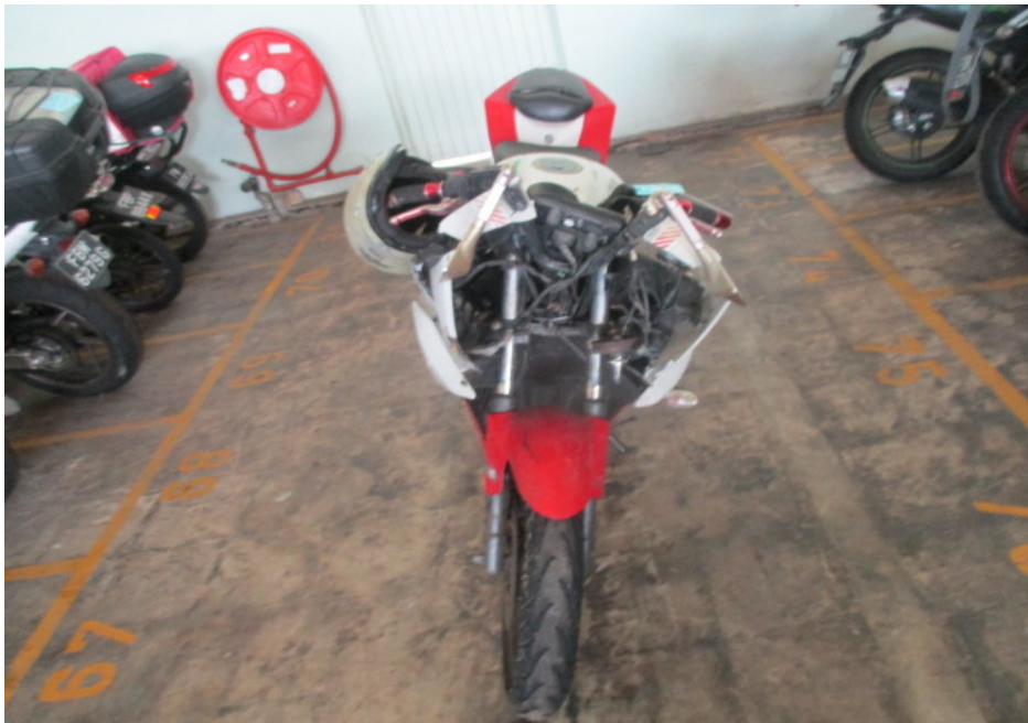
Photo 4 shows a general view of the frontal portion of the Motorcycle at the time of our inspection. The Motorcycle was observed to have sustained damages all around. Amongst the body parts that were found to have been damaged include its headlight assembly, head cowl, front mudguard, side cowlings, right handlebar end, right side mirror, front brake lever, rear brake pedal, right front footrest, rear side covers and exhaust muffler, amongst others.
