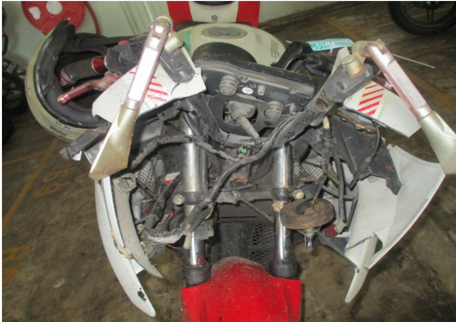
Photo 5 shows a closer view of the missing headlight assembly and head cowling which were amongst the body parts at the front body of the Motorcycle that had sustained damage as a result of the accident.
