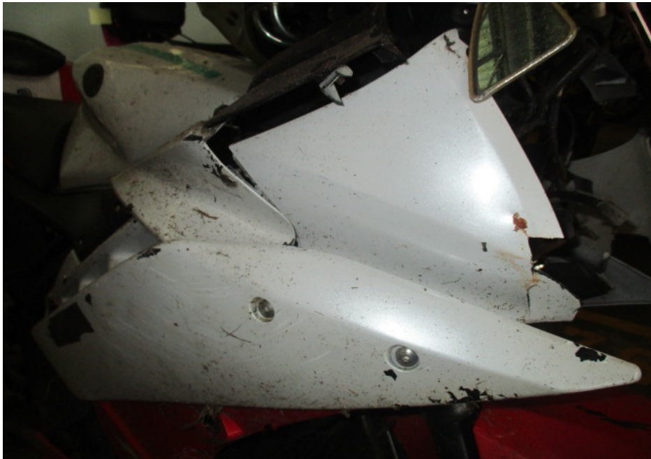
Photo 13 shows a closer view of the cracked right cowling of the Motorcycle as a result of the accident.
