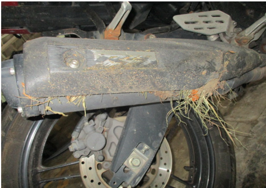
Photo 14 shows a closer view of the exhaust muffler of the Motorcycle that had sustained damages of grazing nature as a result of the accident.
