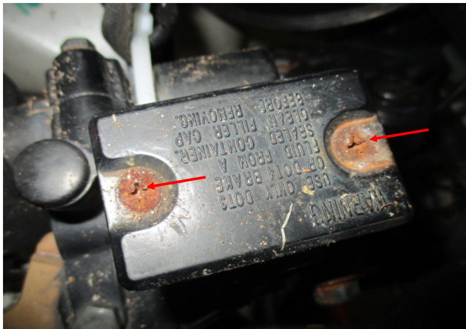
Photo 25 shows the brake fluid reservoir cover for the front brake of the Motorcycle. We were unable to examine whether the brake fluid was of sufficient level and without contamination for operational purposes due to the worn out screws (arrowed).
