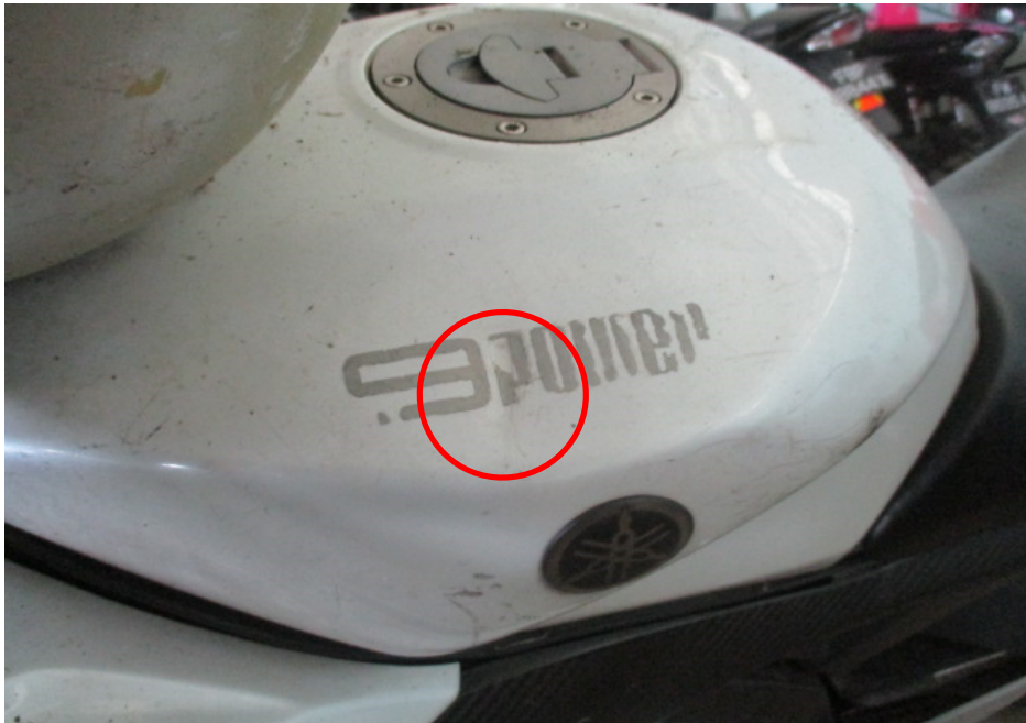
Photo 7 shows a closer view of the dented fuel tank (circled) which was amongst the body parts at the front body of the Motorcycle that had sustained damage as a result of the accident.
