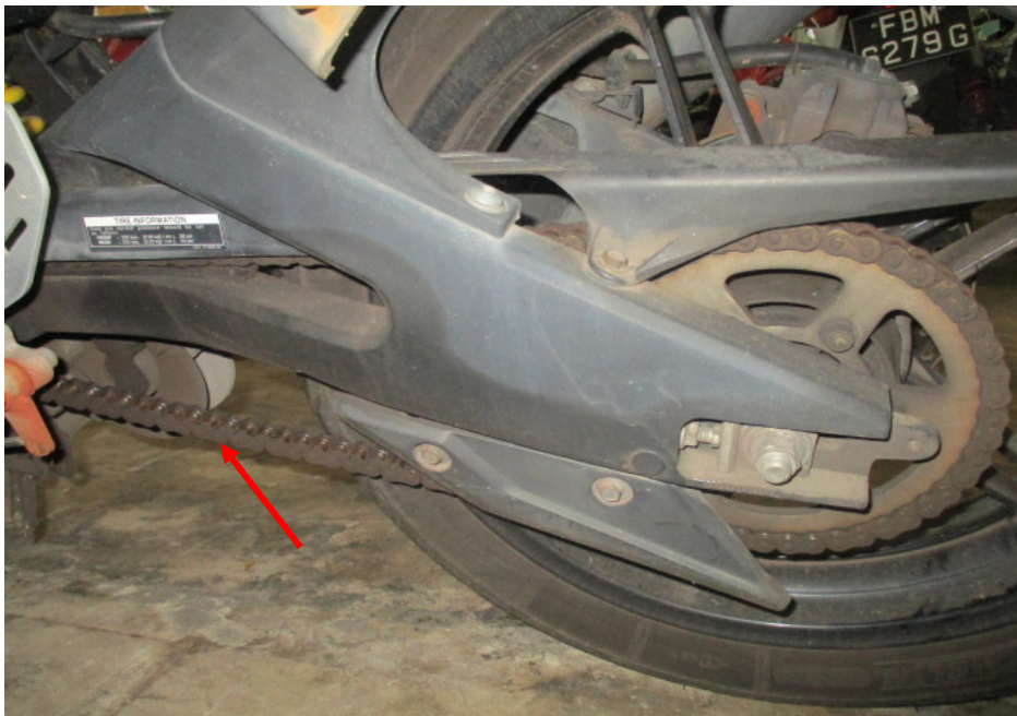
Photo 19 shows the general view of the gear train (arrowed) of the Motorcycle, which was observed to be intact with no misalignment. It was also adequately lubricated for operating purposes.
