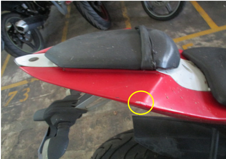
Photo 11 shows the right rear side cover of the Motorcycle which was amongst the body parts of the Motorcycle that had sustained damages of grazing nature as a result of the accident (circled).
