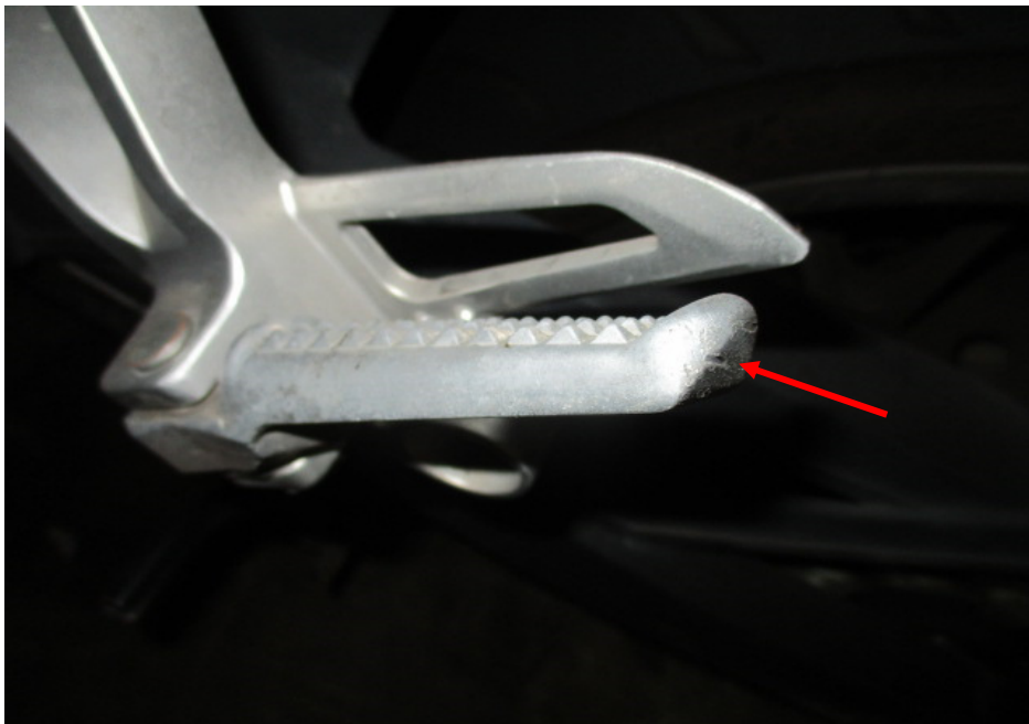
Photo 13 shows the left pillion foot peg which was amongst the body parts of the Motorcycle that had sustained damage as a result of the accident (arrowed).
