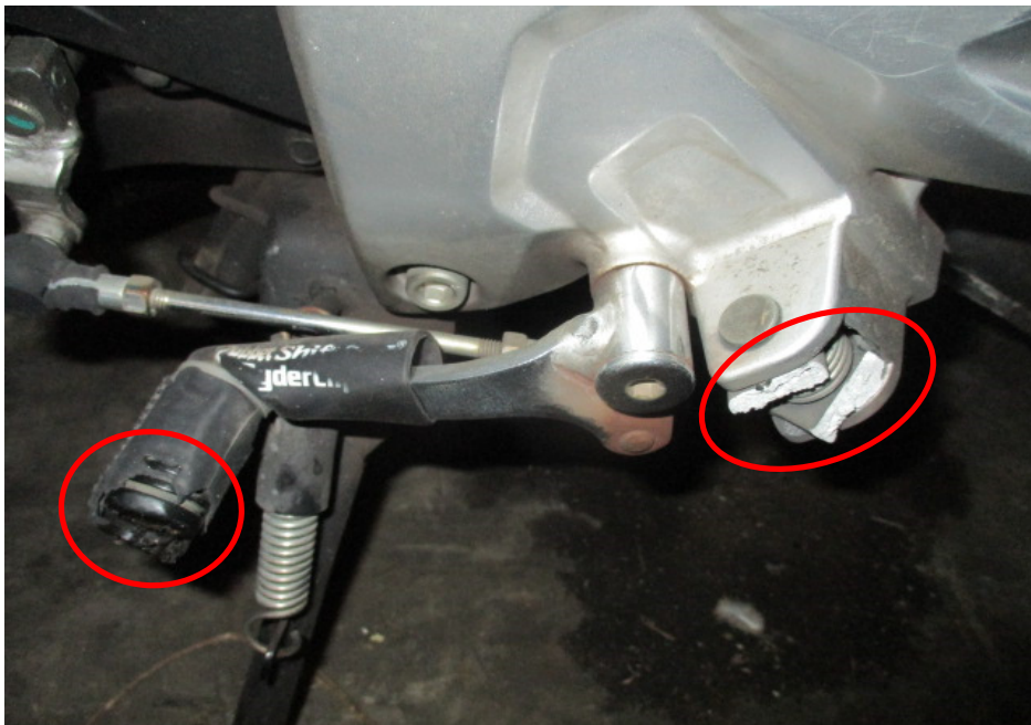
Photo 9 shows a closer view of the gear shift pedal and left front footrest (circled) which were amongst the body parts of the Motorcycle that had sustained damage as a result of the accident.
