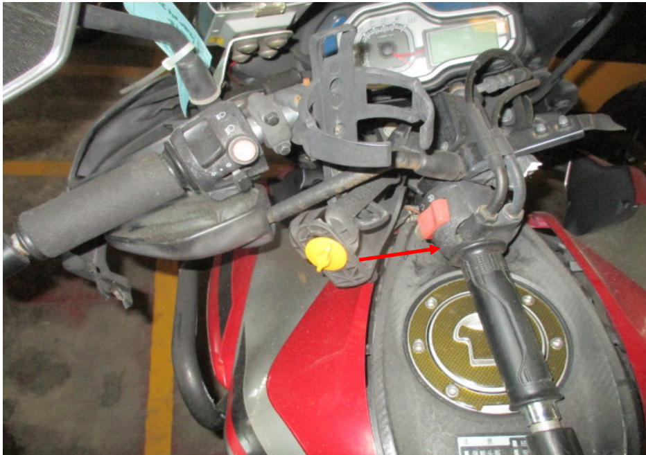
Photo 21 shows a close up view of the bent handlebar of the Motorcycle as a result of the accident (arrowed). We were hence not able to turn the handlebar of the Motorcycle towards the left or right.
