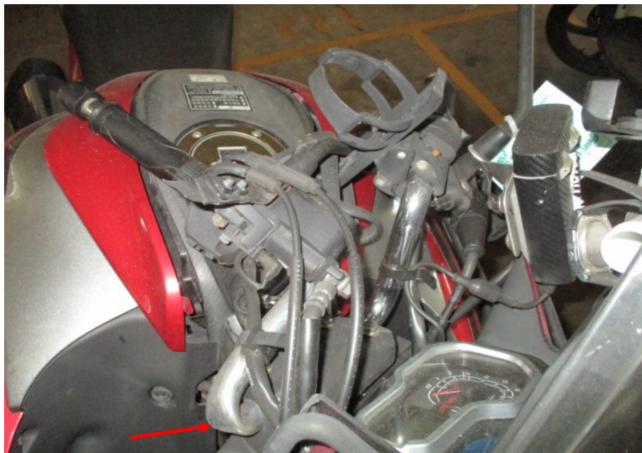
Photo 20 shows the bent handlebar of the Motorcycle as a result of the accident (arrowed). We were hence not able to turn the handlebar of the Motorcycle towards the left or right.
