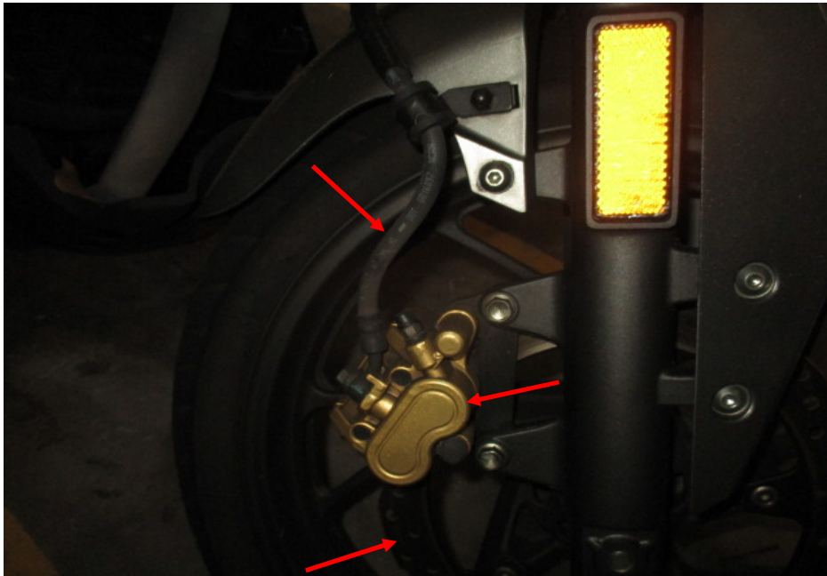
Photo 25 shows a close up view of the front brake caliper, front brake disc and front brake hose (arrowed) of the Motorcycle, which are all part of the components in the hydraulic front brake system of the Motorcycle. Our visual checks of these various components had revealed all to be intact with no visible damage.
