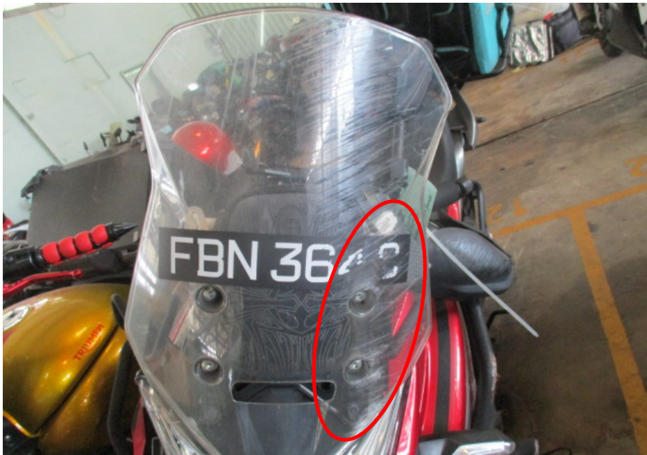
Photo 7 shows a closer view of the windshield (circled) which was amongst the body parts of the Motorcycle that had sustained damage as a result of the accident.
