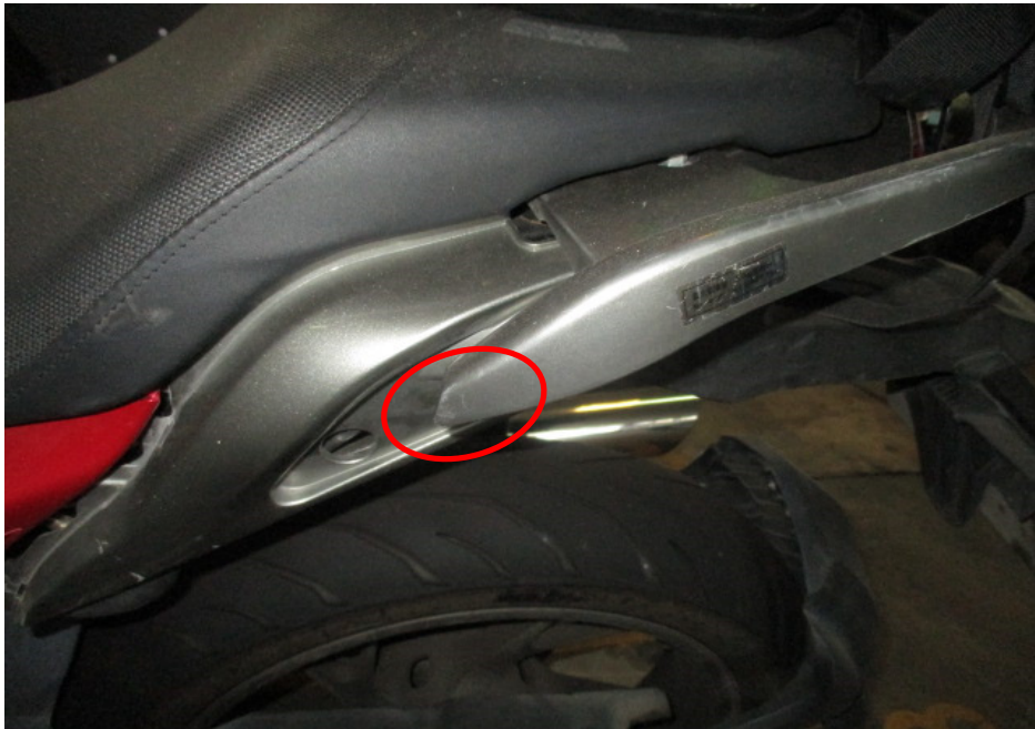
Photo 10 shows a closer view of left rear side cover which was amongst the body parts of the Motorcycle that had sustained damages of grazing nature as a result of the accident (circled).
