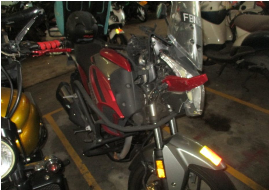
Photo 3 shows a general view of the right frontal portion of the Motorcycle at the time of our inspection. The Motorcycle was observed to have sustained damages along its frontal portion and left body.
