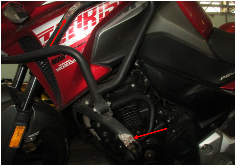
Photo 11 shows the left crash bars (arrowed) of the Motorcycle which sustained damages of grazing nature as a result of the accident.
