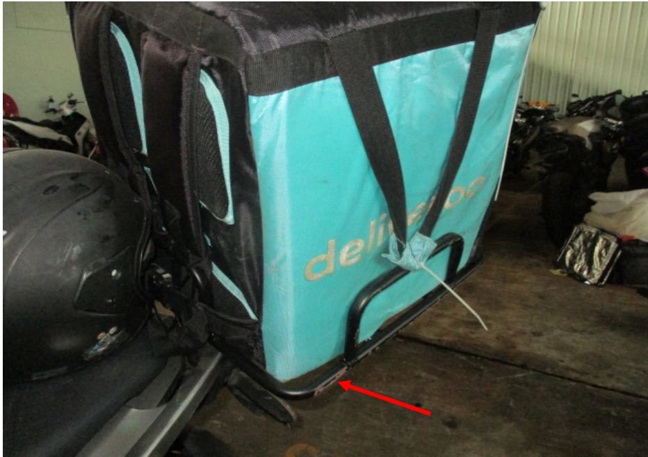
Photo 12 shows the top rack which was amongst the body parts of the Motorcycle that had sustained damage as a result of the accident (arrowed).
