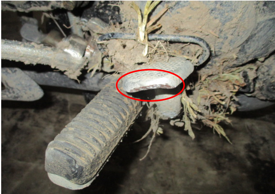
Photo 8 shows a closer view of the rear brake pedal (circled) which was amongst the body parts of the Motorcycle that had sustained damage as a result of the accident.
