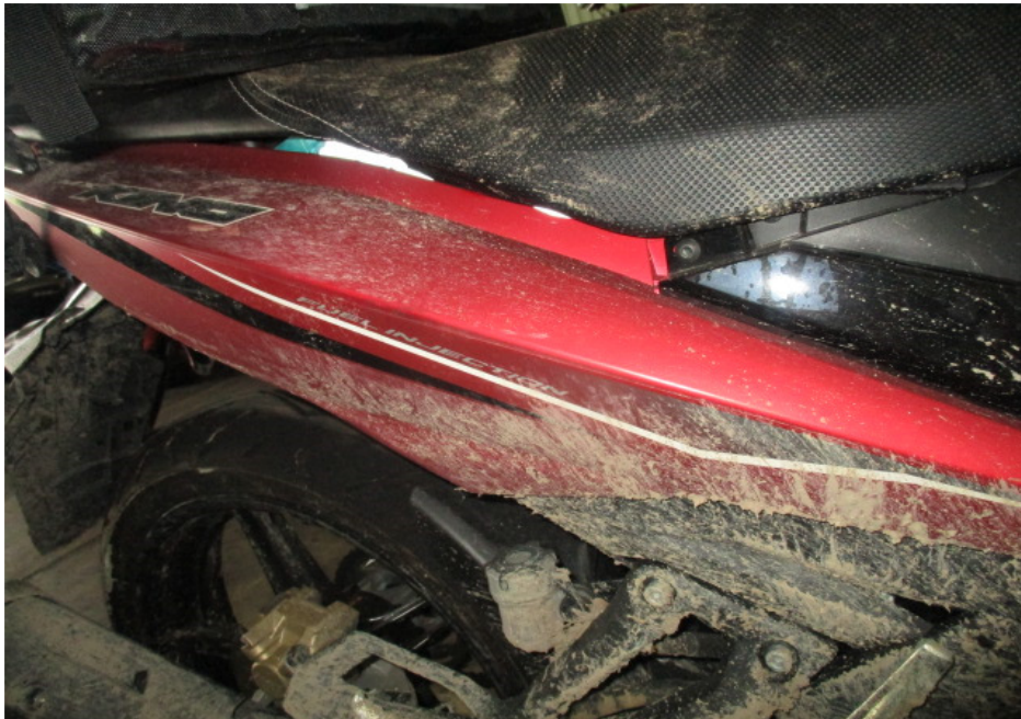
Photo 9 shows a closer view of right rear side cover which was amongst the body parts of the Motorcycle that had sustained damages of grazing nature as a result of the accident.
