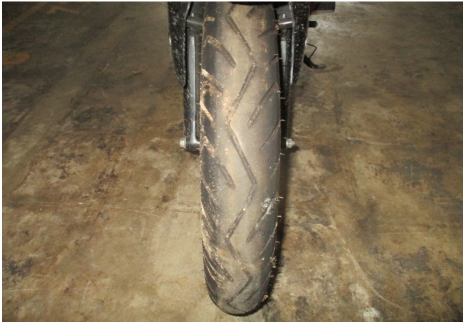
Photo 12 shows the front tyre of the Motorcycle at the time of our inspection. The front tyre was observed to be in serviceable condition with remaining tread depth of approximately 3mm. The pattern of the tread was also clearly visible. There was no tear, burst mark(s) and/or punctured hole(s) on the sidewalls as well as across the tread of the front tyre.
