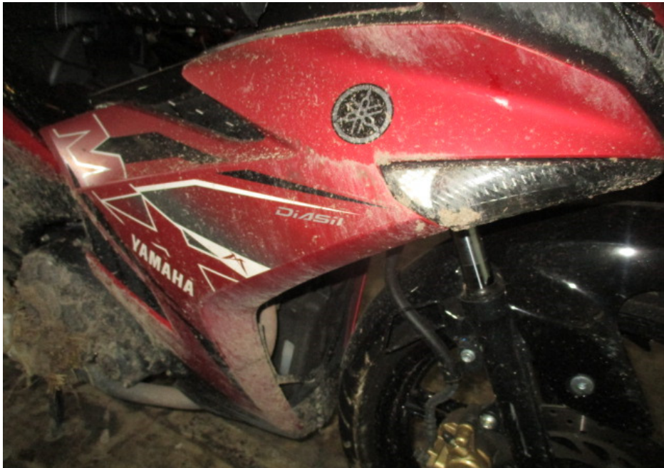
Photo 6 shows a closer view of the right cowling which was amongst the body parts of the Motorcycle that had sustained damage as a result of the accident.
