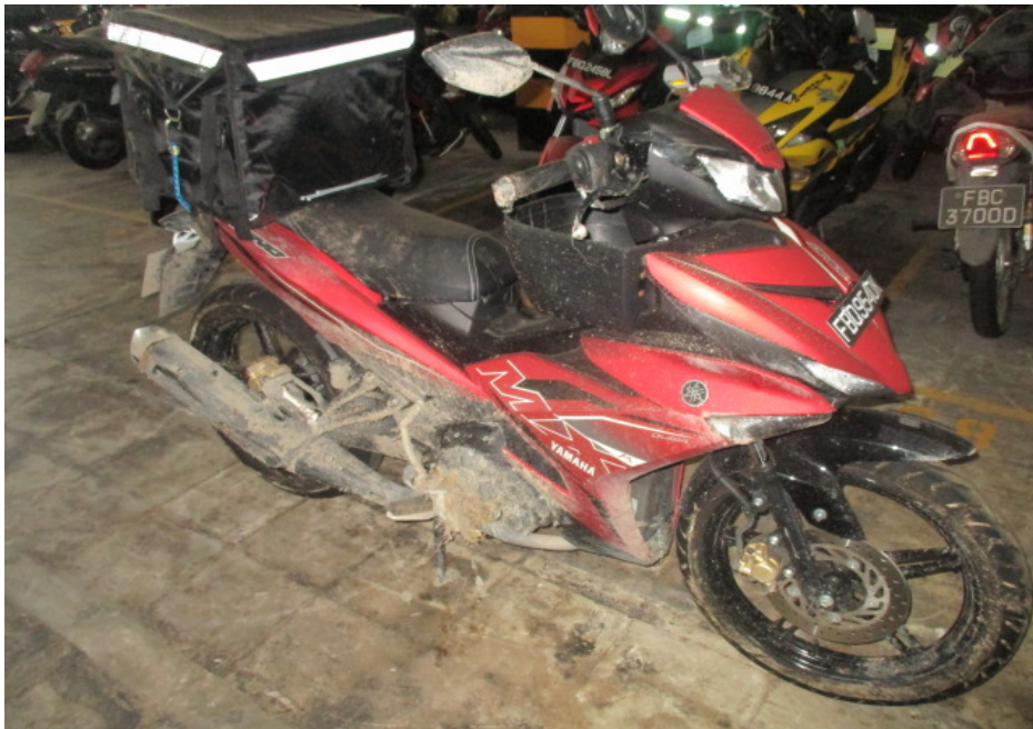
Photo 3 shows a general view of the right body of the Motorcycle at the time of our inspection. The Motorcycle was observed to have sustained damages along its frontal portion, right body and rear portion. The body parts that were found to have been damaged include its head cowl, right cowl, front mudguard, right handlebar end, front brake lever, right side mirror, rear brake pedal, right rear side cover, exhaust muffler and left rear signal lamp, amongst others.
