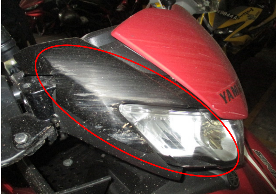
Photo 4 shows a close up view of the head cowling (circled) which was amongst the body parts of the Motorcycle that had sustained damage as a result of the accident.
