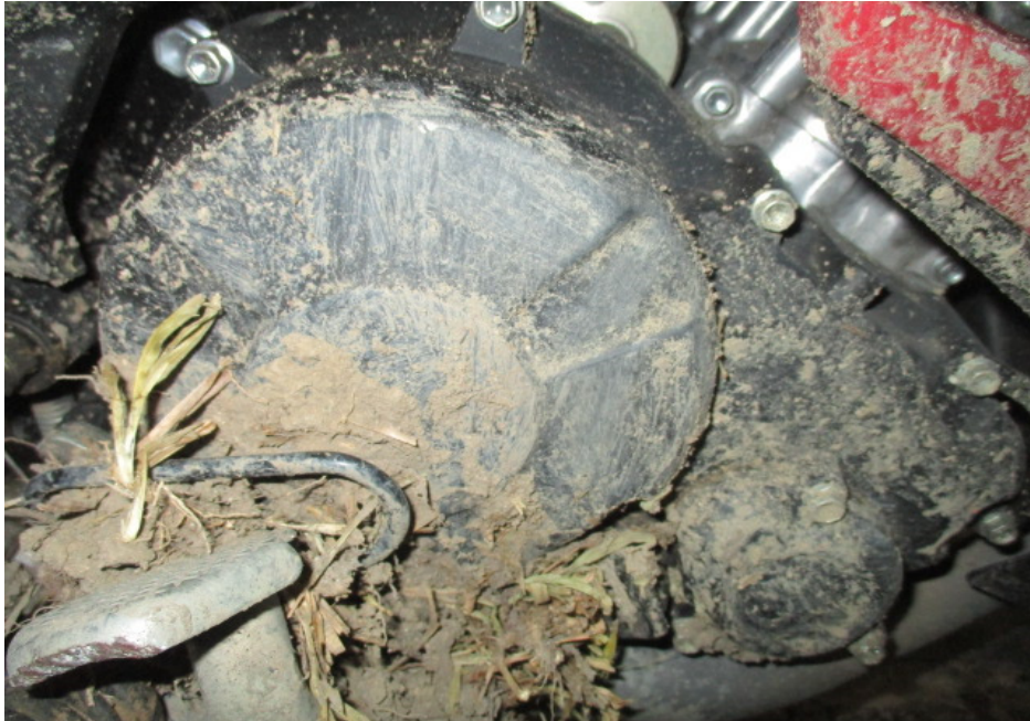
Photo 15 shows the right side of the engine of the Motorcycle at the time of our inspection. The various right engine components had sustained damage of grazing nature as a result of the accident however the engine components were still intact. There was also no fluid leak and/or fluid stain found around the right engine area of the Motorcycle.
