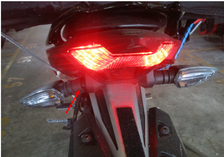
Photo 11 shows the deformed left rear signal lamp of the Motorcycle as a result of the accident (arrowed).
