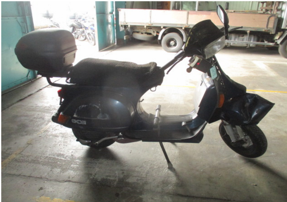
Photo 3 shows a general view of the right body of the Motorcycle at the time of our inspection. The Motorcycle was observed to have sustained damages along its frontal portion and right body.
