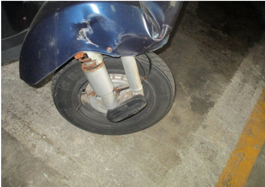
Photo 10 shows the front wheel rim and front tyre of the Motorcycle at the time of our inspection. The front tyre was observed to be in serviceable condition with remaining tread depth of approximately 3mm. The tyre was also observed to be sufficiently inflated for vehicular operation. There was no significant damage observed on the front wheel rim.
