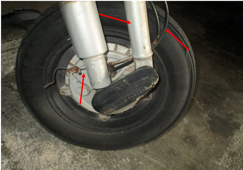
Photo 18 shows a close up view of the front fork, front brake cable and spring of the Motorcycle (arrowed), which are all part of the components in the mechanical front brake system of the Motorcycle. Our visual checks of these various components had revealed all to be intact with no visible damage.
