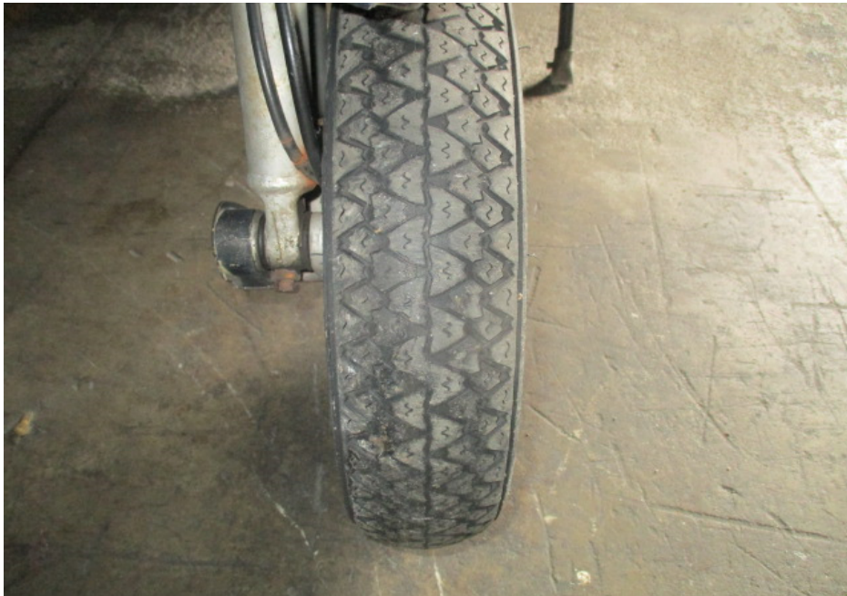
Photo 11 shows the front tyre of the Motorcycle at the time of our inspection. The front tyre was observed to be in serviceable condition. The pattern of the tread was also clearly visible. There was no tear, burst mark(s) and/or punctured hole(s) on the sidewalls as well as across the tread of the front tyre.
