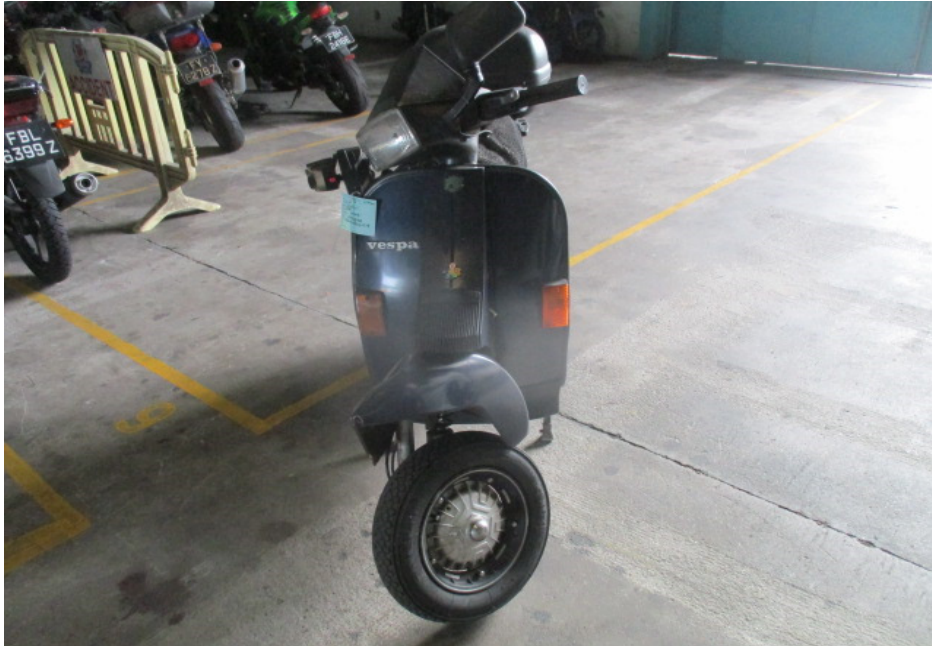
Photo 17 shows the front wheel of the Motorcycle turned towards its full right. Turning the Motorcycle's handle bar towards the left and right did not produce any abnormal free play and/or resistance. This would indicate that the steering system of the Motorcycle was in serviceable condition at the time of our inspection.
