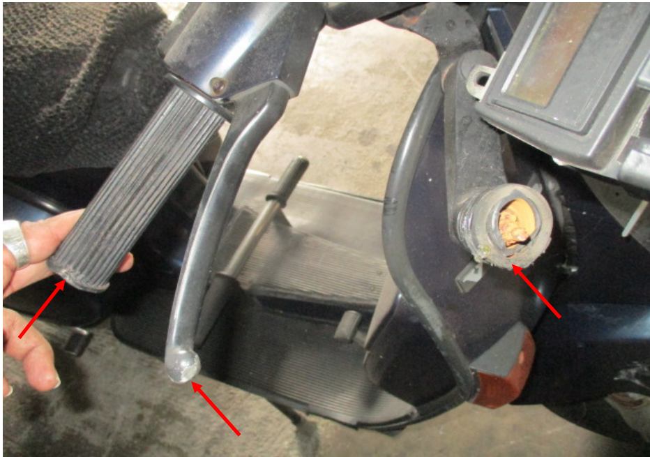
Photo 8 shows a close up view of the right handlebar grip, front brake lever and broken right side mirror of the Motorcycle which had sustained damage as a result of the accident (arrowed).
