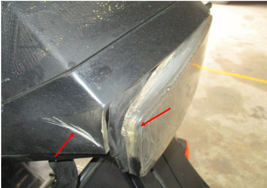
Photo 6 shows a close up view of the headlamp assembly of the Motorcycle at the time of our inspection. Amongst the body parts damaged were its headlight assembly and headlight (arrowed).
