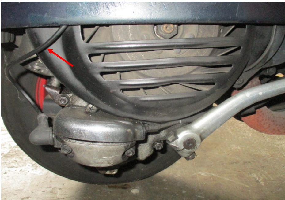
Photo 14 shows the general view of the drive train of the Motorcycle, which was observed to be intact with no misalignment. There was also no visible tear or cut observed on the connecting hoses and cables (arrowed).
