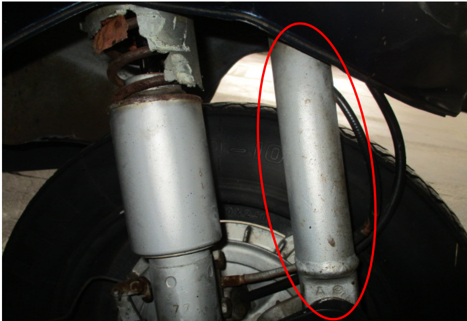
Photo 15 shows the front fork (circled) of the Motorcycle. The front fork of the Motorcycle was both found to be intact and undamaged. Turning the Motorcycle's handle bar towards the left and right did not produce any abnormal free play and/or resistance. The steering system of the Motorcycle was in serviceable condition at the time of our inspection.
