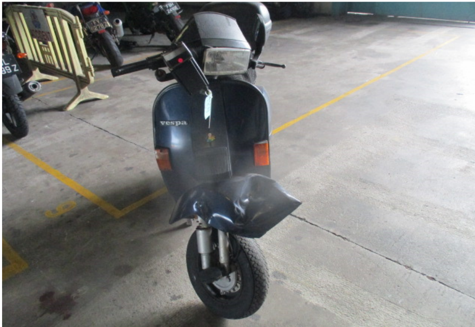
Photo 16 shows the front wheel of the Motorcycle turned towards its full left. Turning the Motorcycle's handle bar towards the left and right did not produce any abnormal free play and/or resistance. This would indicate that the steering system of the Motorcycle was in serviceable condition at the time of our inspection.
