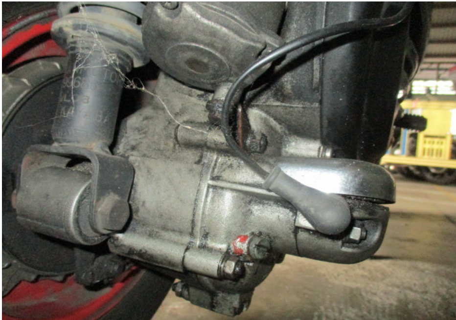
Photo 13 shows the bottom of the Motorcycle's engine area where upon closer examination, we had observed that the various engine related parts and components were intact with no visible damage. There was also no sign(s) or indication(s) of fluid leak observed around the engine area of the Motorcycle.
