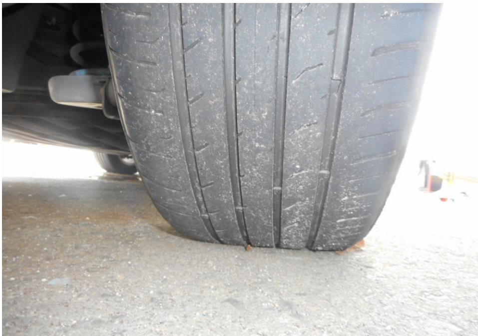
Photo 10 shows the condition of the rear right tyre of the Motor Car, which was observed to be in serviceable condition with remaining tread depth of approximately 4.2mm. The tyre was also observed to be sufficiently inflated for vehicular operation with no tear, cut or burst mark(s).
