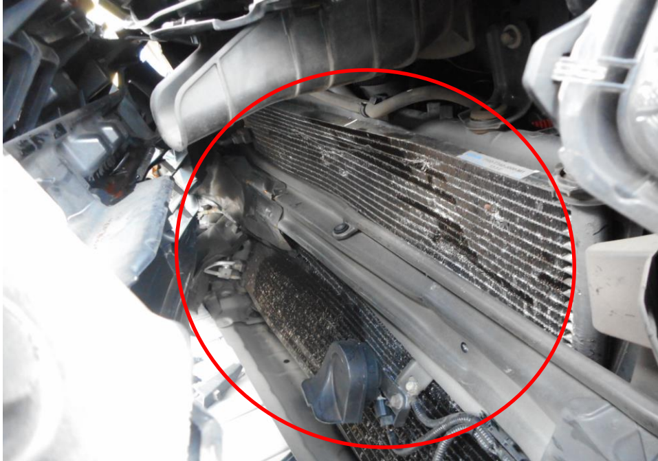
Photo 5 shows a close up view of the Motor Car's engine compartment at the time of my inspection. The Motor car was observed to have sustained damage at its front portion. Its front engine radiator (red circle) was amongst the body parts and various components in the engine compartments were also damaged as a result of the accident.
