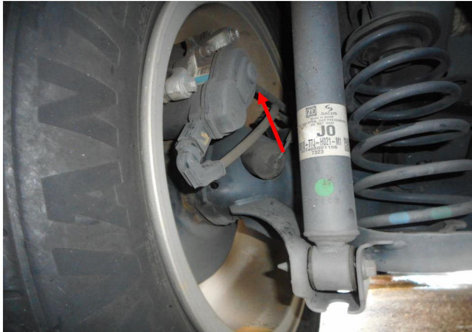
Photo 19 shows the brake hose/pipe (arrowed) at the rear left wheel of the Motor Car. No leakage of brake fluid was observed. Visual examination of the various components of the braking system like the drum brake, brake booster, brake pedal etc. had revealed all to be intact and without visible damage.
