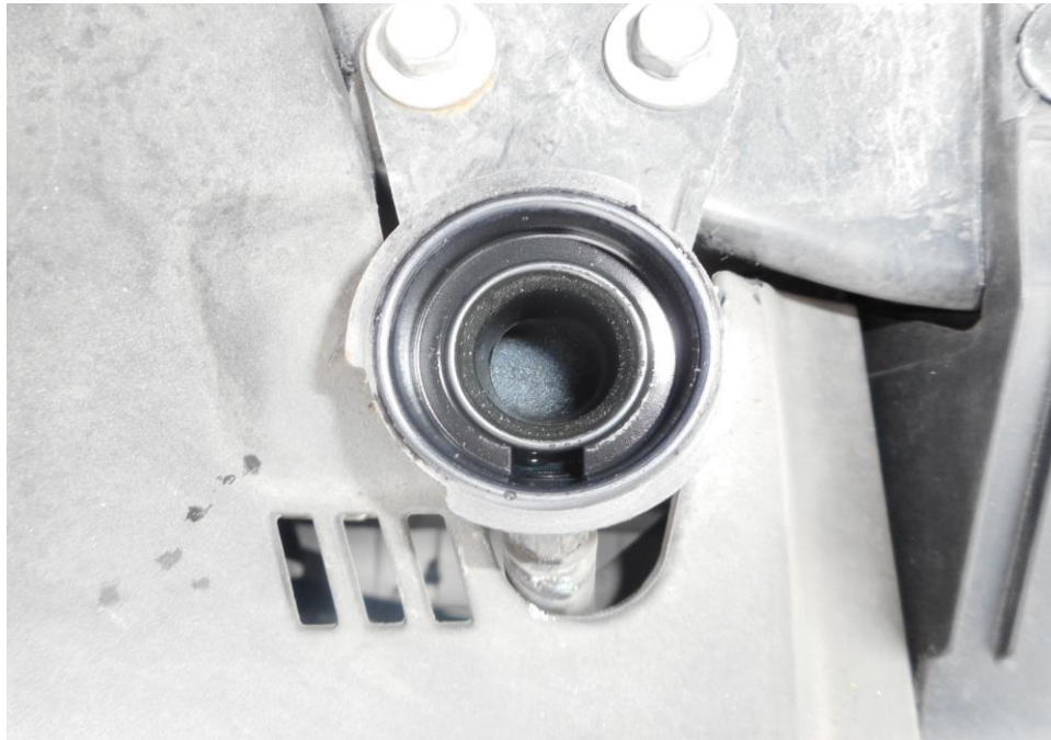
Photo 16 shows the engine coolant reservoir of the Motor Car at the time of my inspection. The engine coolant was observed to be of insufficient level due to the damaged to the radiator that cause all the coolant to depleted from the coolant reservoir.
