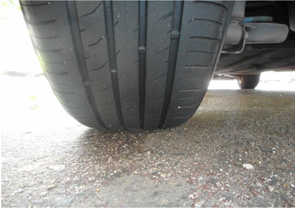
Photo 11 shows the condition of the rear left tyre of the Motor Car, which was observed to be in serviceable condition with remaining tread depth of approximately 4.5mm. The tyre was also observed to be sufficiently inflated for vehicular operation with no tear, cut or burst mark(s).
