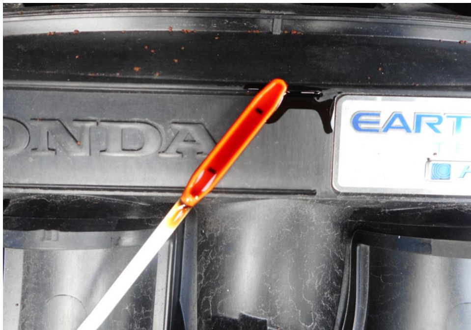
Photo 17 shows the engine oil dip stick of the Motor Car at the time of my inspection. The engine oil was observed to be of sufficient level and without any visible contamination.
