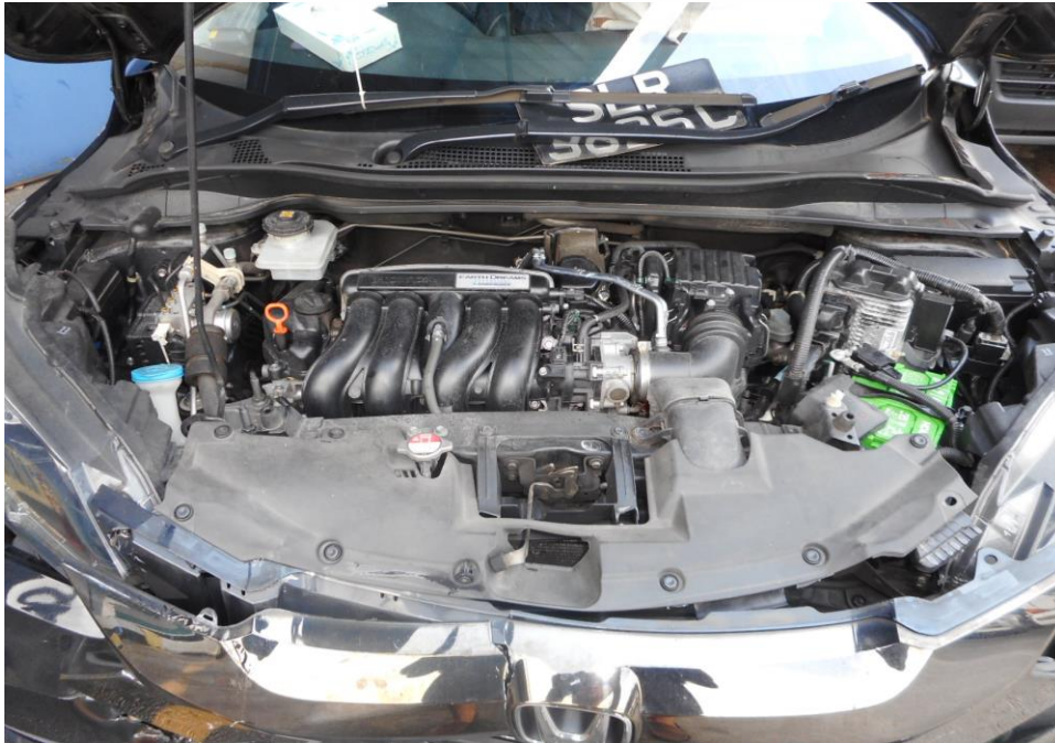
Photo 14 shows a general view of the Motor Car's engine compartment, which was accessed by lifting the front cabin of the Motor Car. The various parts and components inside the engine compartment were unaffected by the accident. There was also no sign(s) or indication(s) of fresh fluid leakage and/or fluid stain within the engine compartment
