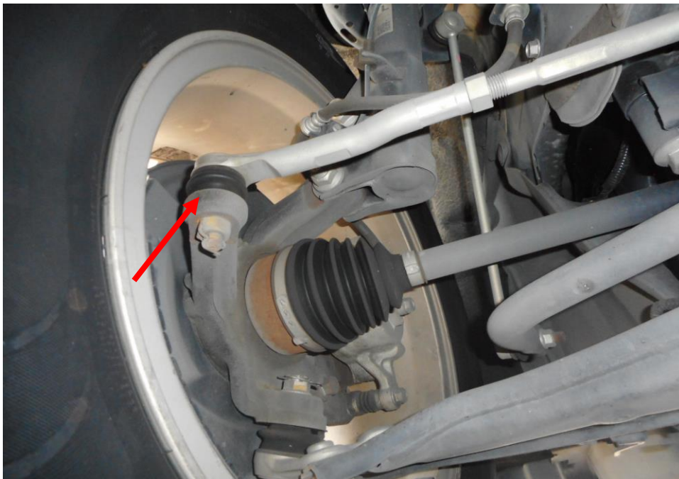
Photo 24 shows the various undercarriage components at the front left wheel of the Motor Car, in particular the steering tie rod end (arrowed). The various Undercarriage components of the Motor Car were all found to be intact without any visible damage. There was also no sign of fluid stain(s) observed on the various undercarriage components.
