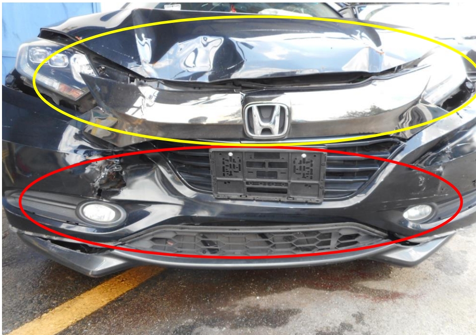
Photo 4 shows the close up view of the Motor Car's front body at the time of my inspection. The Motor car was observed to have sustained damage at its front portion. Its front bonnet (yellow circle) and front bumper (red circle) was amongst the body parts and various components in the engine compartments were also damaged as a result of the accident.
