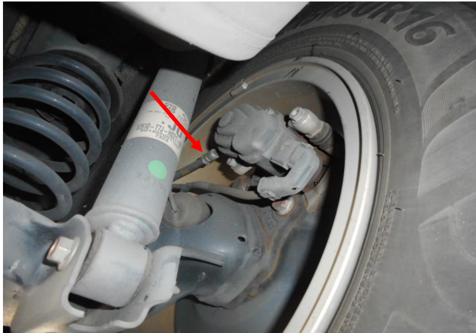
Photo 20 shows the brake hose/pipe (arrowed) at the rear right wheel of the Motor Car. No leakage of brake fluid was observed. Visual examination of the various components of the braking system like the drum brake, brake booster, brake pedal etc. had revealed all to be intact and without visible damage.
