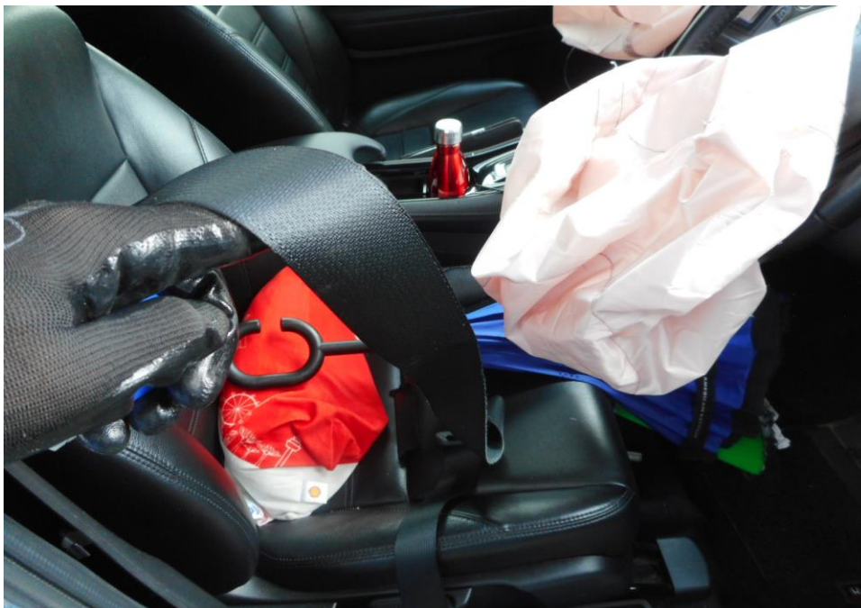
Photo 25 shows that the seat belt on the right seat was worn at the material time of accident as the safety pre-tensioners was activated at the moment of impact and caused the seat belt to be locked into the last position.
