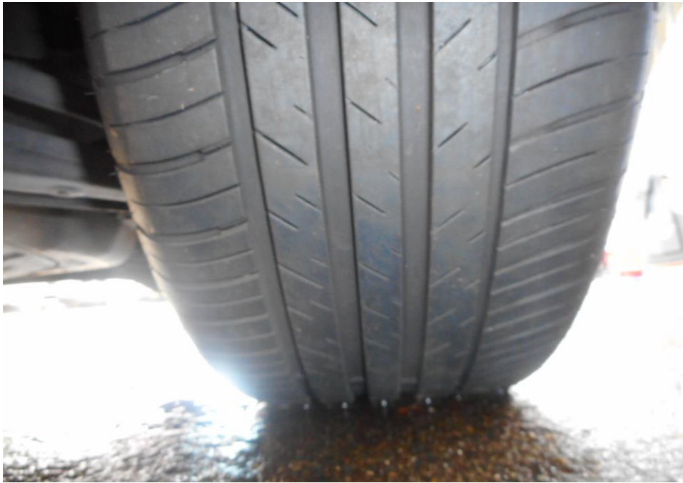
Photo 9 shows the condition of the front right tyre of the Motor Car, which was observed to be in serviceable condition with remaining tread depth of approximately 5.2mm. The tyre, which was wrapped around alloy wheel rim, was also observed to be sufficiently inflated for vehicular operation.
