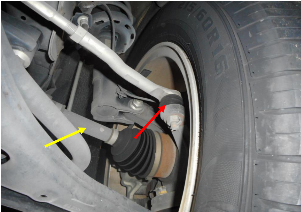
Photo 23 shows the various undercarriage components at the front right wheel of the Motor Car, in particular the steering tie rod end (arrowed) and drive shaft (yellow arrow). The various steering components were all found to be intact, suggesting that the steering system of the Motor Car was likely to be in serviceable condition at the material time of accident. There was also no sign of fluid stain(s) observed on the various undercarriage components.
