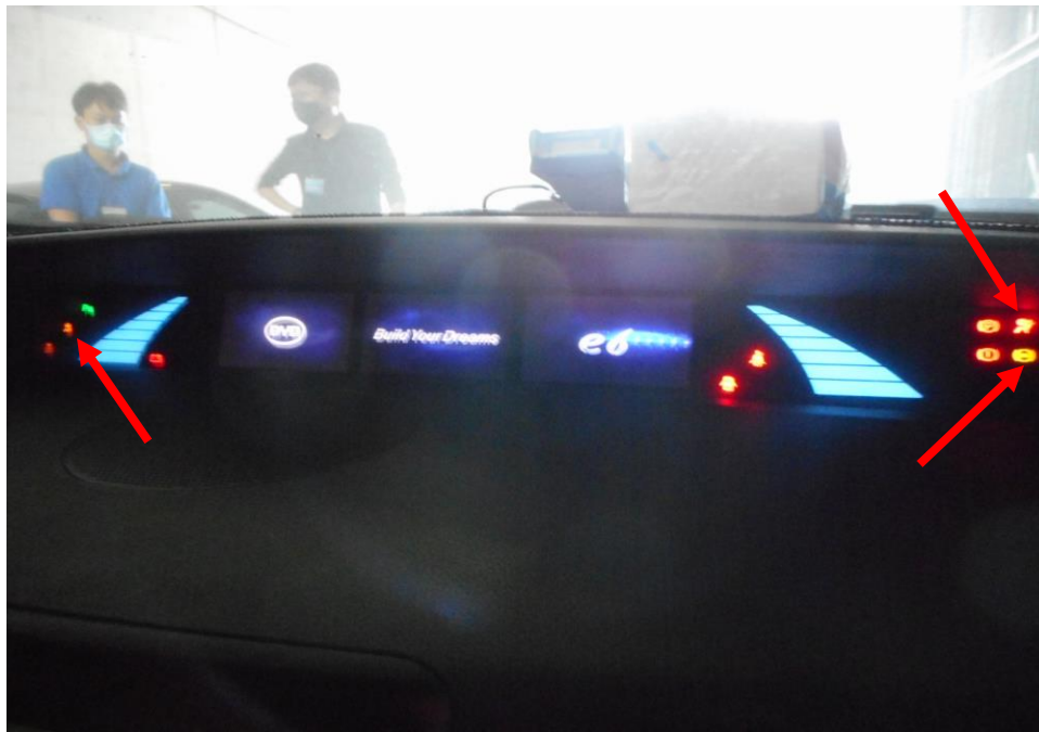
Photo 22 shows the warning light for Anti-Lock Brake System (ABS), Supplemental Restraint System (SRS) and Traction Control System (TC) appearing on the instrument panel of the Motor Taxi during the self-test of its various electronic operating systems when its engine was cranked.
