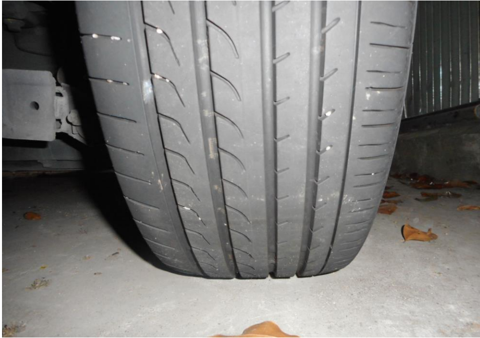
Photo 8 shows the condition of the rear right tyre of the Motor Taxi, which was observed to be in serviceable condition with remaining tread depth of approximately 6.1mm. The tyre, which was wrapped around standard alloy wheel rim, was also observed to be sufficiently inflated for vehicular operation.
