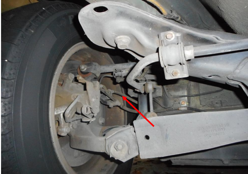
Photo 18 shows the brake pipe (arrowed) at the rear left wheel of the Motor Taxi. I did not observe any leakage of brake fluid at the time of my inspection of the Motor Taxi. My static tests of the Motor Taxi's braking system, along with my visual examination of the various mechanical components in the braking system had indicated that there was no internal leakage of pressure/vacuum. Hence the braking system of the Motor Taxi was likely to be in serviceable condition at the material time of accident.
