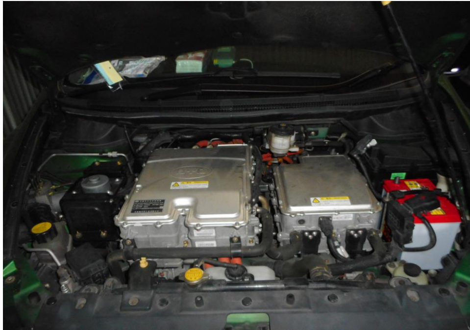
Photo 11 shows a general view of the Motor Taxi's engine compartment, which was accessed by lifting the front cabin of the Motor Taxi. The various parts and components inside the engine compartment were unaffected by the accident. There was also no sign(s) or indication(s) of fresh fluid leakage and/or fluid stain within the engine compartment
