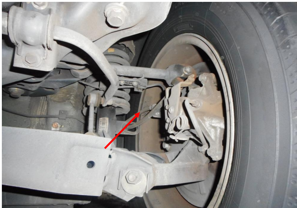
Photo 17 shows the brake pipe (arrowed) at the rear right wheel of the Motor Taxi. I did not observe any leakage of brake fluid at the time of my inspection of the Motor Taxi. My static tests of the Motor Taxi's braking system, along with my visual examination of the various mechanical components in the braking system, had indicated that there was no internal leakage of pressure/vacuum. Hence the braking system of the Motor Taxi was likely to be in serviceable condition at the material time of accident.
