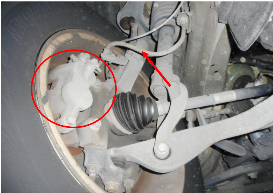
Photo 19 shows the brake hose/pipe (arrowed) at the front right wheel of the Motor Taxi. No leakage of brake fluid was observed. Visual examination of the various components of the braking system like the brake caliper (circled), brake booster, brake pedal etc had revealed all to be intact and without visible damage at the time of accident. There was also no sign of fluid stain(s) observed on the various undercarriage components.
