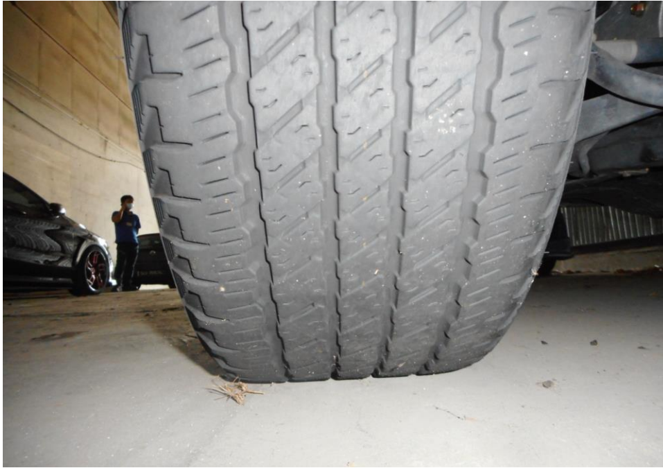
Photo 10 shows the condition of the rear right tyres of the Motor Taxi, which were observed to be in serviceable condition with remaining, tread depth of approximately 5.1mm. There was also no tear, cut or burst mark(s) on the outer and the inner sidewalls as well as across the tread of the 4 tyres that were fitted on the Motor Taxi.
