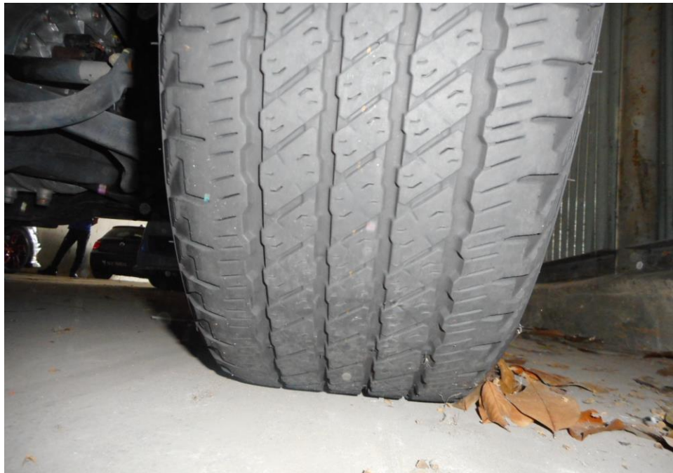
Photo 7 shows the condition of the front right tyre of the Motor Taxi, which was observed to be in serviceable condition with remaining tread depth of approximately 5mm. The tyre, which was wrapped around standard alloy wheel rim, was also observed to be sufficiently inflated for vehicular operation. There was no tear, cut or burst mark(s) on the outer and the inner sidewalls as well as across the tread of the 4 tyres that were fitted on the Motor Taxi.
