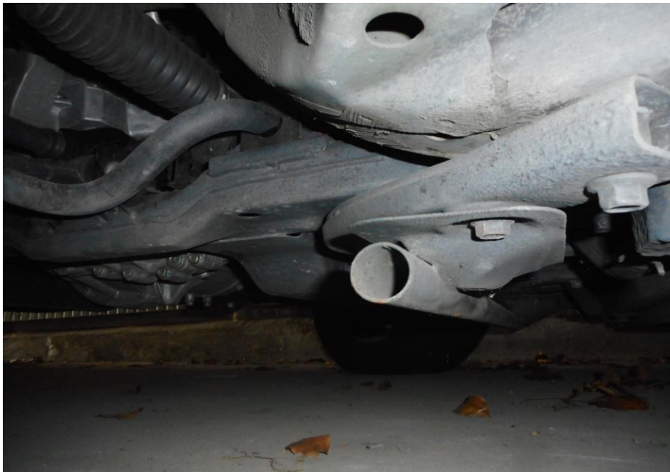
Photo 14 shows the undercarriage of the Motor Taxi, at the area where the engine housing and transmission housing are located. . I did not find any sign(s) or indication(s) of fluid leak and/or fluid stain(s) on the underside of the Motor Taxi.
