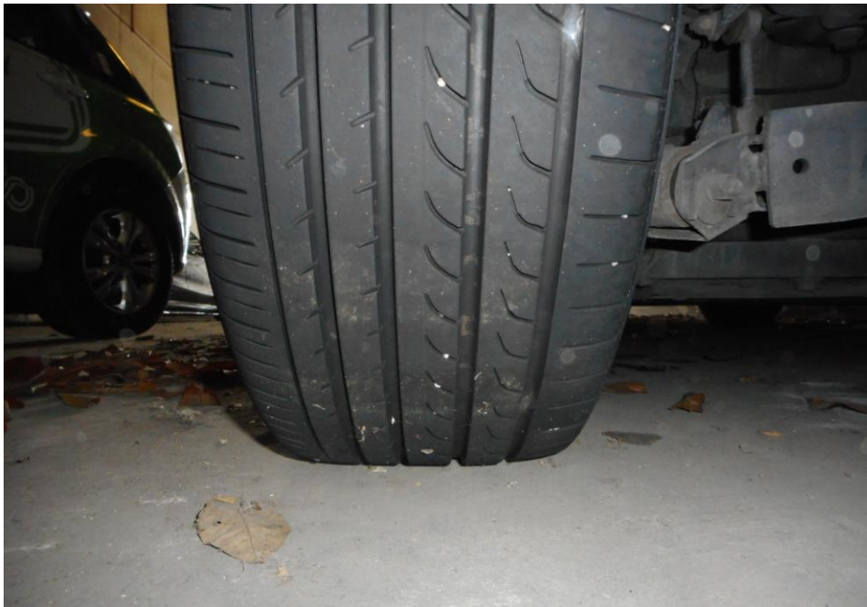
Photo 9 shows the condition of the rear left tyres of the Motor Taxi, which was observed to be in serviceable condition with remaining tread depth of approximately 6mm. The tyres, which were wrapped around standard alloy wheel rim, were also observed to be sufficiently inflated for vehicular operation. There was also no damage found on all 4 alloy wheel rims of the Motor Taxi.
