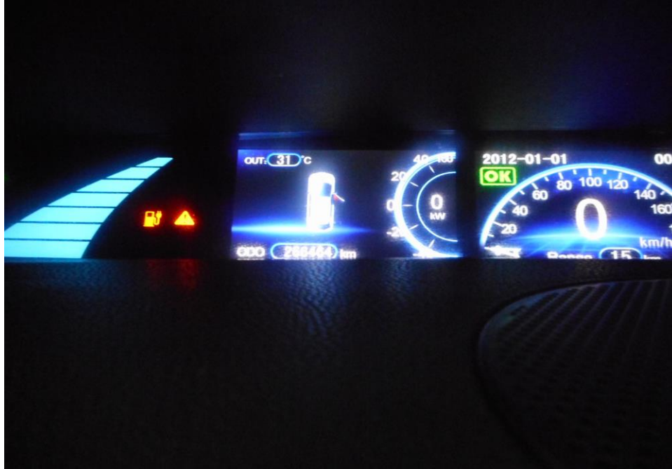
Photo 23 shows no warning lights illuminated on the instrument panel of the Motor Taxi after the engine was cranked. This would suggest that there was no abnormality to the various electronic operating systems of the Motor Taxi, like the ABS, SRS and TC.
