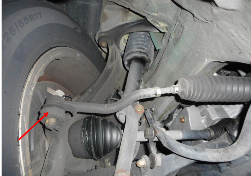
Photo 16 shows the various undercarriage components at the front left wheel of the Motor Taxi, in particular the steering tie rod end (arrowed). The various Undercarriage components of the Motor Taxi were all found to be intact without any visible damage. There was also no sign of fluid stain(s) observed on the various undercarriage components.
