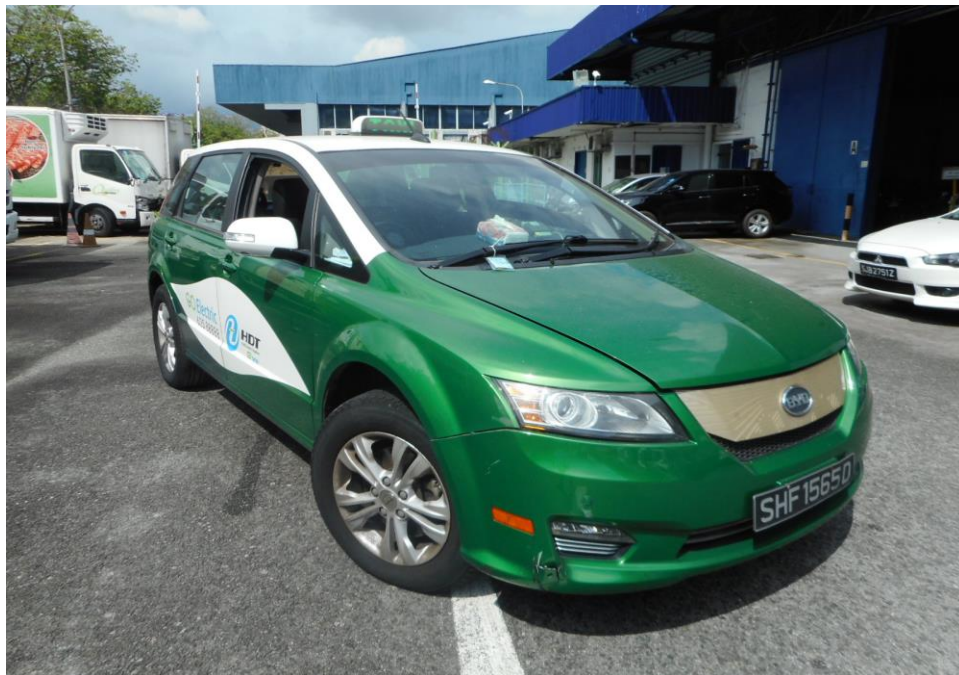
Photo 21 shows the front right wheel of the Motor Taxi turned to its full left. During my steering system test, I did not experience any abnormal free play and/or resistance when I had turned the steering wheel towards full left and full right. This would suggest that the steering system of the Motor Taxi was likely to be in serviceable condition at the material time of accident.
