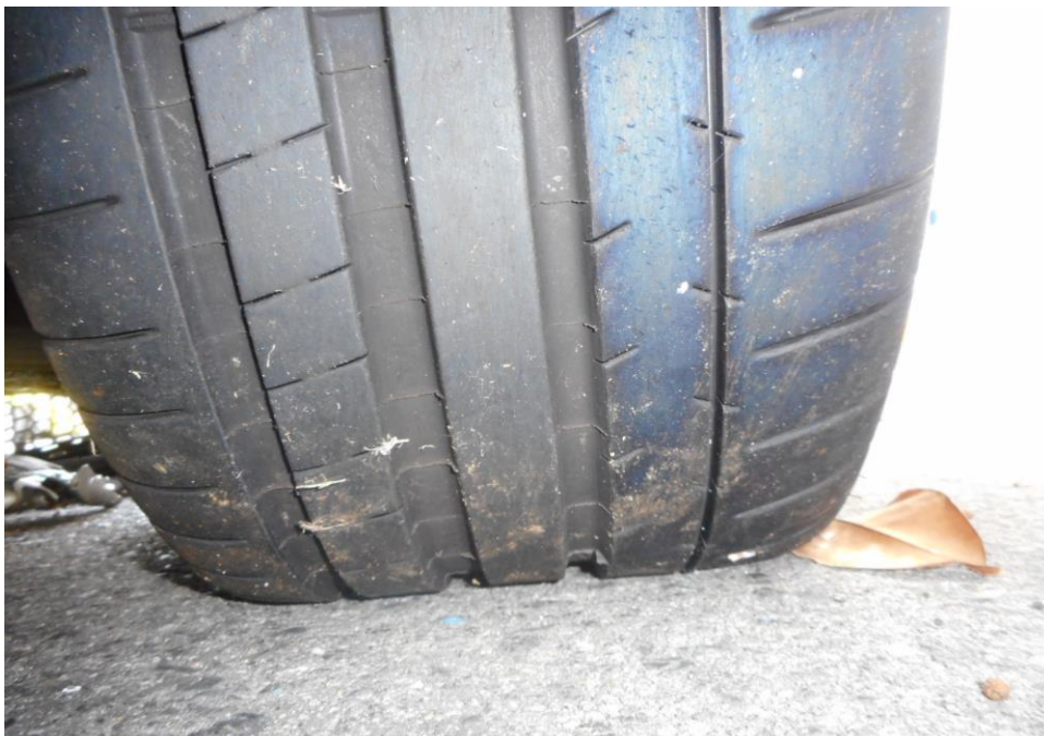
Photo 12 shows the condition of the front right tyre of the Motor Car, which was observed to be in serviceable condition with remaining tread depth of approximately 6.2mm. The tyre, which was wrapped around alloy wheel rim, was also observed to be sufficiently inflated for vehicular operation.
