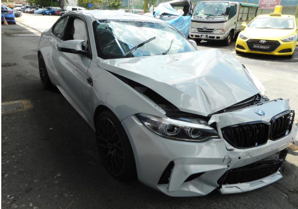
Photo 9 shows a general view of the Motor Car's right body at the time of my inspection. The right portion of the Motor Car was observed to have been undamaged by the accident.
