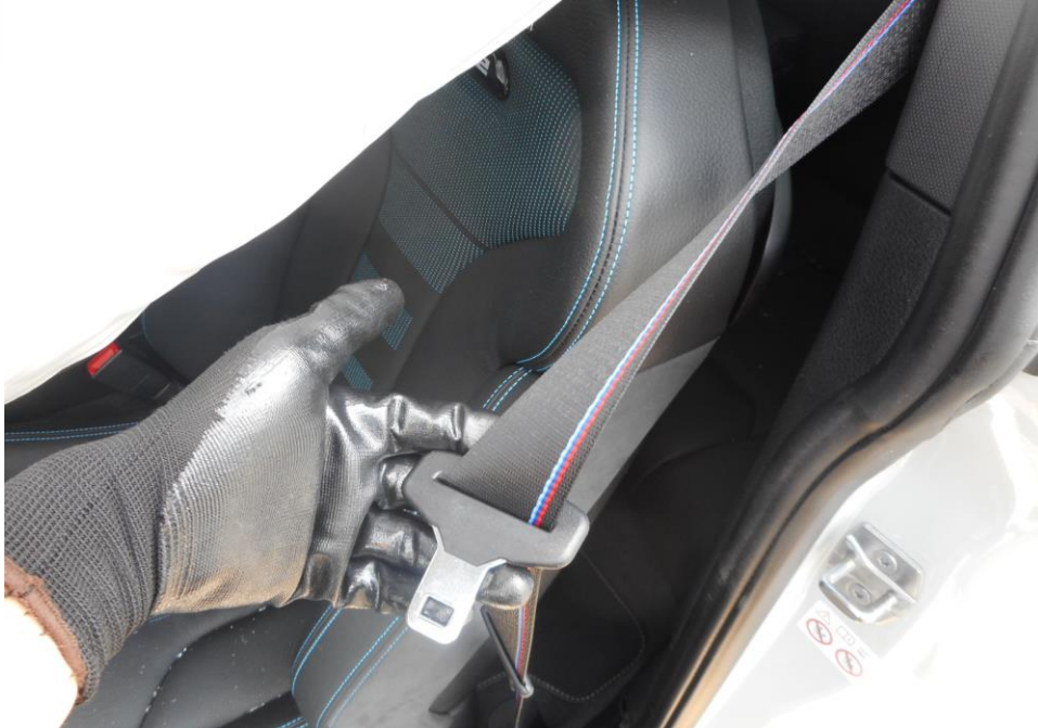
Photo 26 shows that the seat belt on the right seat was worn at the material time of accident as the safety pre-tensioners was activated at the moment of impact and caused the seat belts to be locked into the last position of the user.
