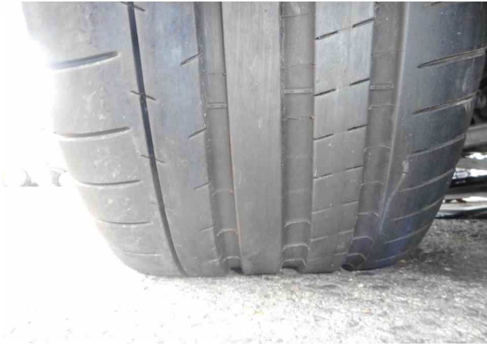
Photo 15 shows the condition of the front left tyre of the Motor Car, which was observed to be in serviceable condition with remaining tread depth of approximately 6.5mm. The tyre was also observed to be sufficiently inflated for vehicular operation with no tear, cut or burst mark(s).
