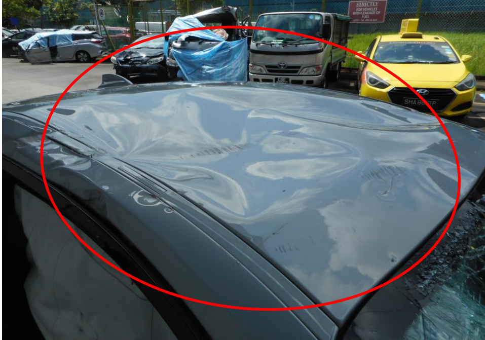
Photo 11 shows a close up view of the Motor Car's roof top at the time of my inspection. The Motor car was observed to have sustained damage at its roof portion. Its roof (red circle) was amongst the body parts damaged as a result of the accident.
