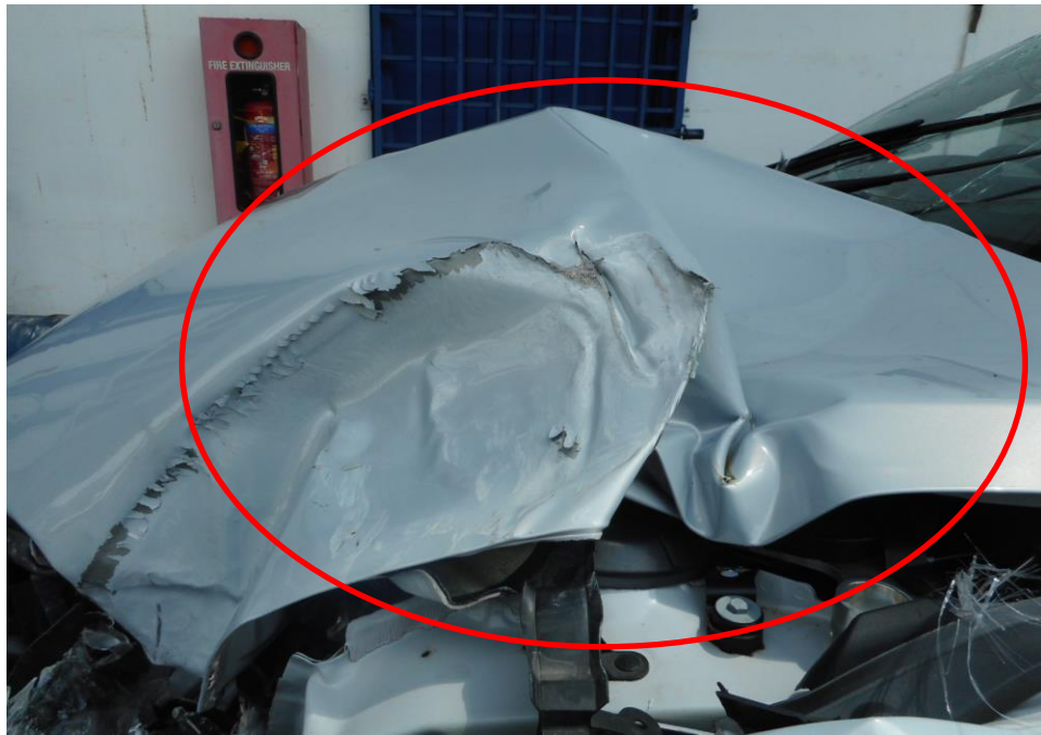
Photo 17 shows a close up view of the damaged front bonnet lock mechanism and the structure of the engine compartment of the Motor Car at the time of my inspection resulting it unable to open a result of the accident. (circled) (Unable to open)
