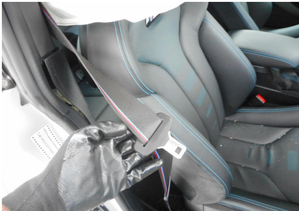
Photo 25 shows that the seat belt on the right seat was worn at the material time of accident as the safety pre-tensioners was activated at the moment of impact and caused the seat belts to be locked into the last position of the user.
