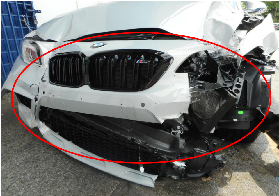
Photo 6 shows the close up view of the Motor Car's front body at the time of my inspection. The Motor car was observed to have sustained damage at its front portion. Its front bumper (red circle) was amongst the body parts and various components in the engine compartments were also damaged as a result of the accident.
