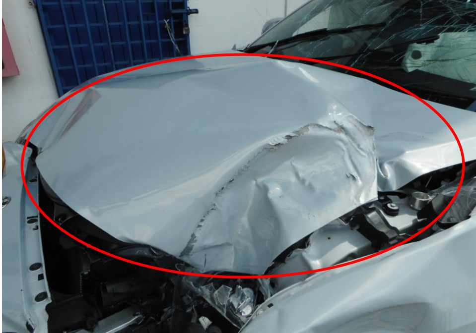
Photo 5 shows the close up view of the Motor Car's front body at the time of my inspection. The Motor car was observed to have sustained damage at its front portion. Its front bonnet (red circle) was amongst the body parts and various components were also damaged as a result of the accident.
