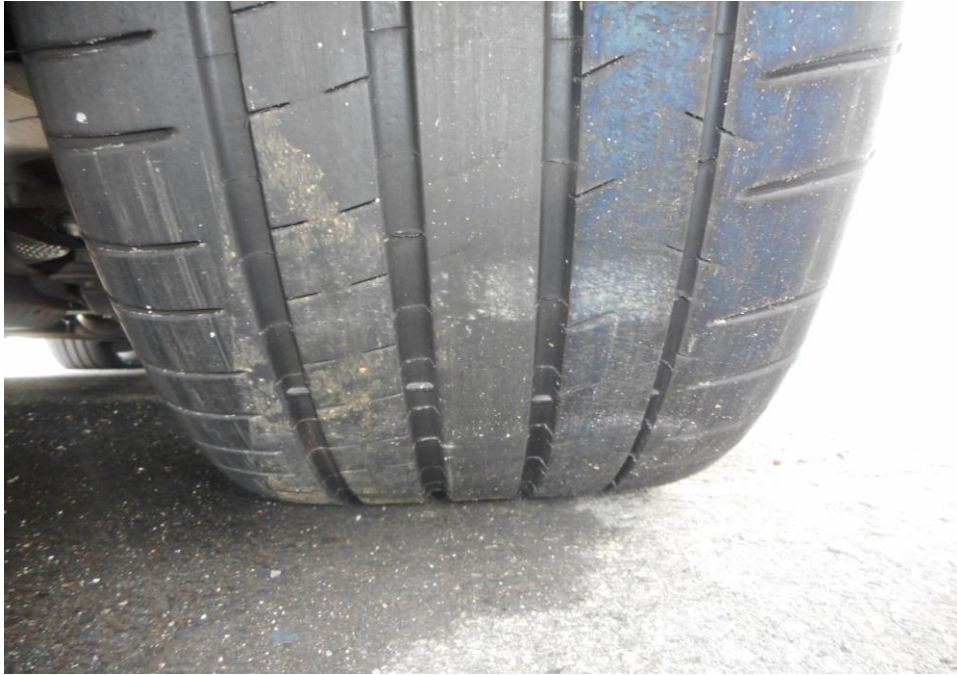
Photo 13 shows the condition of the rear right tyre of the Motor Car, which was observed to be in serviceable condition with remaining tread depth of approximately 5.9mm. The tyre was also observed to be sufficiently inflated for vehicular operation with no tear, cut or burst mark(s).
