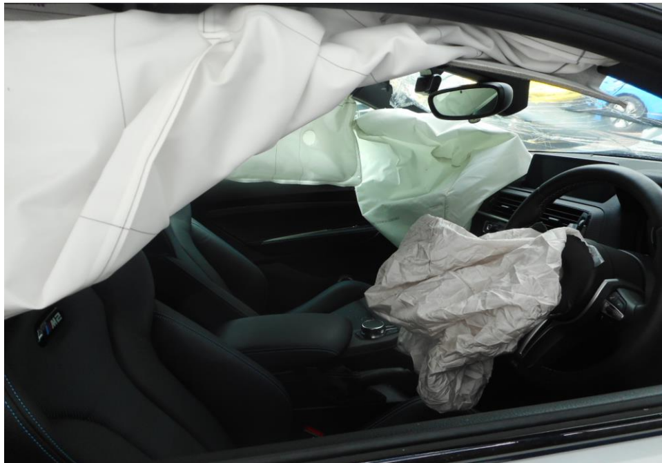
Photo 16 shows the deployment of the Supplemental Restraint System (SRS) airbag (arrowed) in the Motor Car as a result of the accident.
