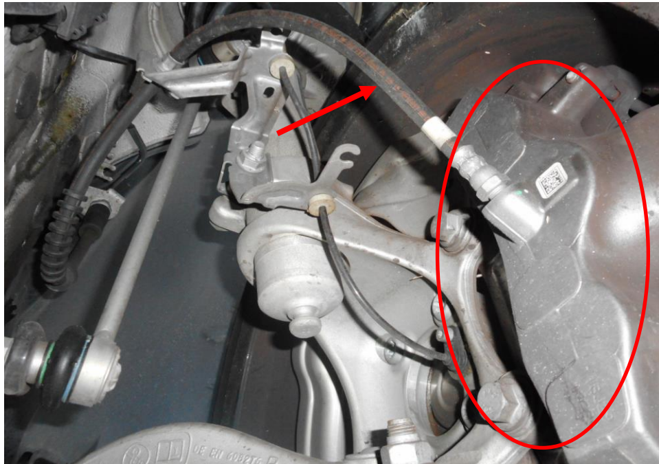
Photo 21 shows the brake hose/pipe (arrowed) at the front left wheel of the Motor Car. No leakage of brake fluid was observed. Visual examination of the various components of the braking system like the brake caliper (circled), brake booster, brake pedal etc had revealed all to be intact and without visible damage at the time of accident. There was also no sign of fluid stain(s) observed on the various undercarriage components.
