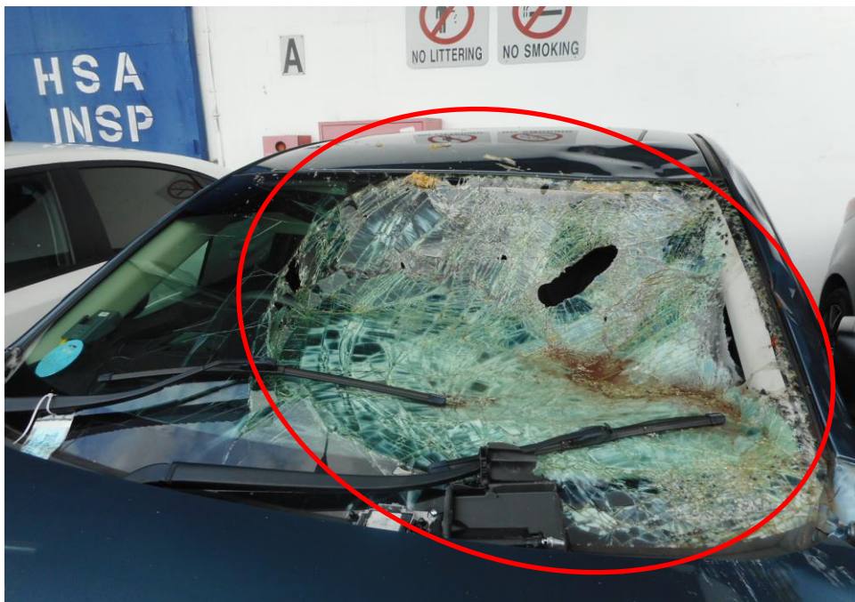
Photo 2 shows a general view of the Motor Car's front body at the time of my inspection. The Motor car was observed to have sustained damage at its front left portion. Its front windscreen (circled) was amongst the body parts and various components in the engine compartments were also damaged as a result of the accident.
