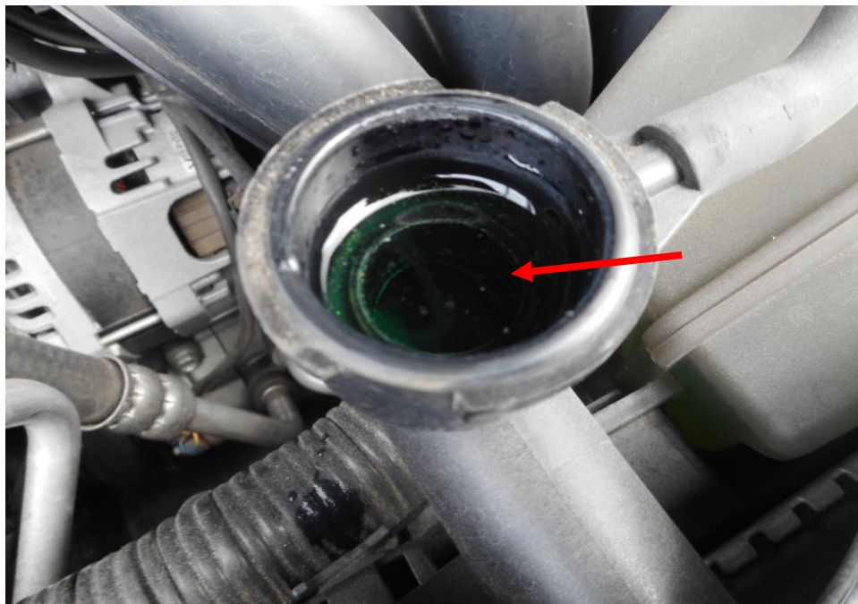
Photo 15 shows the engine coolant reservoir of the Motor Car at the time of my inspection. The engine coolant was observed to be of sufficient level (arrowed) and without any visible contamination.
