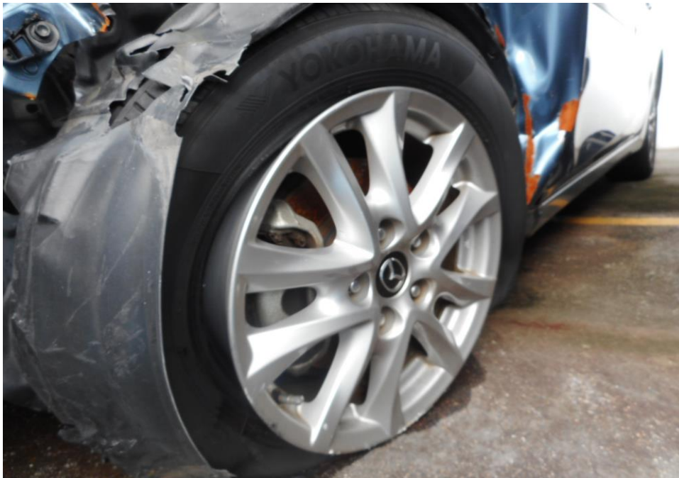
Photo 12 shows the condition of the front left tyre of the Motor Car, which was observed to be in unserviceable condition as the tyres had slipped off the rim as a result of the accident. The remaining tread depth of approximately 5.1mm. The tyre was also observed with no tear, cut or burst mark(s).
