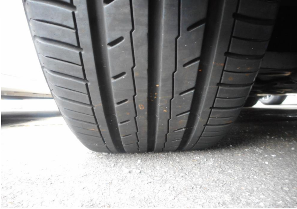
Photo 9 shows the condition of the front right tyre of the Motor Car, which was observed to be in serviceable condition with remaining tread depth of approximately 5.8mm. The tyre, which was wrapped around alloy wheel rim, was also observed to be sufficiently inflated for vehicular operation.
