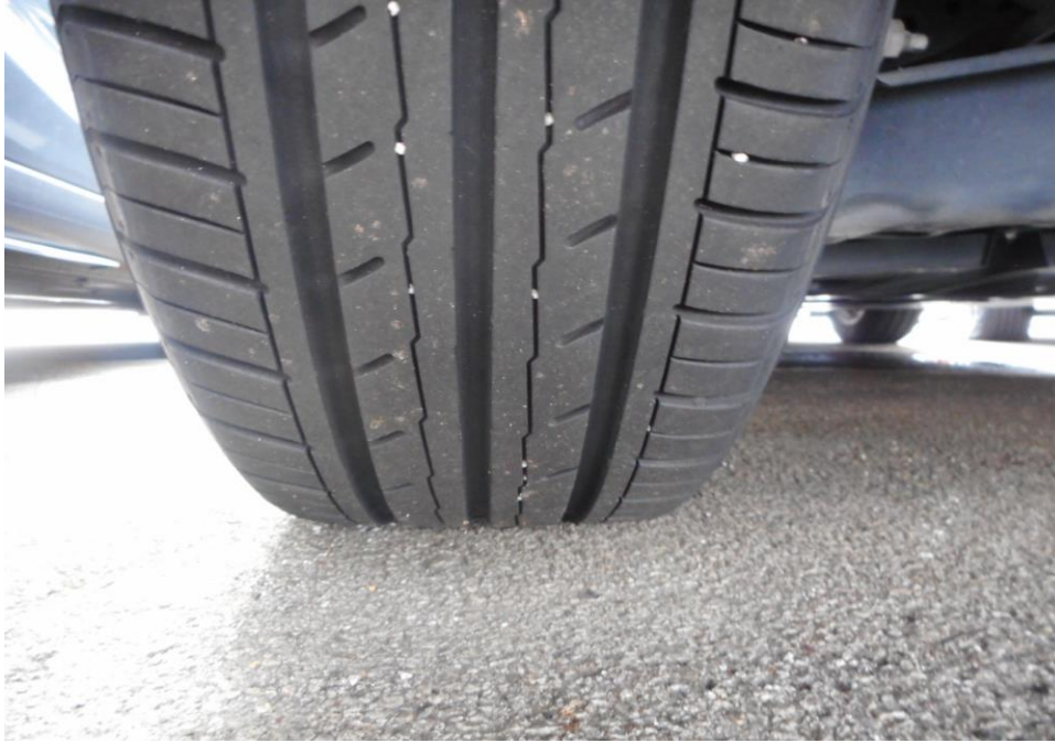
Photo 11 shows the condition of the rear left tyre of the Motor Car, which was observed to be in serviceable condition with remaining tread depth of approximately 5.4mm. The tyre was also observed to be sufficiently inflated for vehicular operation with no tear, cut or burst mark(s).
