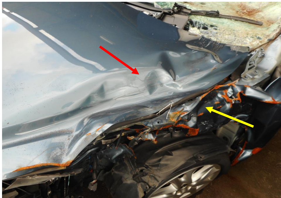
Photo 4 shows a close up view of the Motor Car's left portion at the time of my inspection. The Motor car was observed to have sustained damage at its front left portion. Its front bonnet (red arrow) and front left fender (yellow arrow) was amongst the body parts and various components in the engine compartments were also damaged as a result of the accident.
