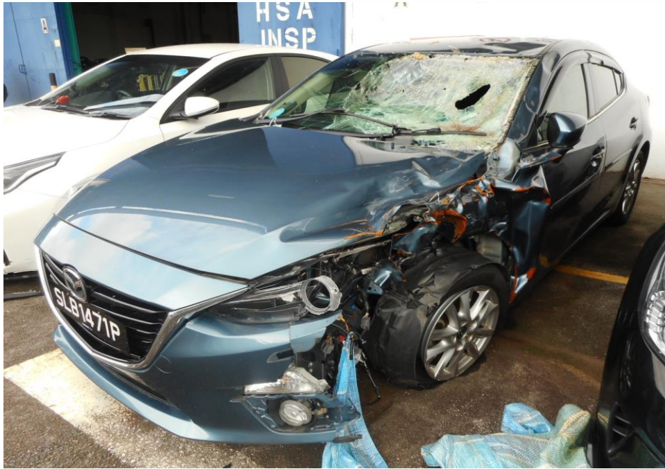
Photo 3 shows a general view of the Motor Car's left portion at the time of my inspection. The Motor car was observed to have sustained damage at its front left portion. Its front windscreen, front bonnet, front bumper, front left fender and front left headlamp was amongst the body parts and various components in the engine compartments were also damaged as a result of the accident.
