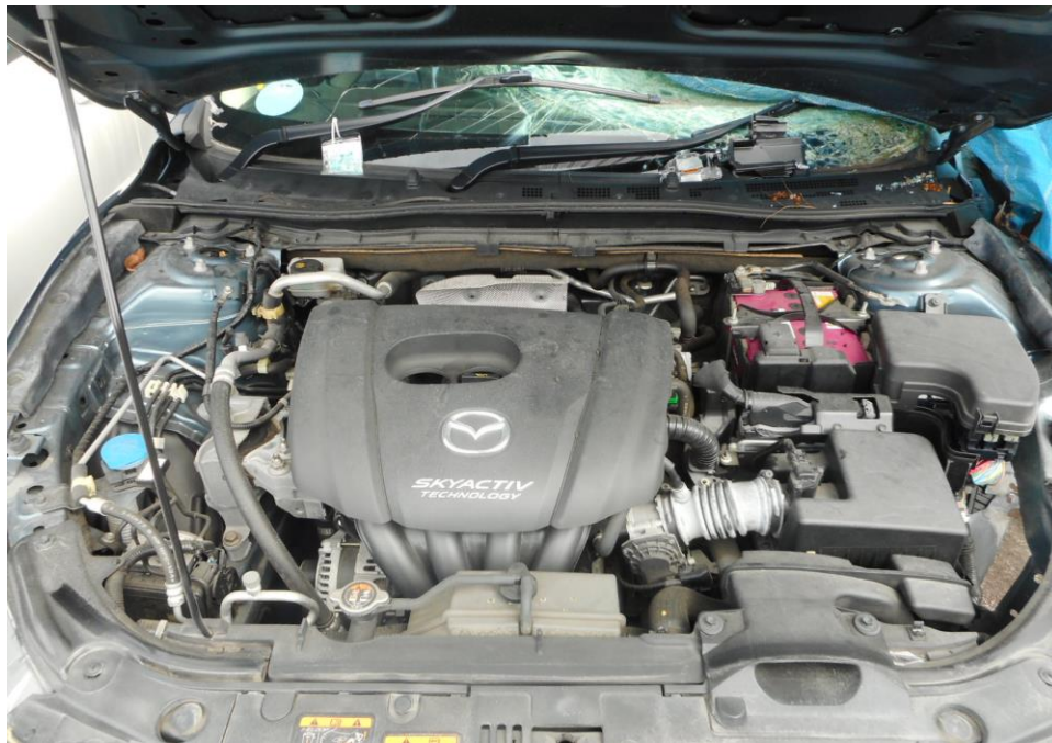
Photo 13 shows a general view of the Motor Car's engine compartment, which was accessed by lifting the front cabin of the Motor Car. The various parts and components inside the engine compartment were unaffected by the accident. There was also no sign(s) or indication(s) of fresh fluid leakage and/or fluid stain within the engine compartment
