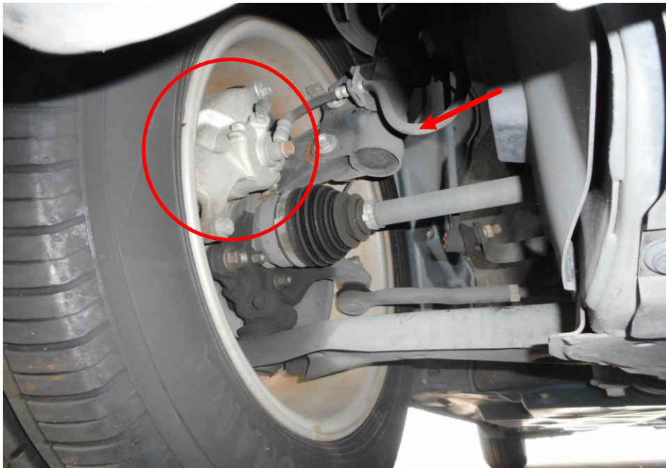
Photo 20 shows the brake hose/pipe (arrowed) at the front right wheel of the Motor Car. No leakage of brake fluid was observed. Visual examination of the various components of the braking system like the brake caliper (circled), brake booster, brake pedal etc. had revealed all to be intact and without visible damage at the time of accident. There was also no sign of fluid stain(s) observed on the various undercarriage components.
