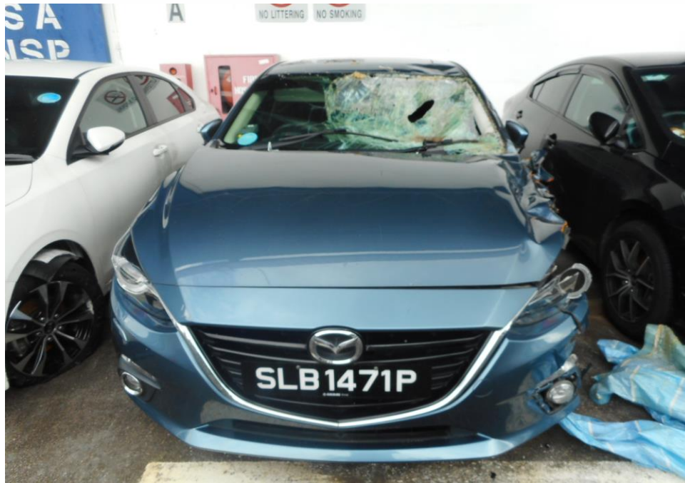
Photo 1 shows a general view of the Motor Car's front body at the time of my inspection. The Motor car was observed to have sustained damage at its front left portion. Its front windscreen, front bonnet, front bumper, front left fender and front left headlamp was amongst the body parts and various components in the engine compartments were also damaged as a result of the accident.
