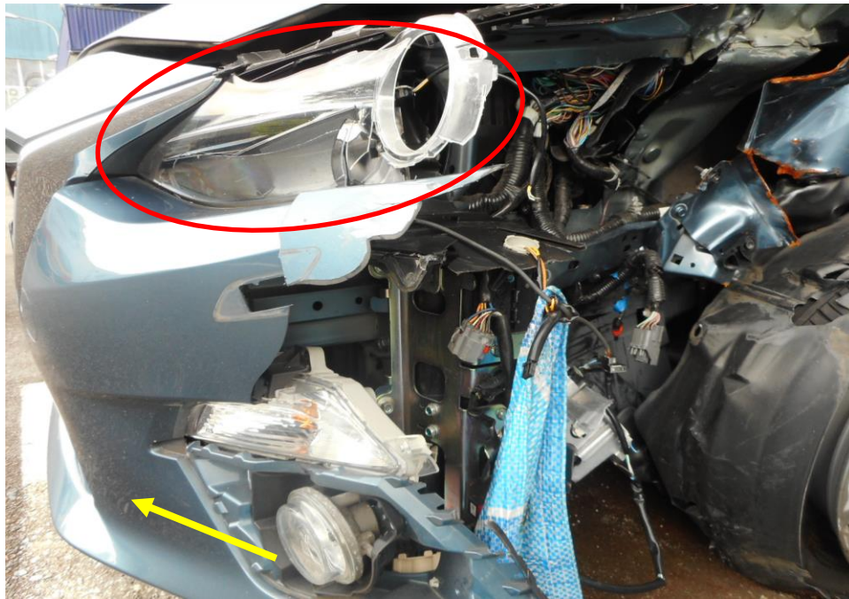
Photo 5 shows a close up view of the Motor Car's left portion at the time of my inspection. The Motor car was observed to have sustained damage at its front left portion. Its front bumper (arrowed) and front left headlamp (circled) was amongst the body parts and various components in the engine compartments were also damaged as a result of the accident.
